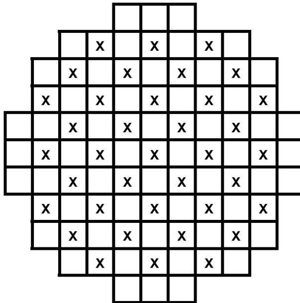
**Fig. 2 IRIS core configuration and a typical RCCA pattern**
