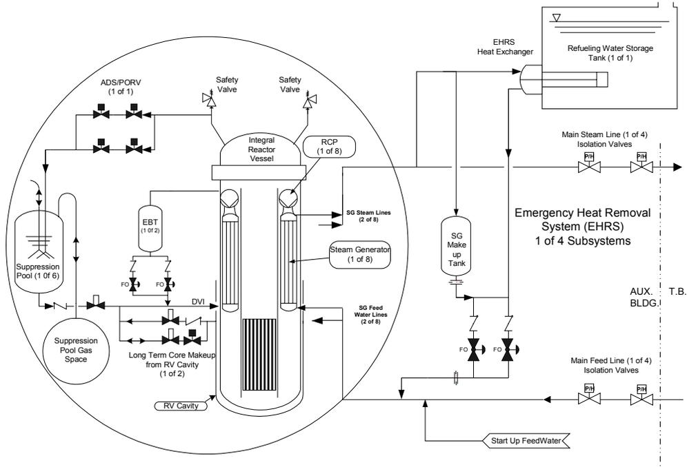
**Figure 5 Passive core and containment cooling system**
