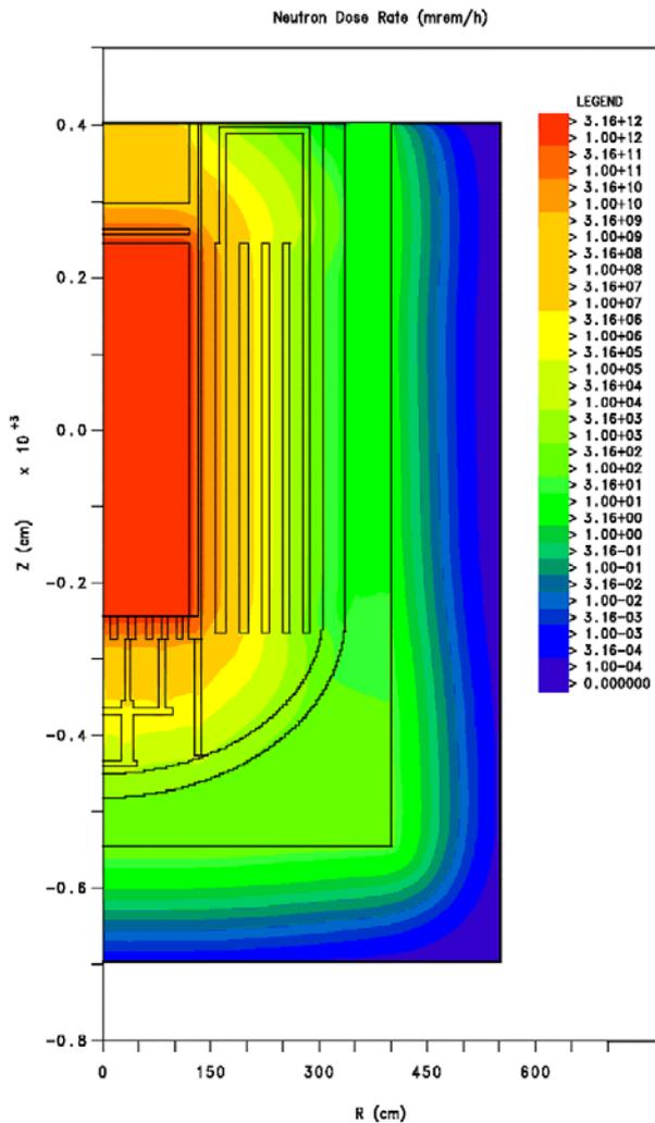
Figure 2.a Neutron dose rate in operation
