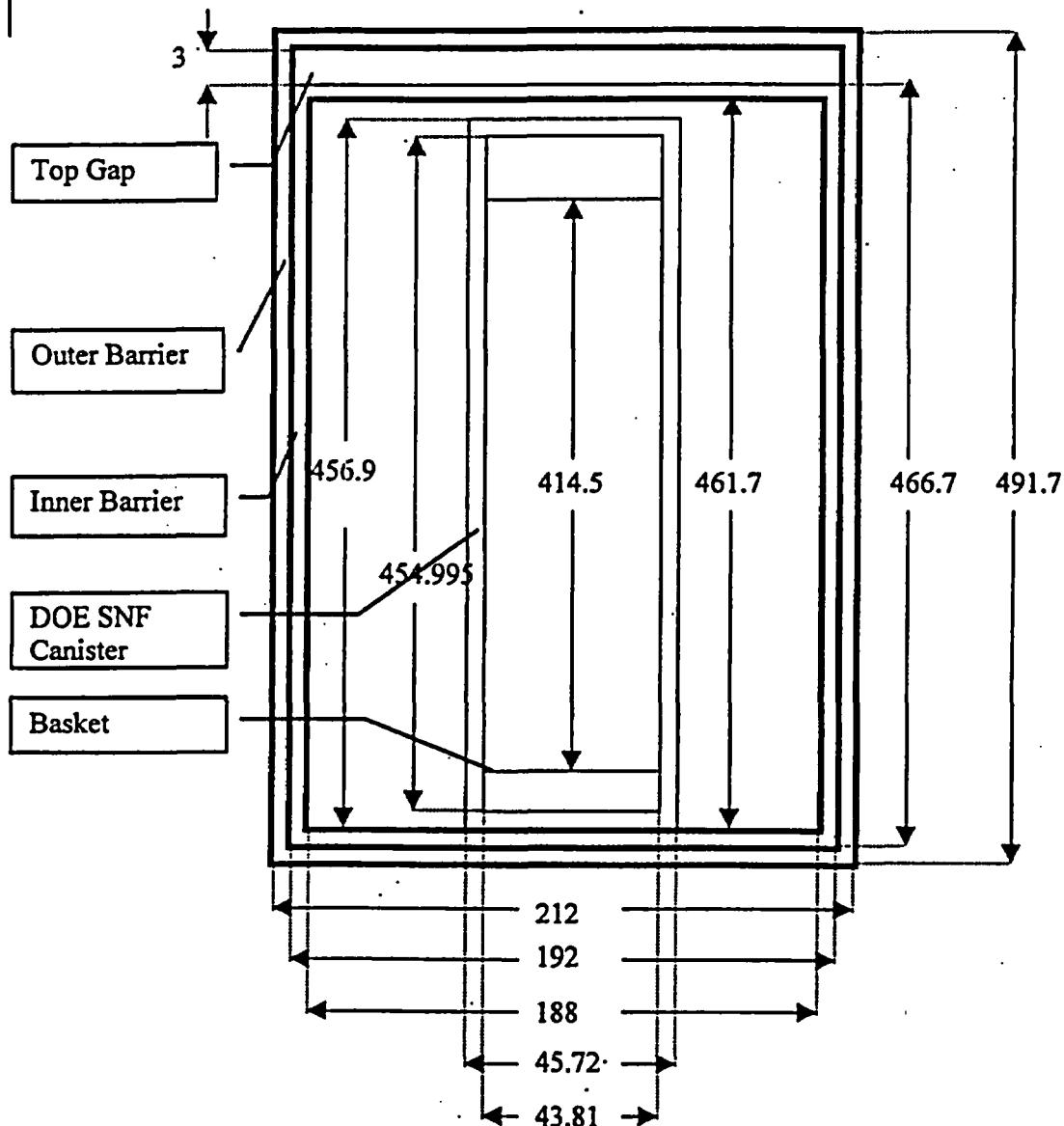
Figure 5.2-5. Dimensions of the WP and the DOE SNF Canister in cm (not to scale)
