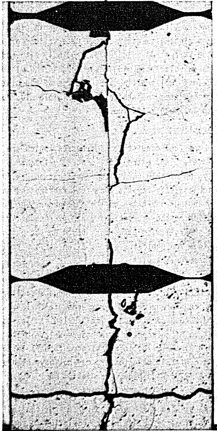
FIGURE 8.4. Photomicrograph of Polished Longitudinal Sample 104-MKP109-JJ from a Region at Approximately 72% of Peak Power ( \sim 10\times ) (Neg. No. 8704675-18) (Note: Photo taken at an oblique angle to fuel surface.)
