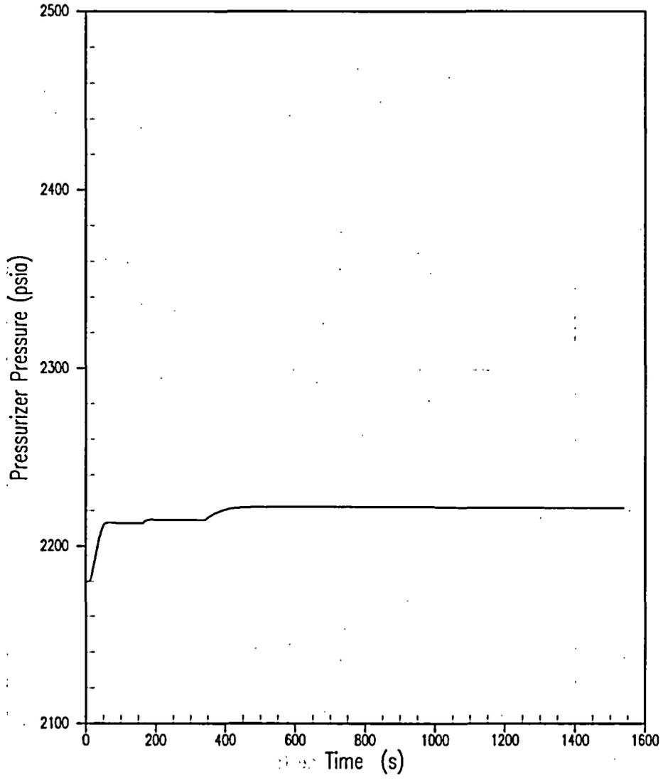
Figure 5.1.21-2 CVCS Malfunction at Power – Pressurizer Pressure
