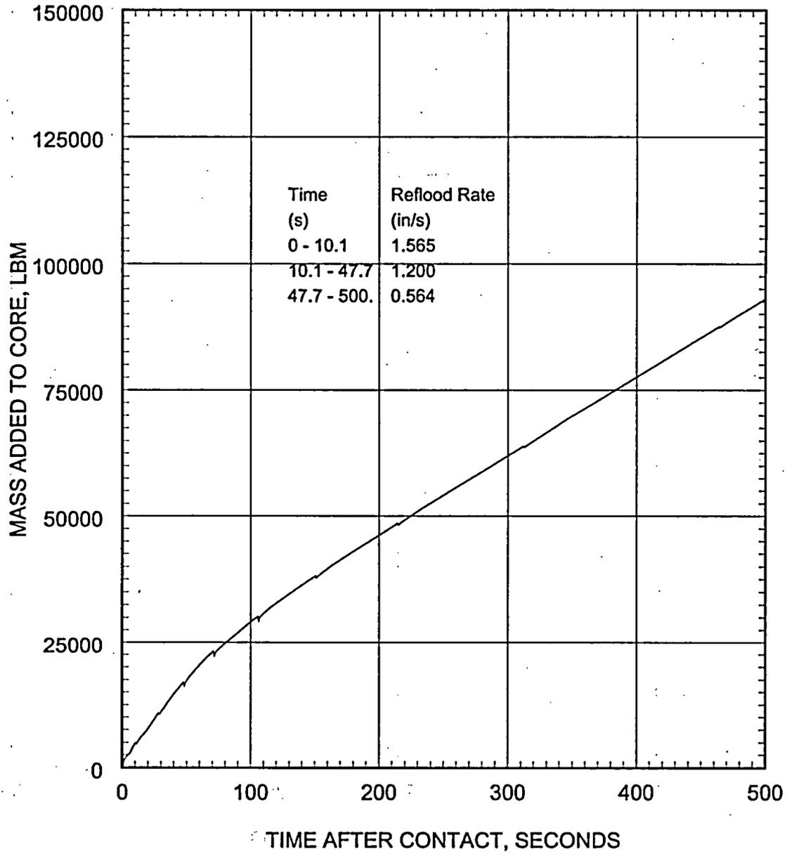
Figure 5.2.3.3-8 Large Break LOCA ECCS Performance Analysis 1.0 DEG/PD Break Mass Added to Core During Reflood
