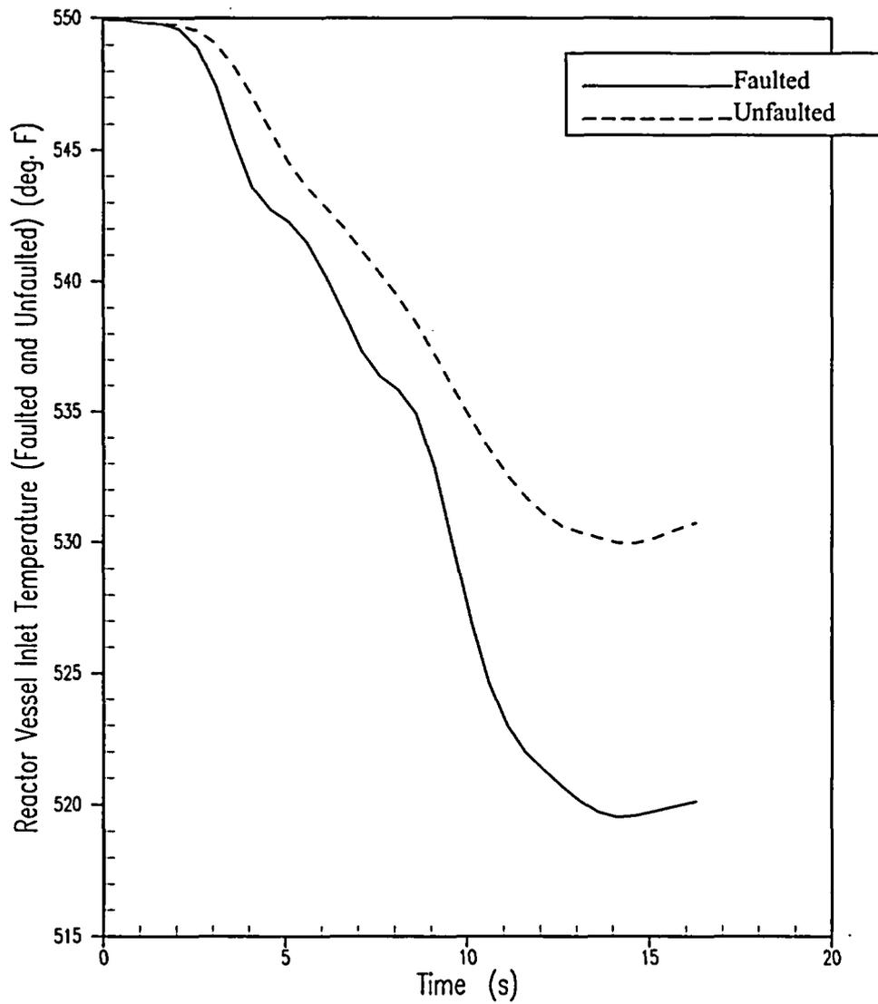
Figure 5.1.5-6 Pre-Trip Main Steamline Break – Reactor Vessel Inlet Temperature versus Time
