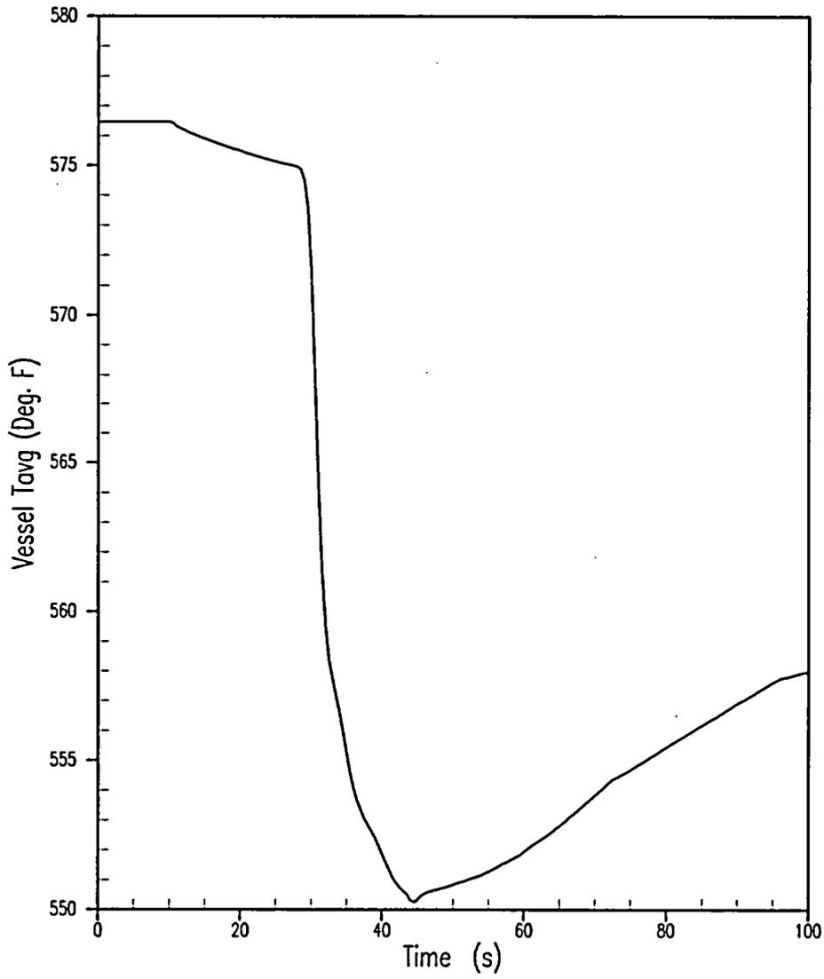
Figure 5.1.22-3 Vessel Tavg for an Accidental Depressurization of the Reactor Coolant System Event
