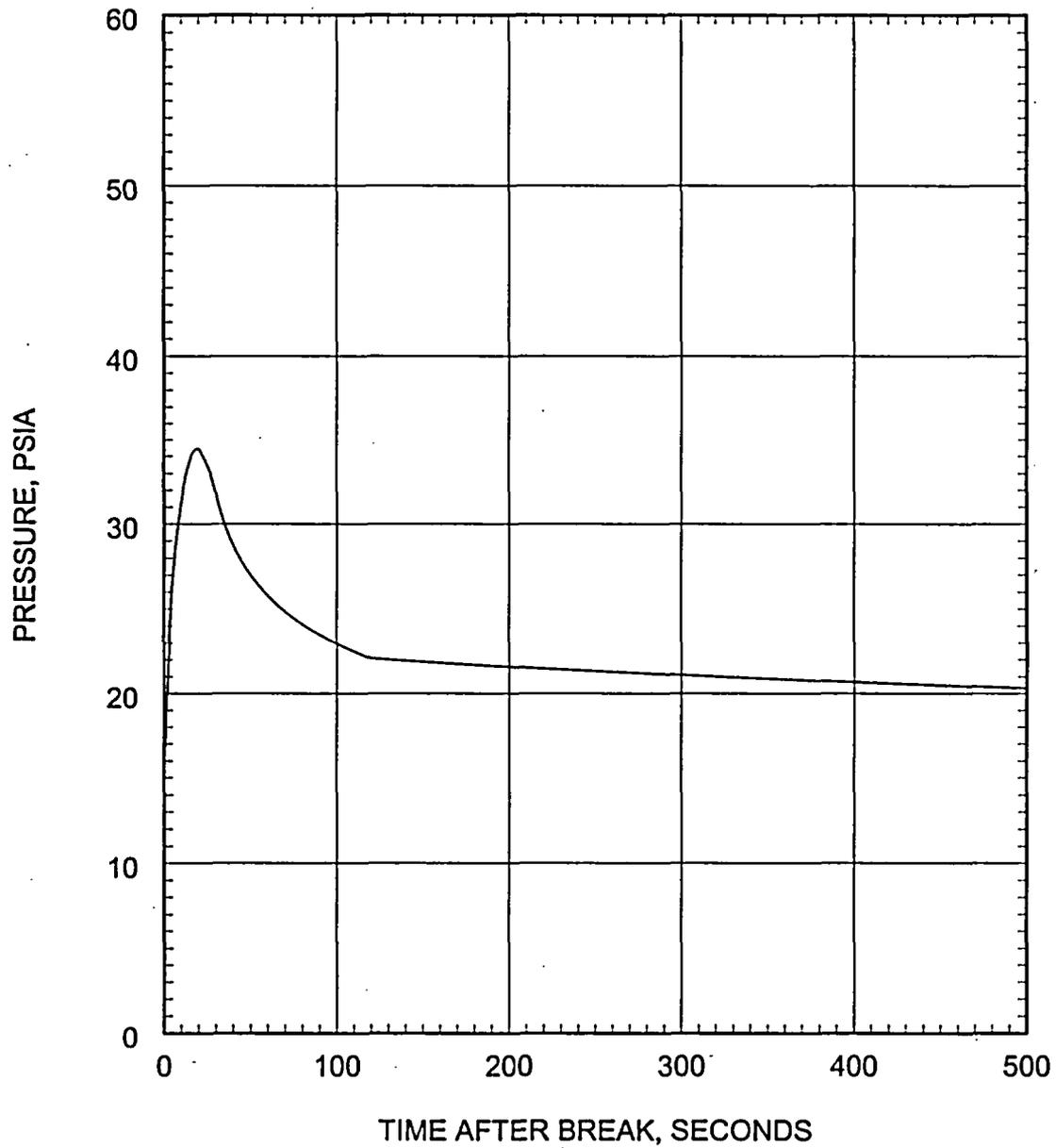
Figure 5.2.3.3-45 Large Break LOCA ECCS Performance Analysis 0.4 DEG/PD Break
