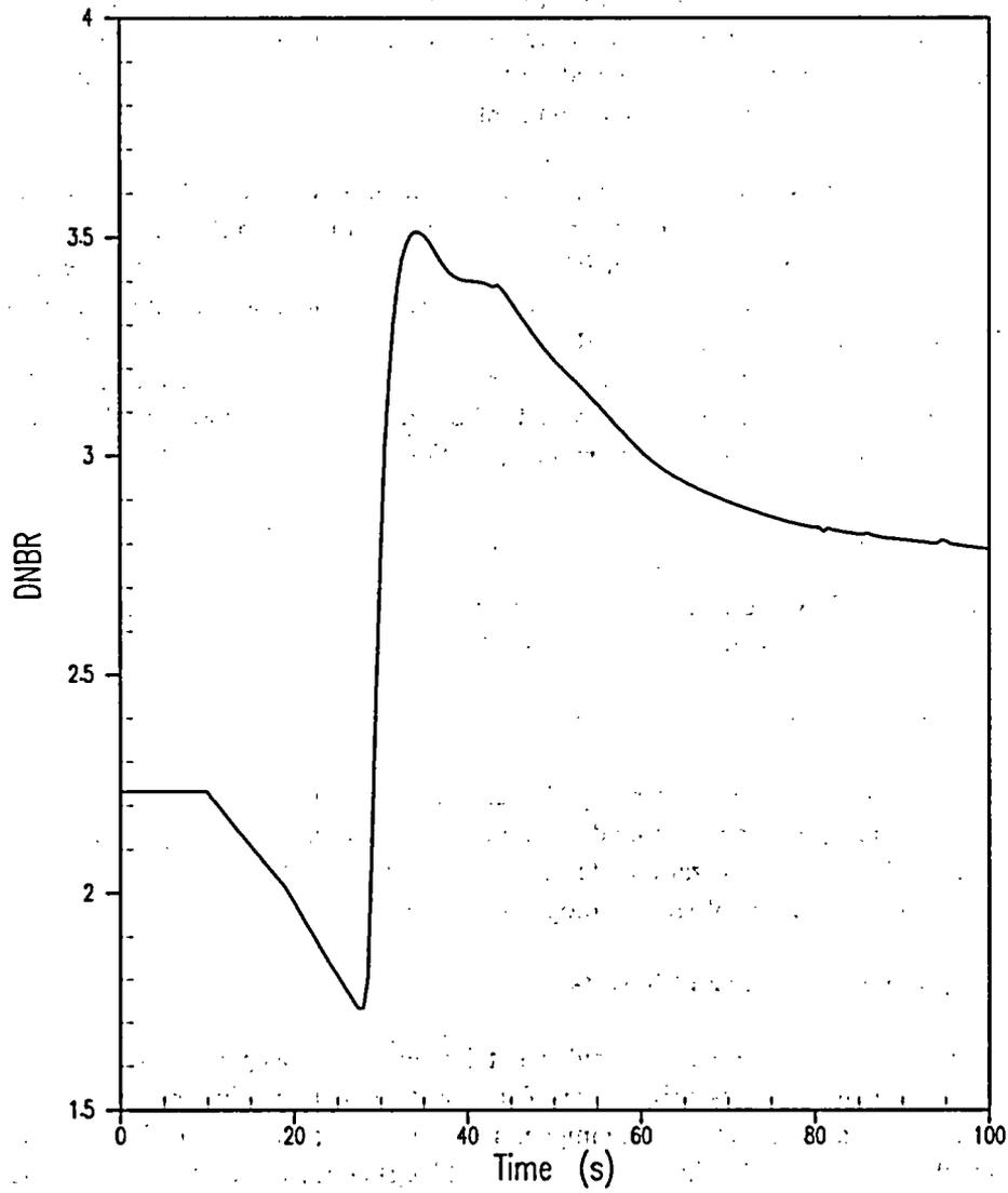
**Figure 5.1.22-4 DNBR for an Accidental Depressurization of the Reactor Coolant System Event**
