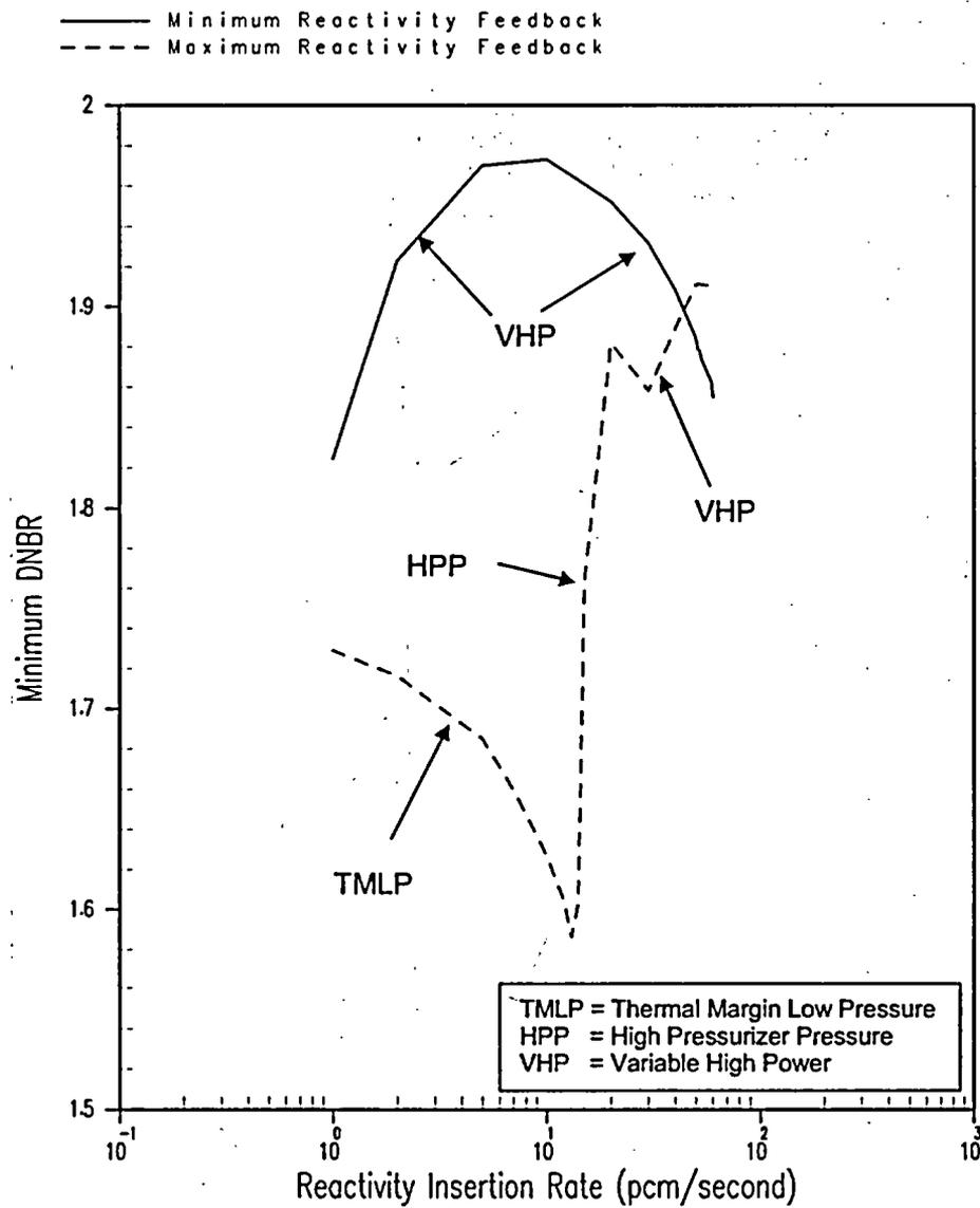
Figure 5.1.16-3 Uncontrolled CEA Bank Withdrawal at Power Initial Power Level of 100% (Sheet 1 of 4)
