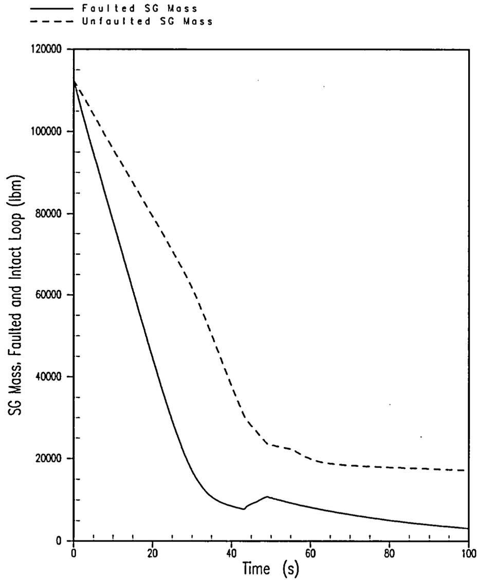
Figure 5.1.12-19 Feedwater Line Break DNB Case Limiting Break Size = 0.25 ft<sup>2</sup> SG Mass, Faulted and Intact Loop
