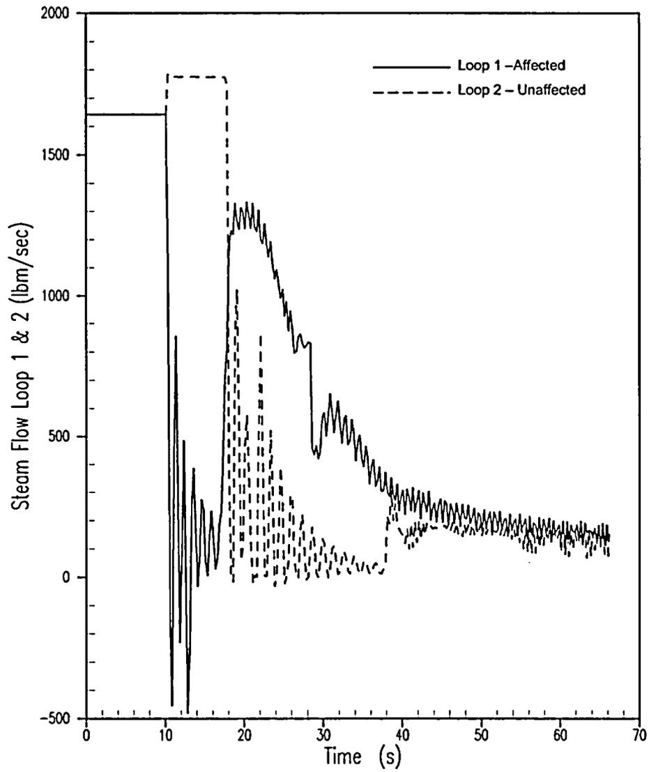
Figure 5.1.11-19 Steam Flow for Asymmetric Steam Generator Transient 30% Tube Plugging
