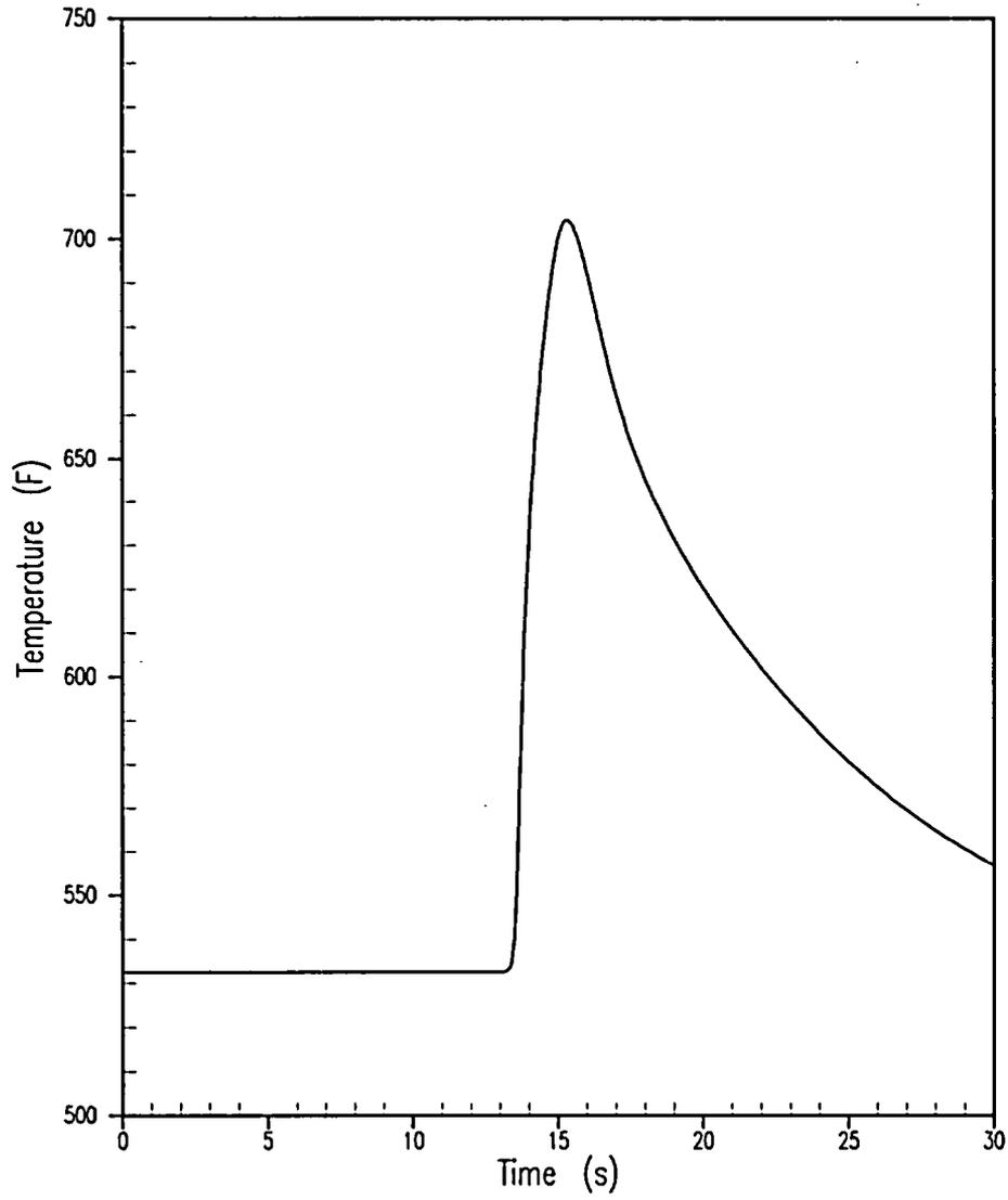
**Figure 5.1.17-5 Uncontrolled CEA Withdrawal from a Subcritical Condition – Hot Spot Cladding Temperature versus Time**
