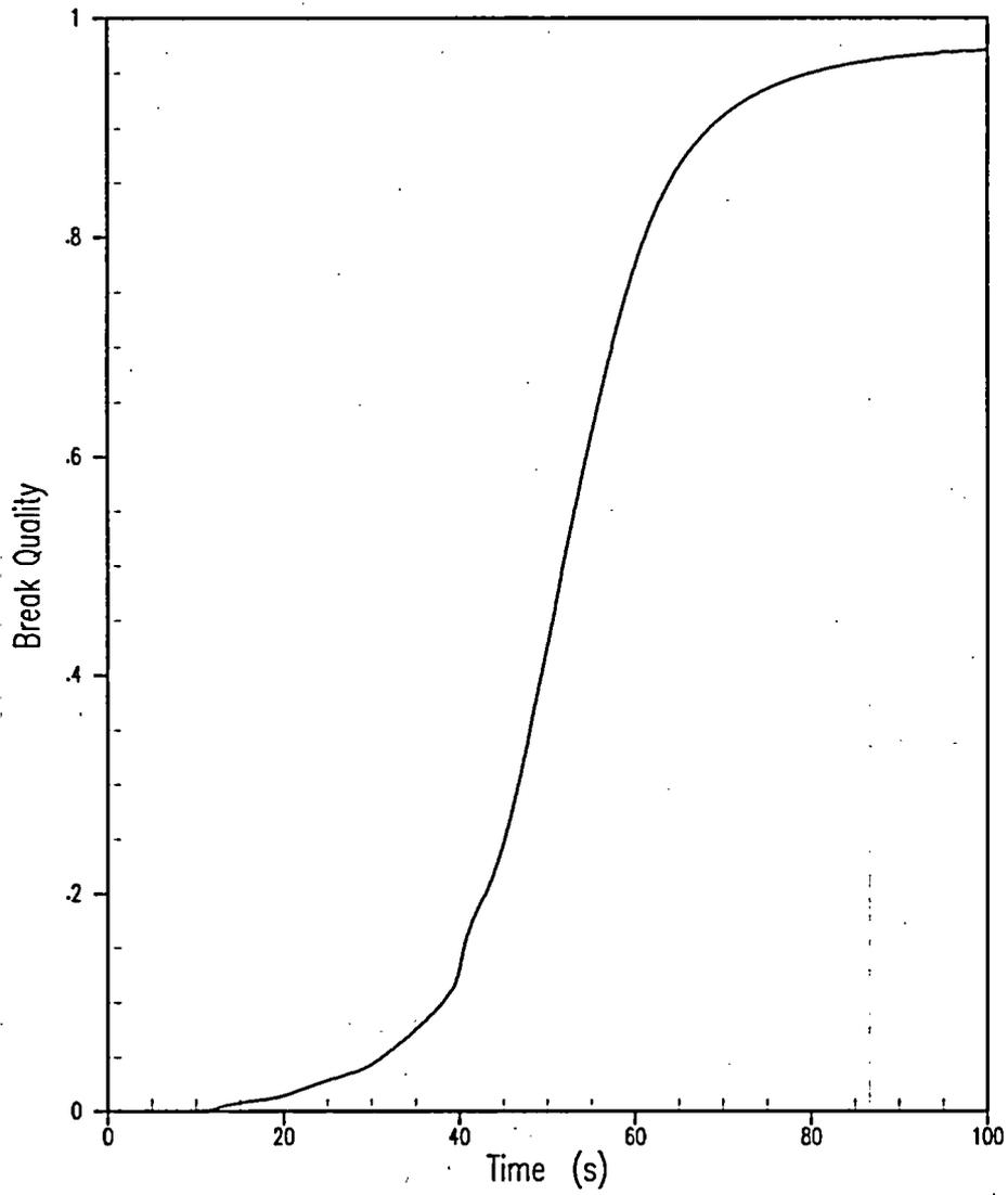
**Figure 5.1.12-14 Feedwater Line Break MSS Overpressure Case Limiting Break Size = 0.05 ft<sup>2</sup>
