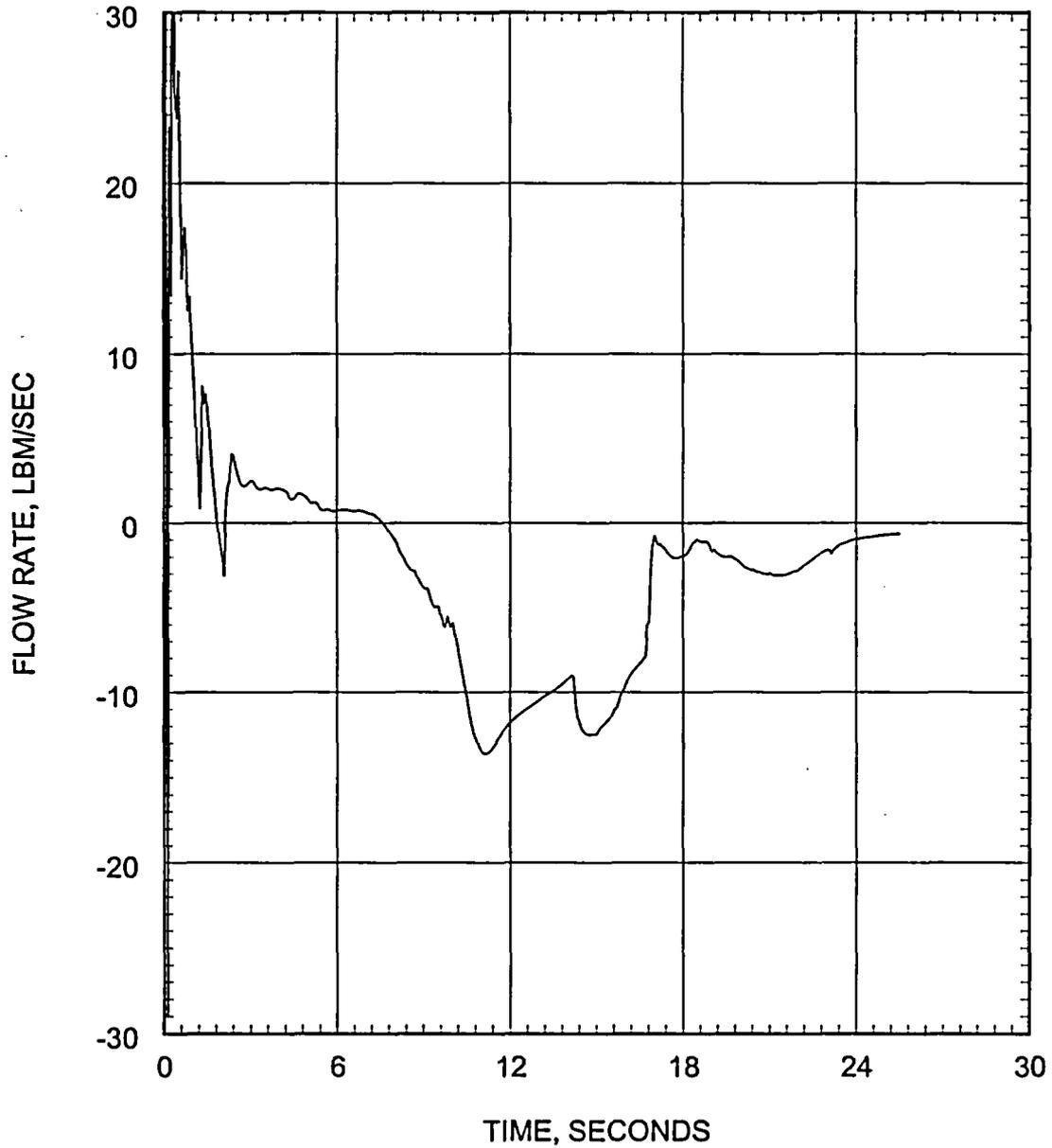
Figure 5.2.3.3-23 Large Break LOCA ECCS Performance Analysis 0.6 DEG/PD Break Hot Assembly Flow Rate (Above Hot Spot)
