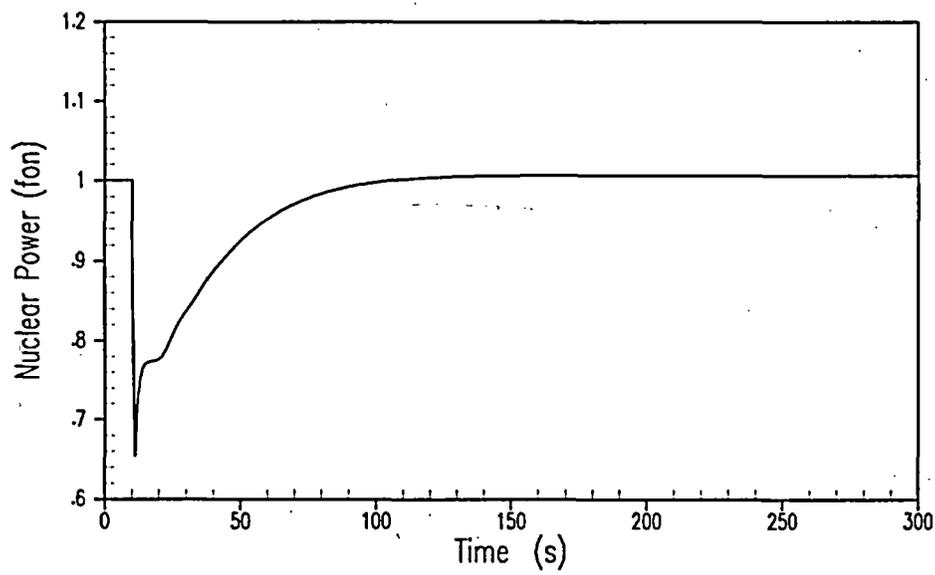
**Figure 5.1.18-5 Representative Transient Response to a Dropped CEA Worth of 500 pcm at a Moderator Temperature Coefficient of -25 pcm/°F – Nuclear Power versus Time**
