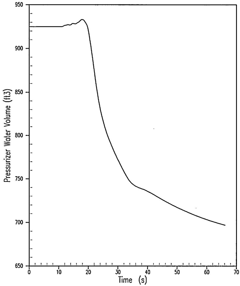
**Figure 5.1.11-3 Pressurizer Water Volume for Asymmetric Steam Generator Transient 0% Tube Plugging**
