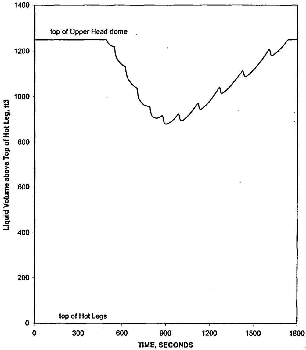
**Figure 5.1.24-11 Steam Generator Tube Rupture with Loss of Offsite Power – Liquid Volume Above Top of Hot Leg vs. Time**
