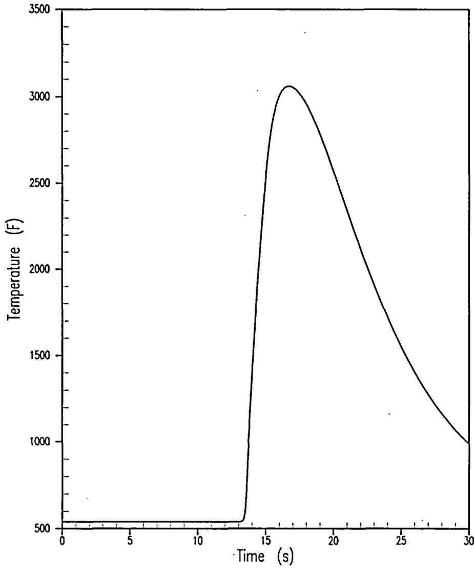
**Figure 5.1.17-3 Uncontrolled CEA Withdrawal from a Subcritical Condition – Hot Spot Fuel Centerline Temperature versus Time**
