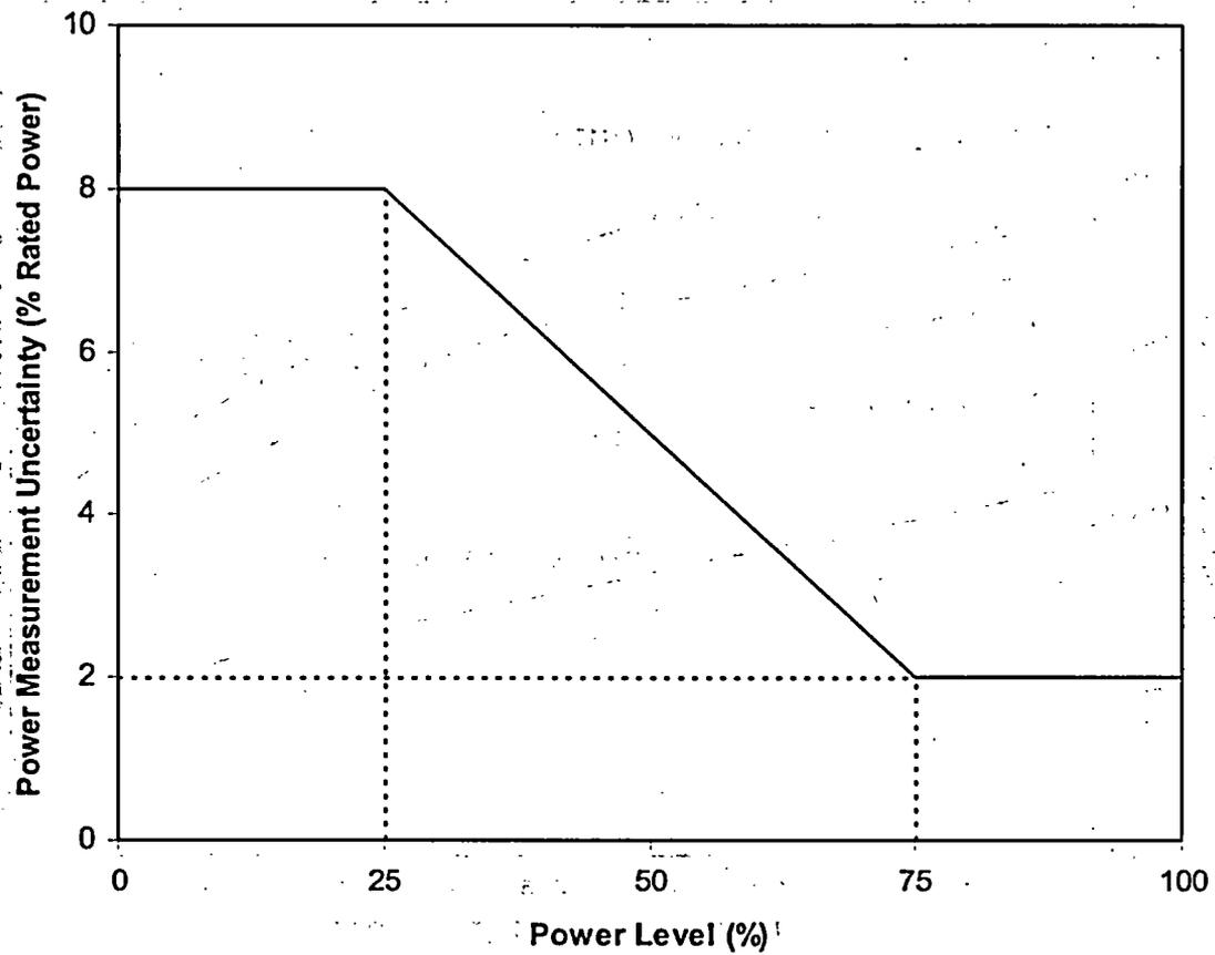
Figure 5.1.0-1 Power Measurement Uncertainty Used in Accident Analysis
