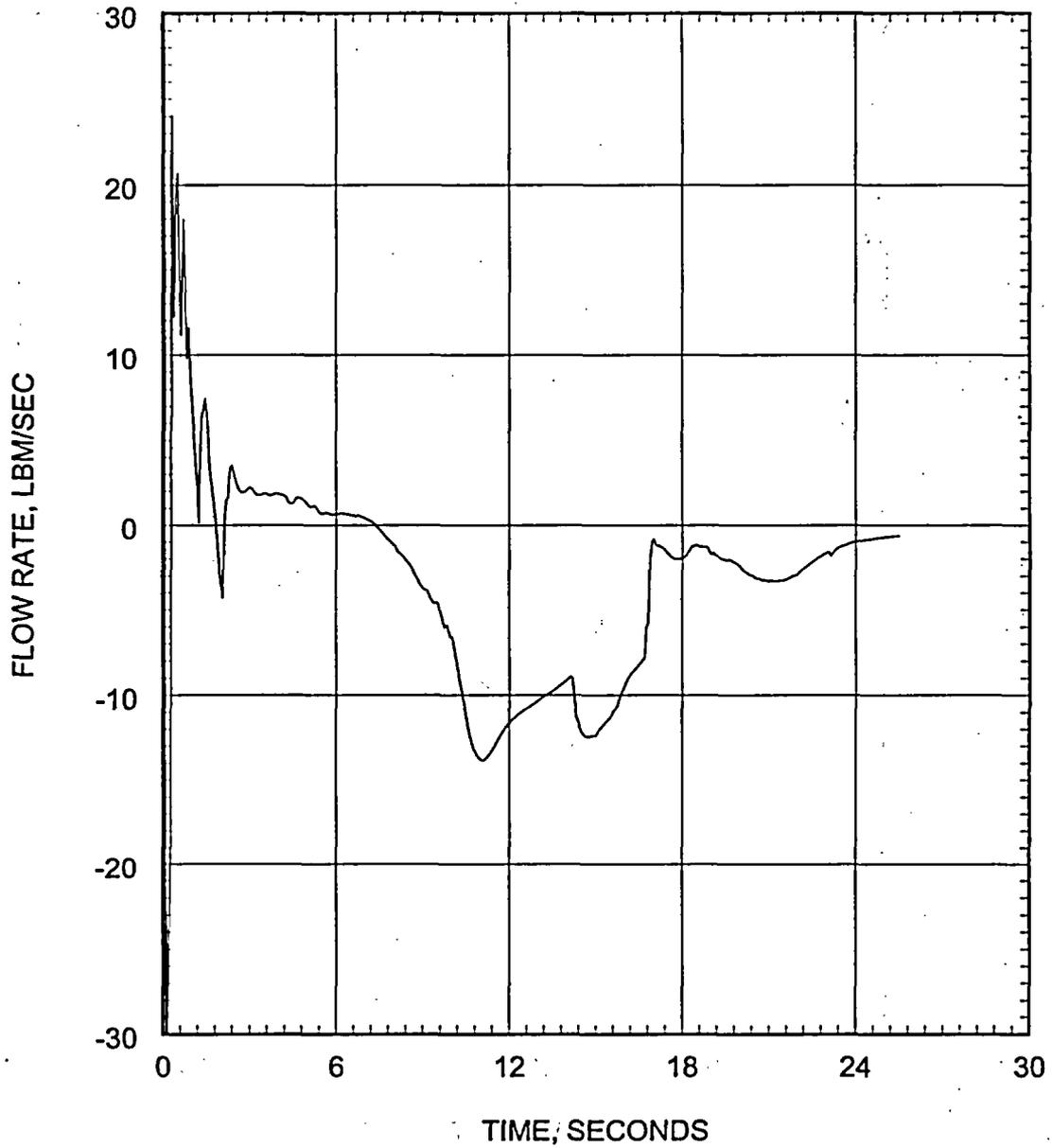
Figure 5.2.3.3-22 Large Break LOCA ECCS Performance Analysis 0.6 DEG/PD Break Hot Assembly Flow Rate (Below Hot Spot)
