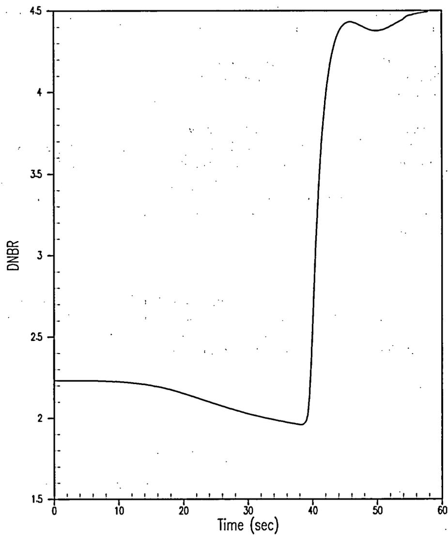
**Figure 5.1.3-7 DNBR for a Feedwater Malfunction Reduced Feedwater Temperature at HFP Initial Conditions**
