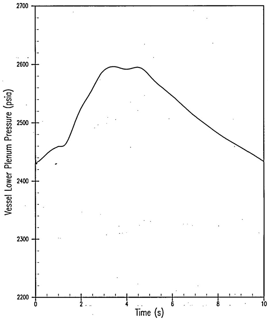
Figure 5.1.15-6 Vessel Lower Plenum Pressure versus Time – Locked Rotor/Shaft
