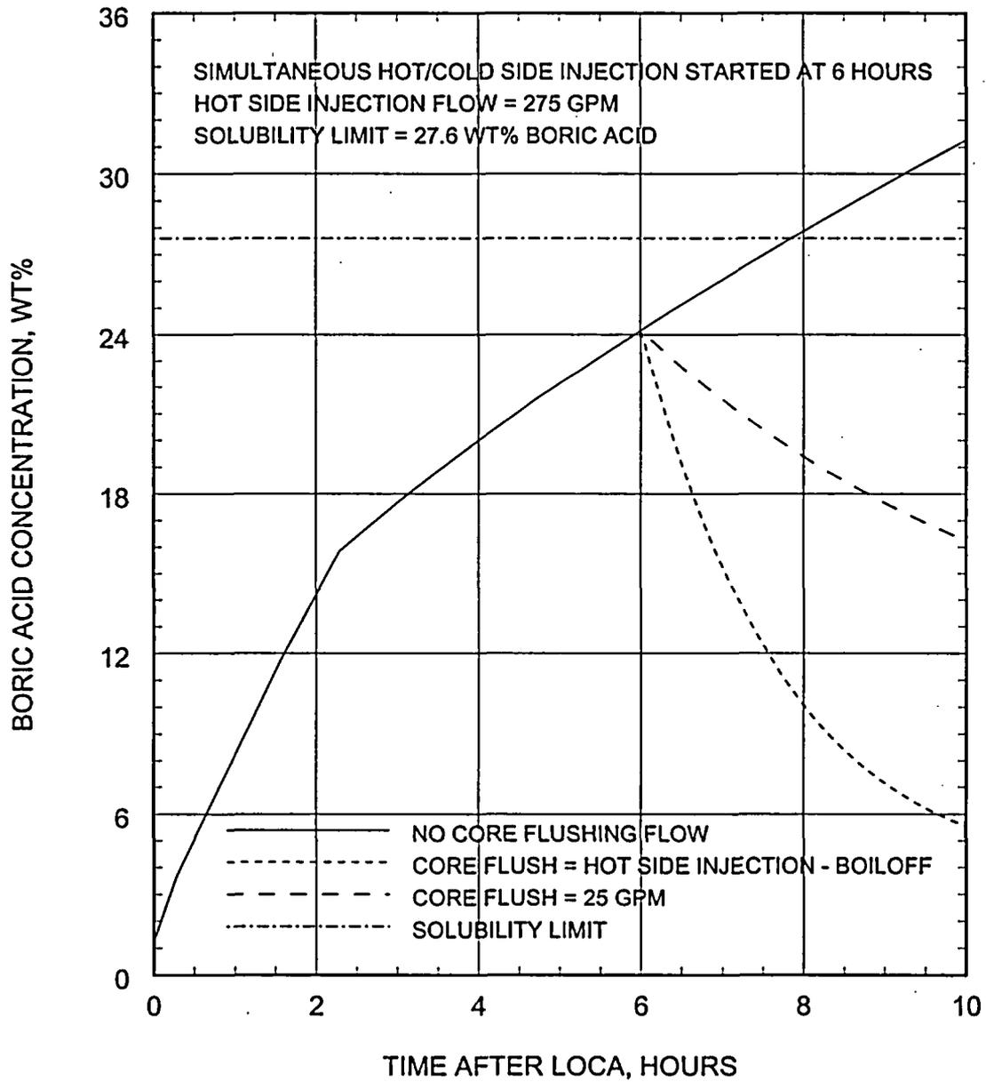
Figure 5.2.5.3-2 Long-Term Cooling Analysis Boric Acid Concentration in the Core Versus Time
