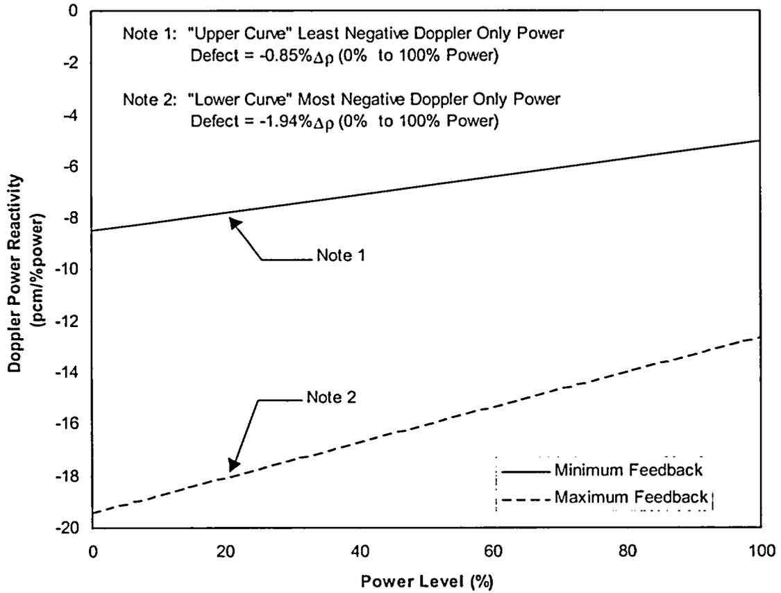
Figure 5.1.0-6 Doppler Power Coefficient Used in Accident Analyses
