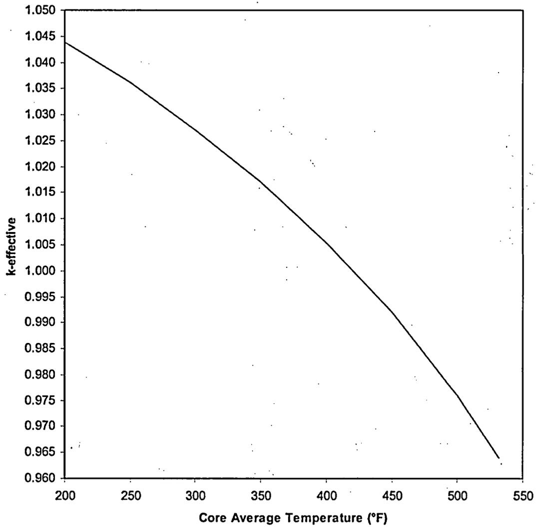
Figure 5.1.6-1 Variation of  $K_{\text{eff}}$  with Core Temperature (3.6 % $\Delta k$  SDM, 900 psia)
