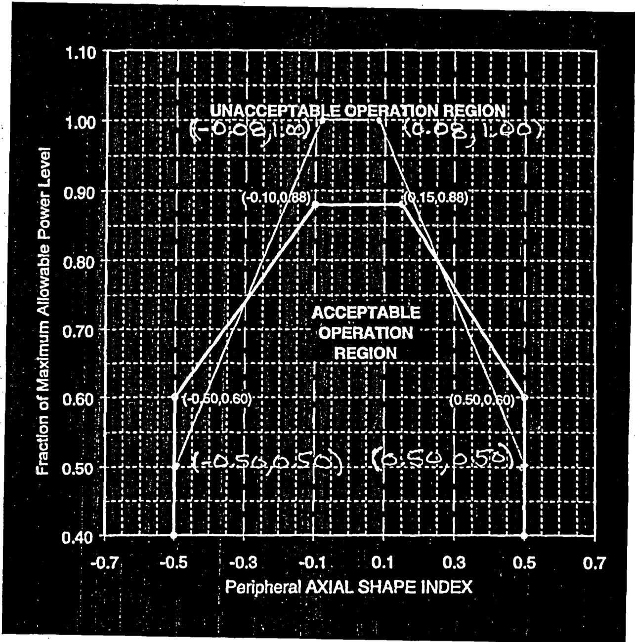
Figure A-1 Proposed AXIAL SHAPE INDEX Limits for Linear Heat Rate when Using Excure Detector Monitoring System (COLR Figure 3.2.2)
