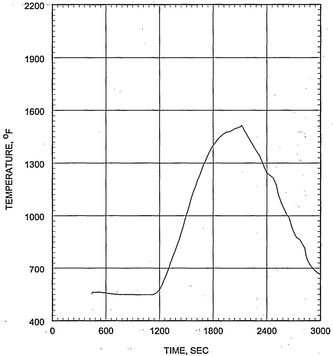
Figure 5.2.4.3-7 : Small Break LOCA ECCS Performance Analysis 0.04 ft<sup>2</sup>/PD Break Coolant Temperature at Hot Spot
