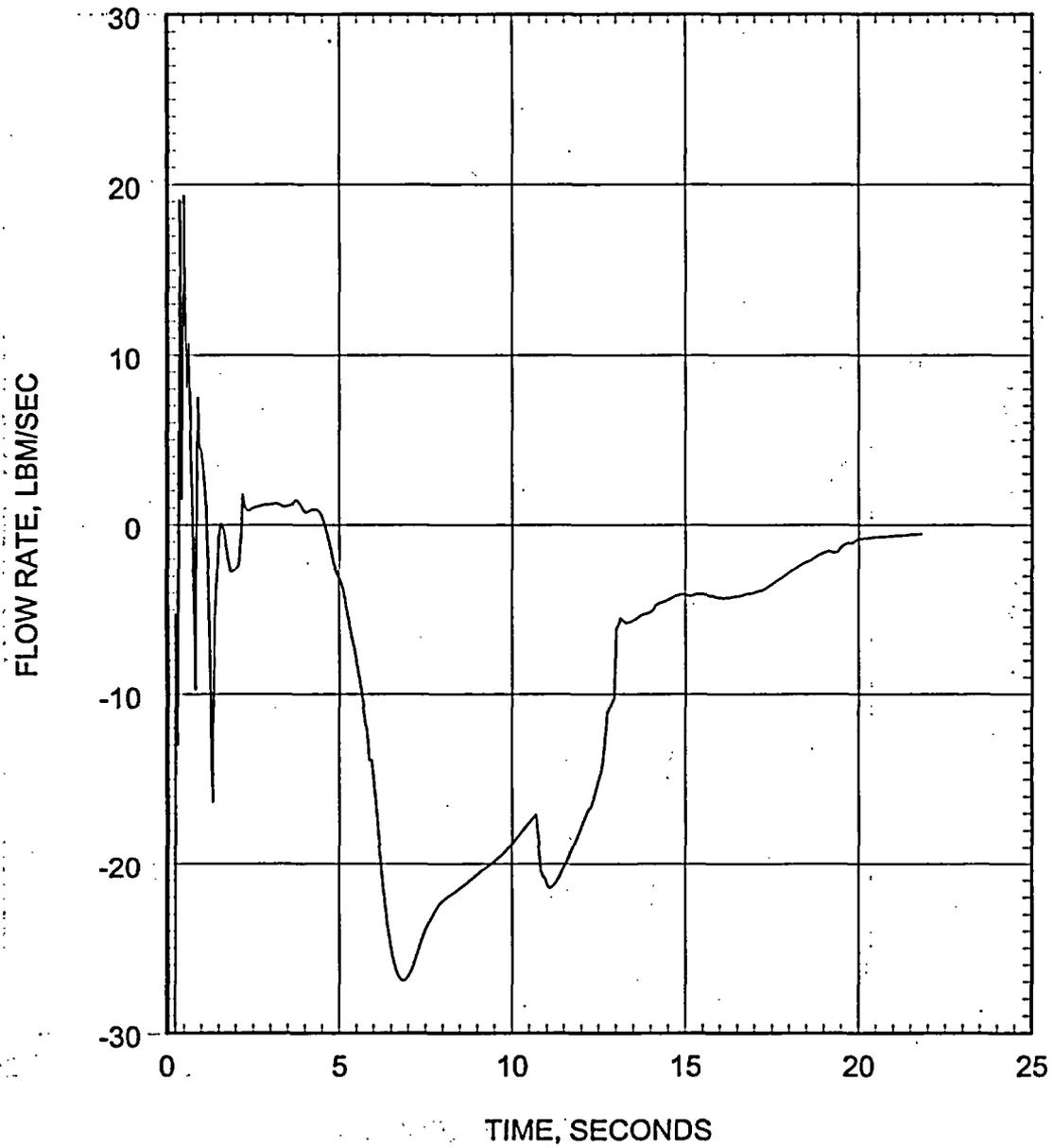
Figure 5.2.3.3-4 Large Break LOCA ECCS Performance Analysis 1.0 DEG/PD Break Hot Assembly Flow Rate (Below Hot Spot)
