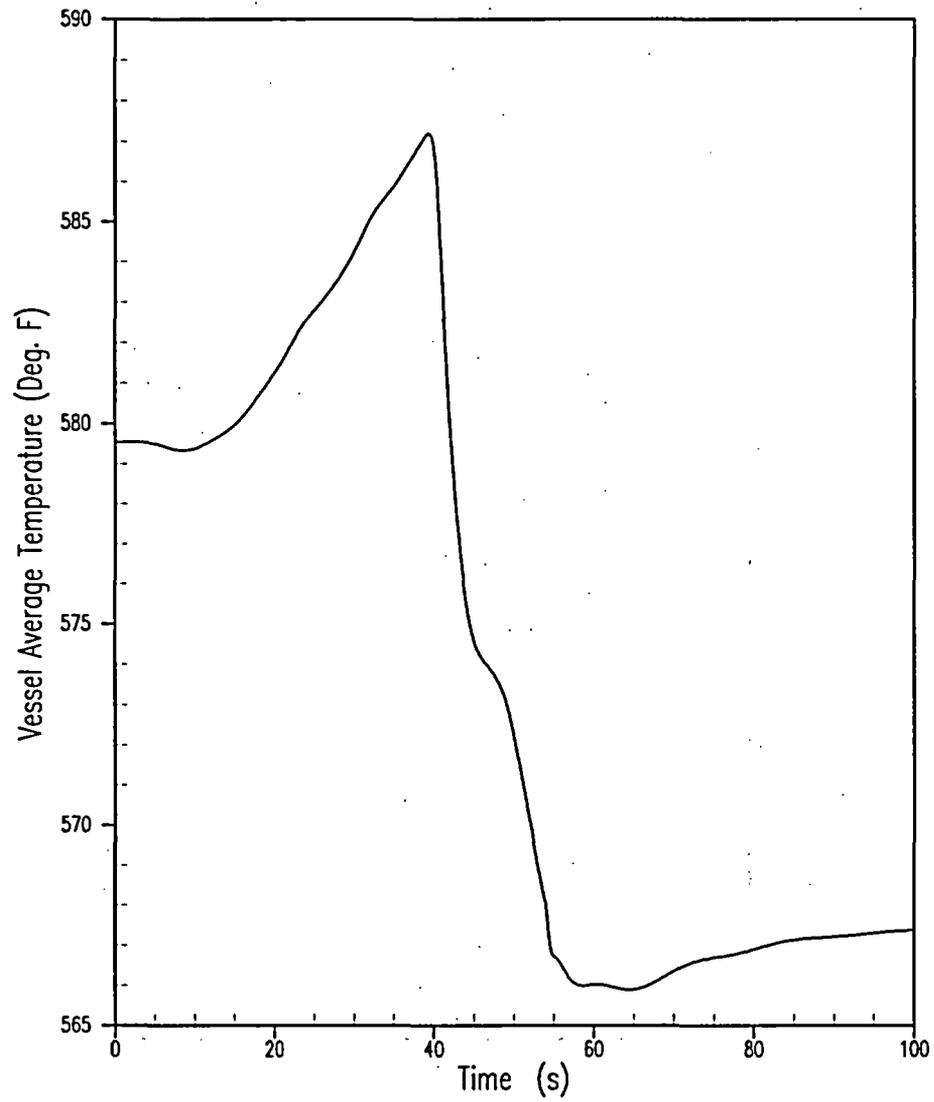
**Figure 5.1.12-10 Feedwater Line Break MSS Overpressure Case Limiting Break Size = 0.05 ft<sup>2</sup>
