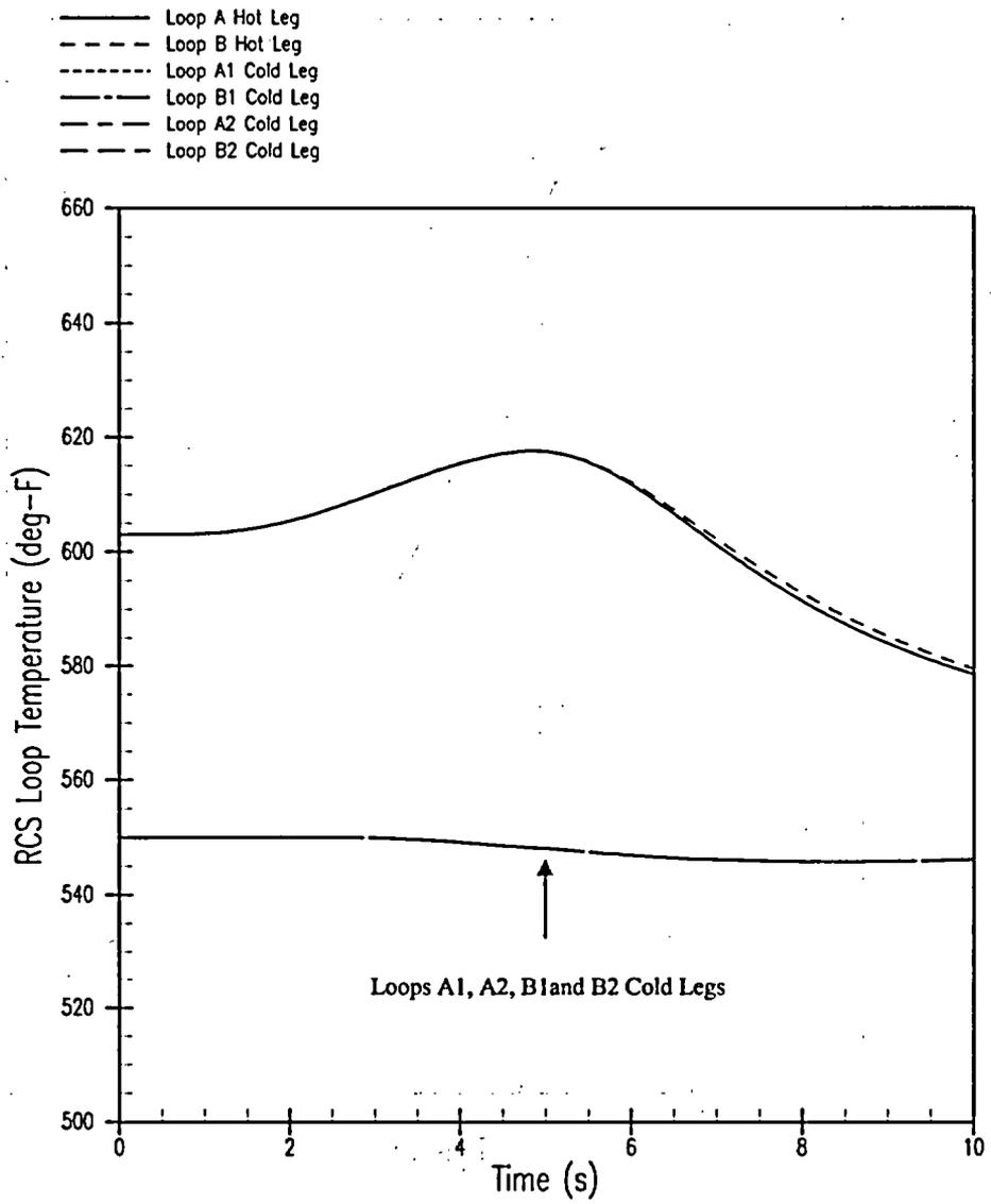
Figure 5.1.14-6 RCS Loop Temperature versus Time – Complete Loss of Flow – Four Pumps Coasting Down (CLOF)
