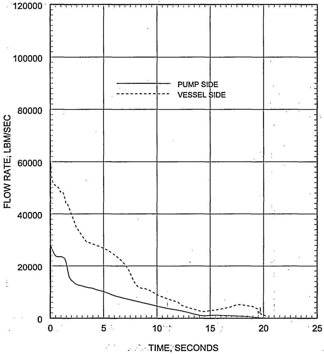
Figure 5.2.3.3-12 Large Break LOCA ECCS Performance Analysis 0.8 DEG/PD Break Leak Flow Rate
