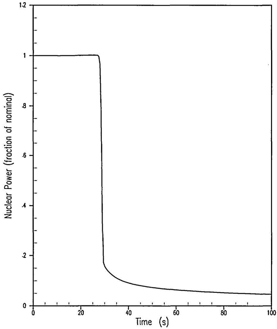
**Figure 5.1.22-1 Nuclear Power for an Accidental Depressurization of the Reactor Coolant System Event**
