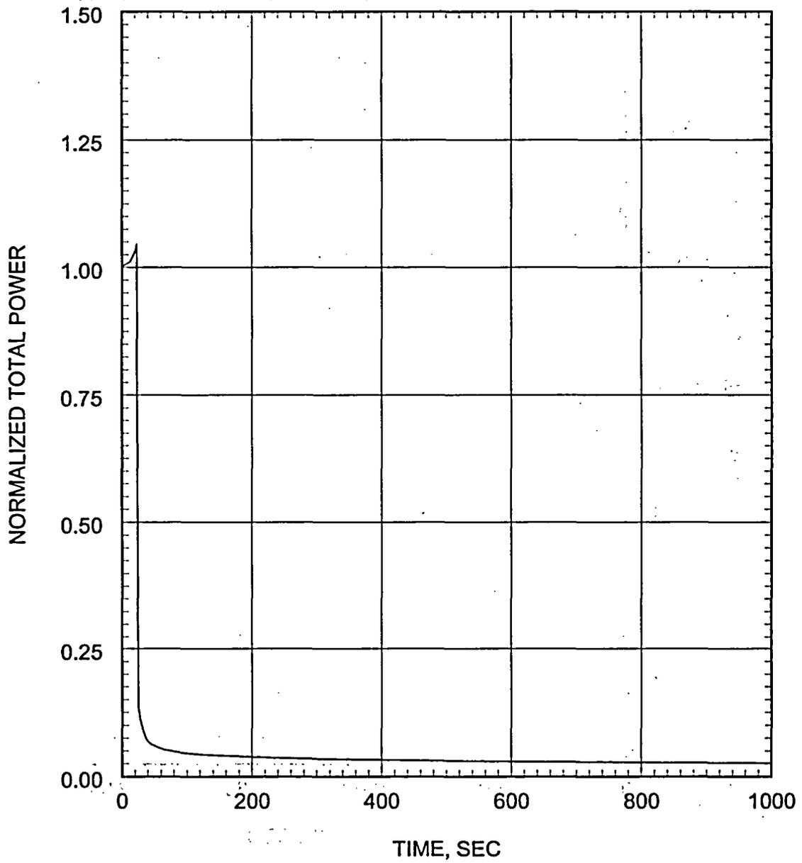
Figure 5.2.43-17 Small Break LOCA ECCS Performance Analysis 0.06 ft<sup>2</sup>/PD Break Core Power
