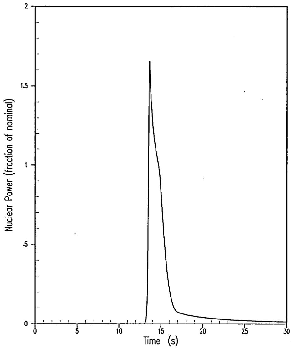
**Figure 5.1.17-1 Uncontrolled CEA Withdrawal from a Subcritical Condition – Reactor Power versus Time**
