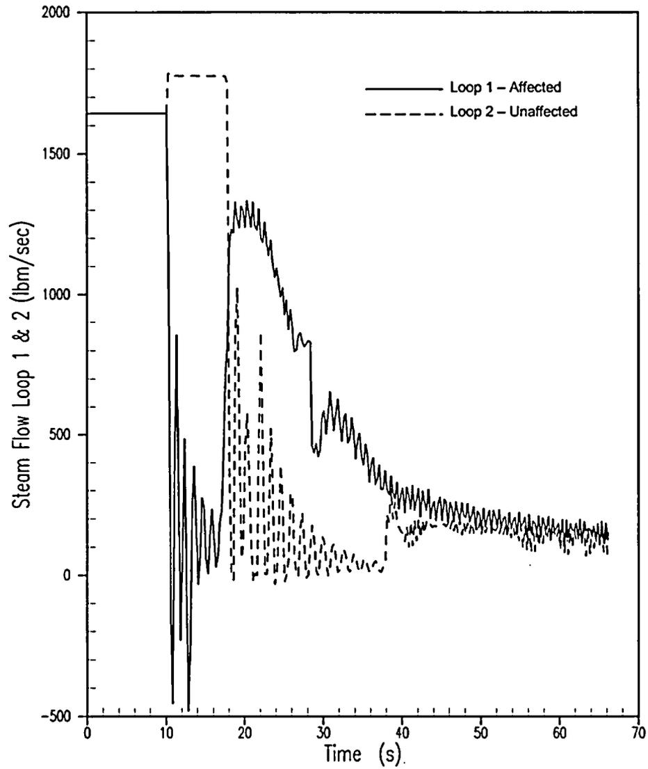
Figure 5.1.11-7 Steam Flow for Asymmetric Steam Generator Transient 0% Tube Plugging
