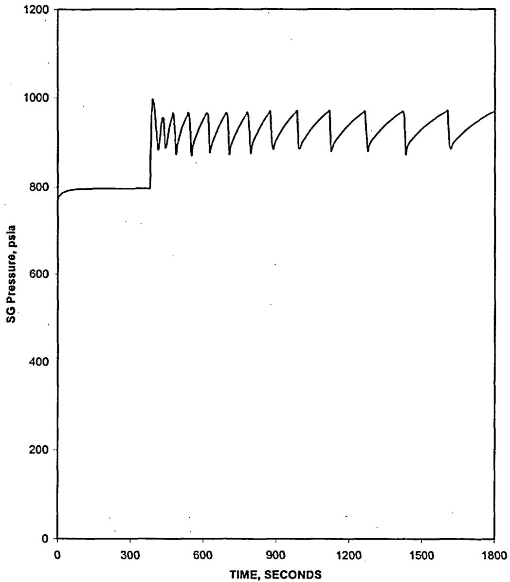
Figure 5.1.24-5 Steam Generator Tube Rupture with Loss of Offsite Power – Steam Generator Pressure vs. Time
