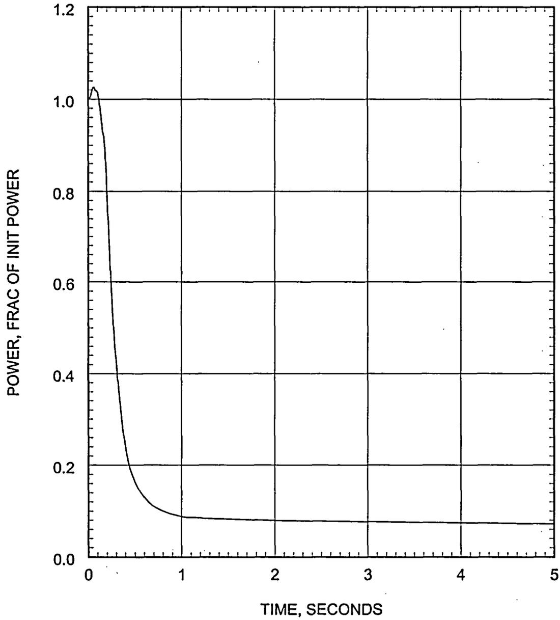
Figure 5.2.3.3-19 Large Break LOCA ECCS Performance Analysis 0.6 DEG/PD Break Core Power
