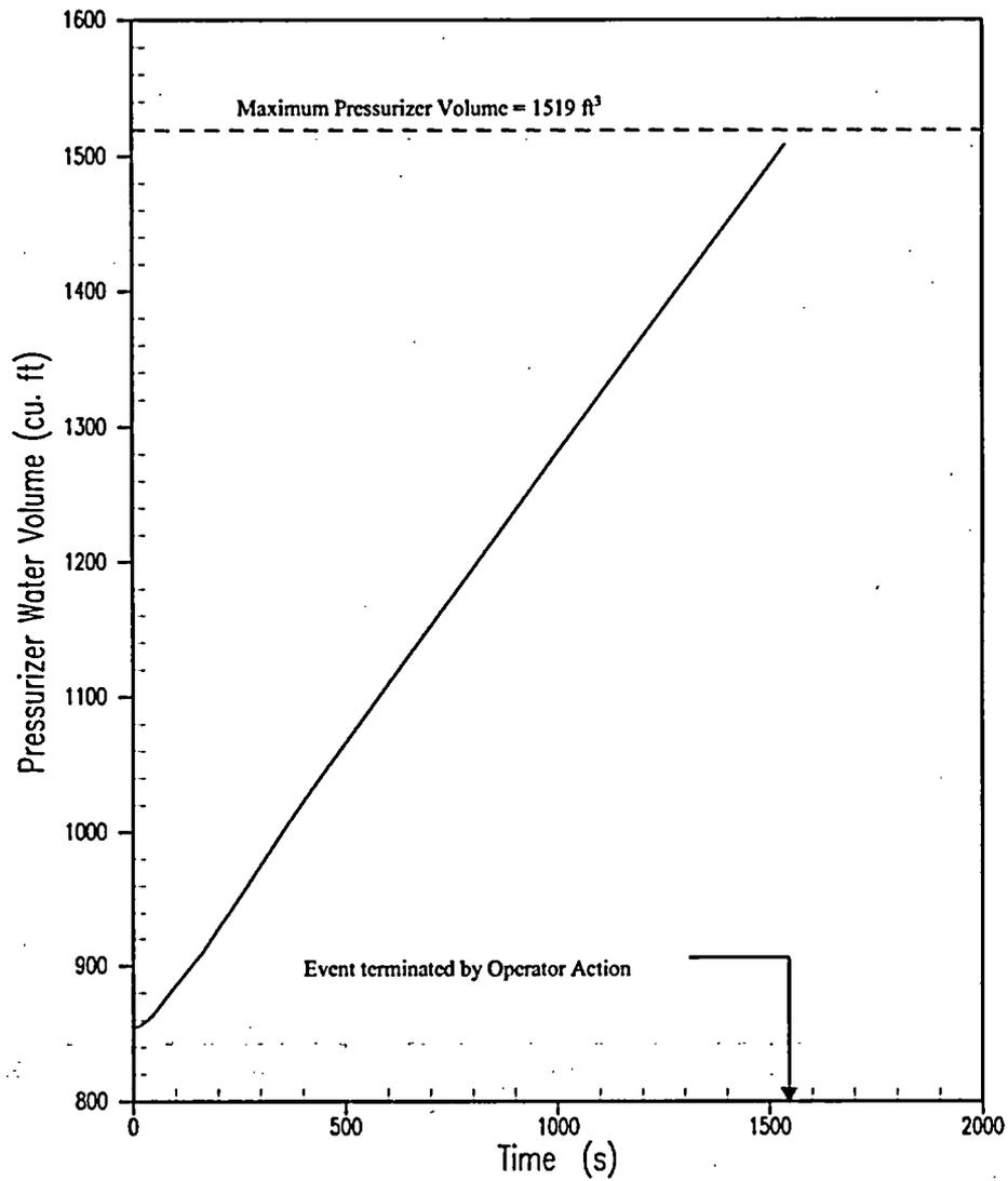
Figure 5.1.21-4 CVCS Malfunction at Power – Pressurizer Water Volume
