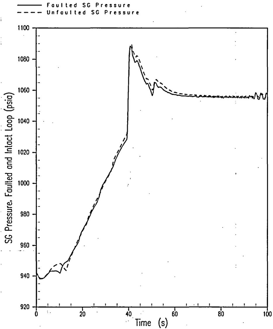
Figure 5.1.12-12 Feedwater Line Break MSS Overpressure Case Limiting Break Size = 0.05 ft<sup>2</sup> SG Pressure, Faulted and Intact Loop
