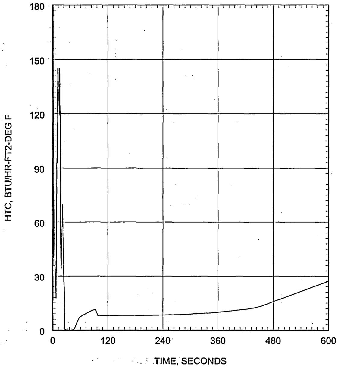
Figure 5.2.3.3-36 Large Break LOCA ECCS Performance Analysis 0.6 DEG/PD Break Hot Spot Heat Transfer Coefficient
