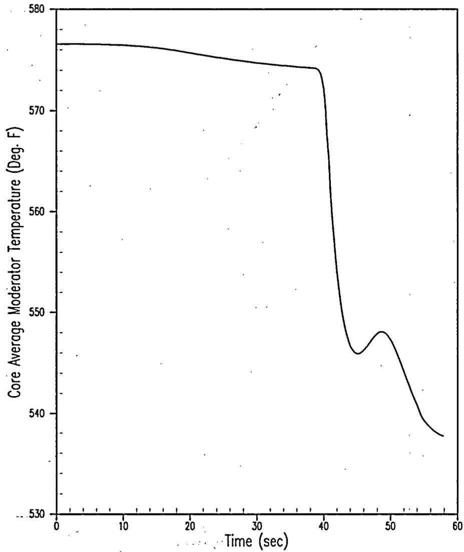
**Figure 5.1.3-5 Core Average Moderator Temperature for a Feedwater Malfunction Reduced Feedwater Temperature at HFP Initial Conditions**
