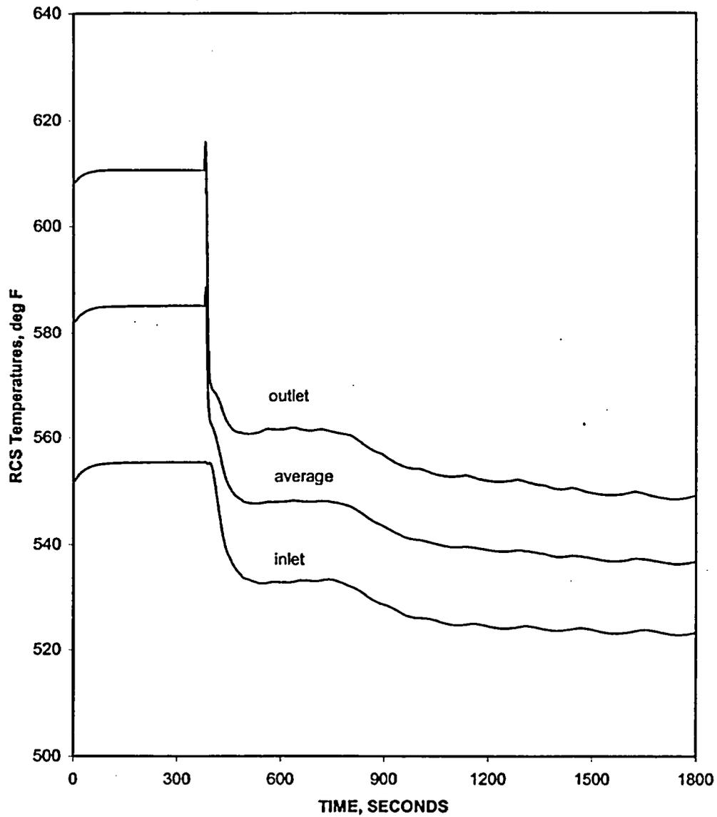
**Figure 5.1.24-3 Steam Generator Tube Rupture with Loss of Offsite Power – Reactor Coolant System Temperatures vs. Time**
