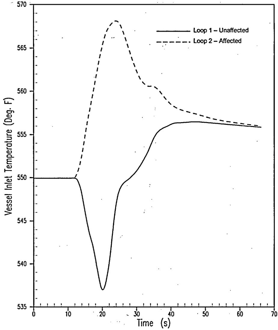
**Figure 5.1.11-4 Vessel Inlet Temperature for Asymmetric Steam Generator Transient 0% Tube Plugging**
