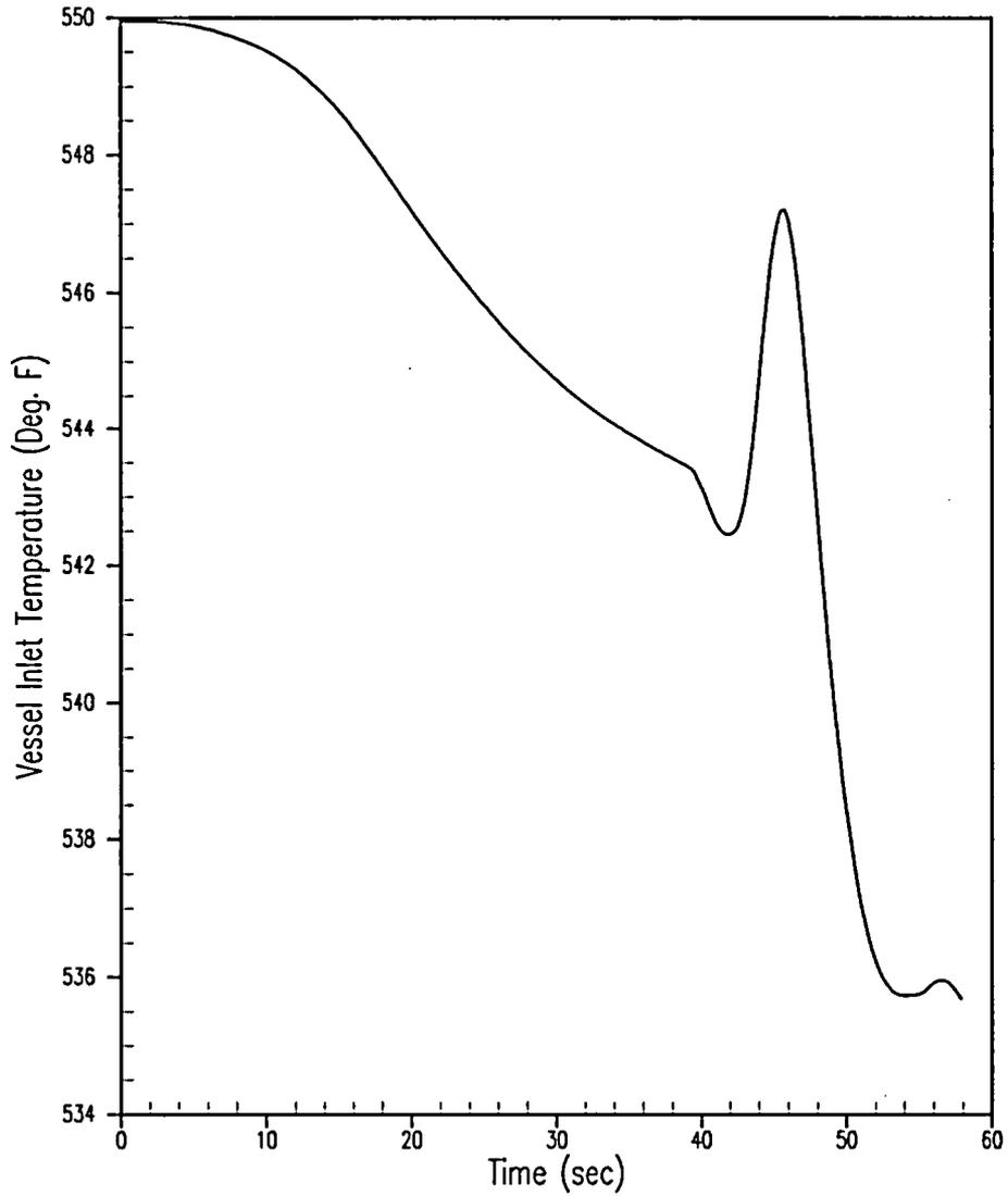
**Figure 5.1.3-6 Vessel Inlet Temperature for a Feedwater Malfunction Reduced Feedwater Temperature at HFP Initial Conditions**
