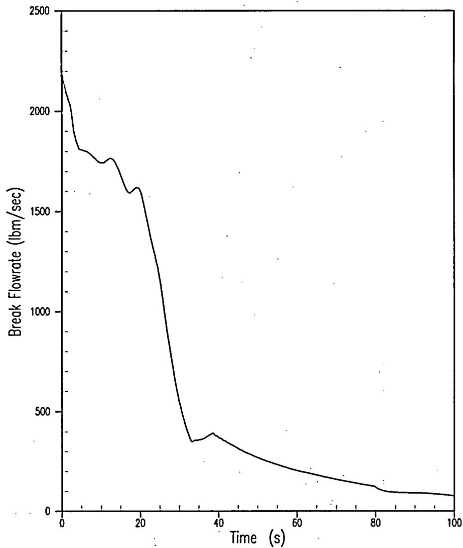
Figure 5.1.12-6 Feedwater Line Break RCS Overpressure Case Limiting Break Size = 0.28 ft<sup>2</sup> Break Flowrate
