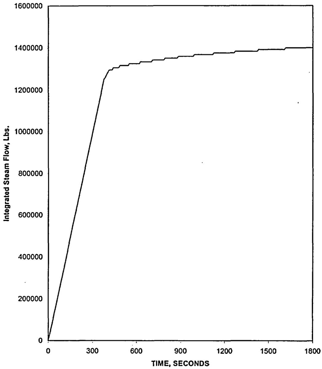
Figure 5.1.24-7 Steam Generator Tube Rupture with Loss of Offsite Power – Integrated Steam Flow vs. Time
