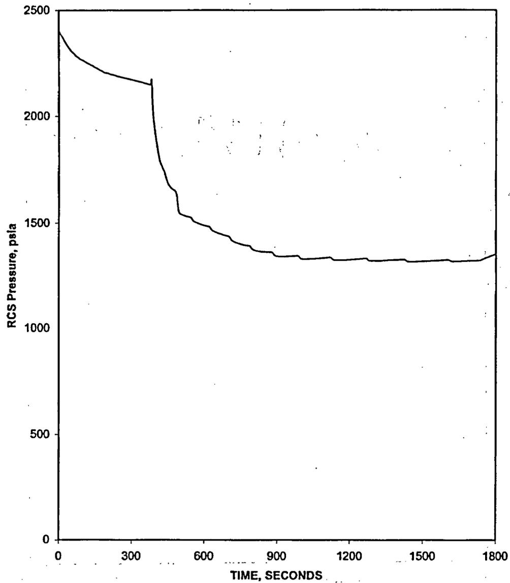
**Figure 5.1.24-4 Steam Generator Tube Rupture with Loss of Offsite Power – Reactor Coolant System Pressure vs. Time**
