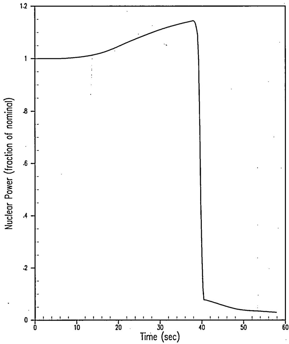
**Figure 5.1.3-1 Nuclear Power for a Feedwater Malfunction Reduced Feedwater Temperature at HFP Initial Conditions**
