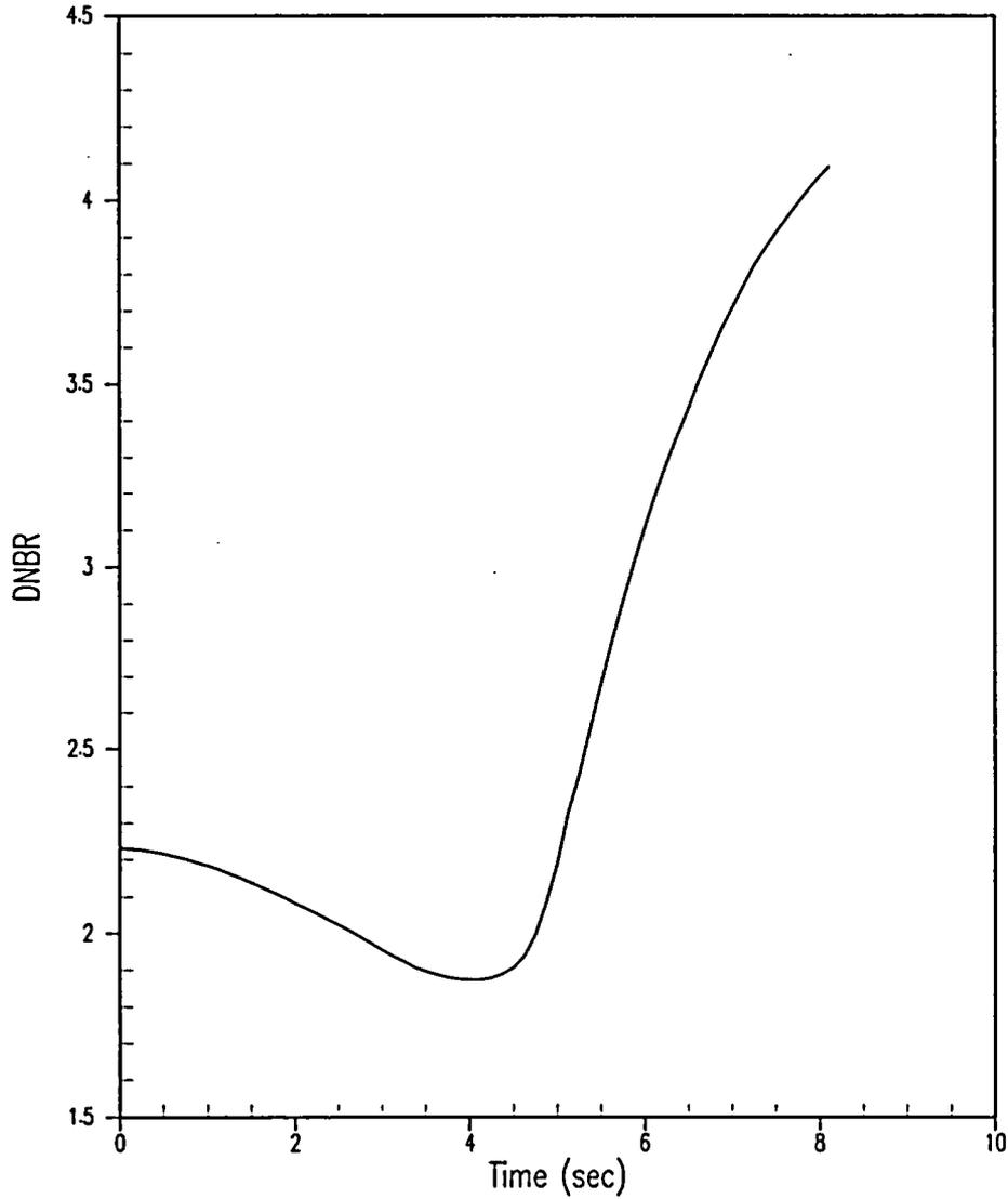
**Figure 5.1.16-1 Uncontrolled CEA Bank Withdrawal at Power 100% Power, 53 pcm/sec Reactivity Insertion Rate & Minimum Feedback Variable High Power Trip & Maximum Nominal RCS Vessel  $T_{avg}$  (Sheet 4 of 4)**
