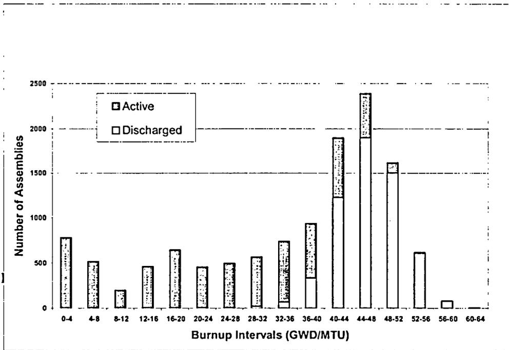
**Figure 2-1** Total Number of Active and Discharged ZIRLO™ Assemblies (as of March 31, 2003, plotted as a function of burnup)
