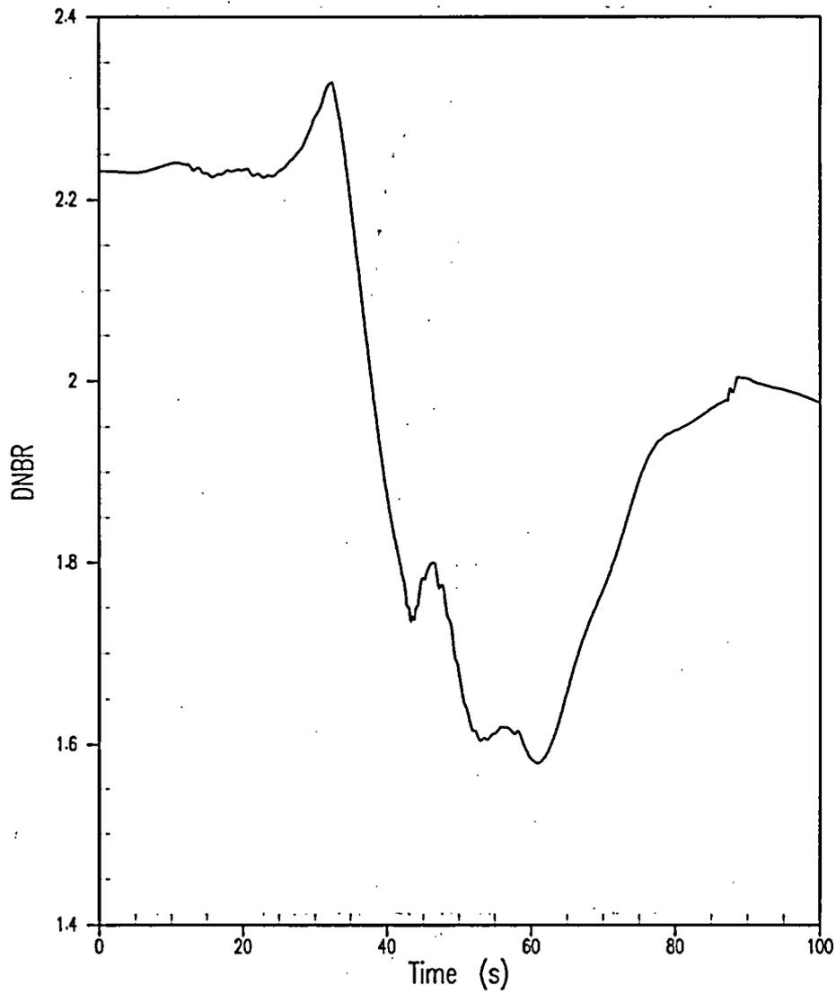
Figure 5.1.12-16 Feedwater Line Break DNB Case Limiting Break Size = 0.25 ft<sup>2</sup> DNBR
