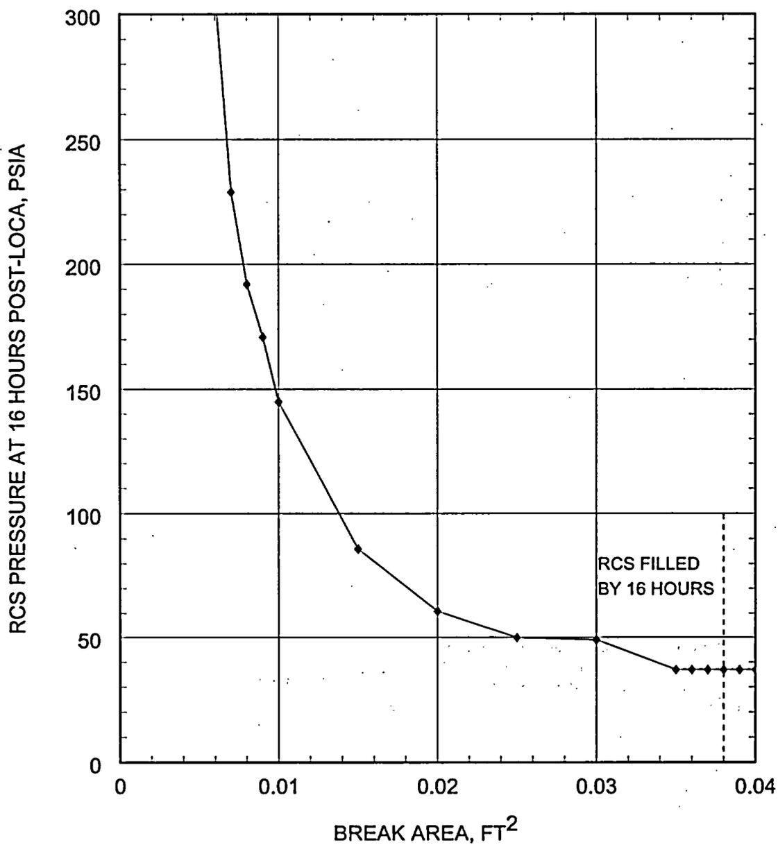
Figure 5.2.5.3-5 Long-Term Cooling Analysis RCS Pressure at the Decision Time Versus Break Area
