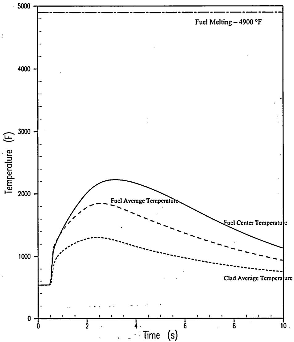
Figure 5.1.20-4 CEA Ejection Accident from Zero Power Beginning of Cycle – Fuel and Cladding Temperatures versus Time
