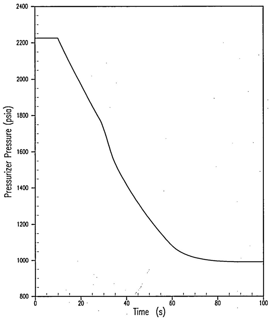
**Figure 5.1.22-2 Pressurizer Pressure for an Accidental Depressurization of the Reactor Coolant System Event**
