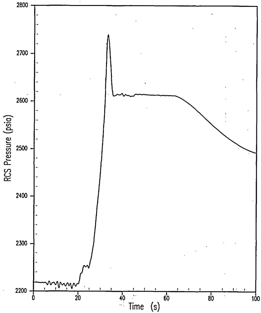
**Figure 5.1.12-2 Feedwater Line Break RCS Overpressure Case Limiting Break Size = 0.28 ft<sup>2</sup> RCS Pressure**
