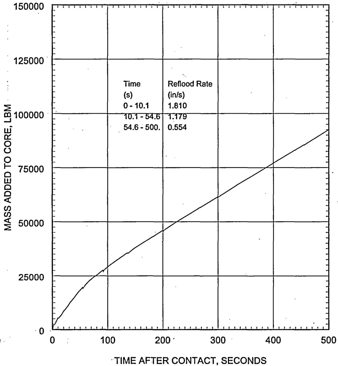
Figure 5.2.3.3-46 Large Break LOCA ECCS Performance Analysis 0.4 DEG/PD Break Mass Added to Core During Reflood
