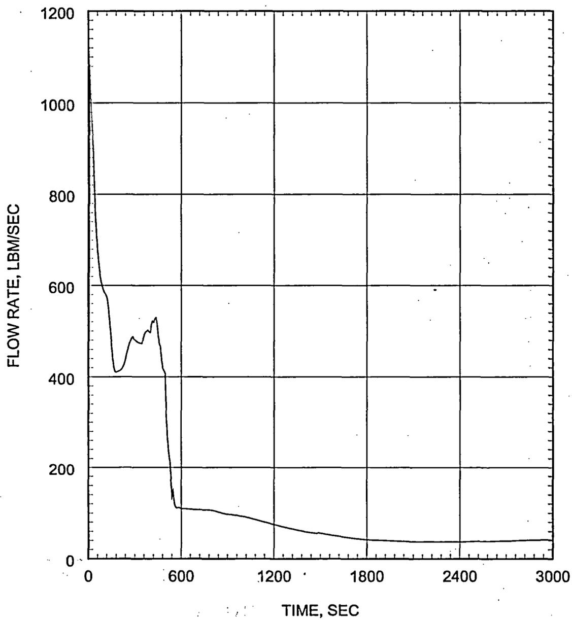
Figure 5.2.4.3-11 Small Break LOCA ECCS Performance Analysis 0.05 ft<sup>2</sup>/PD Break Break Flow Rate
