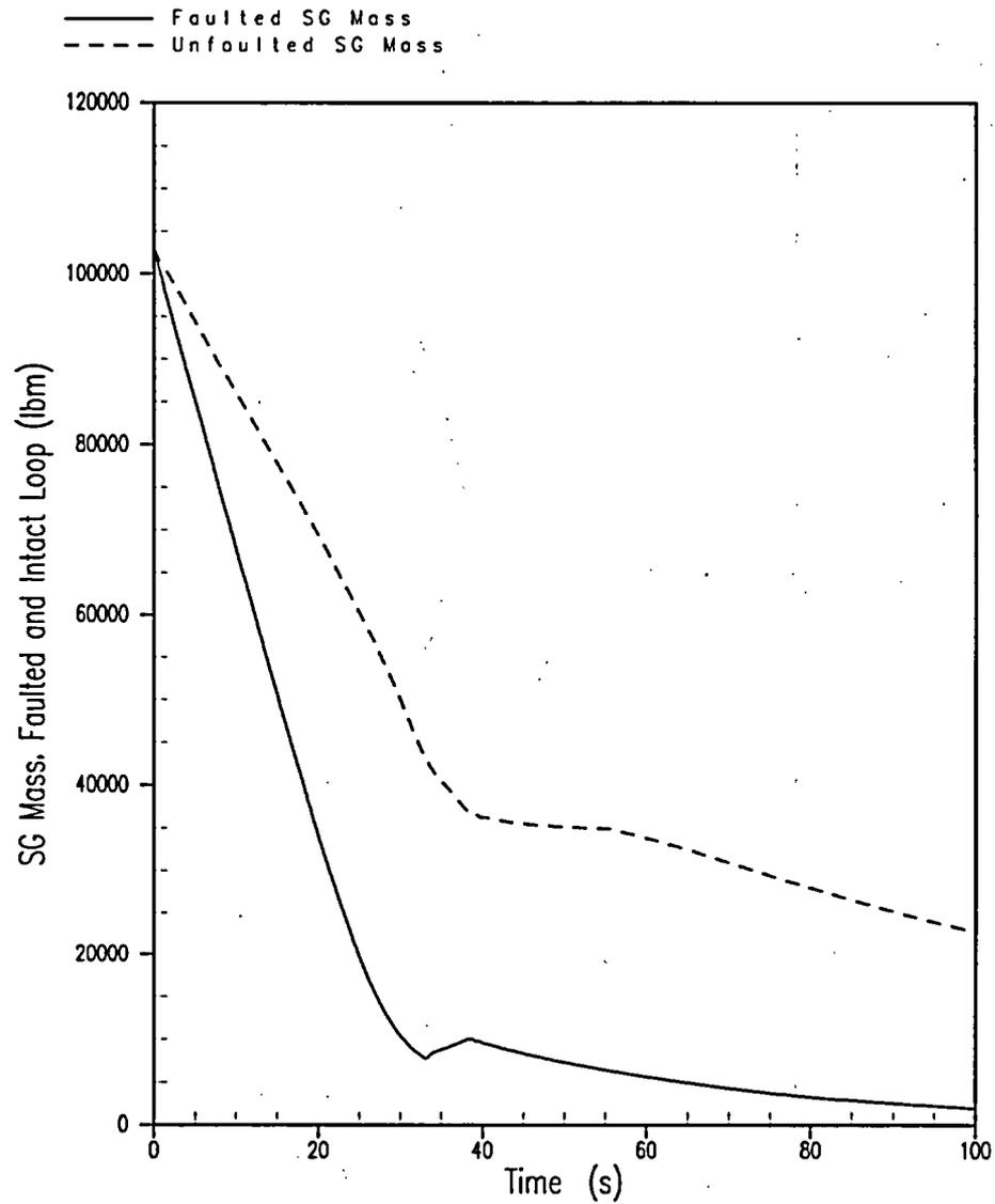
Figure 5.1.12-4 Feedwater Line Break RCS Overpressure Case Limiting Break Size = 0.28 ft<sup>2</sup> SG Mass, Faulted and Intact Loop
