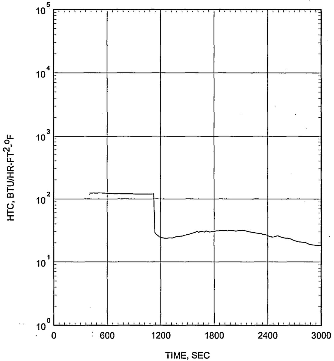
Figure 5.2.4.3-6 Small Break LOCA ECCS Performance Analysis 0.04 ft<sup>2</sup>/PD Break Heat Transfer Coefficient at Hot Spot
