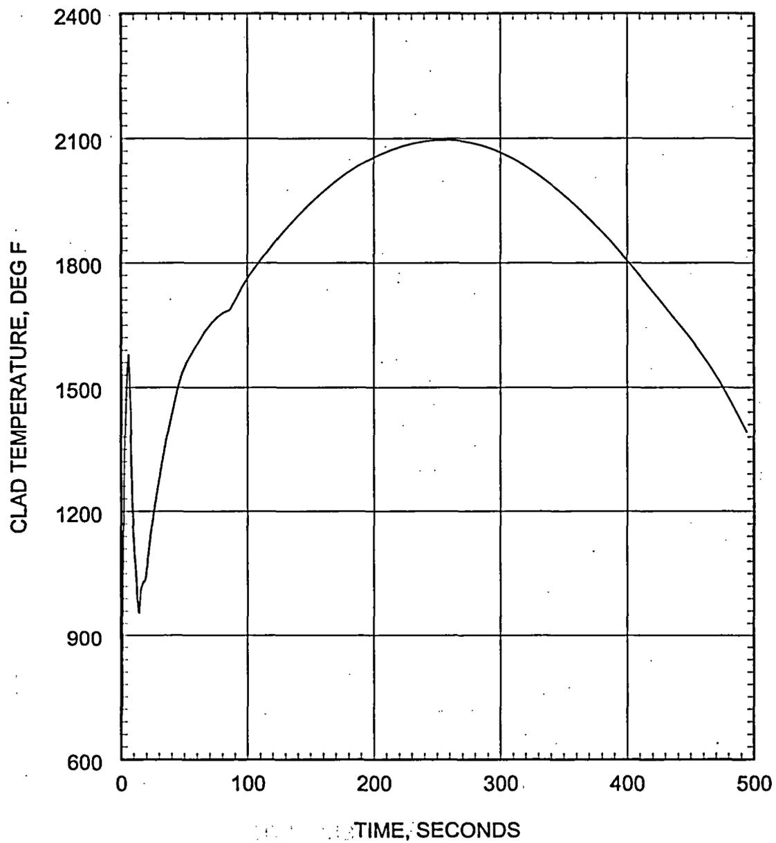
Figure 5.2.3.3-18 Large Break LOCA ECCS Performance Analysis 0.8 DEG/PD Break Peak Cladding Temperature
