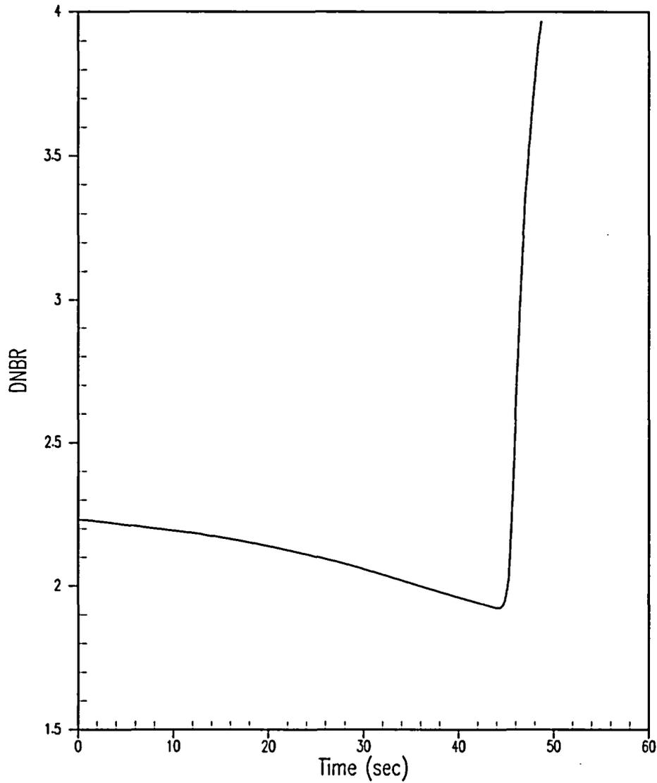
**Figure 5.1.16-2 Uncontrolled CEA Bank Withdrawal at Power 100% Power, 2 pcm/sec Reactivity Insertion Rate & Minimum Feedback Variable High Power Trip & Maximum Nominal RCS Vessel  $T_{avg}$  (Sheet 4 of 4)**
