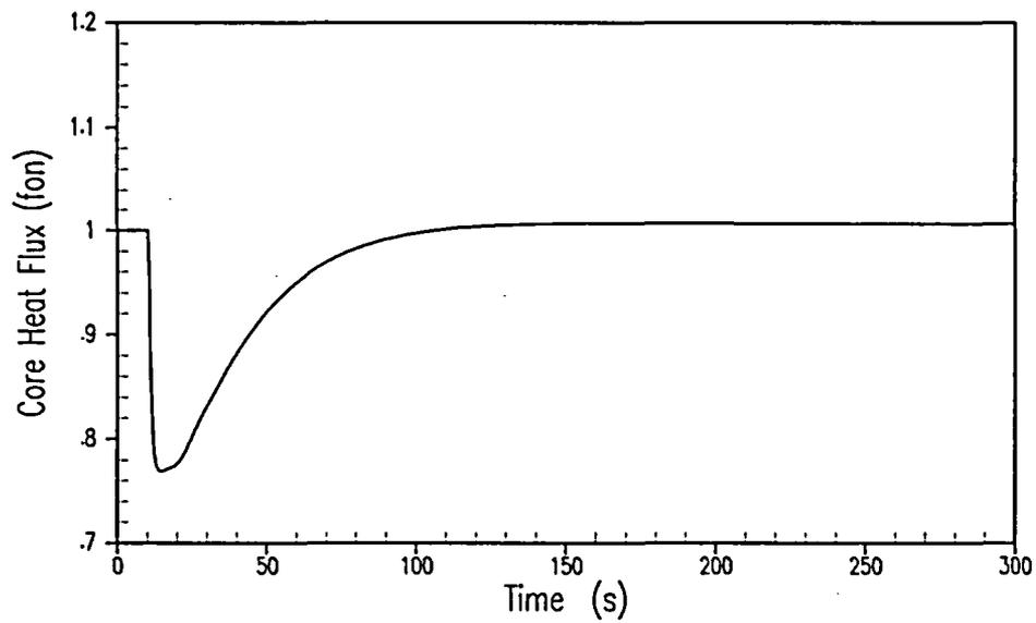
**Figure 5.1.18-6 Representative Transient Response to Dropped CEA Worth of 500 pcm at a Moderator Temperature Coefficient of  $-25 \text{ pcm}/^\circ\text{F}$  – Core Heat Flux versus Time**
