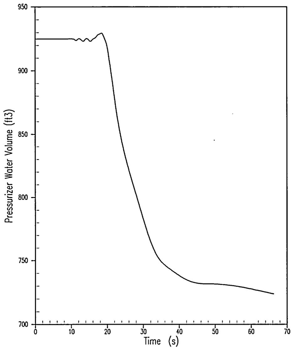
**Figure 5.1.11-15 Pressurizer Water Volume for Asymmetric Steam Generator Transient 30% Tube Plugging**
