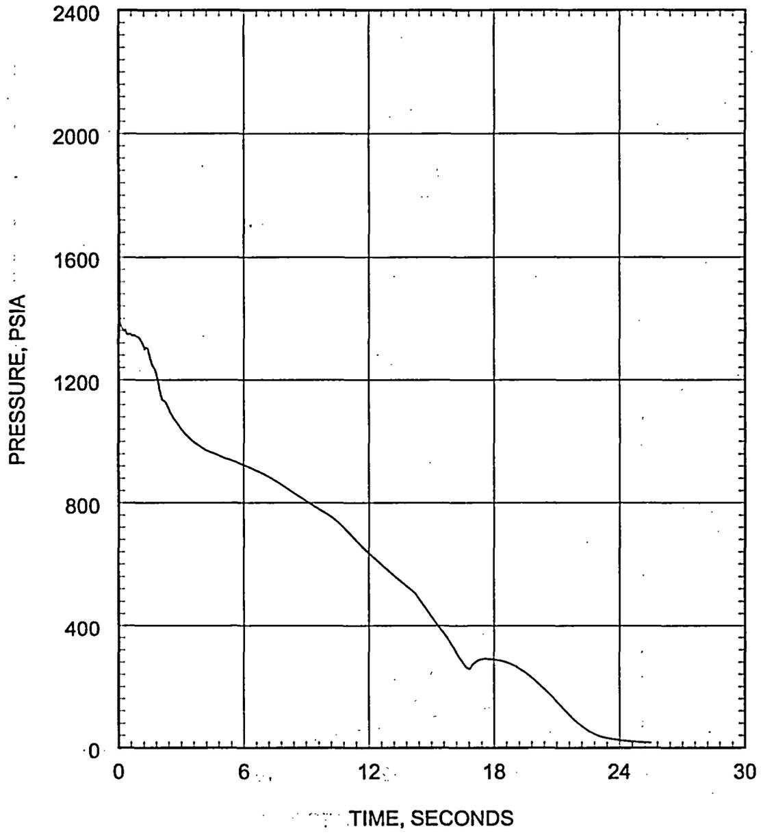
Figure 5.2.3.3-20 Large Break LOCA ECCS Performance Analysis 0.6 DEG/PD Break Pressure in Center Hot Assembly Node
