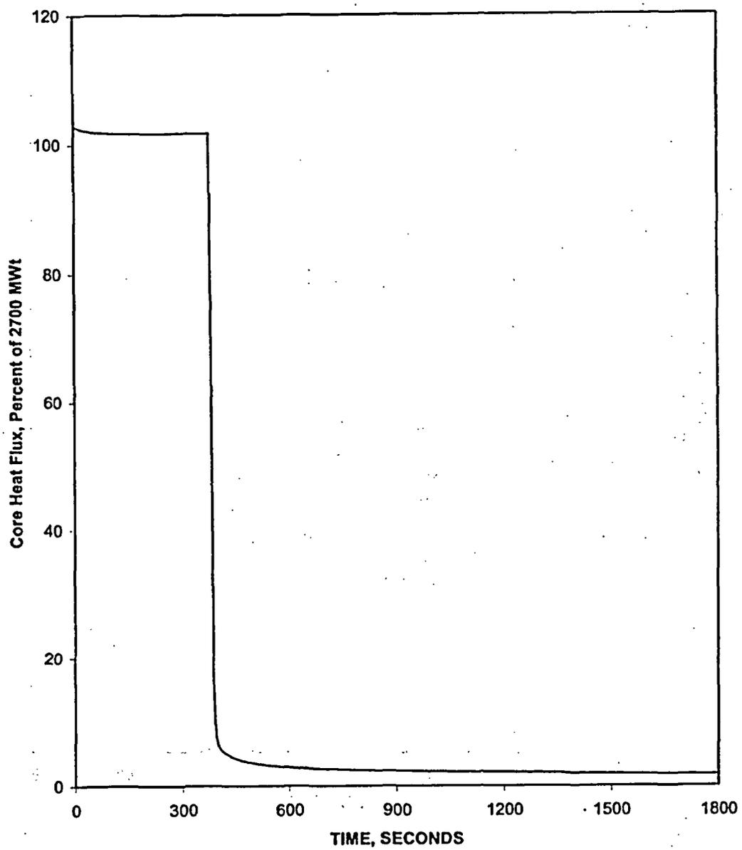
Figure 5.1.24-2 Steam Generator Tube Rupture with Loss of Offsite Power – Core Heat Flux vs. Time
