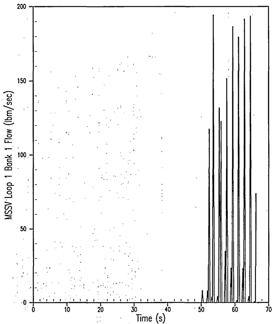
Figure 5.1.11-20. Main Steam Safety Valve Flow (Loop 1 – Bank 1 Unaffected Steam Generator) for Asymmetric Steam Generator Transient 30% Tube Plugging
