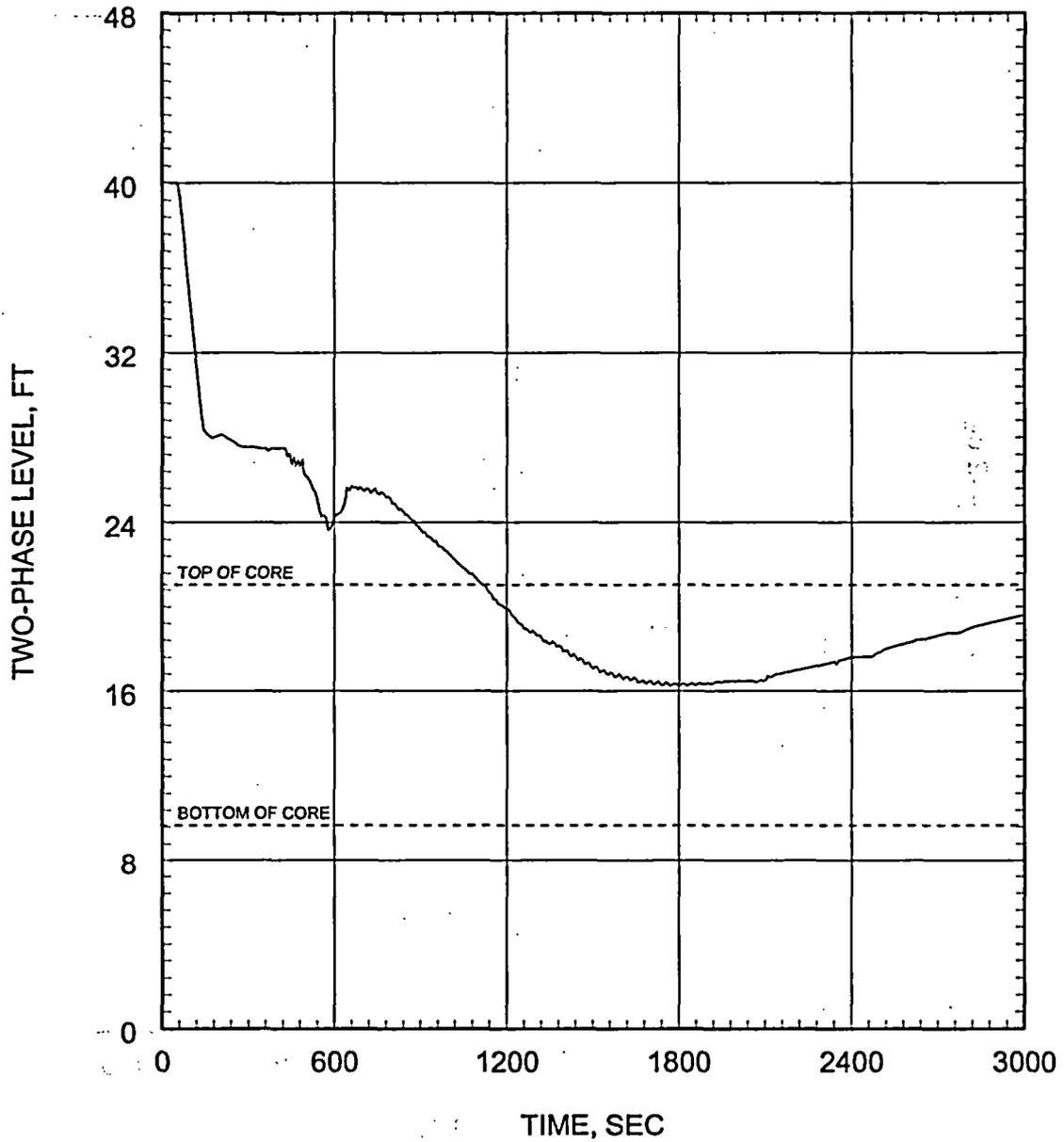
Figure 5.2.4.3-5 Small Break LOCA ECCS Performance Analysis 0.04 ft<sup>2</sup>/PD Break Inner Vessel Two-Phase Mixture Level
