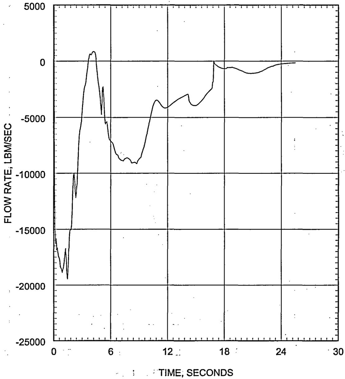
Figure 5.2.3.3-28 Large Break LOCA ECCS Performance Analysis 0.6 DEG/PD Break Mid-Annulus Flow Rate
