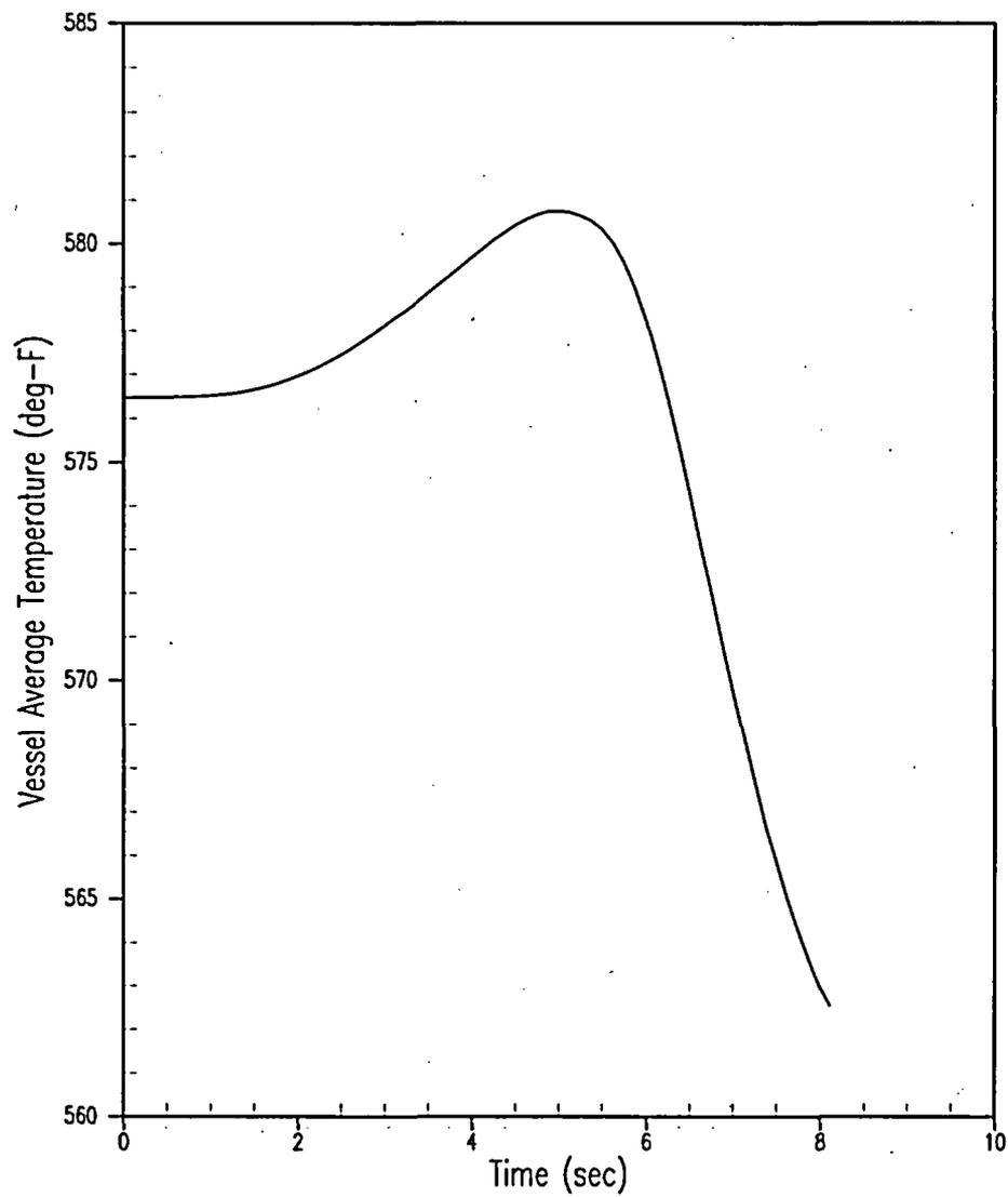
**Figure 5.1.16-1 Uncontrolled CEA Bank Withdrawal at Power 100% Power, 53 pcm/sec Reactivity Insertion Rate & Minimum Feedback Variable High Power Trip & Maximum Nominal RCS Vessel  $T_{avg}$  (Sheet 3 of 4)**
