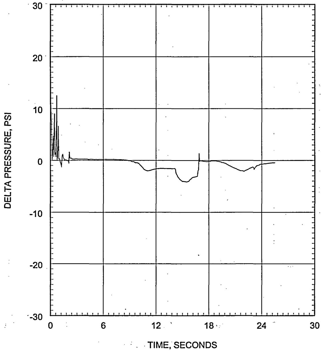
Figure 5.2.3.3-30 Large Break LOCA ECCS Performance Analysis 0.6 DEG/PD Break Core Pressure Drop
