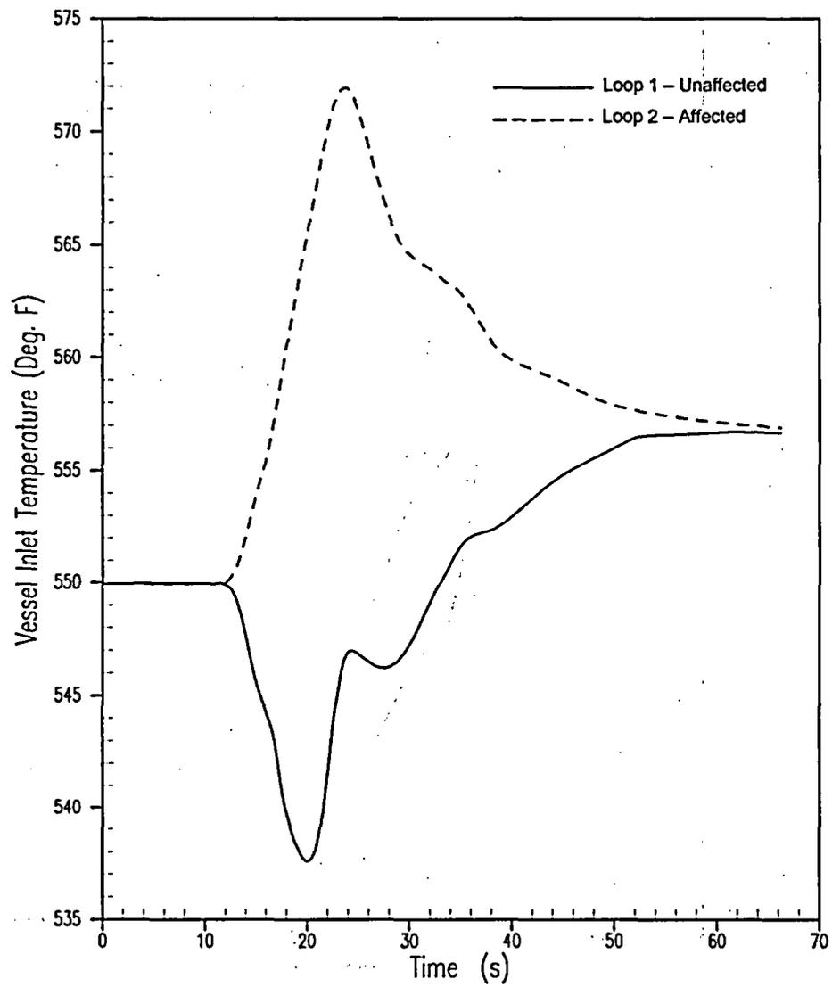
Figure 5.1.11-16 Vessel Inlet Temperature for Asymmetric Steam Generator Transient 30% Tube Plugging
