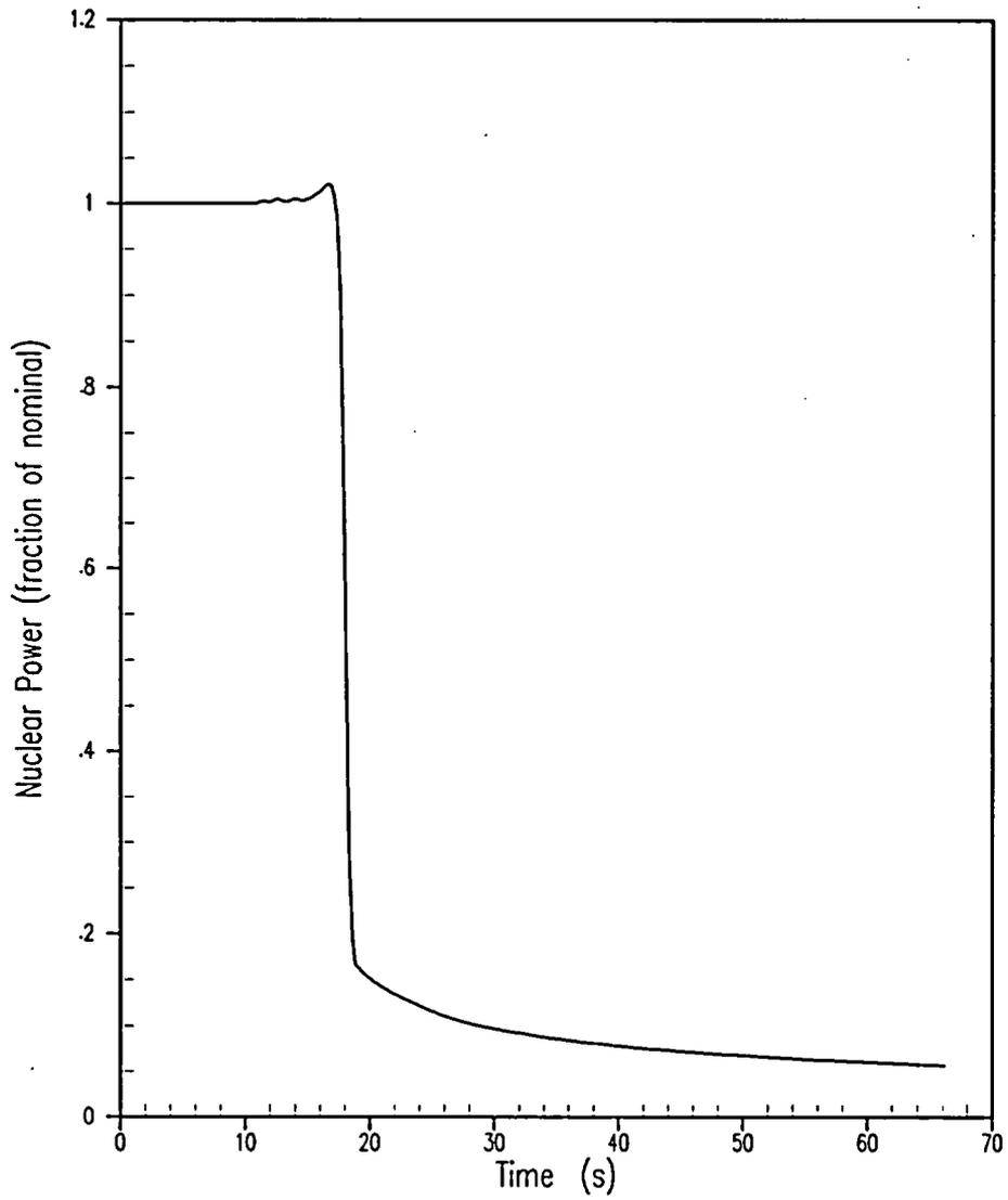
Figure 5.1.11-1 Nuclear Power for Asymmetric Steam Generator Transient 0% Tube Plugging
