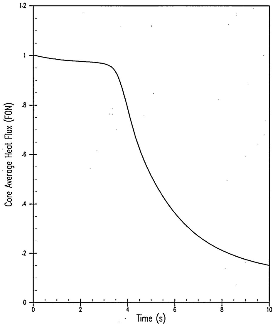
**Figure 5.1.14-4 Core Average Heat Flux versus Time – Complete Loss of Flow – Four Pumps Coasting Down (CLOF)**
