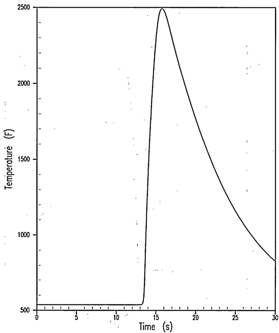
**Figure 5.1.17-4 Uncontrolled CEA Withdrawal from a Subcritical Condition – Hot Spot Fuel Average Temperature versus Time**
