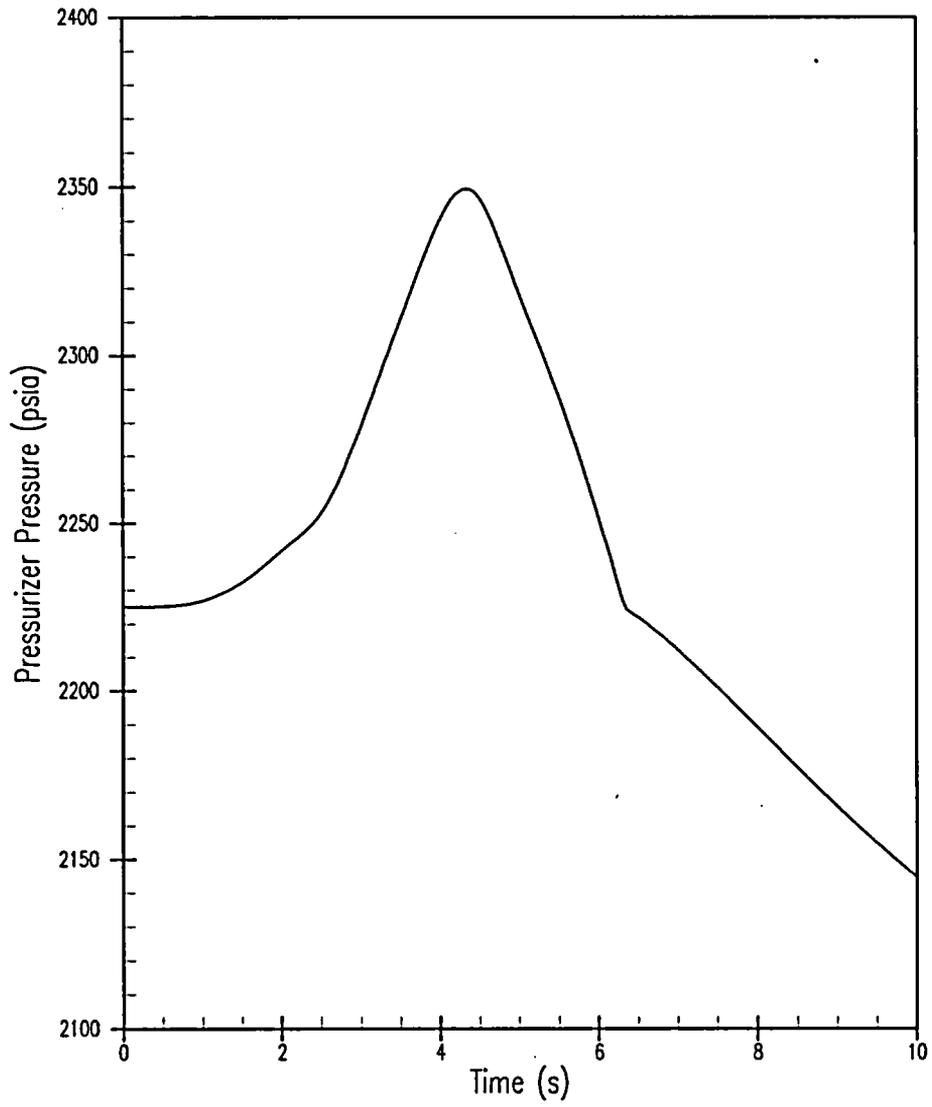
**Figure 5.1.14-5 Pressurizer Pressure versus Time – Complete Loss of Flow – Four Pumps Coasting Down (CLOF)**
