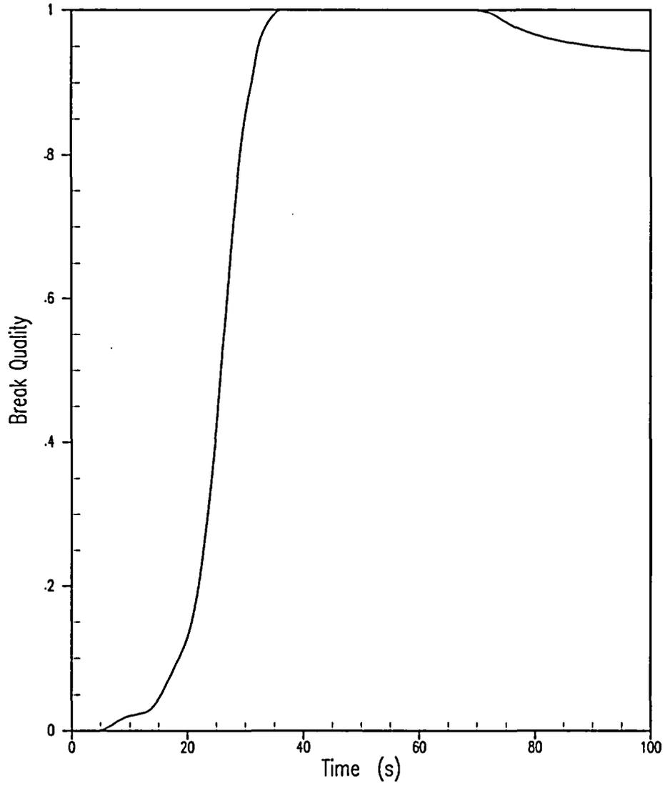
Figure 5.1.12-7 Feedwater Line Break RCS Overpressure Case Limiting Break Size = 0.28 ft<sup>2</sup> Break Quality
