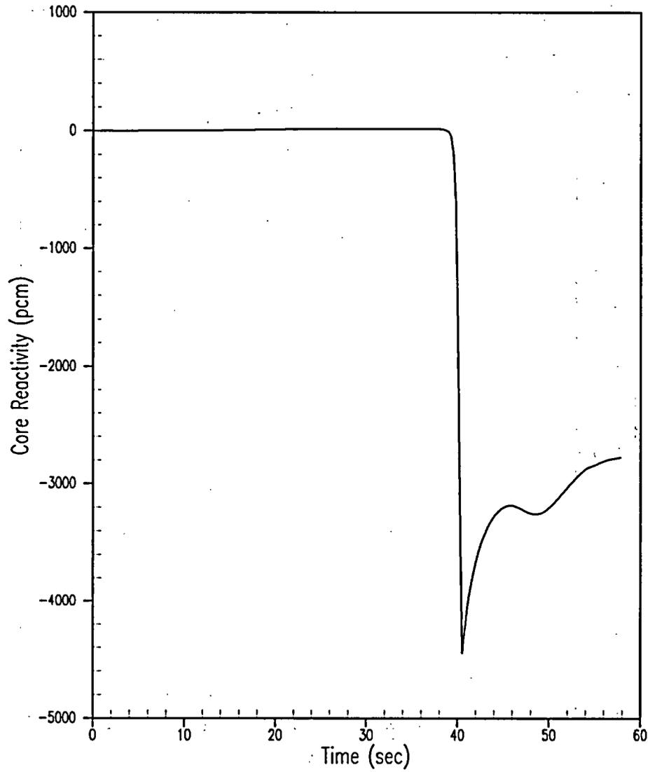
**Figure 5.1.3-3 Core Reactivity for a Feedwater Malfunction Reduced Feedwater Temperature at HFP Initial Conditions**
