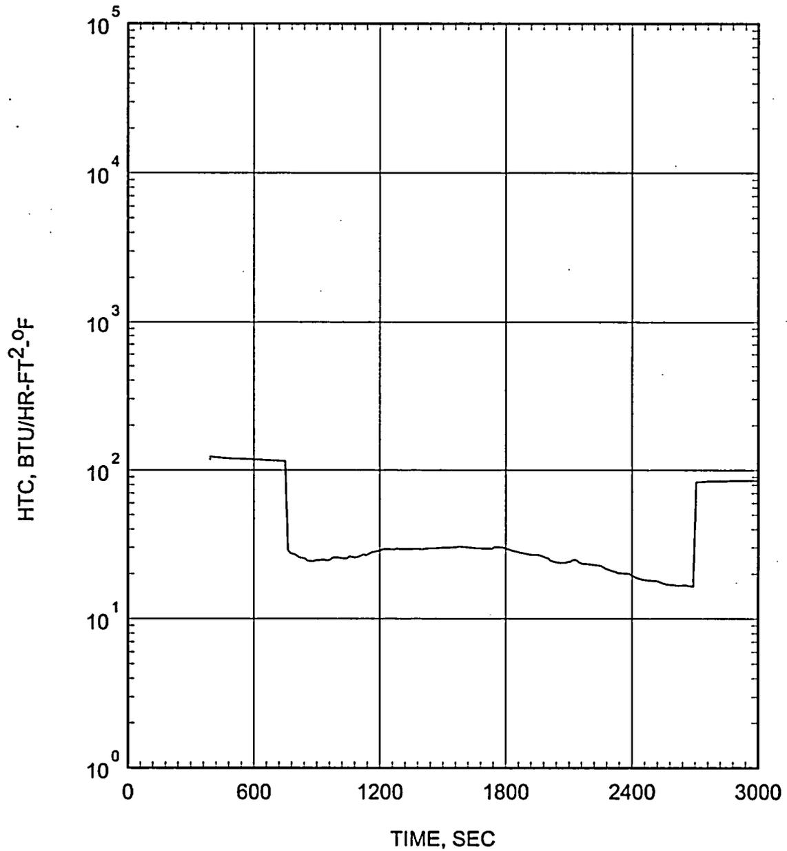
Figure 5.2.4.3-22 Small Break LOCA ECCS Performance Analysis 0.06 ft<sup>2</sup>/PD Break Heat Transfer Coefficient at Hot Spot
