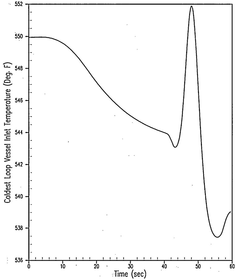
**Figure 5.1.1-6 Vessel Inlet Temperature for a Feedwater Malfunction Increased Feedwater Flow at HFP Initial Conditions**
