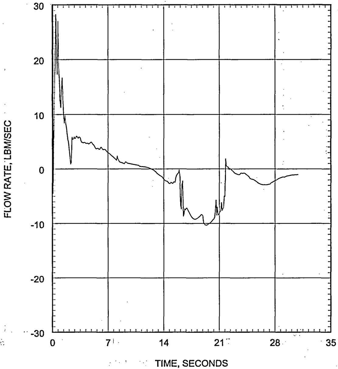
Figure 5.2.3.3-42 Large Break LOCA ECCS Performance Analysis 0.4 DEG/PD Break Hot Assembly Flow Rate (Below Hot Spot)
