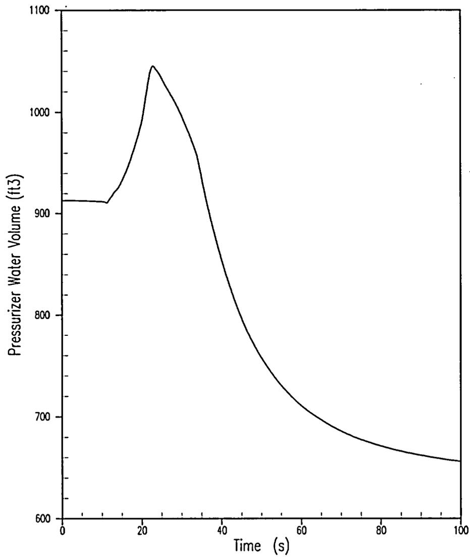
Figure 5.1.10-3 Loss of Condenser Vacuum (RCS Overpressure Case) Pressurizer Water Volume
