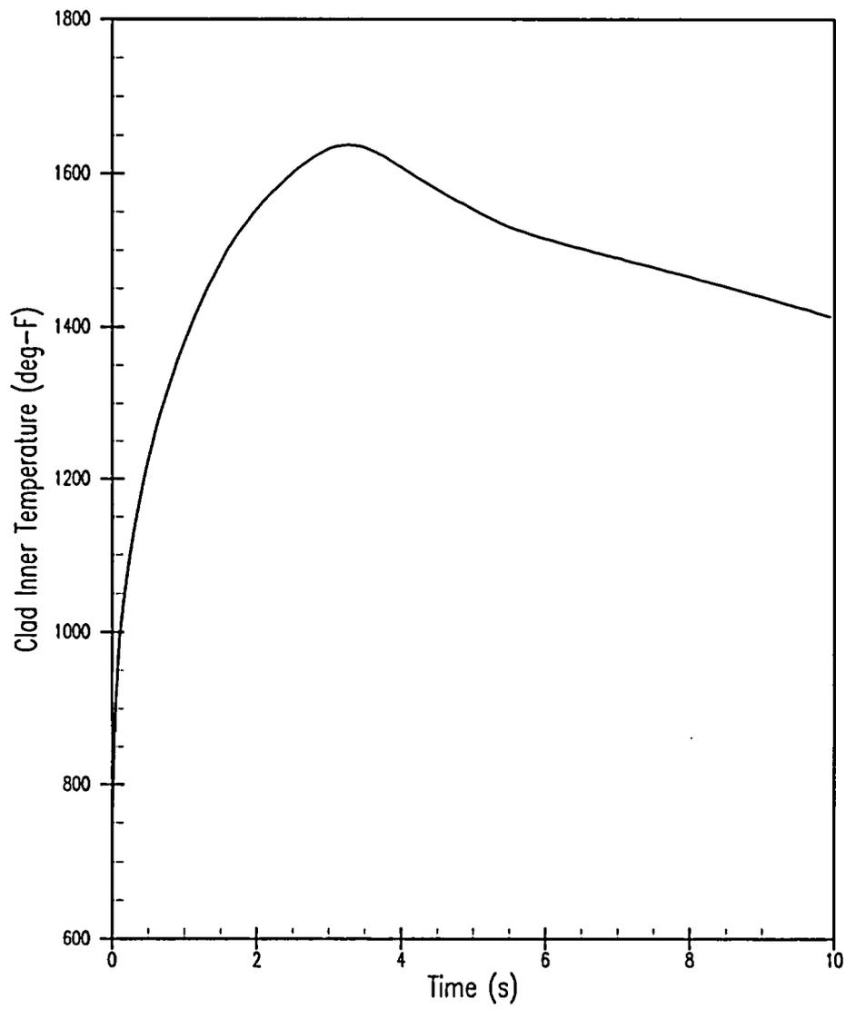
Figure 5.1.15-9 Hot-Spot Cladding Inner Temperature versus Time – Locked Rotor/Shaft Break
