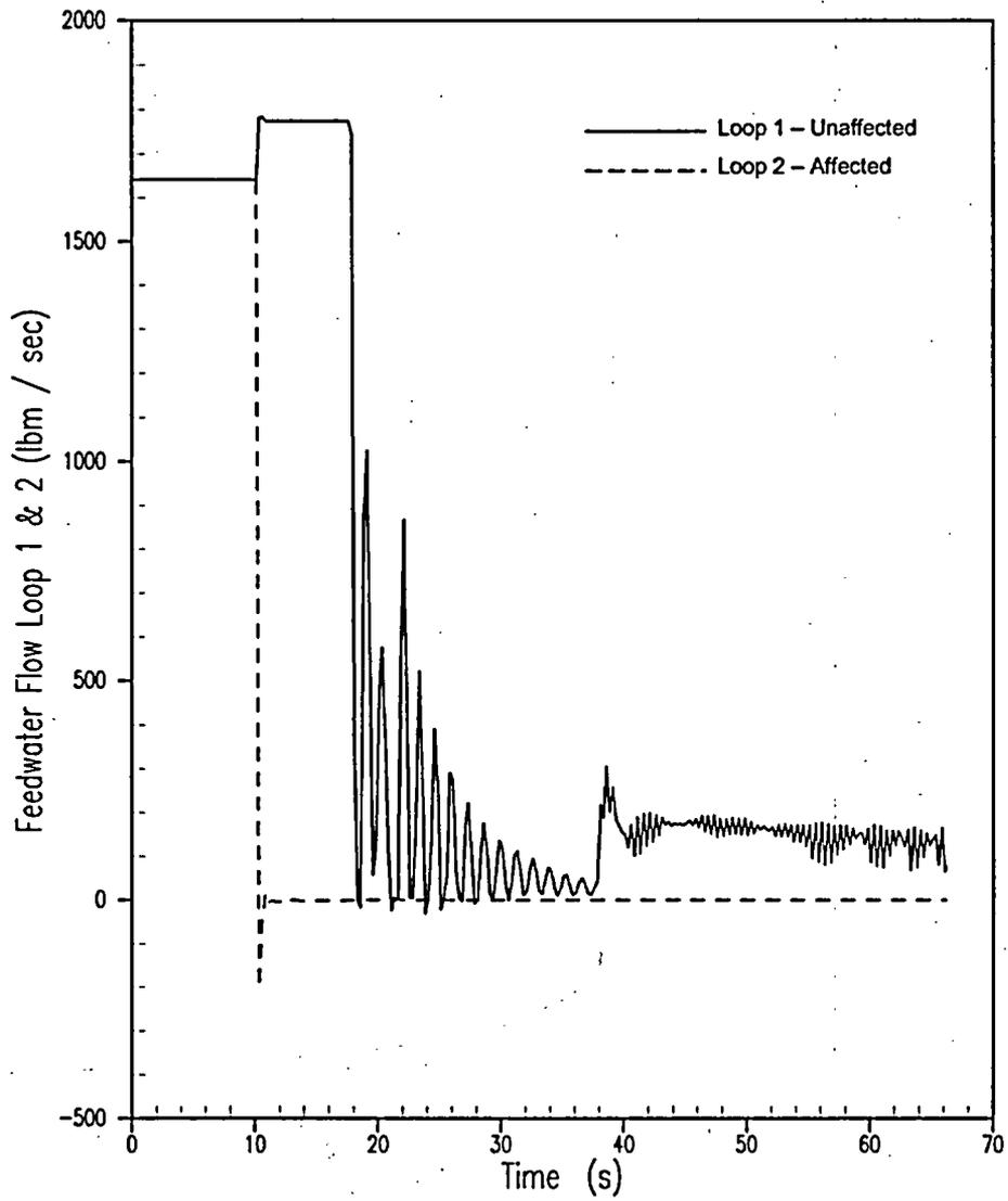
Figure 5.1.11-12 Feedwater Flow for Asymmetric Steam Generator Transient 0% Tube Plugging
