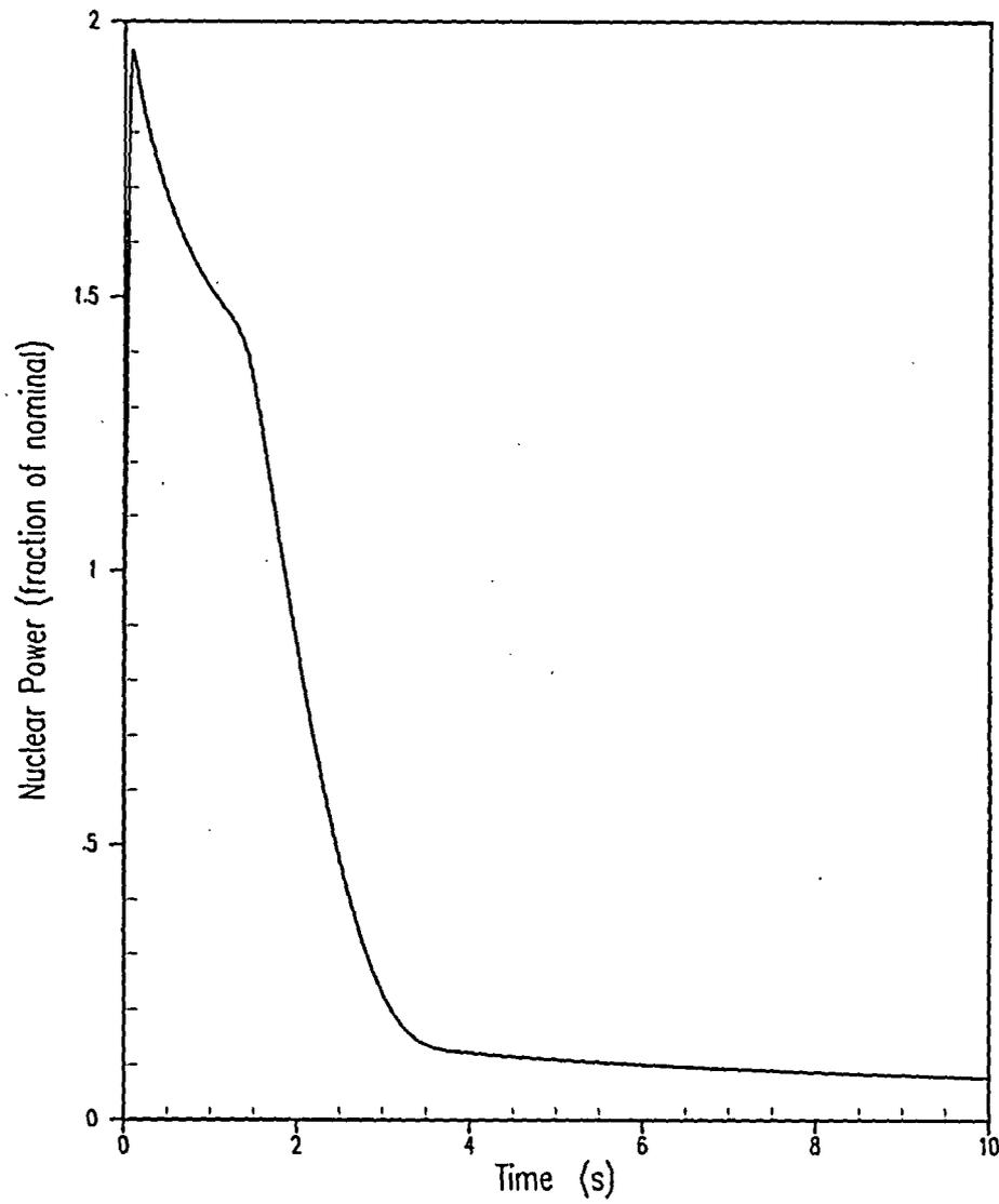
Figure 5.1.20-1 CEA Ejection Accident from Full Power Beginning of Cycle – Reactor Power versus Time
