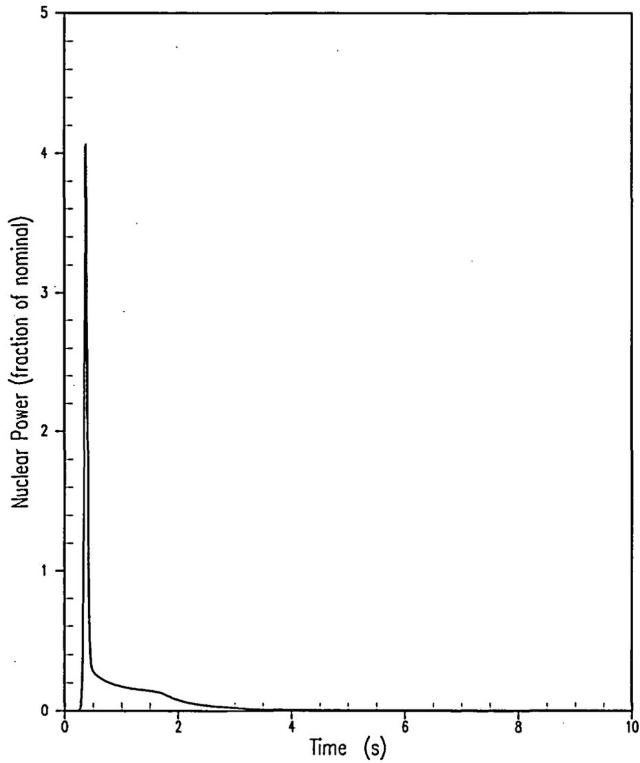
Figure 5.1.20-7 CEA Ejection Accident from Zero Power End of Cycle – Reactor Power versus Time
