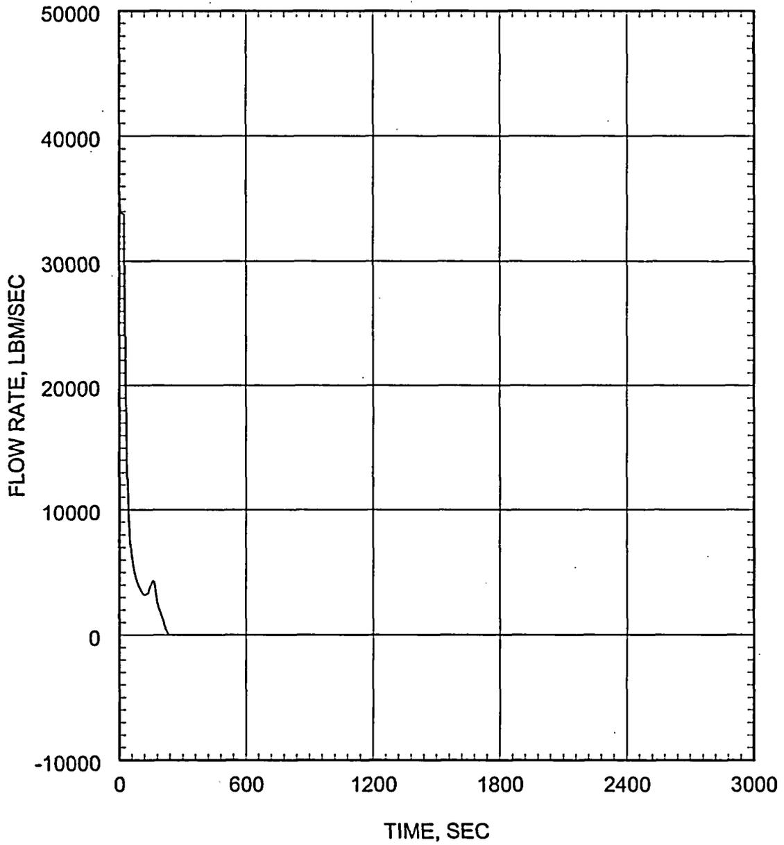
Figure 5.2.4.3-12 Small Break LOCA ECCS Performance Analysis 0.05 ft<sup>2</sup>/PD Break Inner Vessel Inlet Flow Rate
