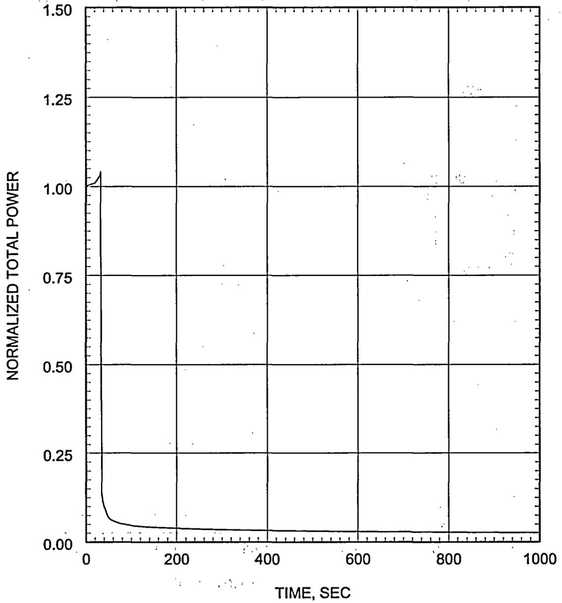
Figure 5.2.4.3-1 Small Break LOCA ECCS Performance Analysis 0.04 ft<sup>2</sup>/PD Break Core Power
