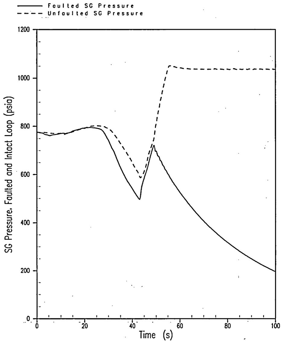
**Figure 5.1.12-20 Feedwater Line Break DNB Case Limiting Break Size = 0.25 ft<sup>2</sup> SG Pressure, Faulted and Intact Loop**
