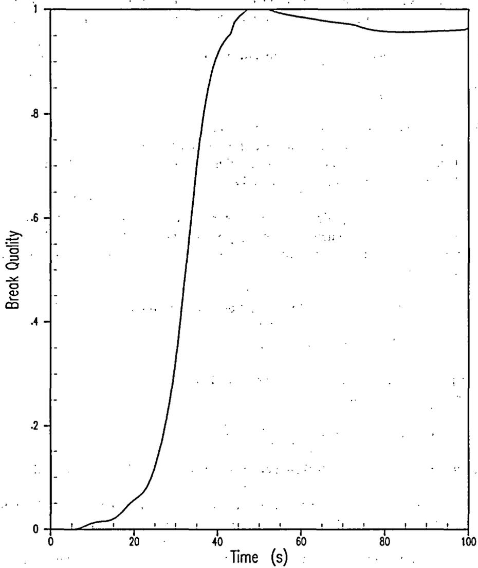
Figure 5.1.12-22 Feedwater Line Break DNB Case Limiting Break Size = 0.25 ft<sup>2</sup> Break Quality
