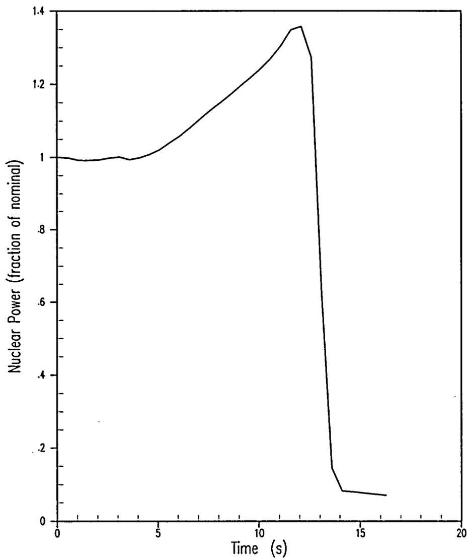
Figure 5.1.5-2 Pre-Trip Main Steamline Break – Nuclear Power versus Time
