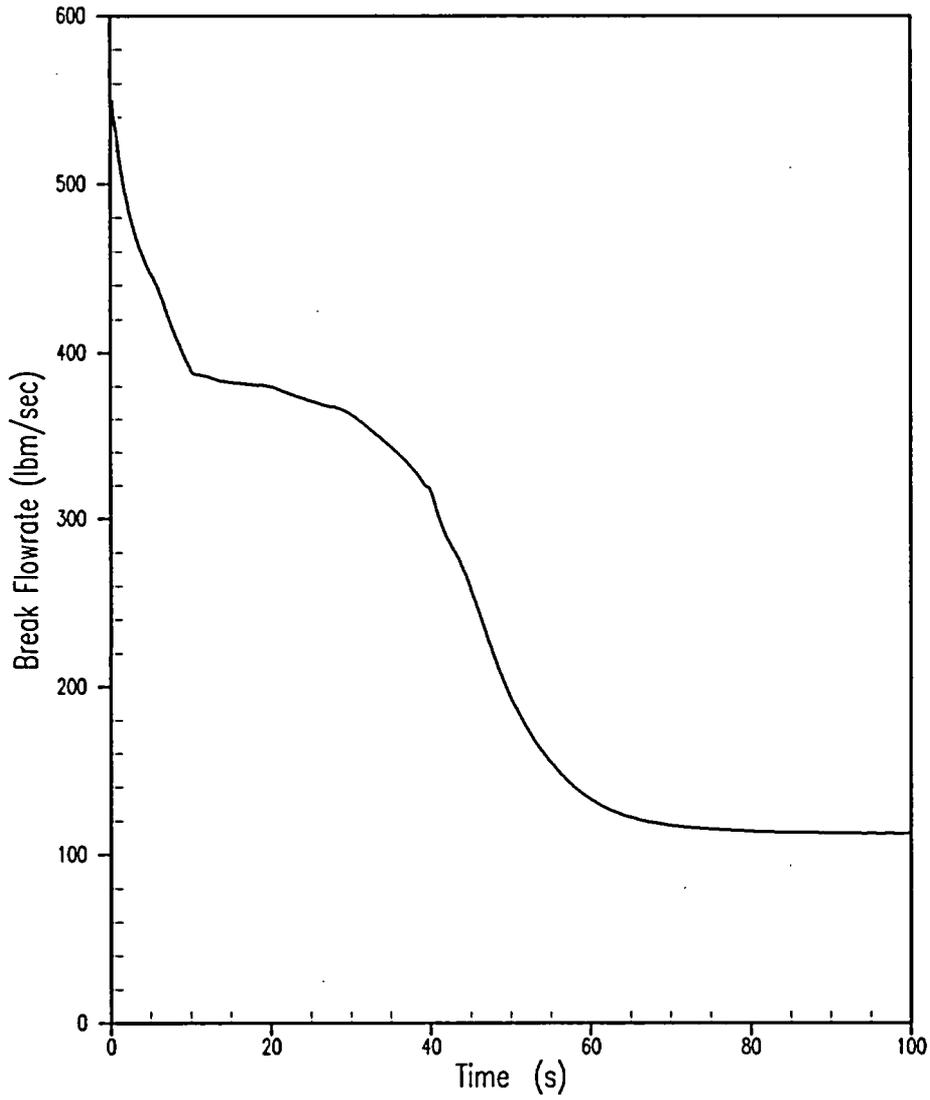
Figure 5.1.12-13 Feedwater Line Break MSS Overpressure Case Limiting Break Size = 0.05 ft<sup>2</sup>
