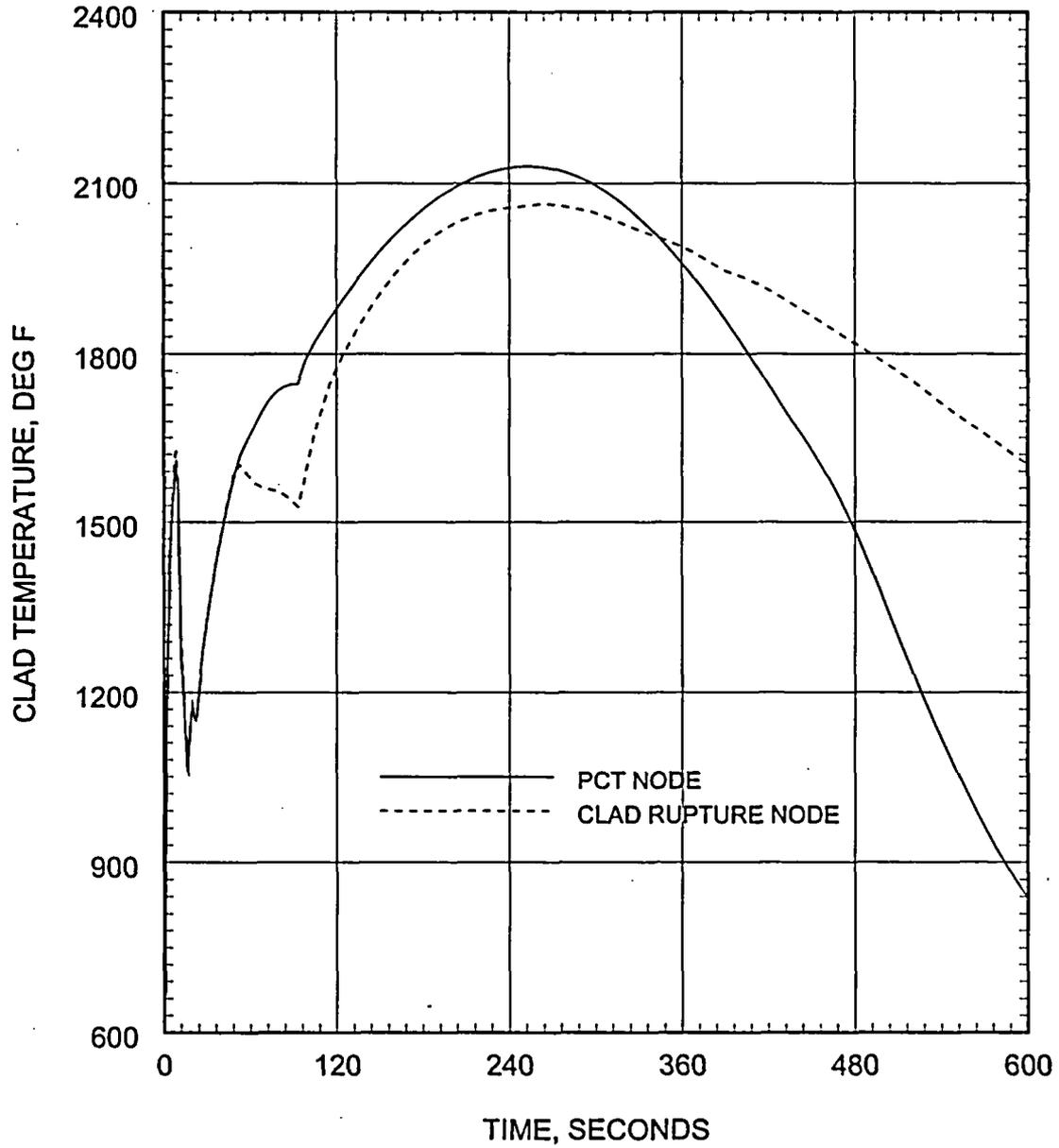
Figure 5.2.3.3-27 Large Break LOCA ECCS Performance Analysis 0.6 DEG/PD Break Peak Cladding Temperature
