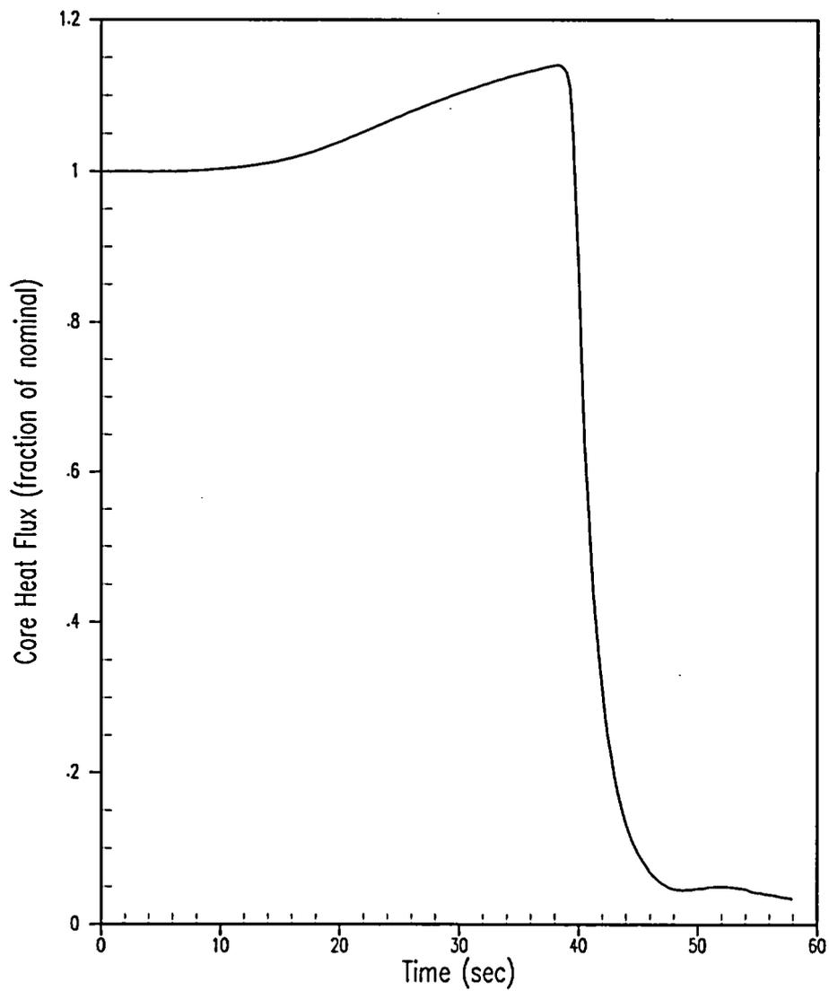
**Figure 5.1.3-2 Core Heat Flux for a Feedwater Malfunction Reduced Feedwater Temperature at HFP Initial Conditions**
