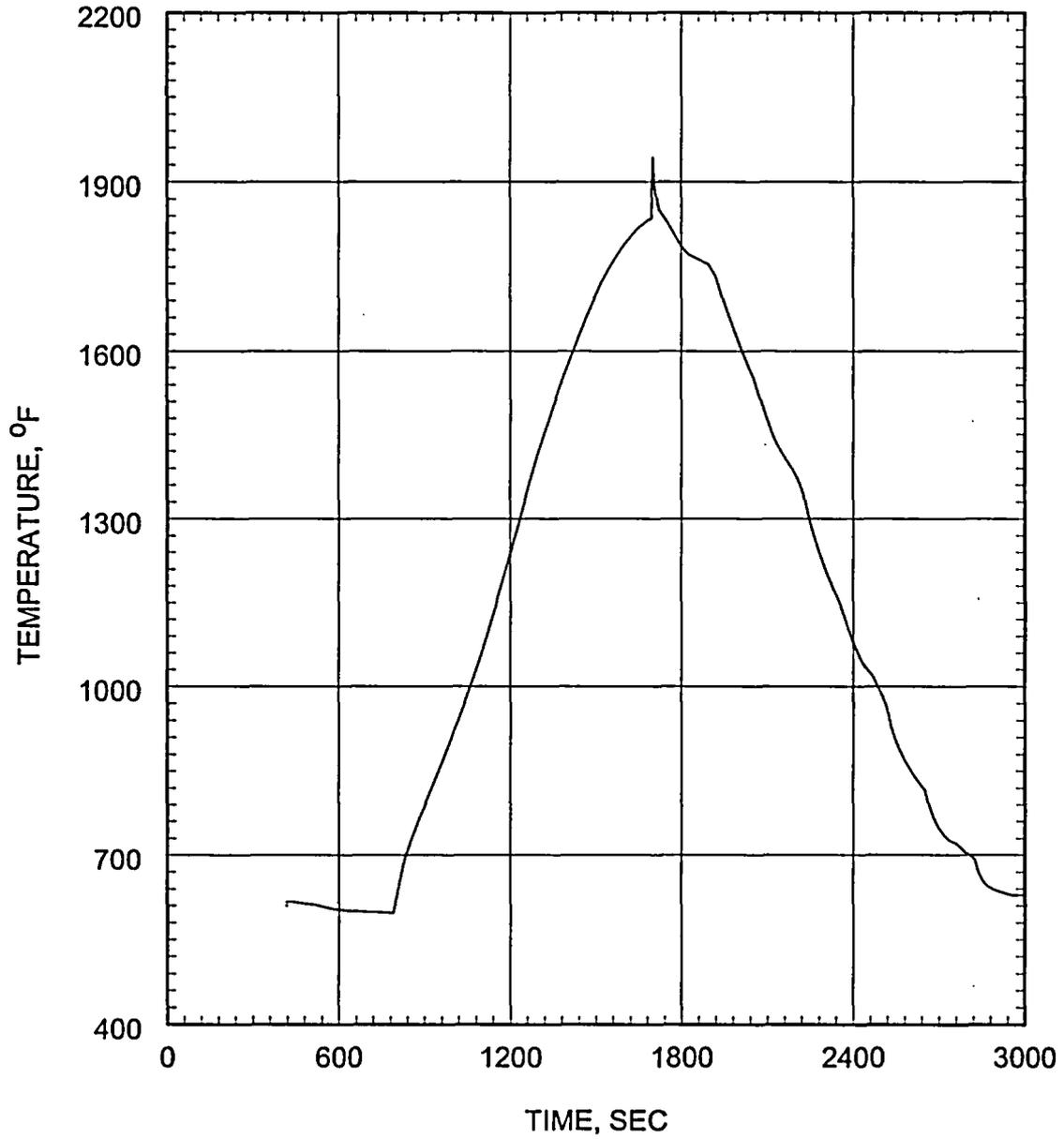
Figure 5.2.4.3-16 Small Break LOCA ECCS Performance Analysis 0.05 ft<sup>2</sup>/PD Break Cladding
