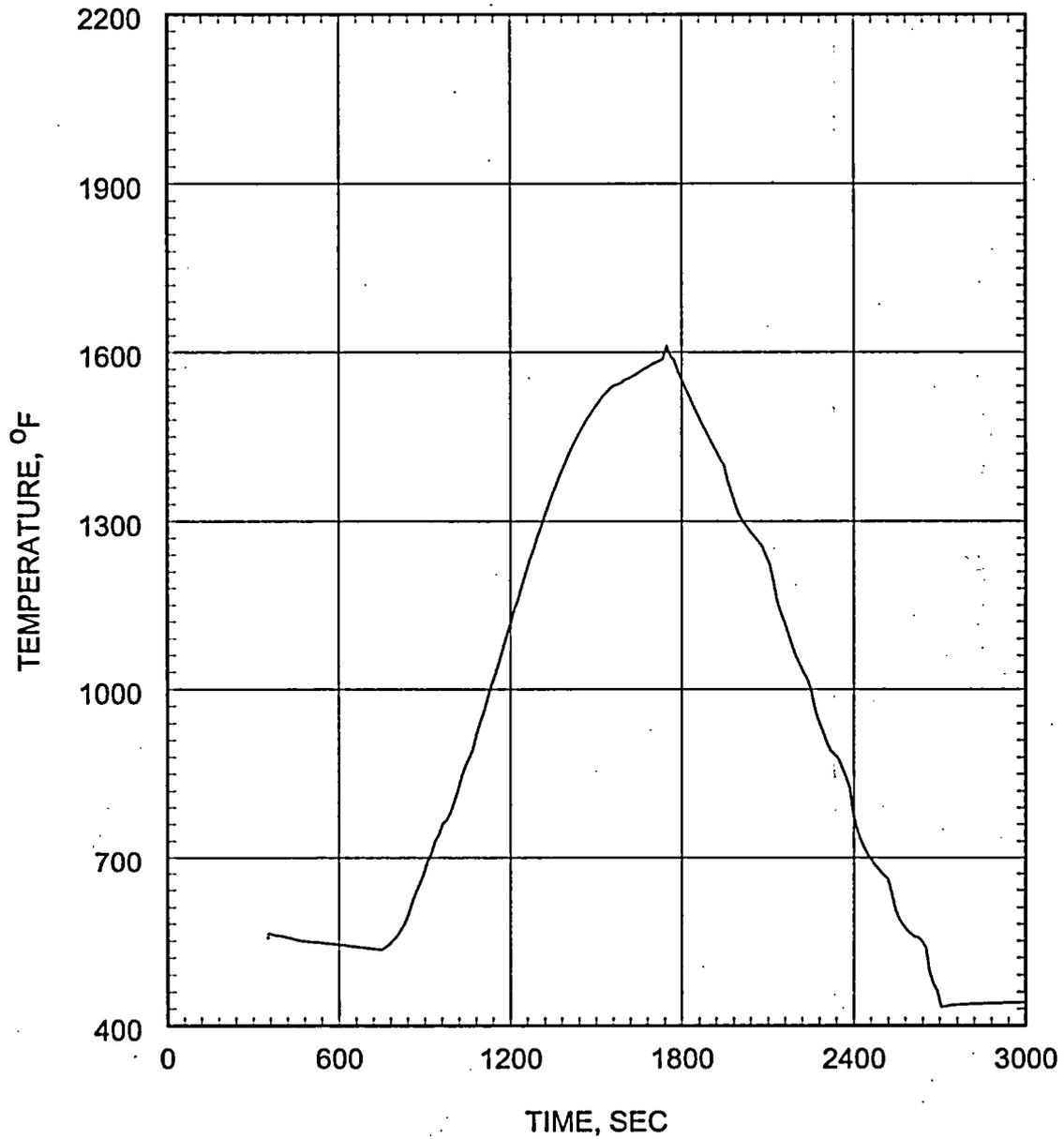
Figure 5.2.4.3-23 Small Break LOCA ECCS Performance Analysis 0.06 ft<sup>2</sup>/PD Break Coolant Temperature at Hot Spot
