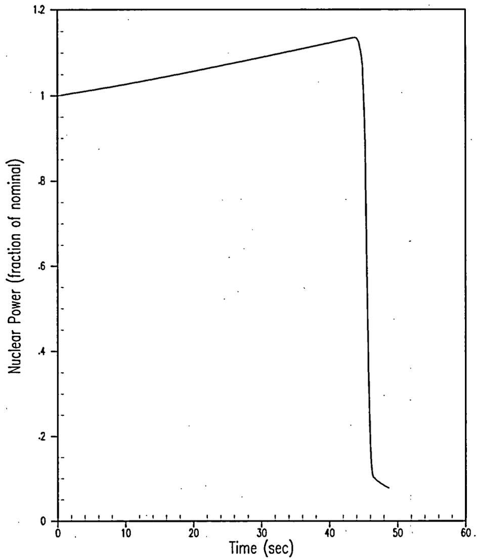
Figure 5.1.16-2 Uncontrolled CEA Bank Withdrawal at Power 100% Power, 2 pcm/sec Reactivity Insertion Rate & Minimum Feedback Variable High Power Trip & Maximum Nominal RCS Vessel  $T_{avg}$  (Sheet 1 of 4)
