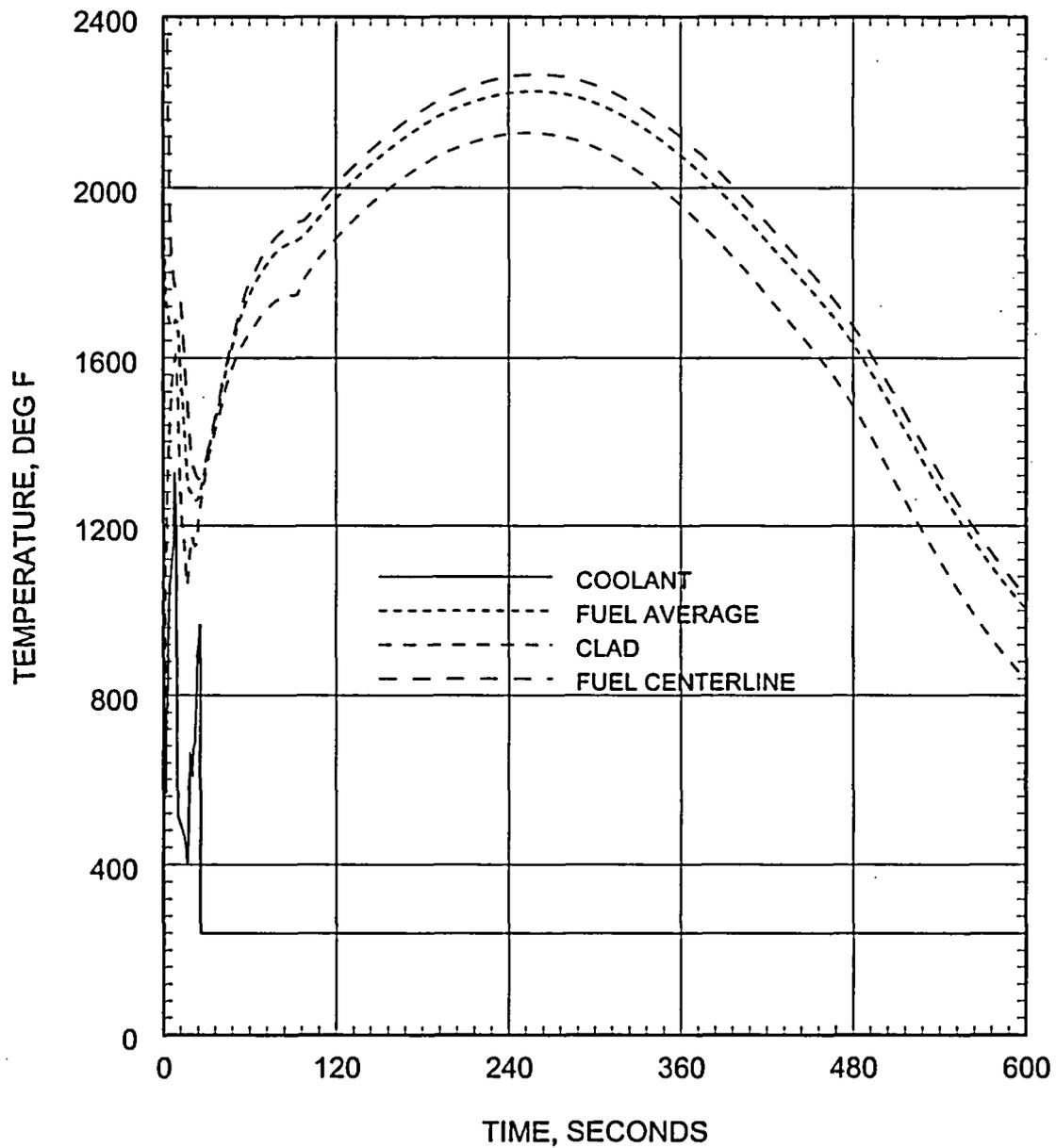
Figure 5.2.3.3-35 Large Break LOCA ECCS Performance Analysis 0.6 DEG/PD Break Fuel Centerline, Fuel Average, Cladding, and Coolant Temperature at the Hot Spot
