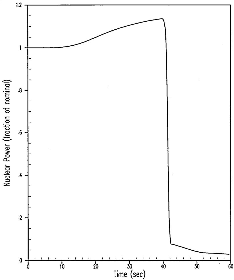
**Figure 5.1.1-1 Nuclear Power for a Feedwater Malfunction Increased Feedwater Flow at HFP Initial Conditions**
