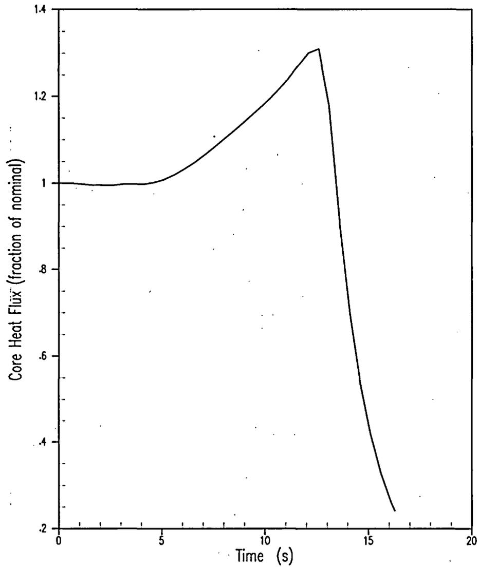
Figure 5.1.5-3 Pre-Trip Main Steamline Break – Core Heat Flux versus Time
