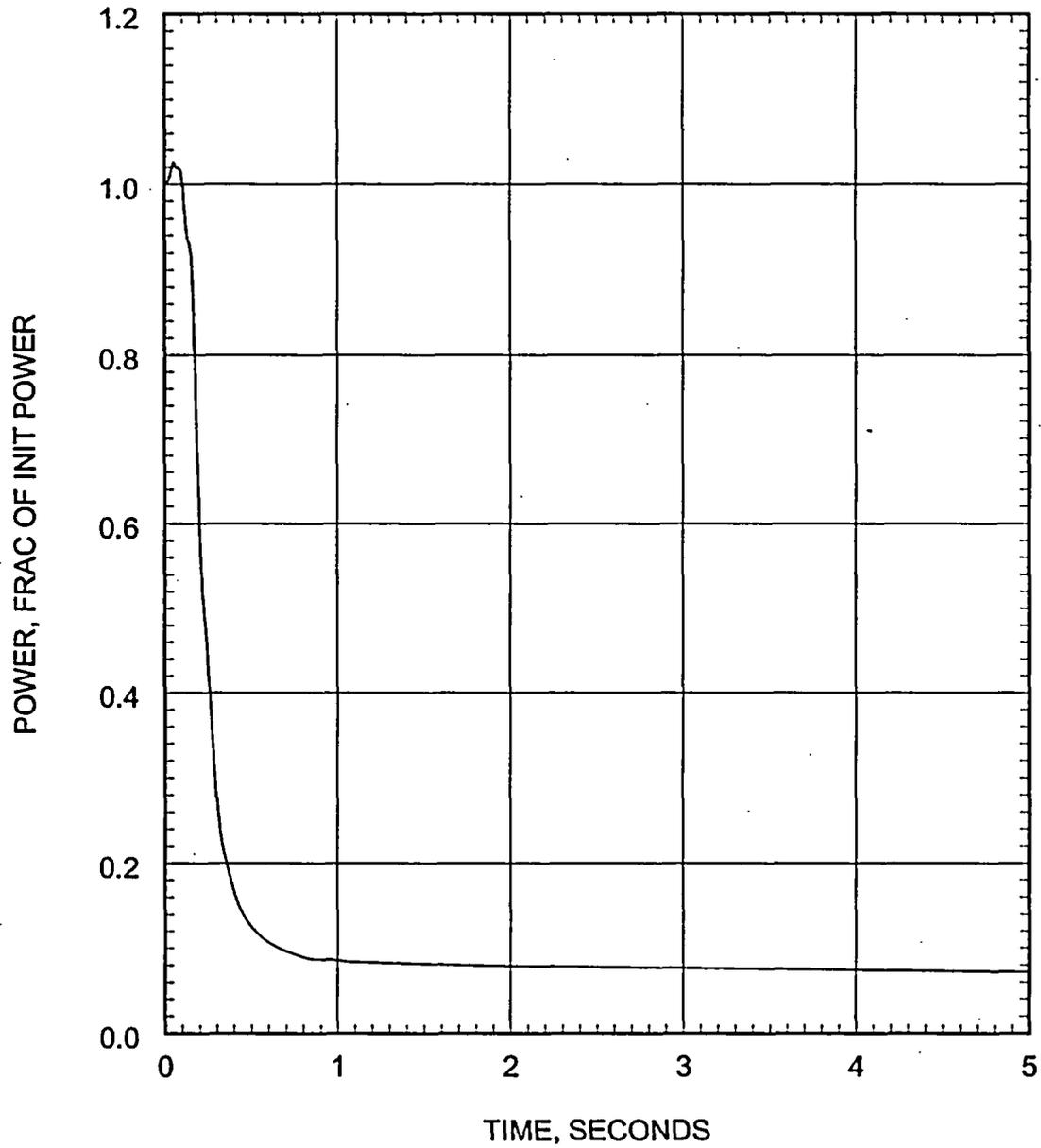
Figure 5.2.3.3-1 Large Break LOCA ECCS Performance Analysis 1.0 DEG/PD Break Core Power
