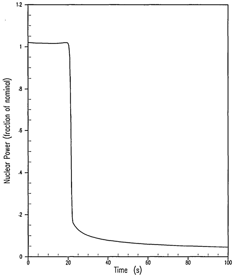
Figure 5.1.10-1 Loss of Condenser Vacuum (RCS Overpressure Case) Nuclear Power
