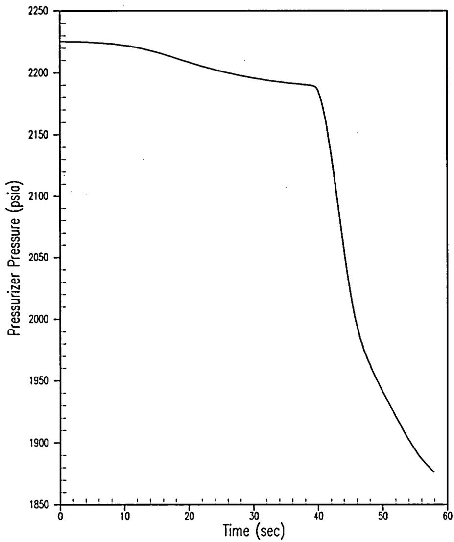
**Figure 5.1.3-4 Pressurizer Pressure for a Feedwater Malfunction Reduced Feedwater Temperature at HFP Initial Conditions**
