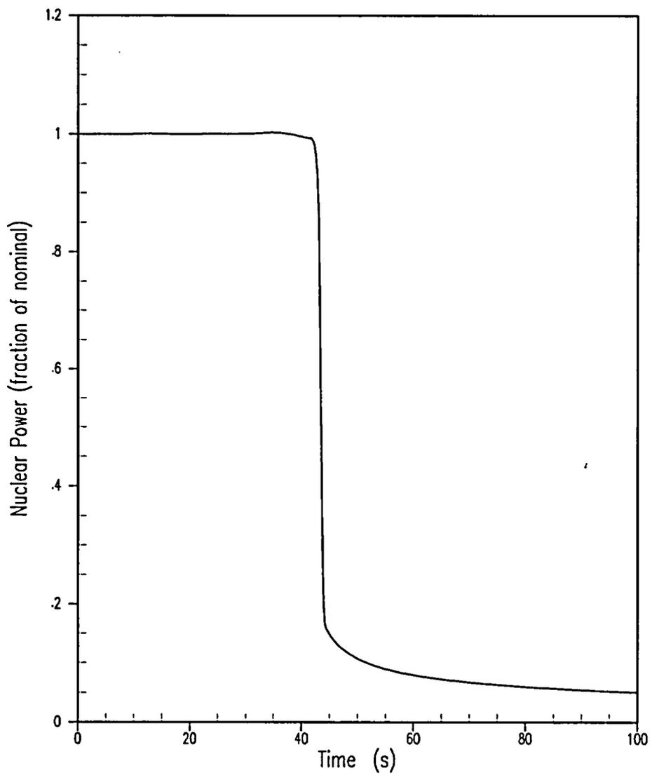
Figure 5.1.12-15 Feedwater Line Break DNB Case Limiting Break Size = 0.25 ft<sup>2</sup> Nuclear Power
