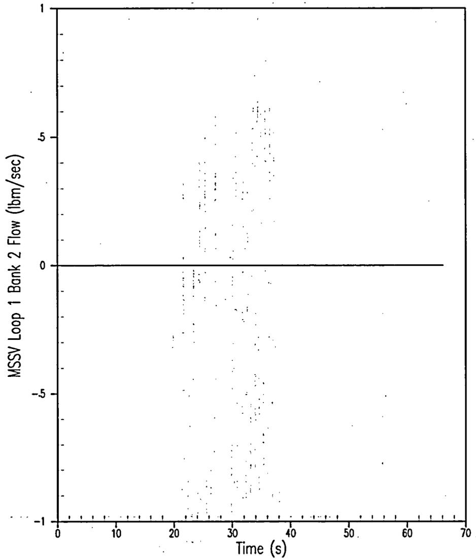
**Figure 5.1.11-10 Main Steam Safety Valve Flow (Loop 1 – Bank 2 Unaffected Steam Generator) for Asymmetric Steam Generator Transient 0% Tube Plugging**
