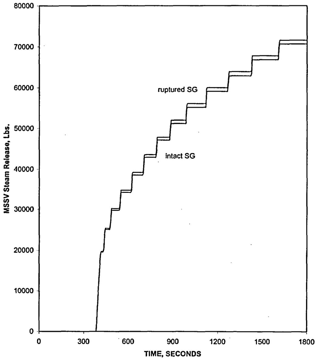
Figure 5.1.24-9 Steam Generator Tube Rupture with Loss of Offsite Power – Steam Release vs. Time
