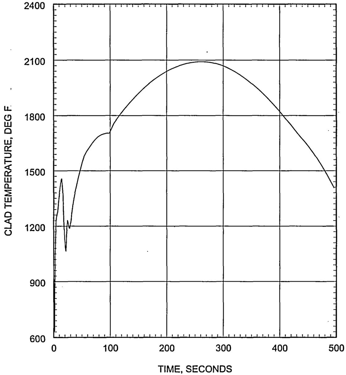
Figure 5.2.3.3-47 Large Break LOCA ECCS Performance Analysis 0.4 DEG/PD Break Peak Cladding Temperature
