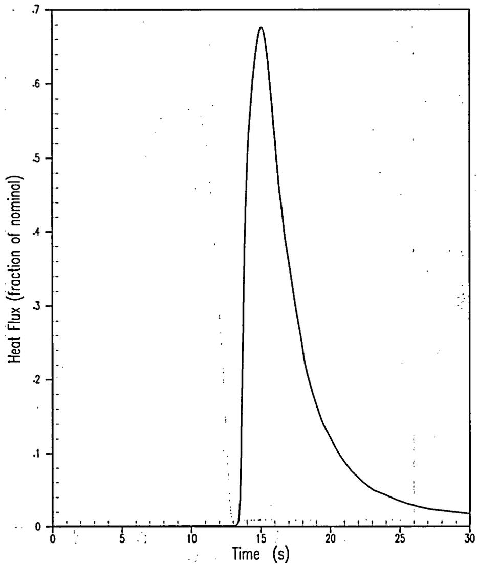
Figure 5.1.17-2 Uncontrolled CEA Withdrawal from a Subcritical Condition – Heat Flux versus Time
