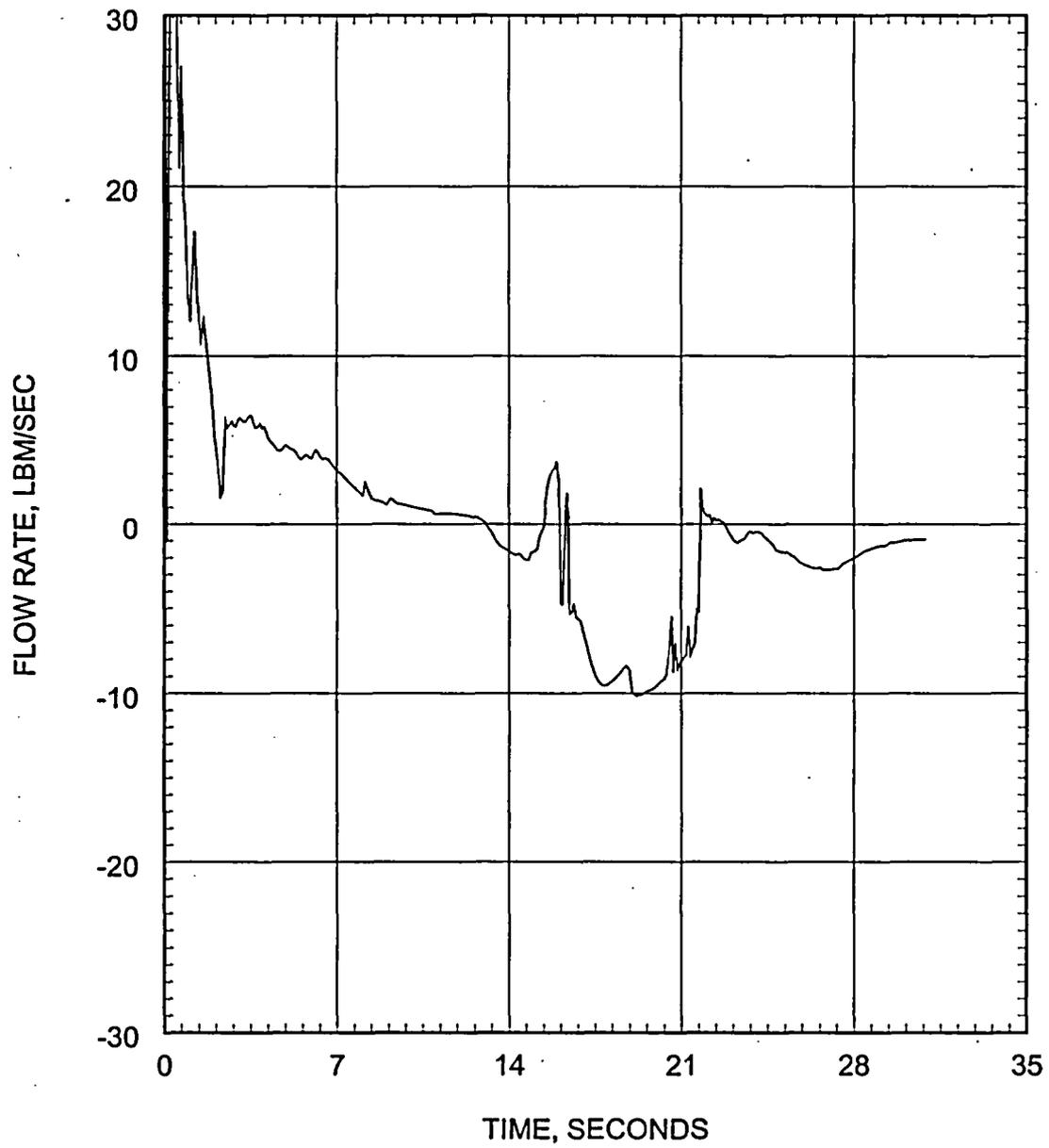
Figure 5.2.3.3-43 Large Break LOCA ECCS Performance Analysis 0.4 DEG/PD Break Hot Assembly Flow Rate (Above Hot Spot)
