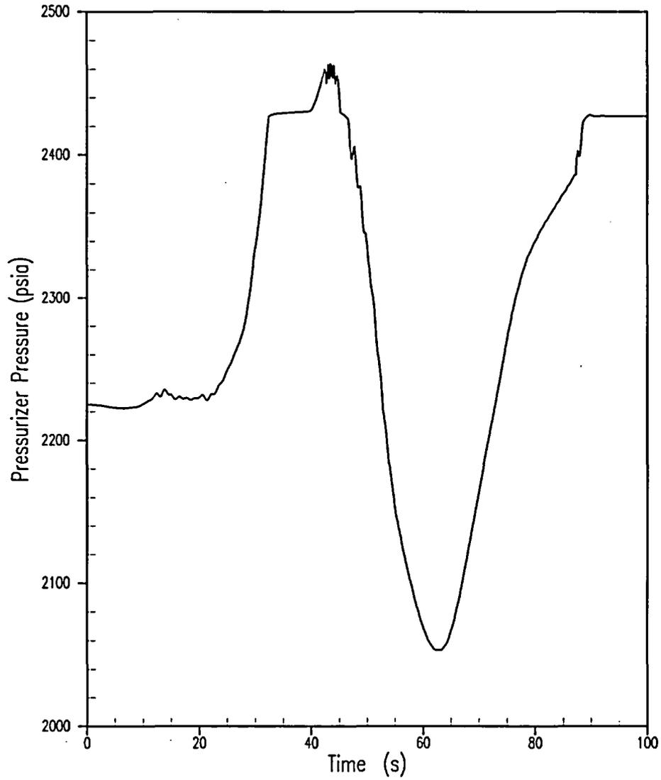
Figure 5.1.12-17 Feedwater Line Break DNB Case Limiting Break Size = 0.25 ft<sup>2</sup> Pressurizer Pressure
