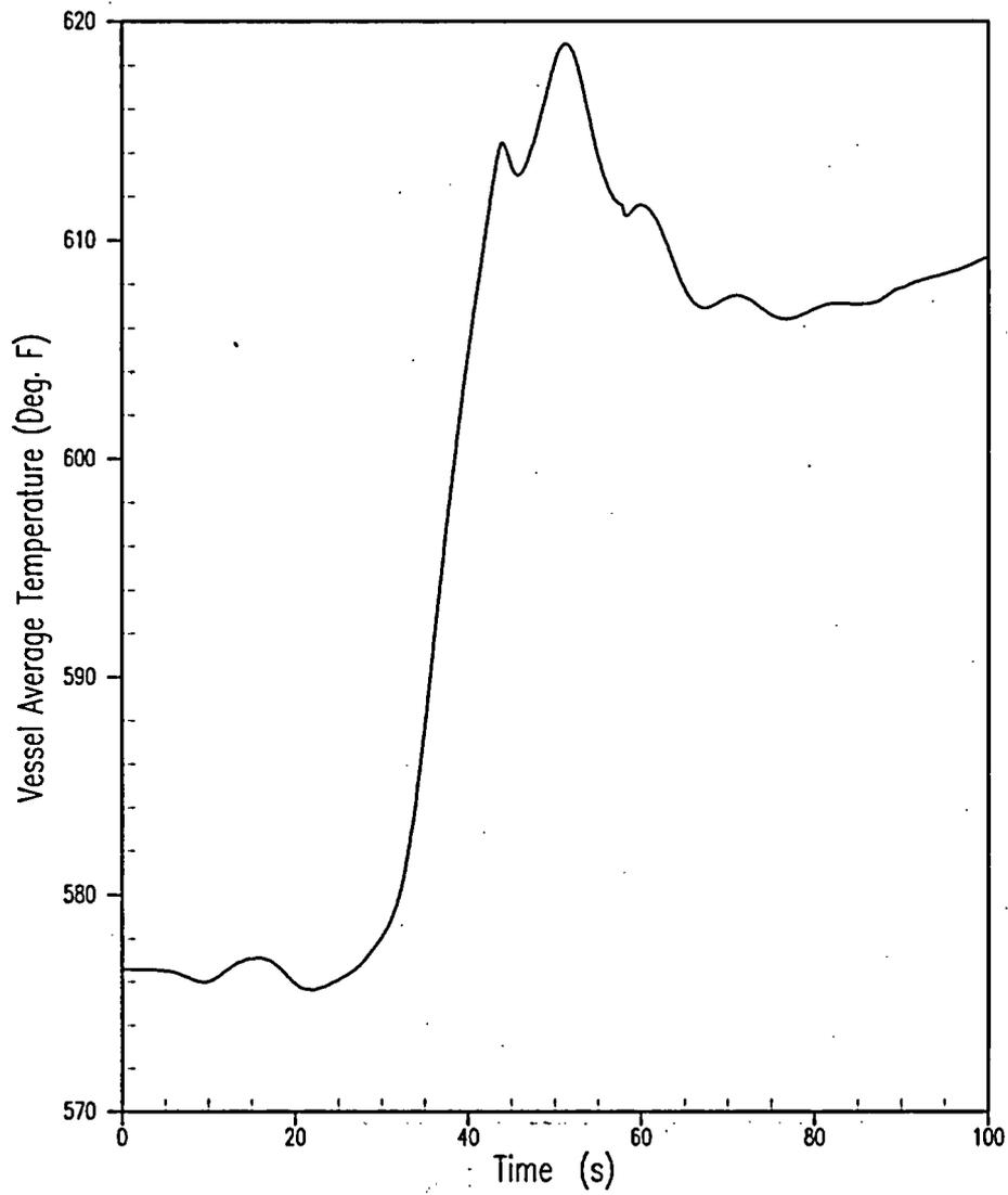
**Figure 5.1.12-18 Feedwater Line Break DNB Case Limiting Break Size = 0.25 ft<sup>2</sup> Vessel Average Temperature**
