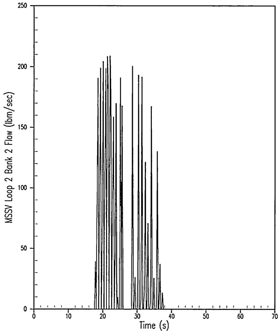
**Figure 5.1.11-11 Main Steam Safety Valve Flow (Loop 2 – Bank 2 Affected Steam Generator) for Asymmetric Steam Generator Transient 0% Tube Plugging**
