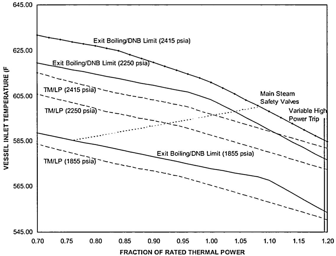
**Figure 5.1.0-2 Core Thermal Limits and Protection Functions
