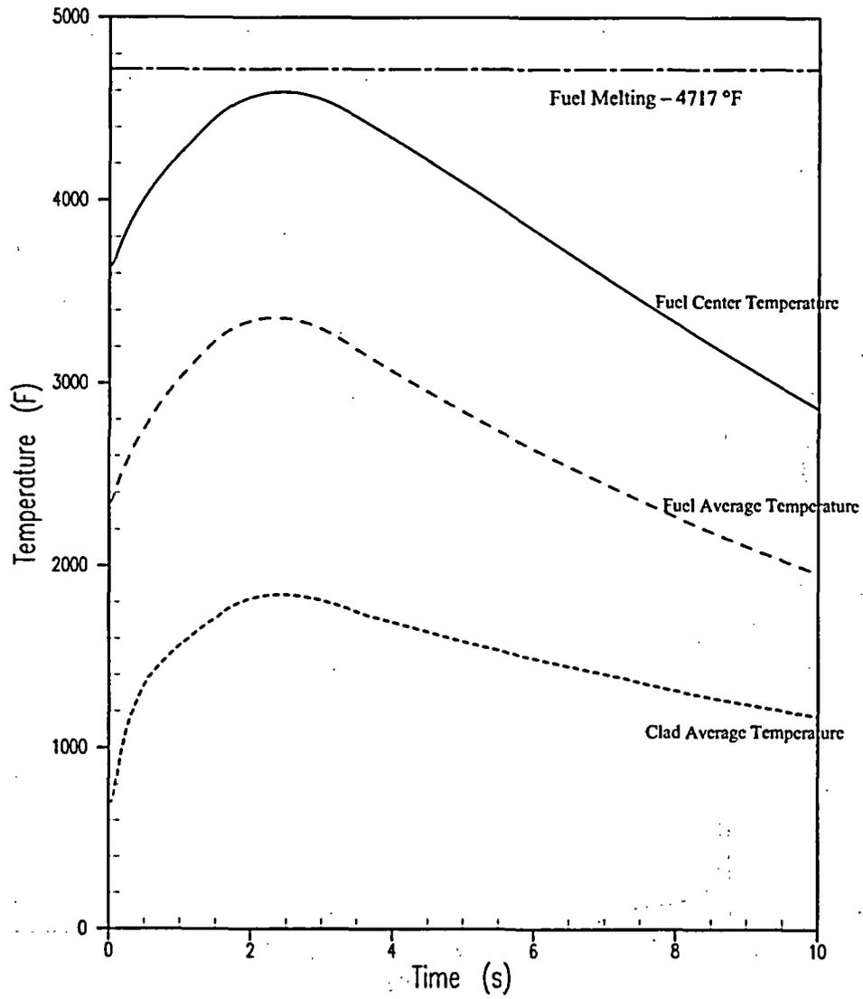
Figure 5.1.20-6 CEA Ejection Accident from Full Power End of Cycle – Fuel and Cladding Temperatures versus Time
