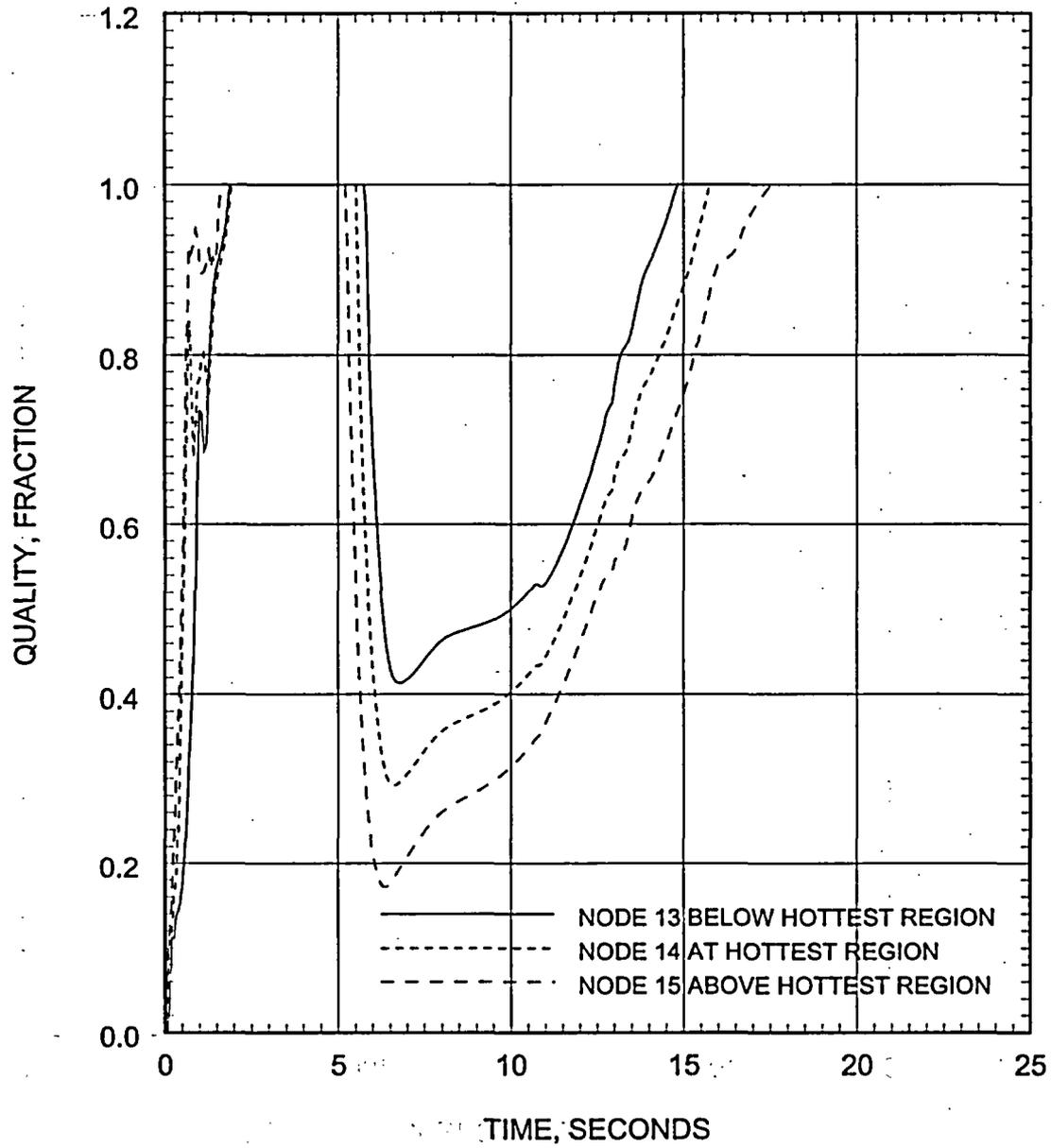
Figure 5.2.3.3-6 Large Break LOCA ECCS Performance Analysis 1.0 DEG/PD Break Hot Assembly Quality
