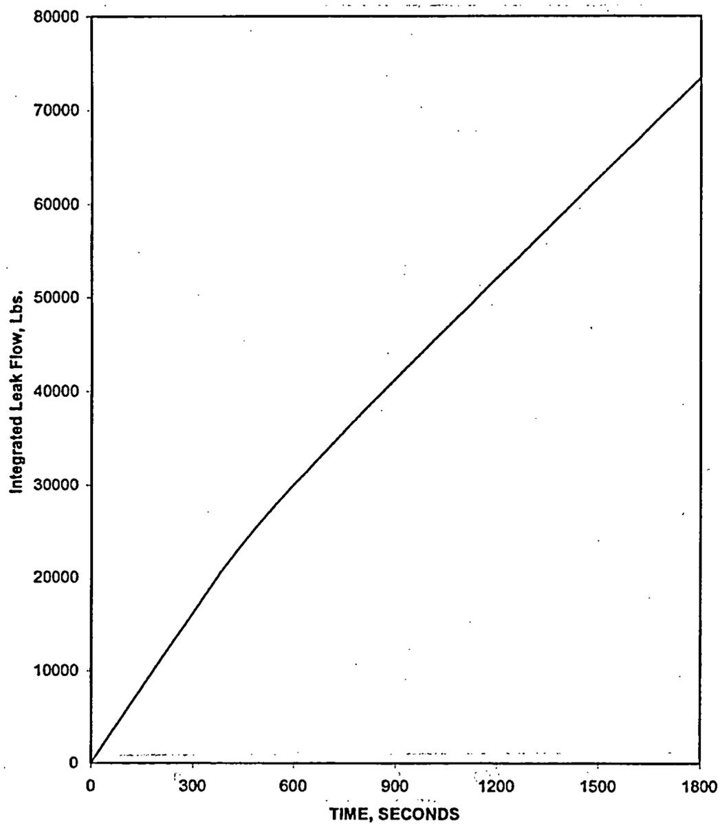
Figure 5.1.24-6 Steam Generator Tube Rupture with Loss of Offsite Power – Integrated Leak Flow vs. Time
