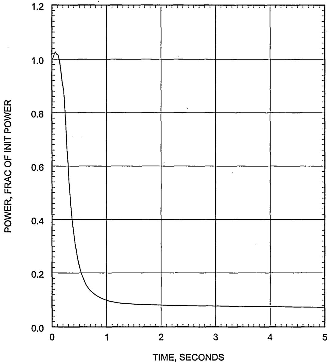
Figure 5.2.3.3-39 Large Break LOCA ECCS Performance Analysis 0.4 DEG/PD Break Core Power
