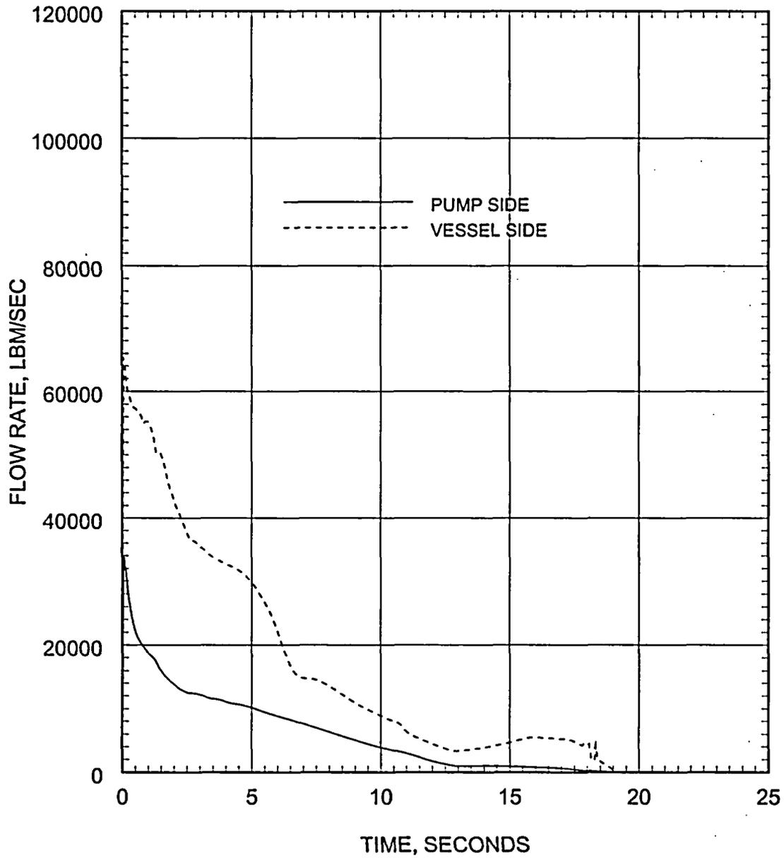
Figure 5.2.3.3-3 Large Break LOCA ECCS Performance Analysis 1.0 DEG/PD Break Leak Flow Rate
