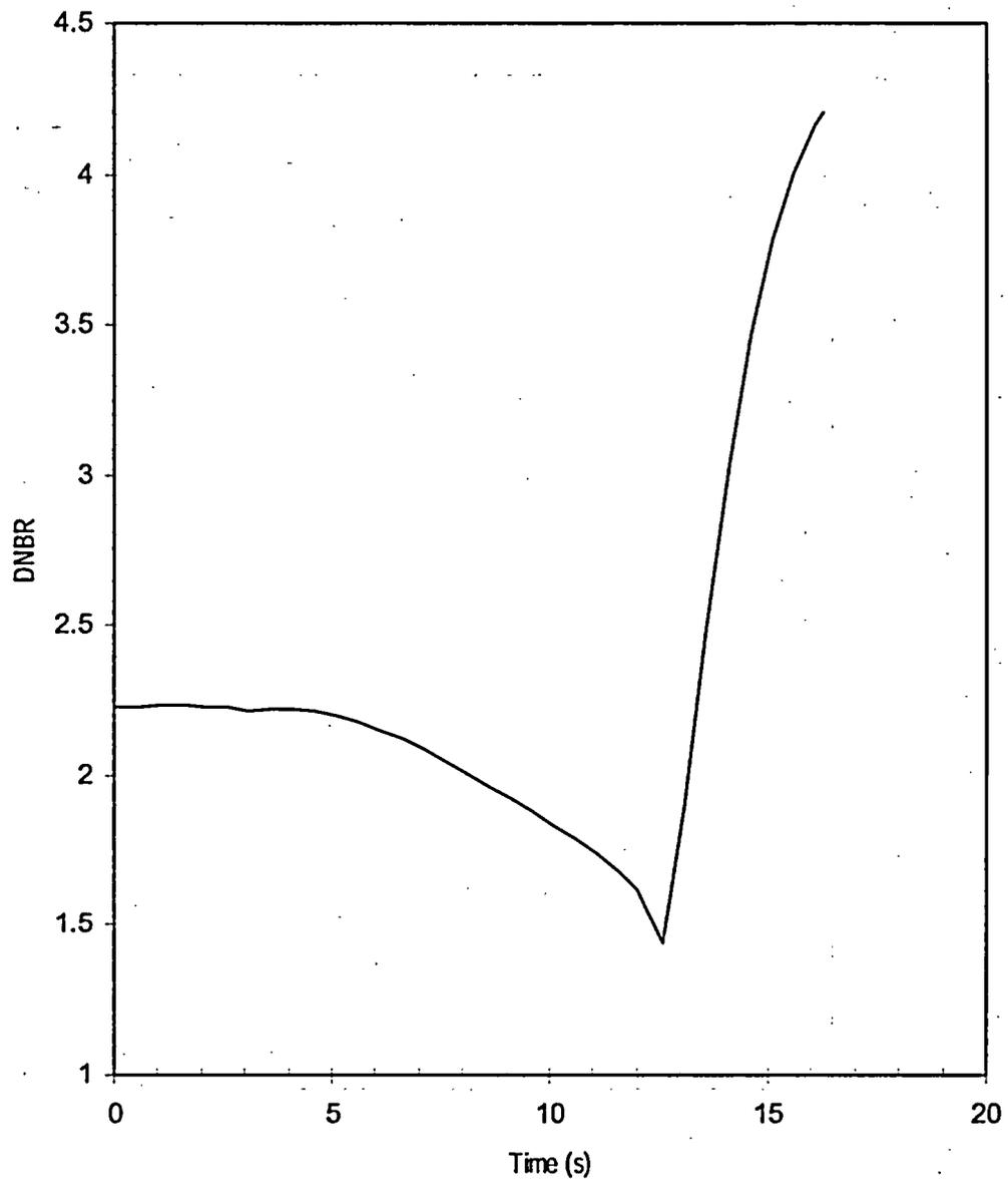
Figure 5.1.5-7 Pre-Trip Main Steamline Break – DNBR versus Time
