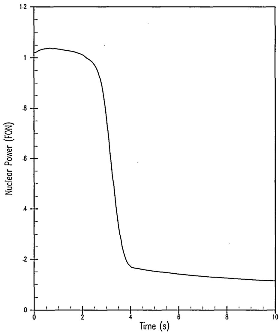
Figure 5.1.15-3 Nuclear Power versus Time – Locked Rotor/Shaft Break
