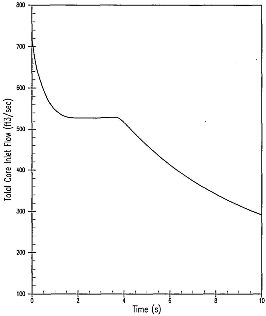
Figure 5.1.15-1 Total Core Inlet Flow versus Time – Locked Rotor/Shaft Break
