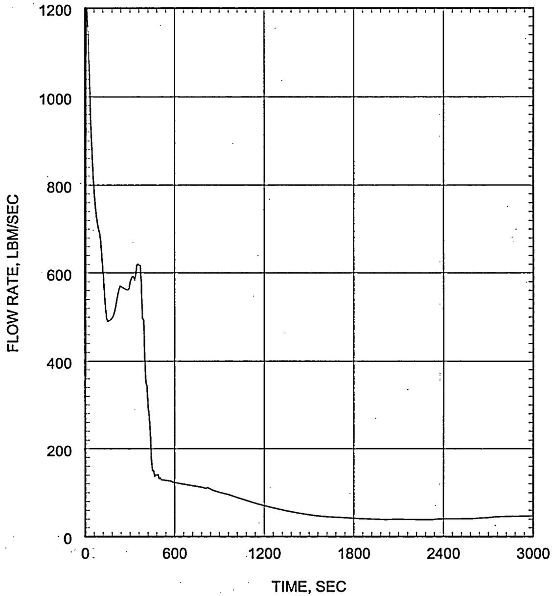
Figure 5.2.4.3-19 Small Break LOCA ECCS Performance Analysis 0.06 ft<sup>2</sup>/PD Break Break Flow Rate
