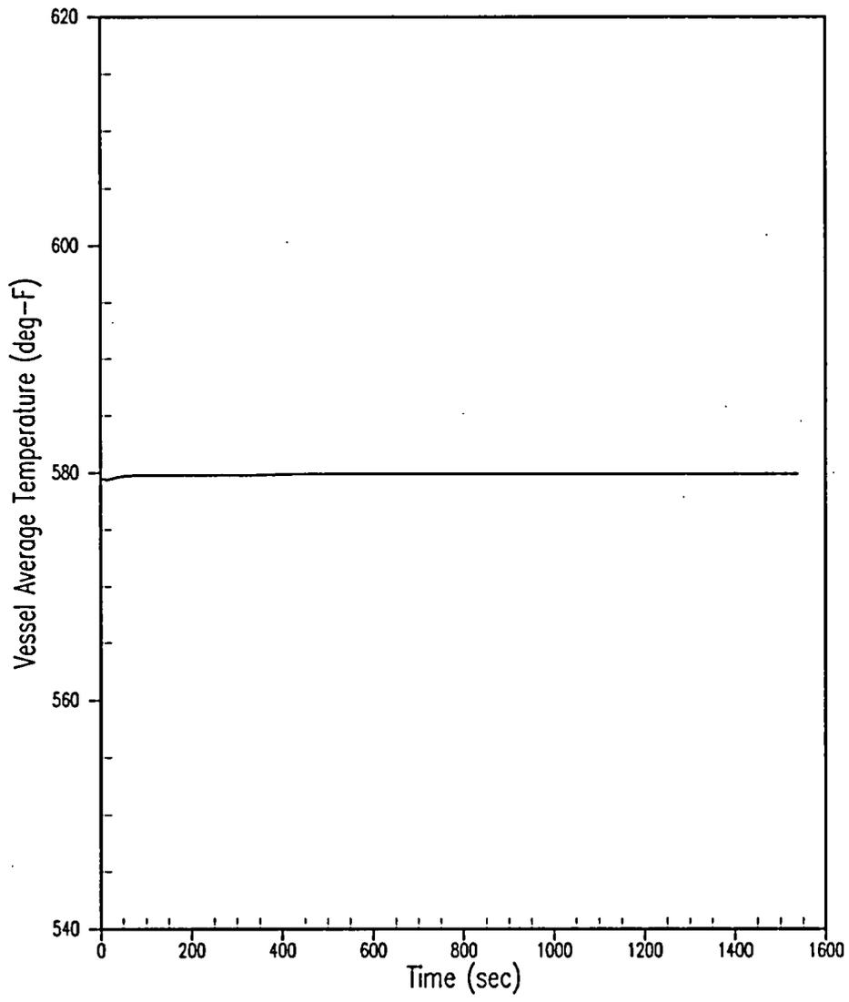
Figure 5.1.21-3 CVCS Malfunction at Power – Vessel Tavg
