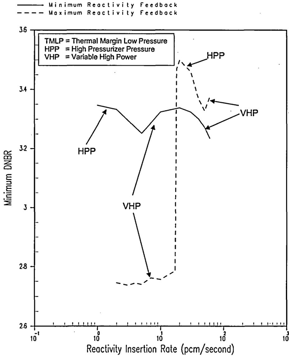
Figure 5.1.16-3 Uncontrolled CEA Bank Withdrawal at Power Initial Power Level of 20%
