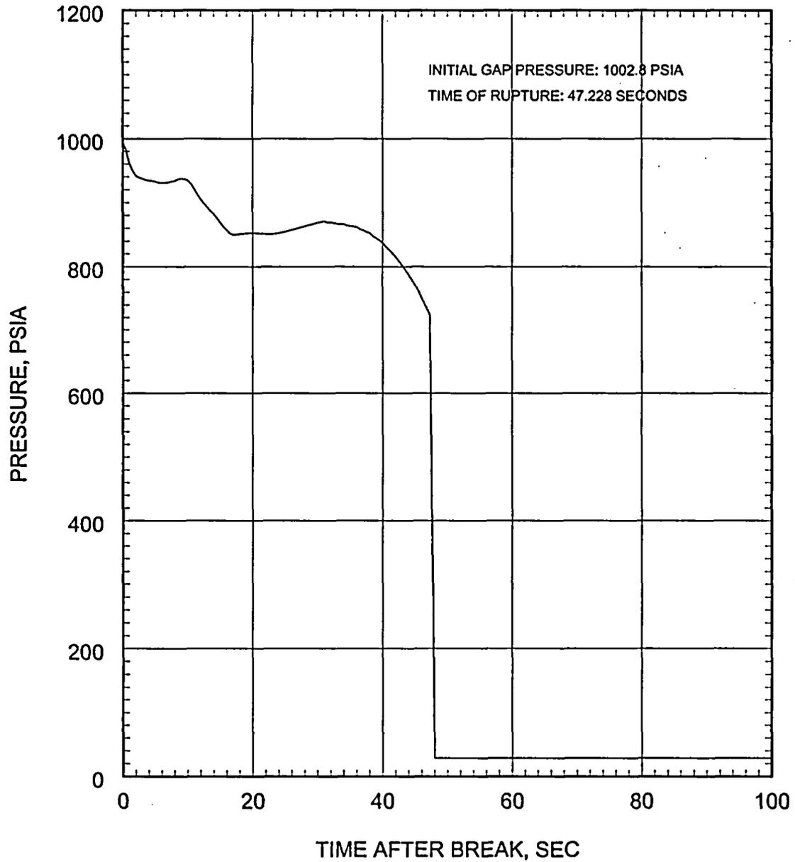
Figure 5.2.3.3-37 Large Break LOCA ECCS Performance Analysis 0.6 DEG/PD Break Hot Rod Internal Gas Pressure
