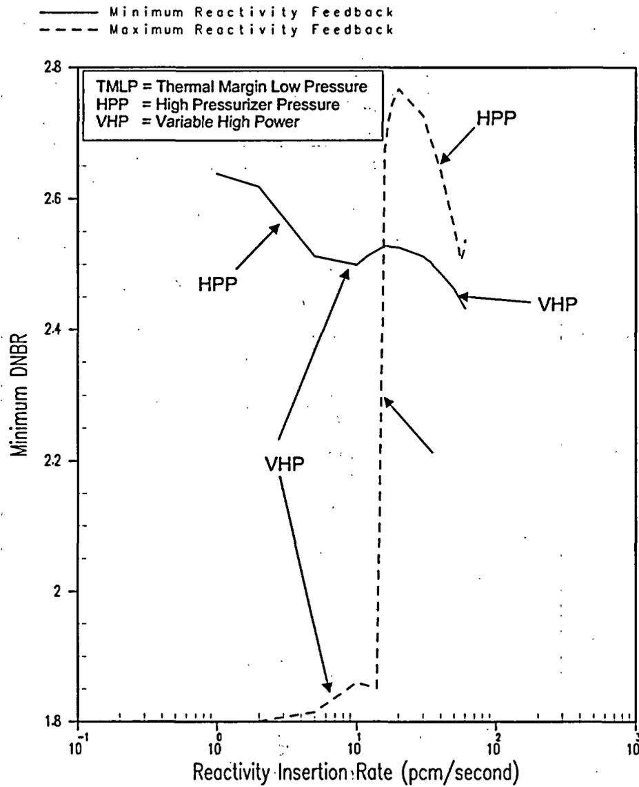
Figure 5.1.16-3 Uncontrolled CEA Bank Withdrawal at Power Initial Power Level of 50%
