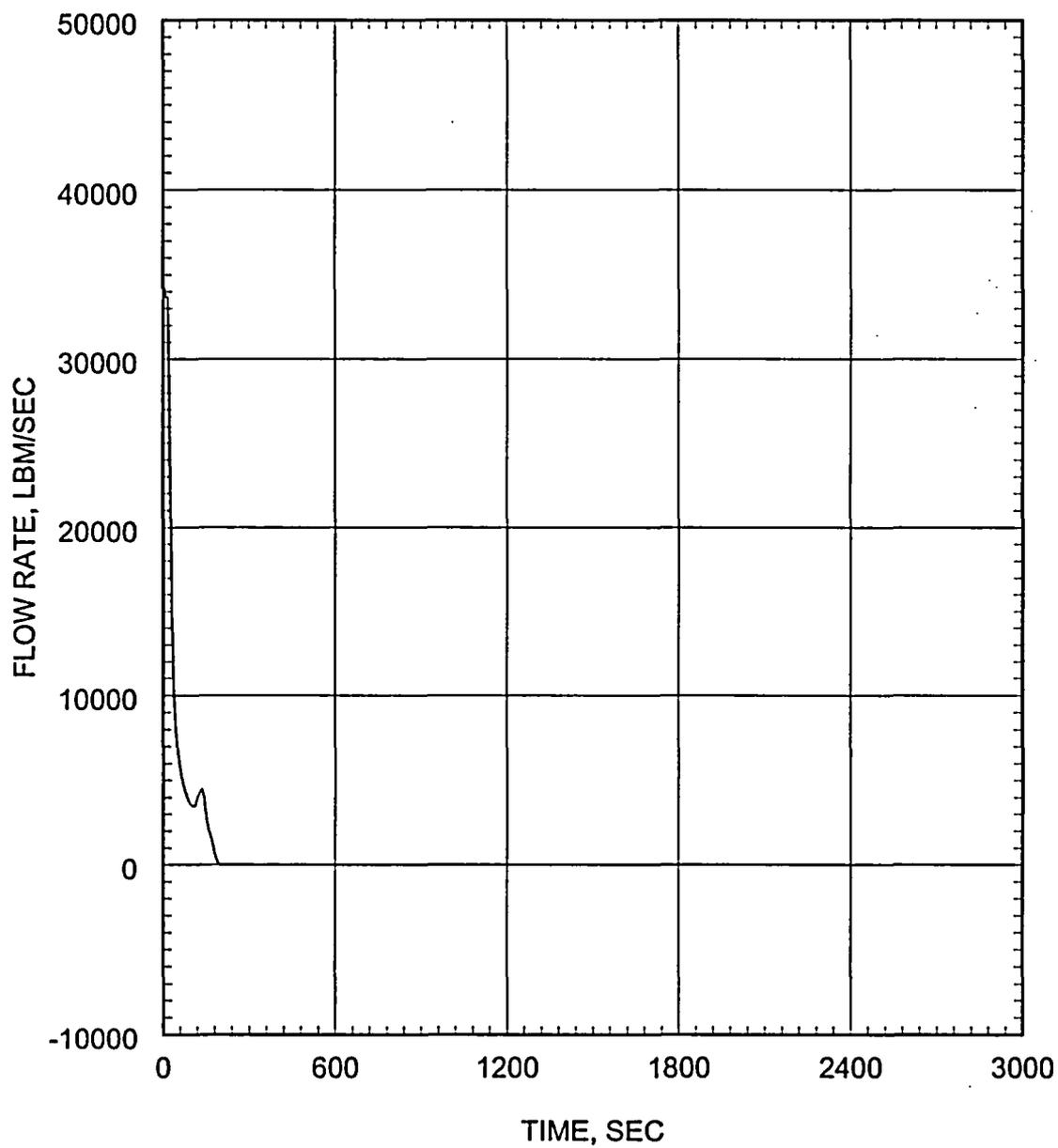
Figure 5.2.4.3-20 Small Break LOCA ECCS Performance Analysis 0.06 ft<sup>2</sup>/PD Break Inner Vessel Inlet Flow Rate
