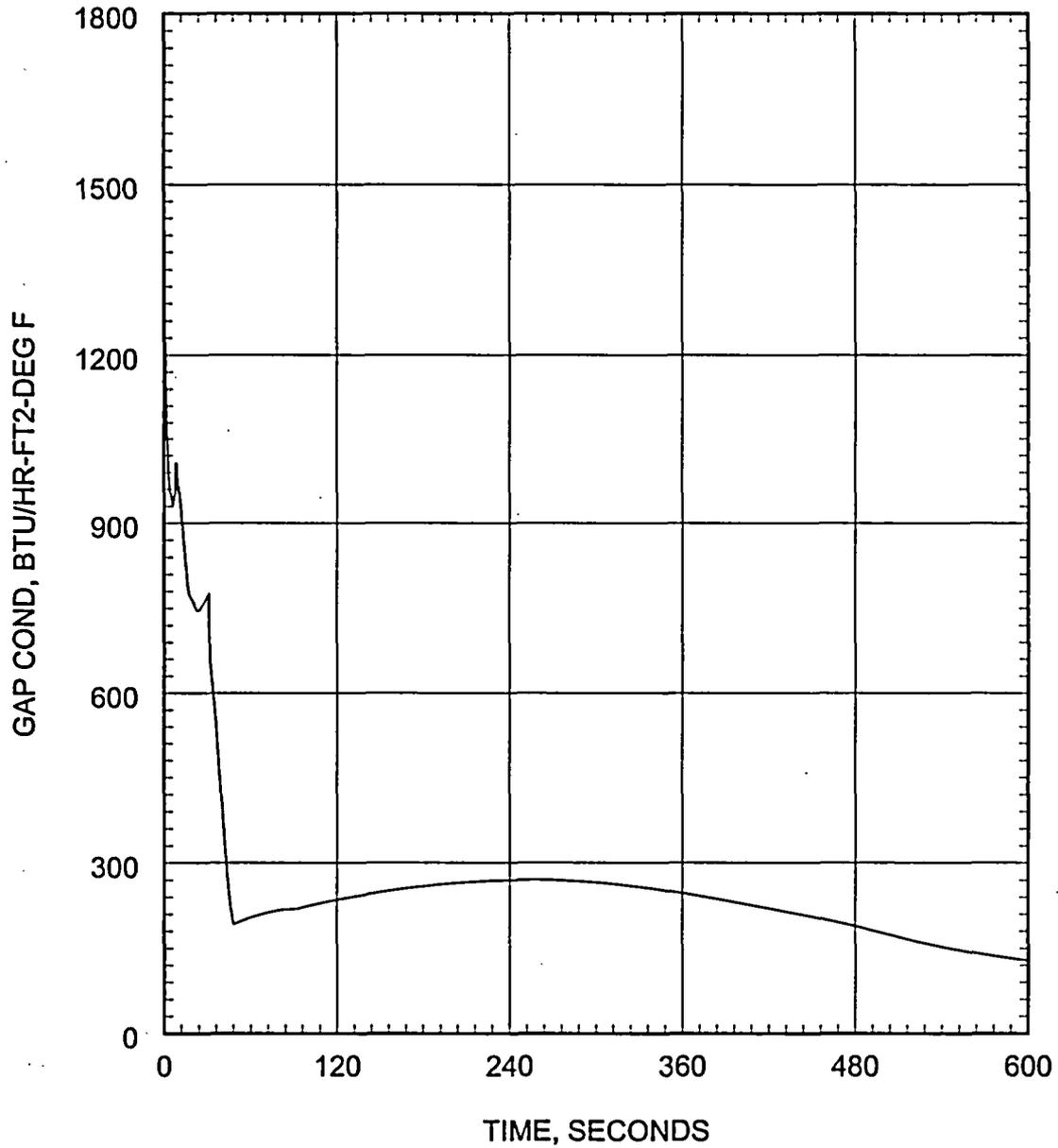
Figure 5.2.3.3-33 Large Break LOCA ECCS Performance Analysis 0.6 DEG/PD Break Hot Spot Gap Conductance
