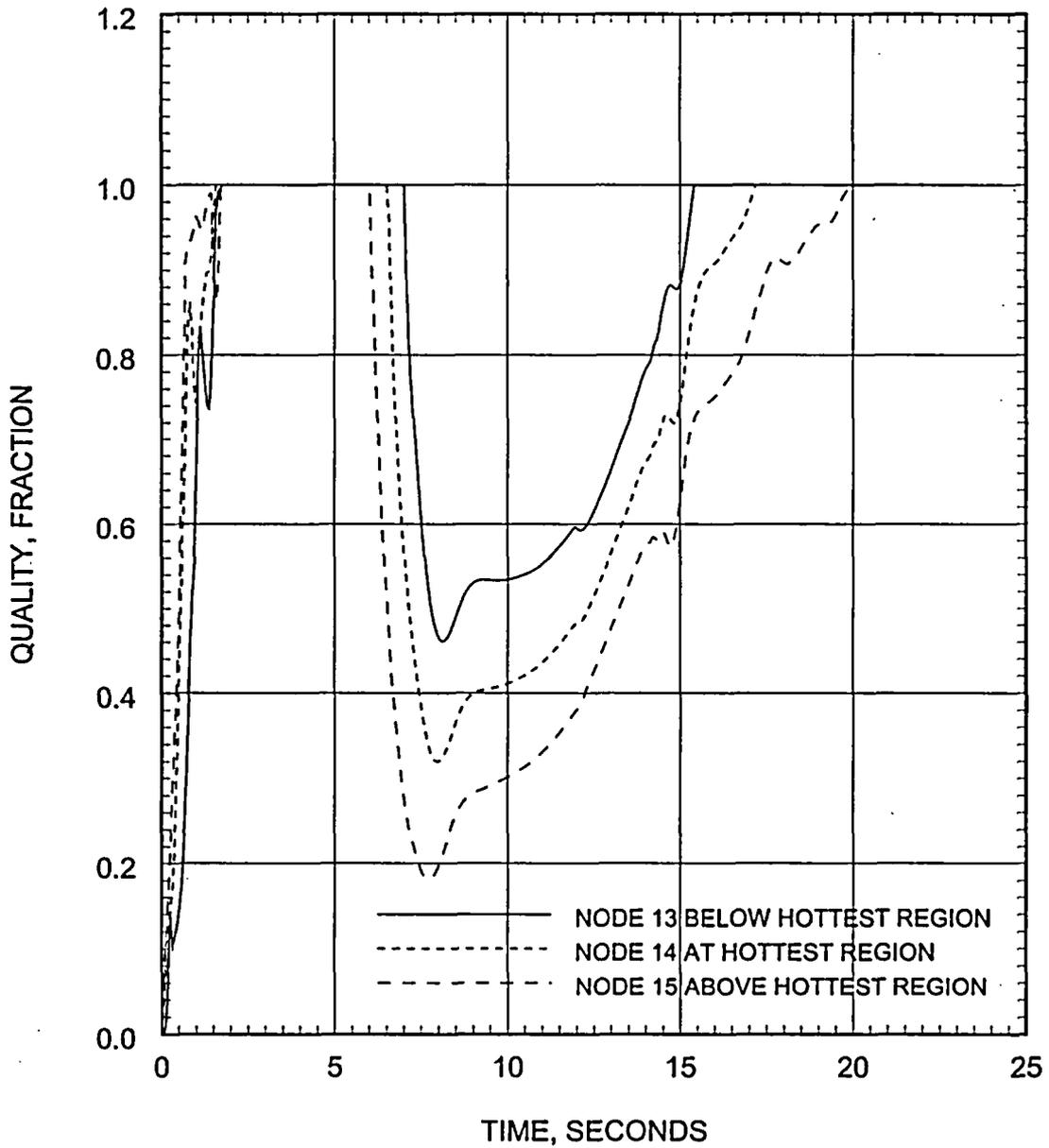
Figure 5.2.3.3-15 Large Break LOCA ECCS Performance Analysis 0.8 DEG/PD Break Hot Assembly Quality
