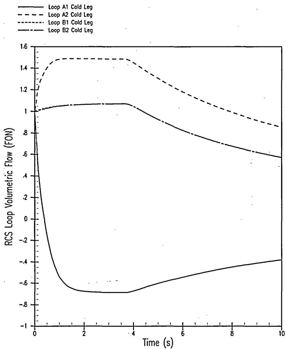
Figure 5.1.15-2 RCS Loop Flow versus Time – Locked Rotor/Shaft Break
