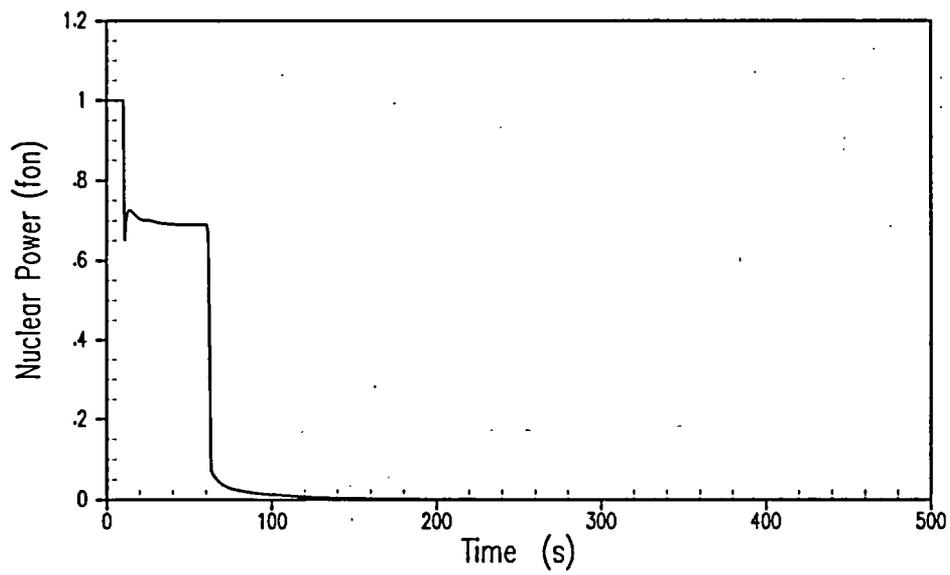
**Figure 5.1.18-1 Representative Transient Response to a Dropped CEA Worth of 500 pcm at a Moderator Temperature Coefficient of 0 pcm/°F – Nuclear Power versus Time**
