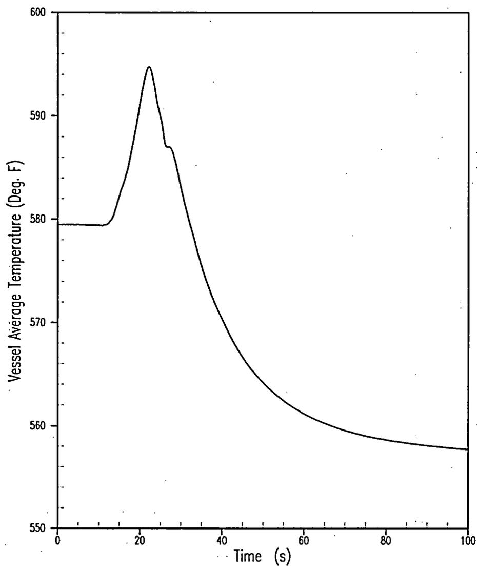
Figure 5.1.10-4 Loss of Condenser Vacuum (RCS Overpressure Case) Vessel Average Temperature
