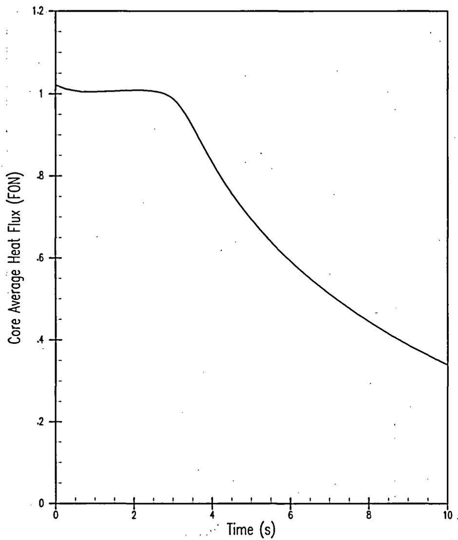
**Figure 5.1.15-4 Core Average Heat Flux versus Time – Locked Rotor/Shaft Break**
