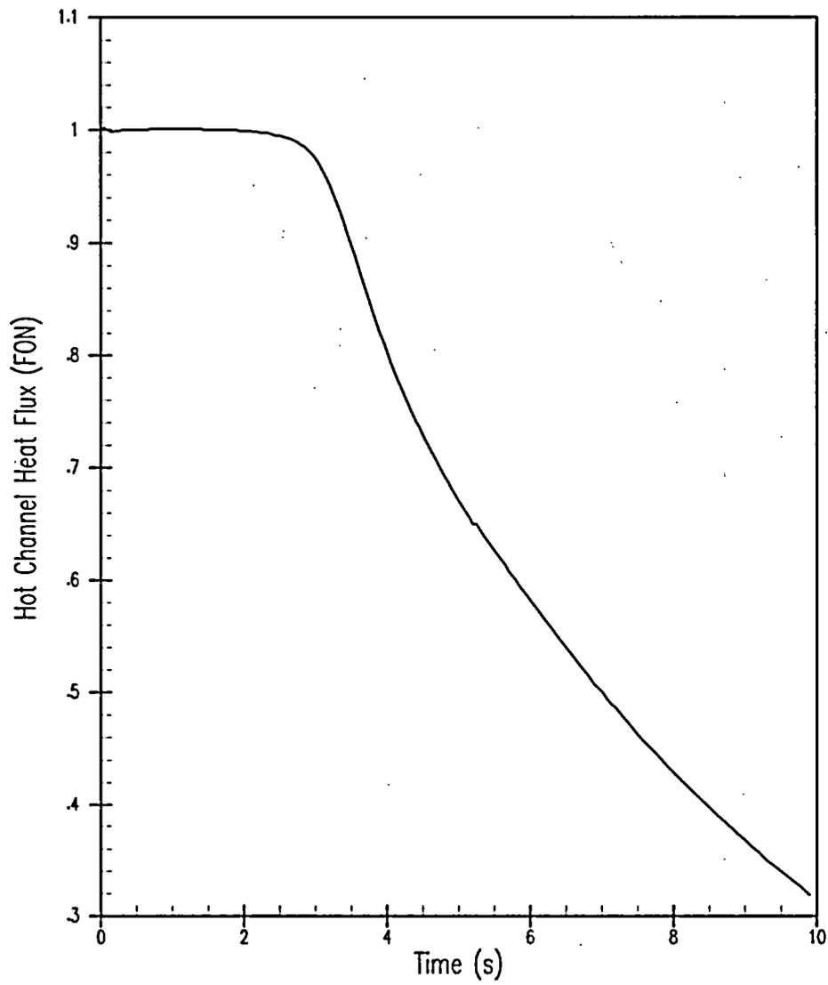
Figure 5.1.15-8 Hot Channel Heat Flux versus Time – Locked Rotor/Shaft Break
