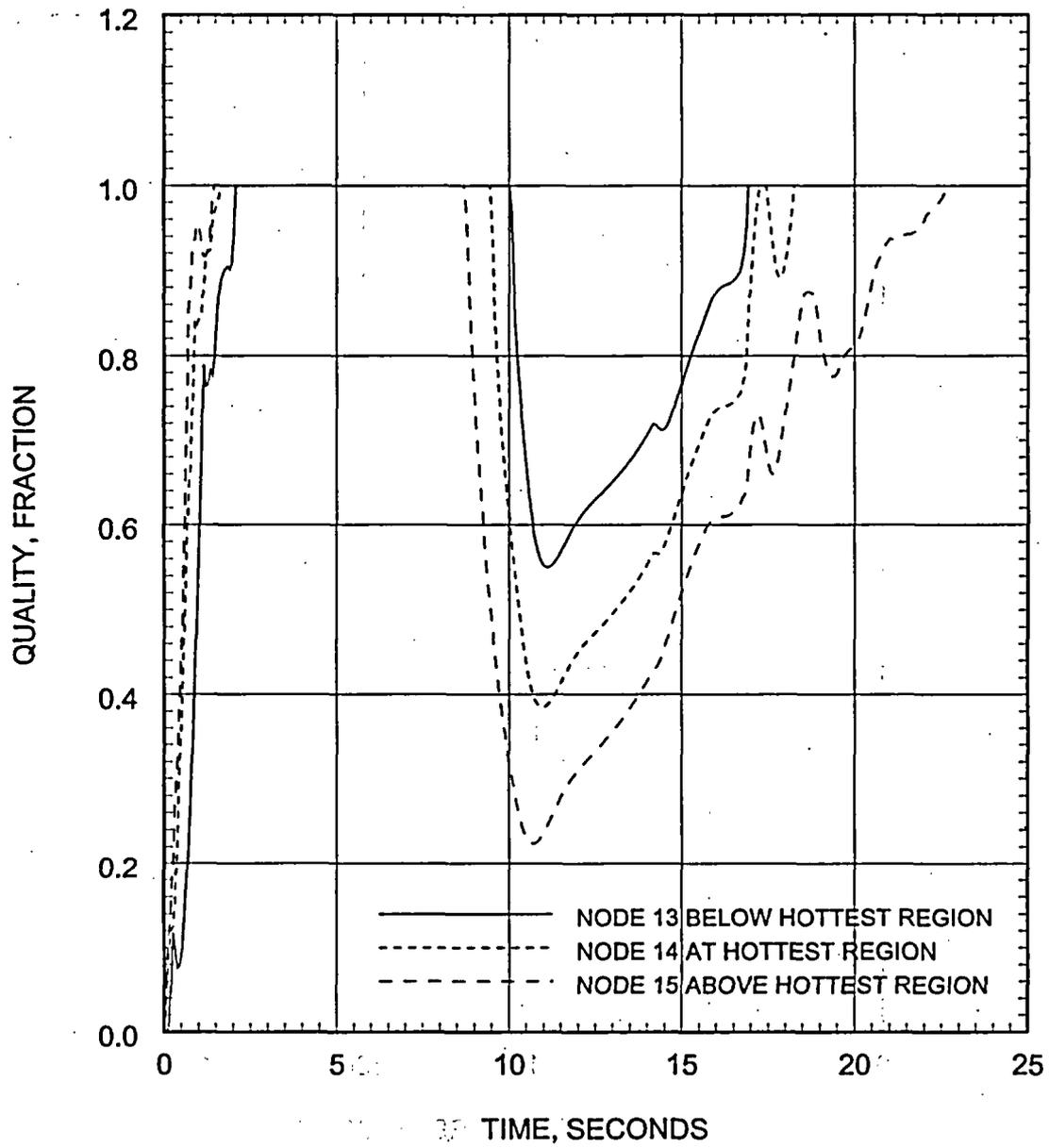
Figure 5.2.3.3-24 Large Break LOCA ECCS Performance Analysis 0.6 DEG/PD Break Hot Assembly Quality
