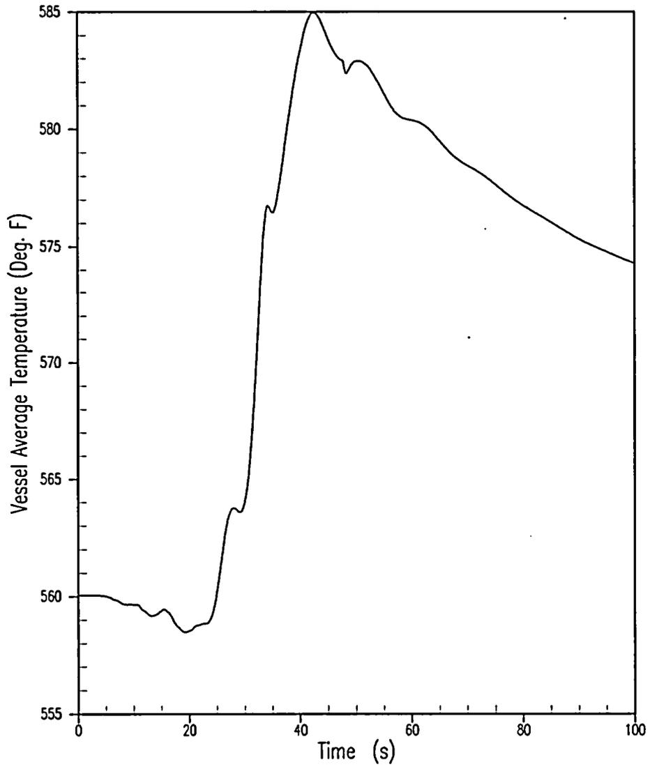
**Figure 5.1.12-3 Feedwater Line Break RCS Overpressure Case Limiting Break Size = 0.28 ft<sup>2</sup> Vessel Average Temperature**
