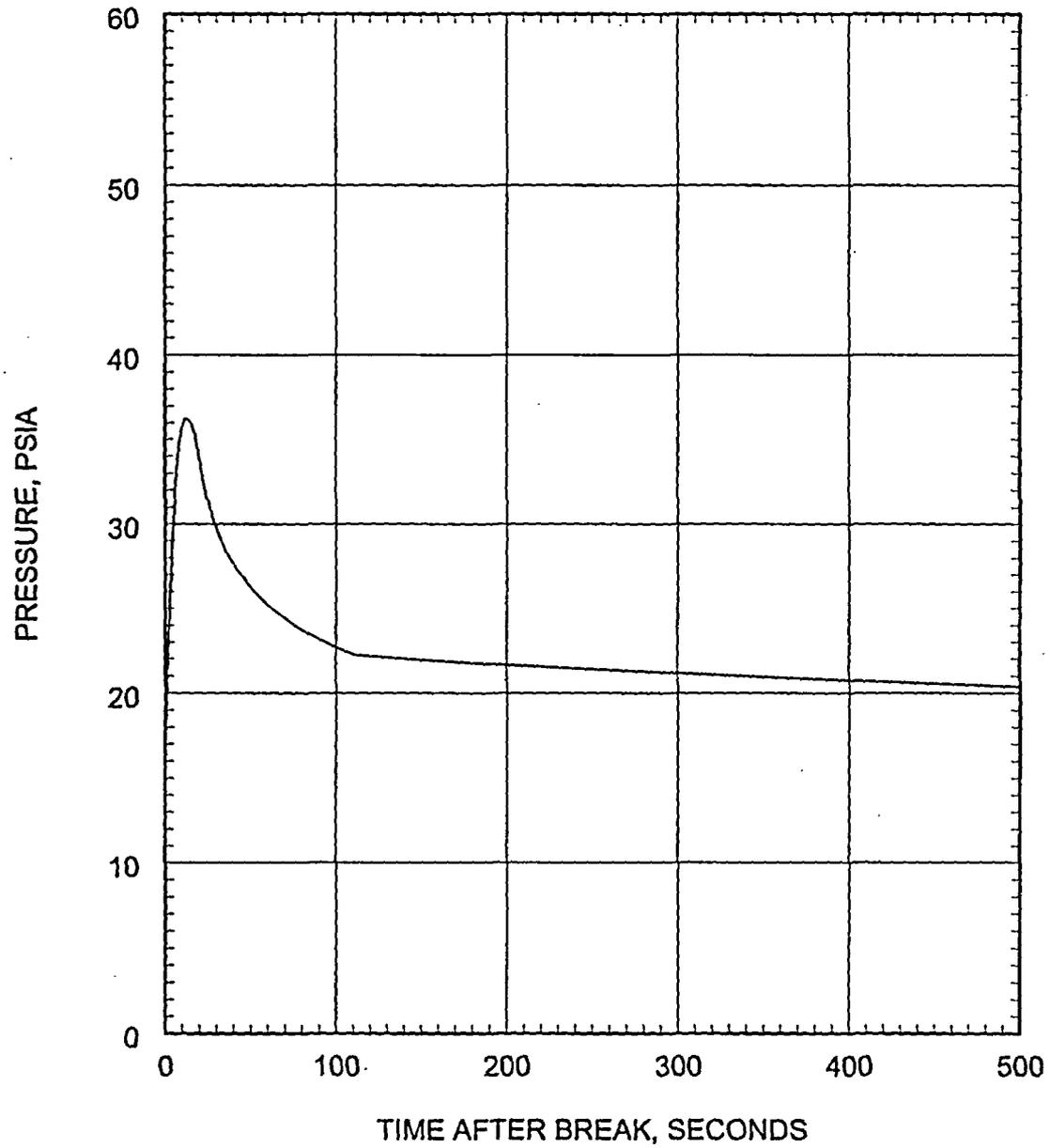
Figure 5.2.3.3-7 Large Break LOCA ECCS Performance Analysis 1.0 DEG/PD Break
