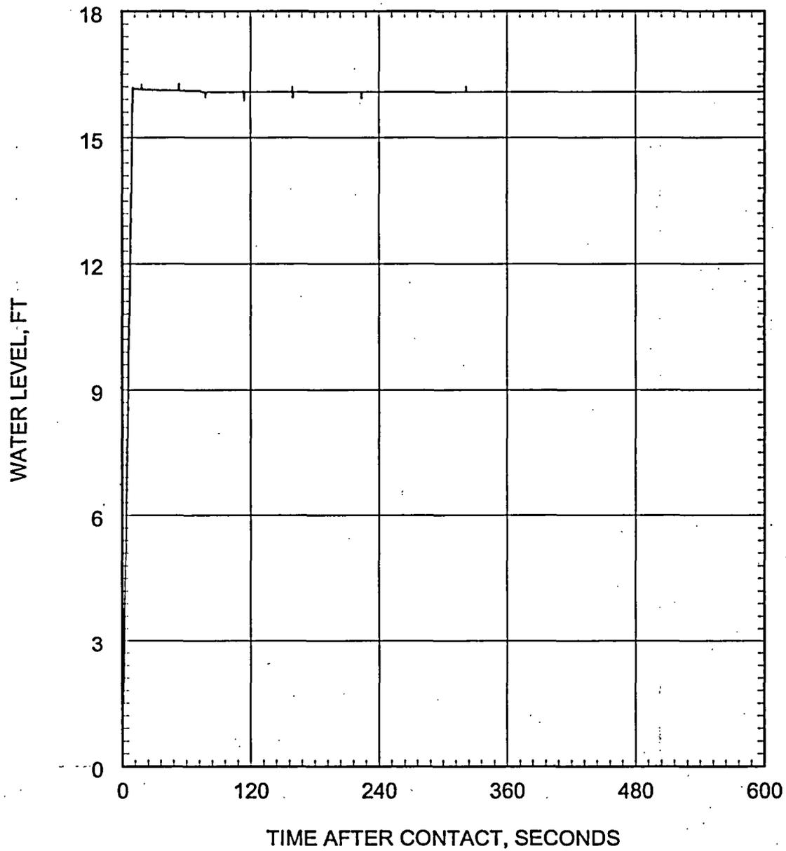
Figure 5.2.3.3-32 Large Break LOCA ECCS Performance Analysis 0.6 DEG/PD Break Water Level in Downcomer During Reflood
