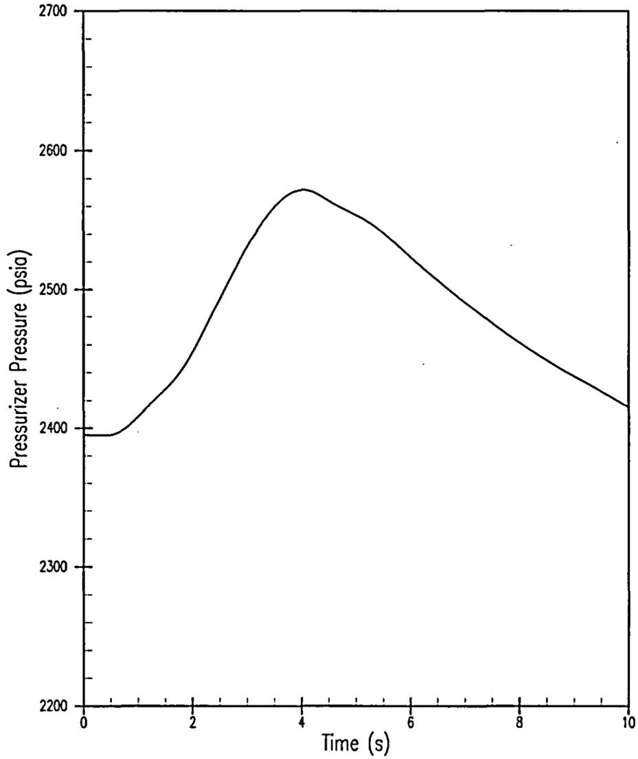
Figure 5.1.15-5 Pressurizer Pressure versus Time – Locked Rotor/Shaft Break
