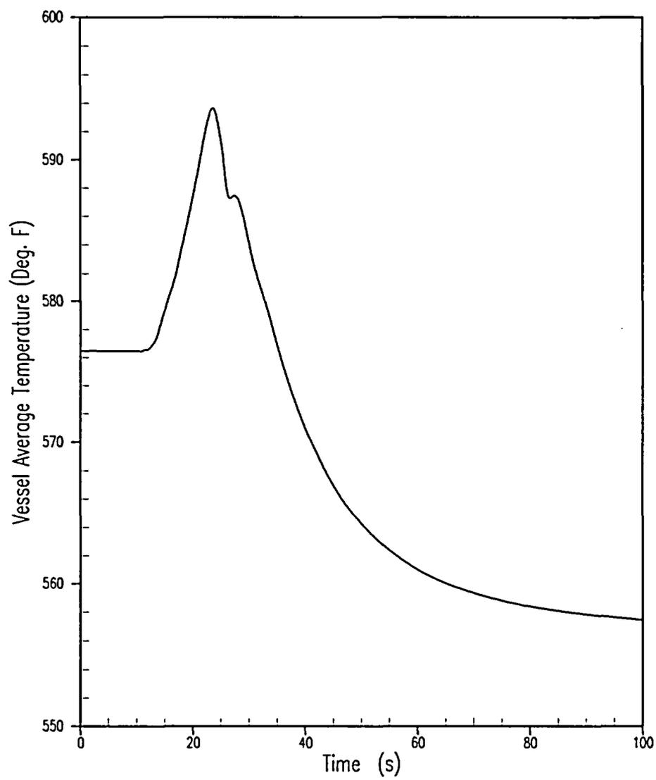
Figure 5.1.10-9 Loss of Condenser Vacuum (DNB Case) Vessel Average Temperature
