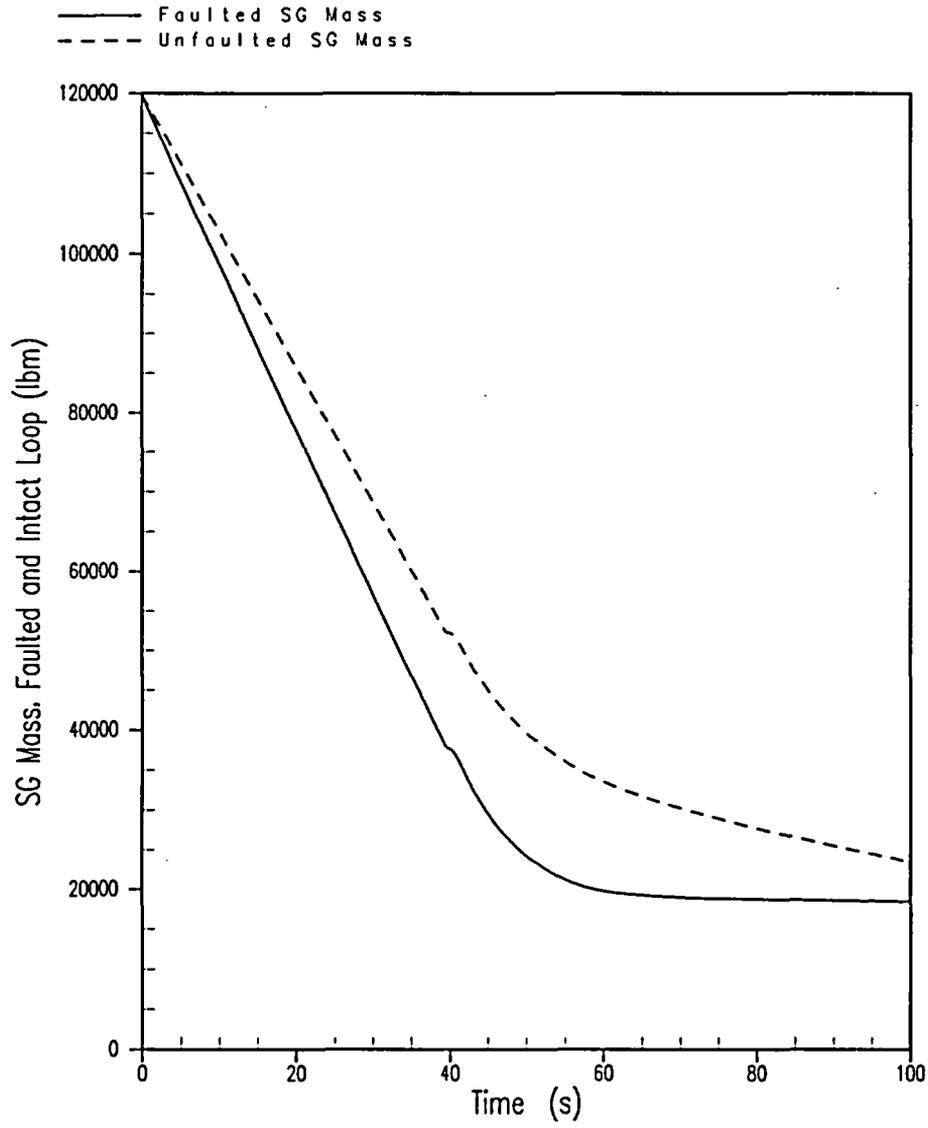
**Figure 5.1.12-11 Feedwater Line Break MSS Overpressure Case Limiting Break Size = 0.05 ft<sup>2</sup> SG Mass, Faulted and Intact Loop**
