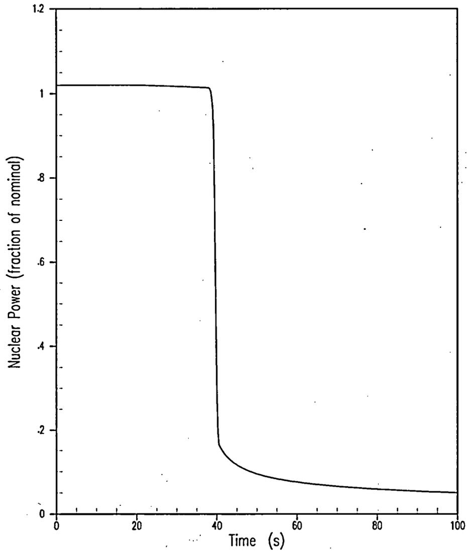
Figure 5.1.12-8 Feedwater Line Break MSS Overpressure Case Limiting Break Size = 0.05 ft<sup>2</sup>
