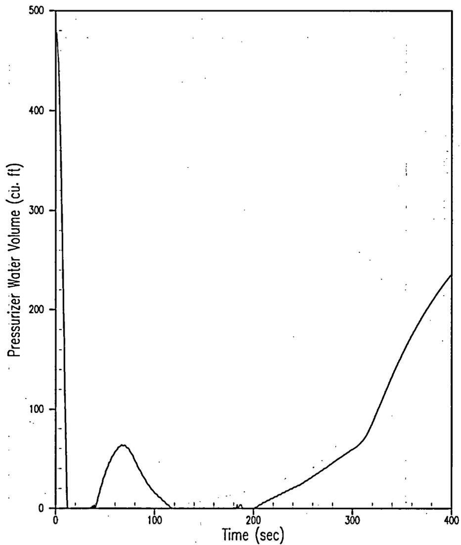
Figure 5.1.6-7 Post-Trip Main Steamline Break – Pressurizer Water Volume versus Time
