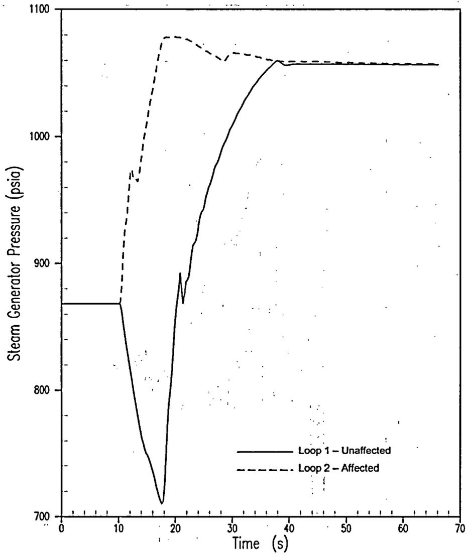
**Figure 5.1.11-6 Steam Generator Pressure for Asymmetric Steam Generator Transient 0% Tube Plugging**
