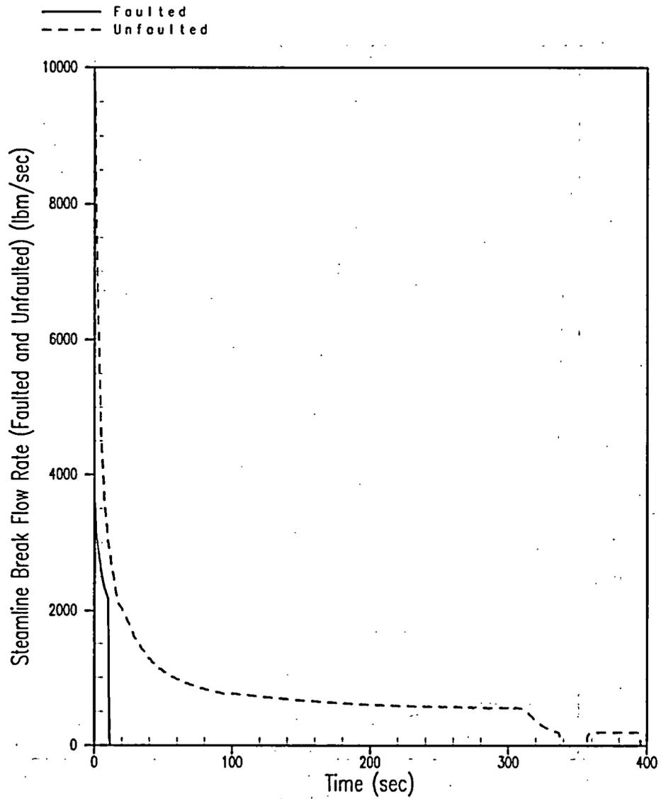
Figure 5.1.6-5 Post-Trip Main Steamline Break – Break Mass Flow Rate versus Time
