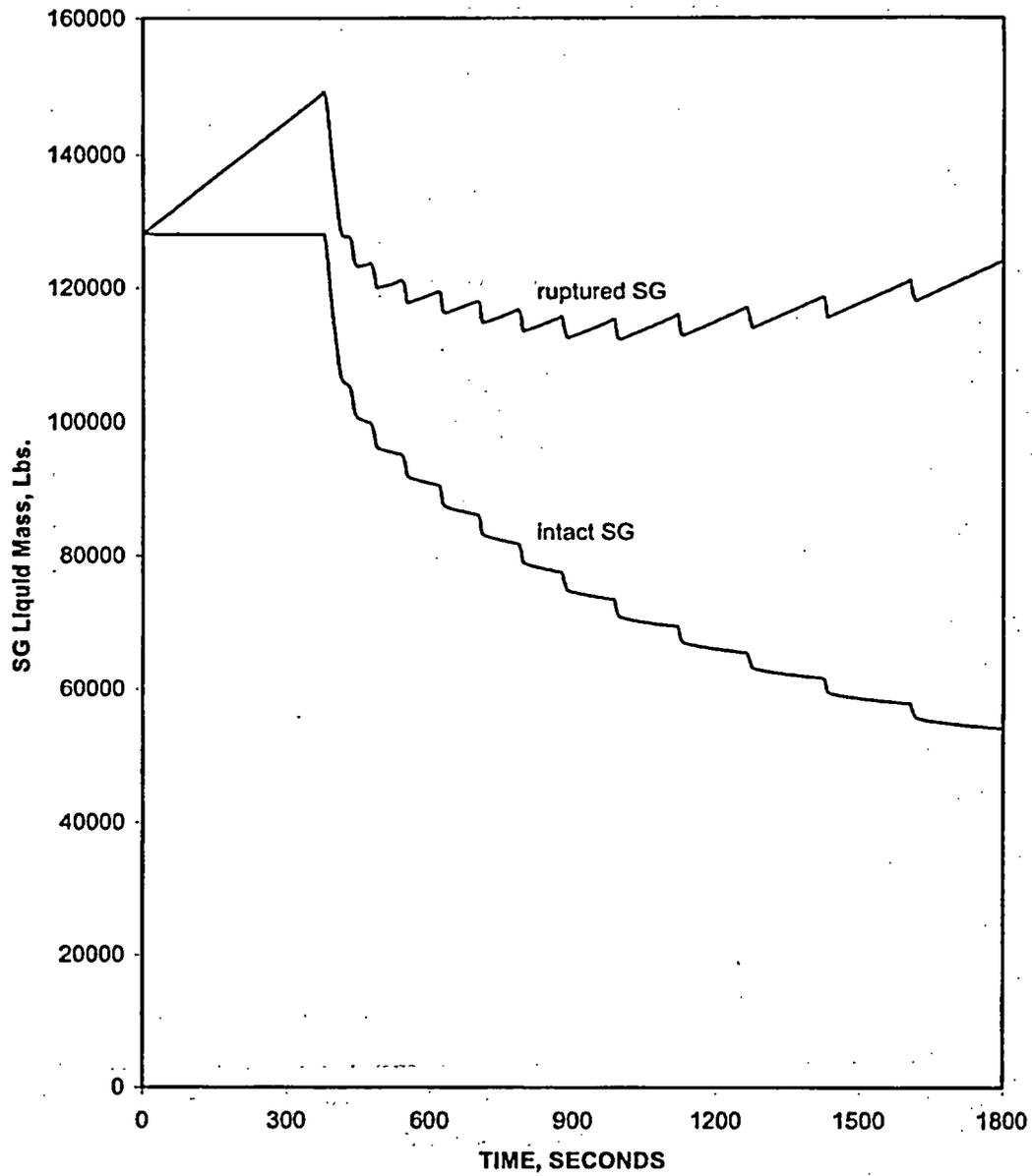
Figure 5.1.24-8 Steam Generator Tube Rupture with Loss of Offsite Power – Water Mass vs. Time
