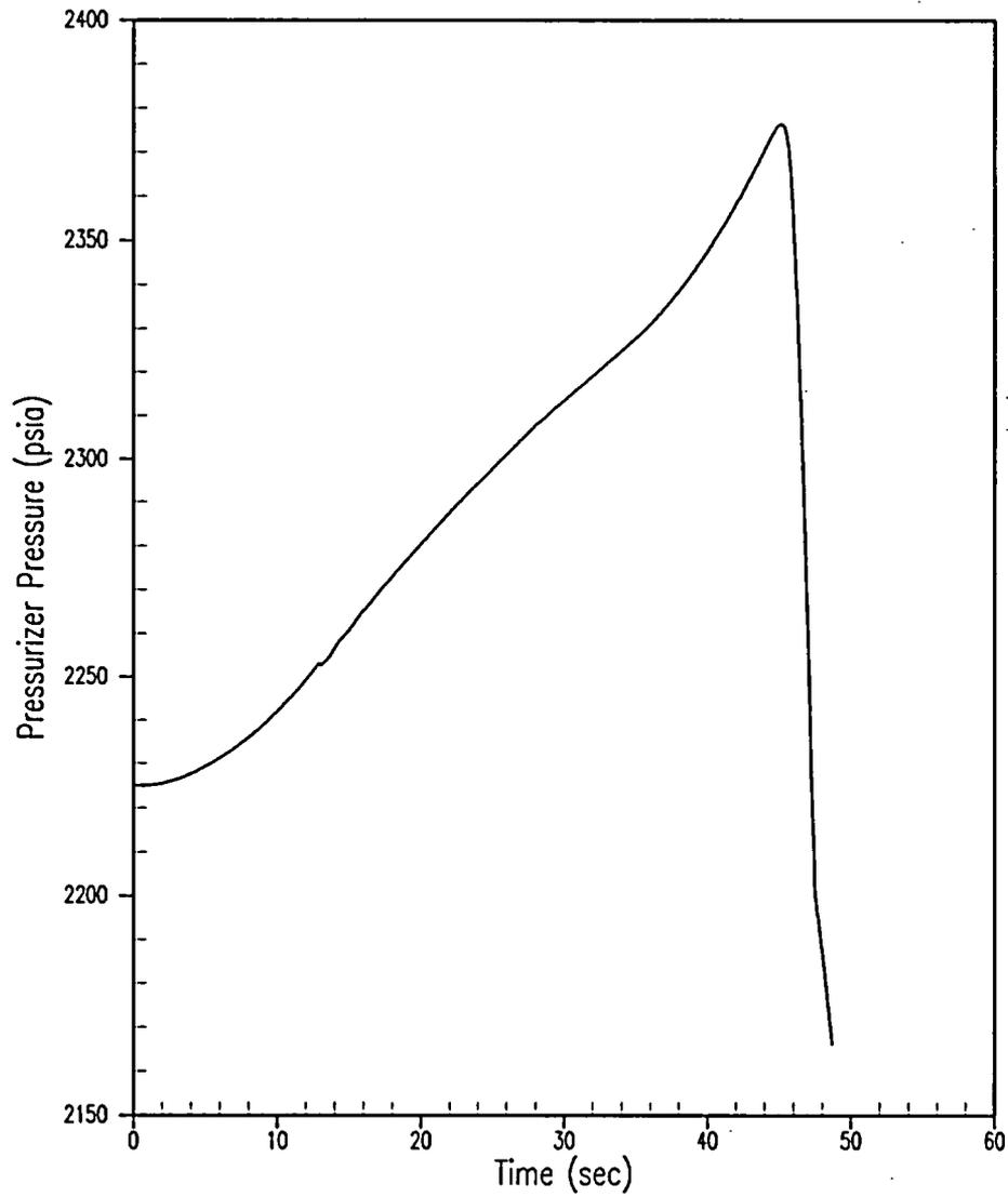
**Figure 5.1.16-2 Uncontrolled CEA Bank Withdrawal at Power 100% Power, 2 pcm/sec Reactivity Insertion Rate & Minimum Feedback Variable High Power Trip & Maximum Nominal RCS Vessel  $T_{avg}$  (Sheet 2 of 4)**
