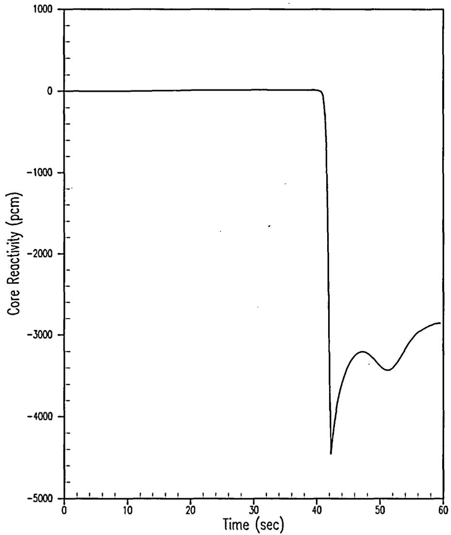
**Figure 5.1.1-3 Core Reactivity for a Feedwater Malfunction Increased Feedwater Flow at HFP Initial Conditions**
