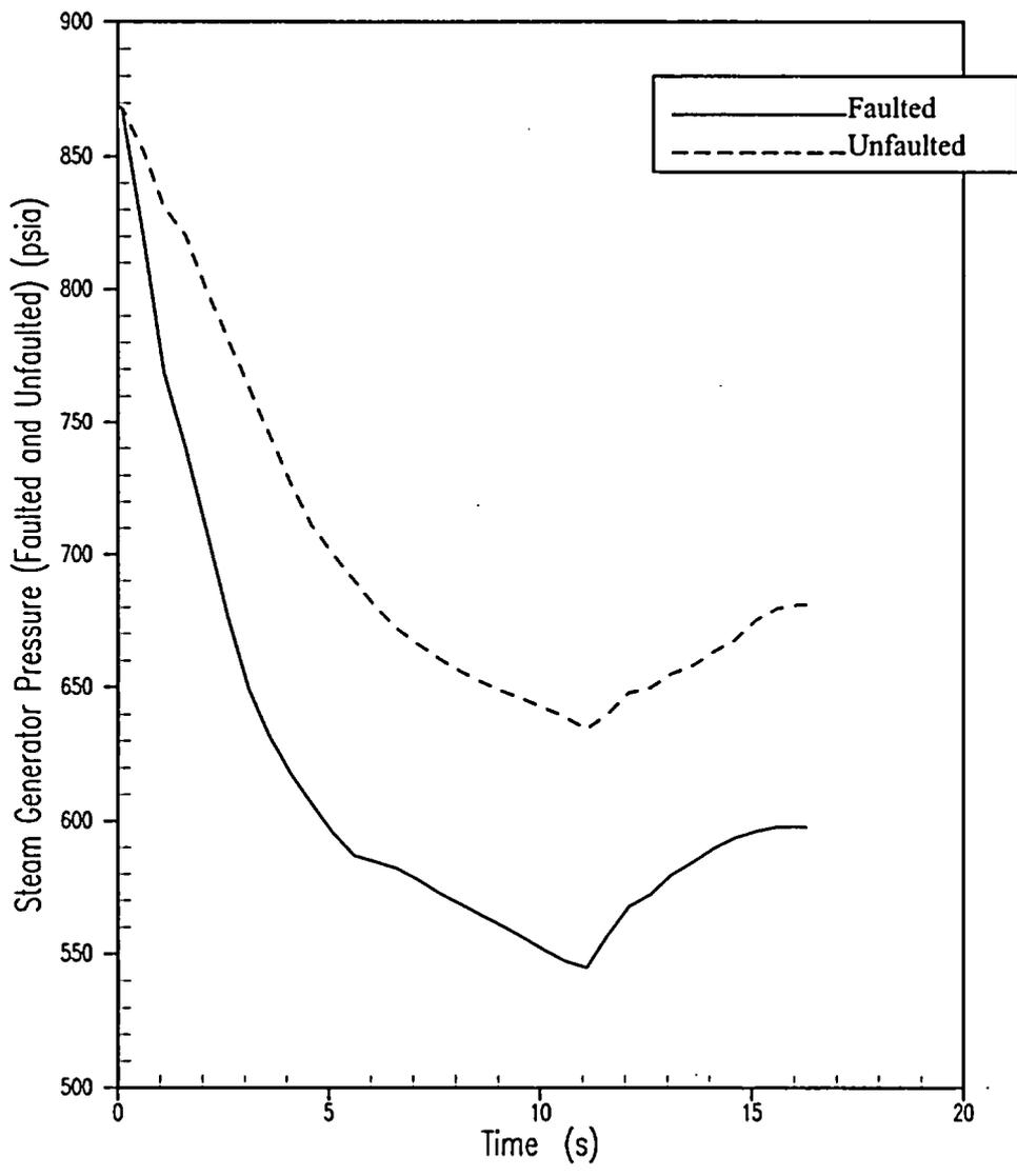
Figure 5.1.5-8 Pre-Trip Main Steamline Break – Steam Generator Steam Pressure versus Time
