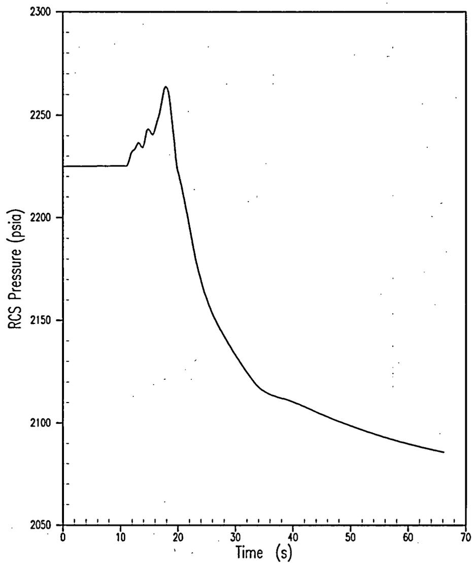
Figure 5.1.11-2 RCS Pressure for Asymmetric Steam Generator: Transient 0% Tube Plugging
