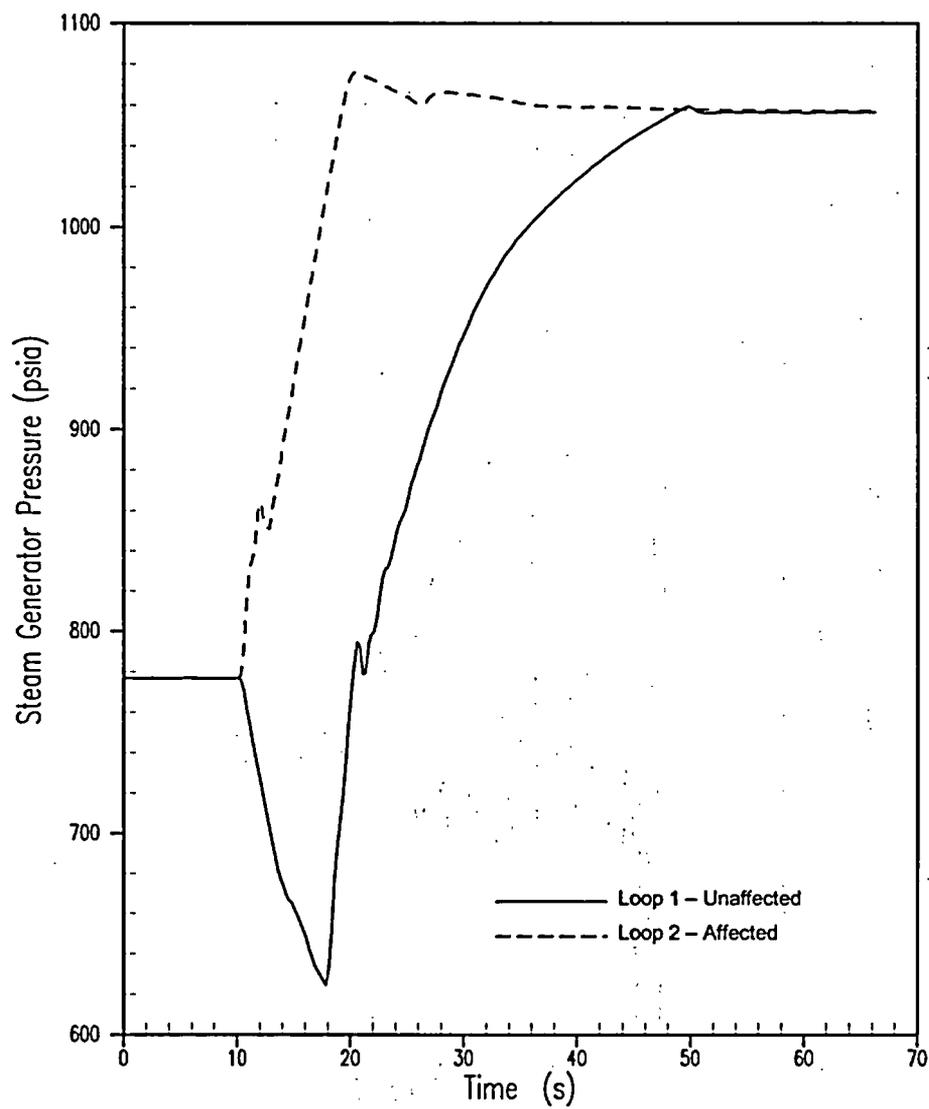
Figure 5.1.11-18 Steam Generator Pressure for Asymmetric Steam Generator Transient 30% Tube Plugging
