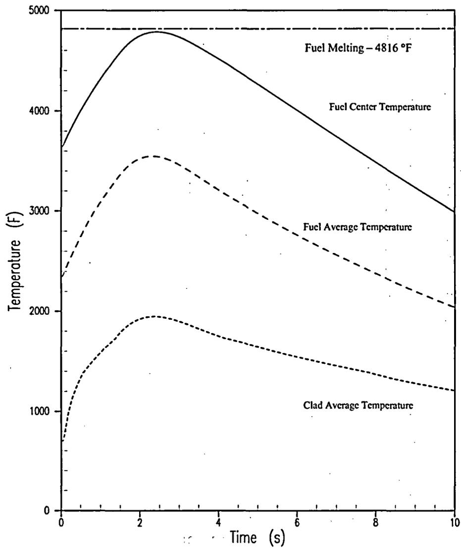
Figure 5.1.20-2 CEA Ejection Accident from Full Power Beginning of Cycle – Fuel and Cladding Temperatures versus Time
