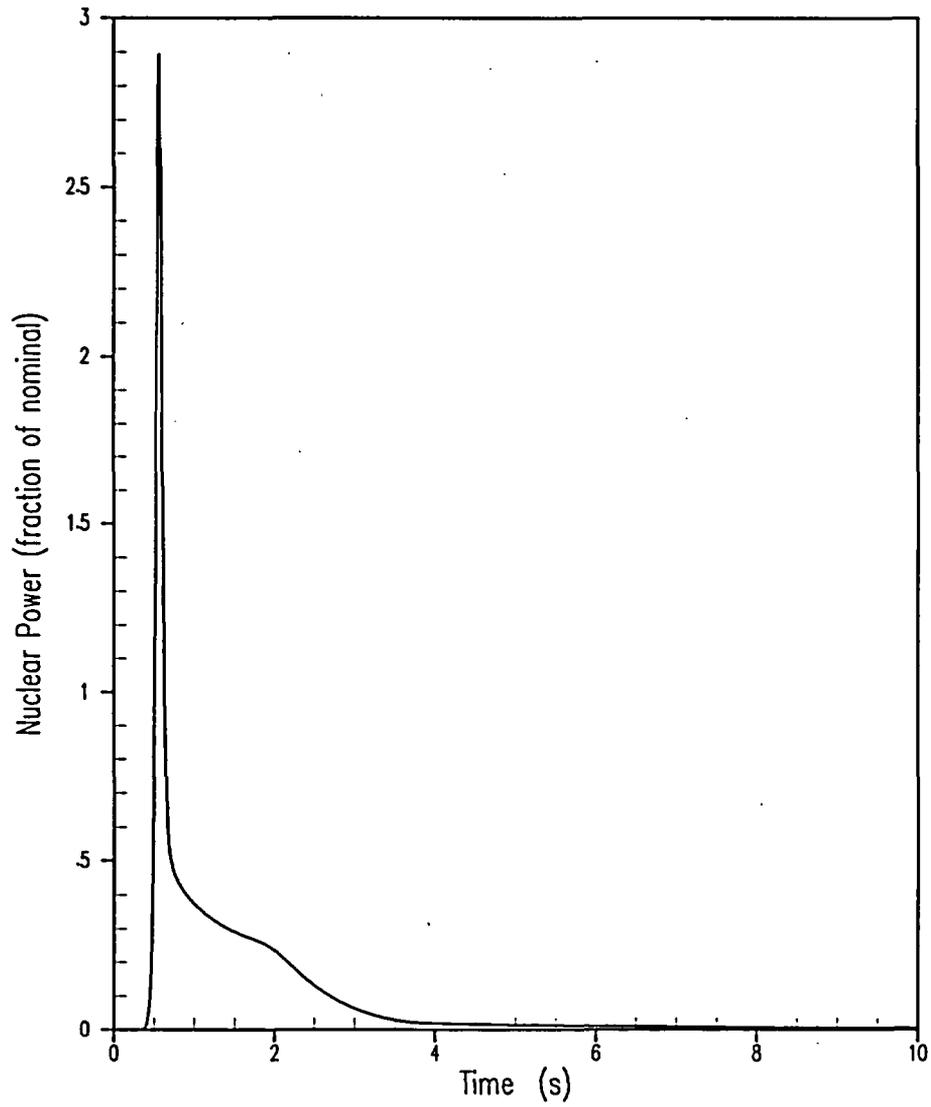
**Figure 5.1.20-3 CEA Ejection Accident from Zero Power Beginning of Cycle – Reactor Power versus Time**
