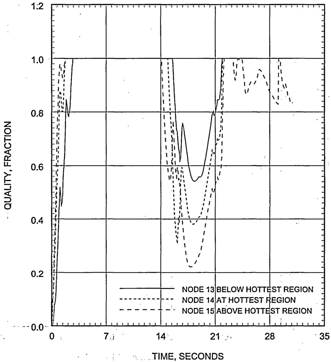
Figure 5.2.3.3-44 Large Break LOCA ECCS Performance Analysis 0.4 DEG/PD Break Hot Assembly Quality
