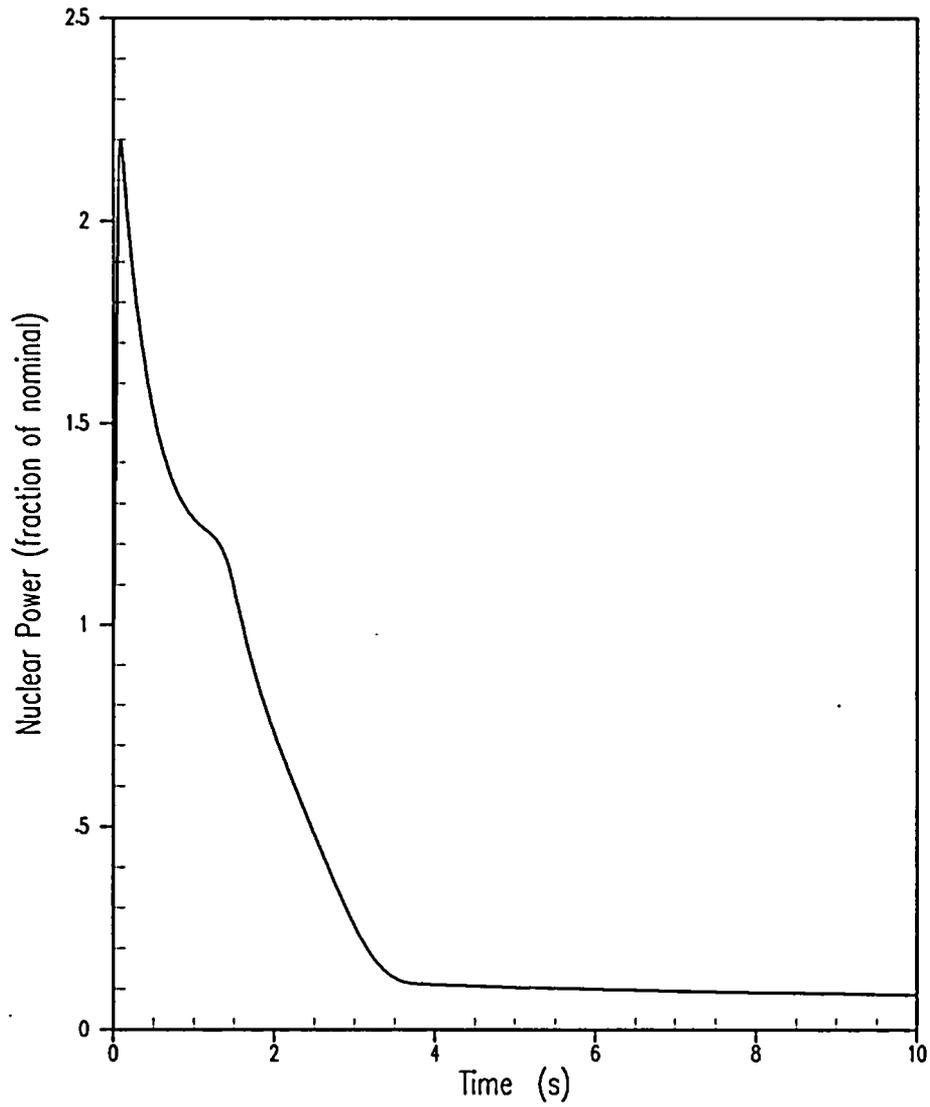
Figure 5.1.20-5 CEA Ejection Accident from Full Power End of Cycle – Reactor Power versus Time
