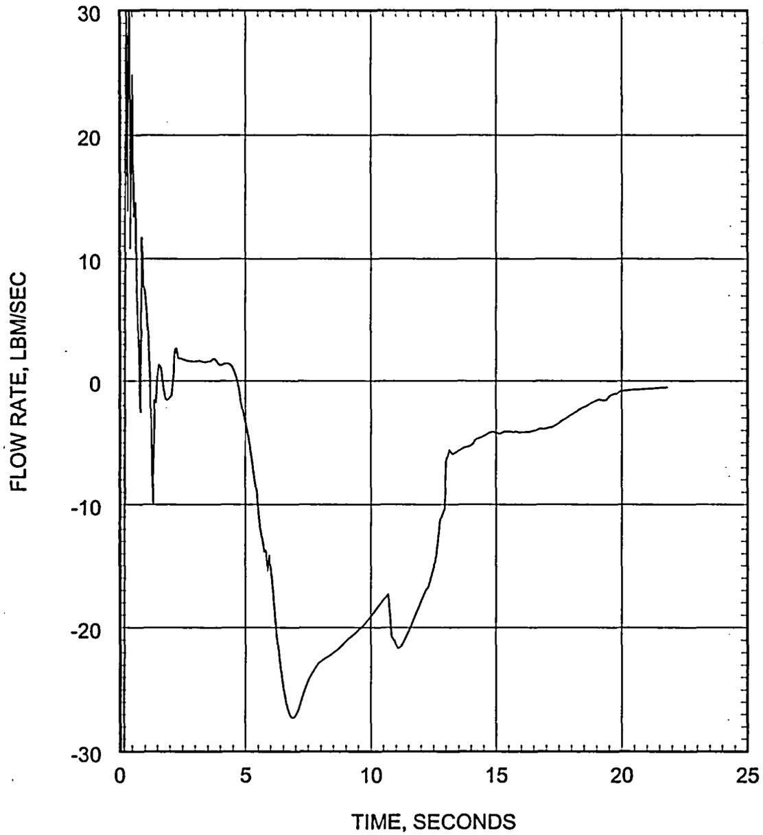
Figure 5.2.3.3-5 Large Break LOCA ECCS Performance Analysis 1.0 DEG/PD Break Hot Assembly Flow Rate (Above Hot Spot)
