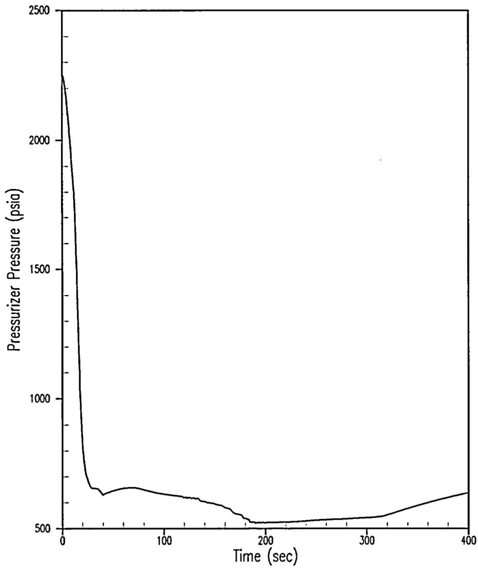
Figure 5.1.6-6 Post-Trip Main Steamline Break – Pressurizer Pressure versus Time
