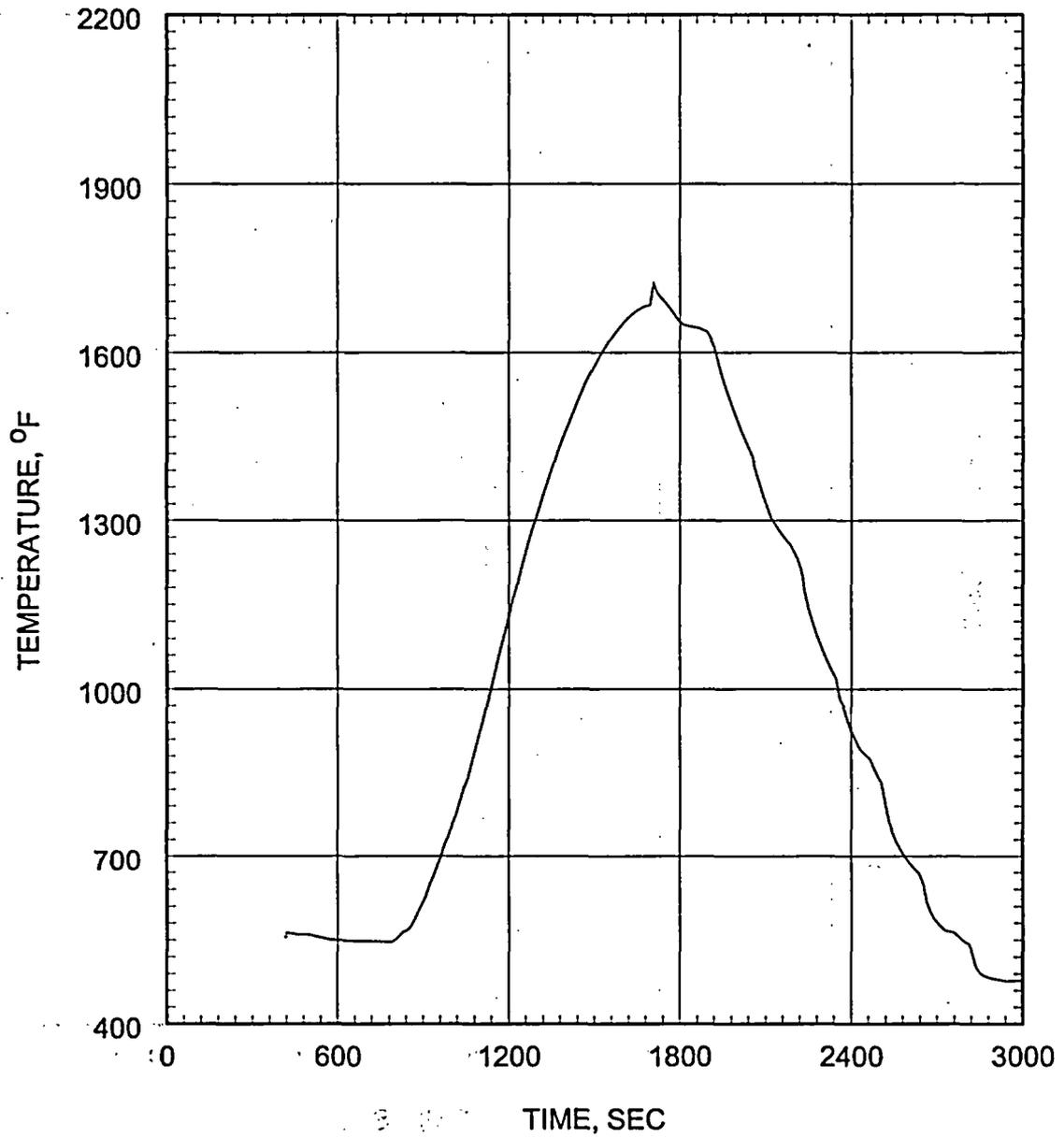
Figure 5.2.4.3-15 Small Break LOCA ECCS Performance Analysis 0.05 ft<sup>2</sup>/PD Break Coolant Temperature at Hot Spot
