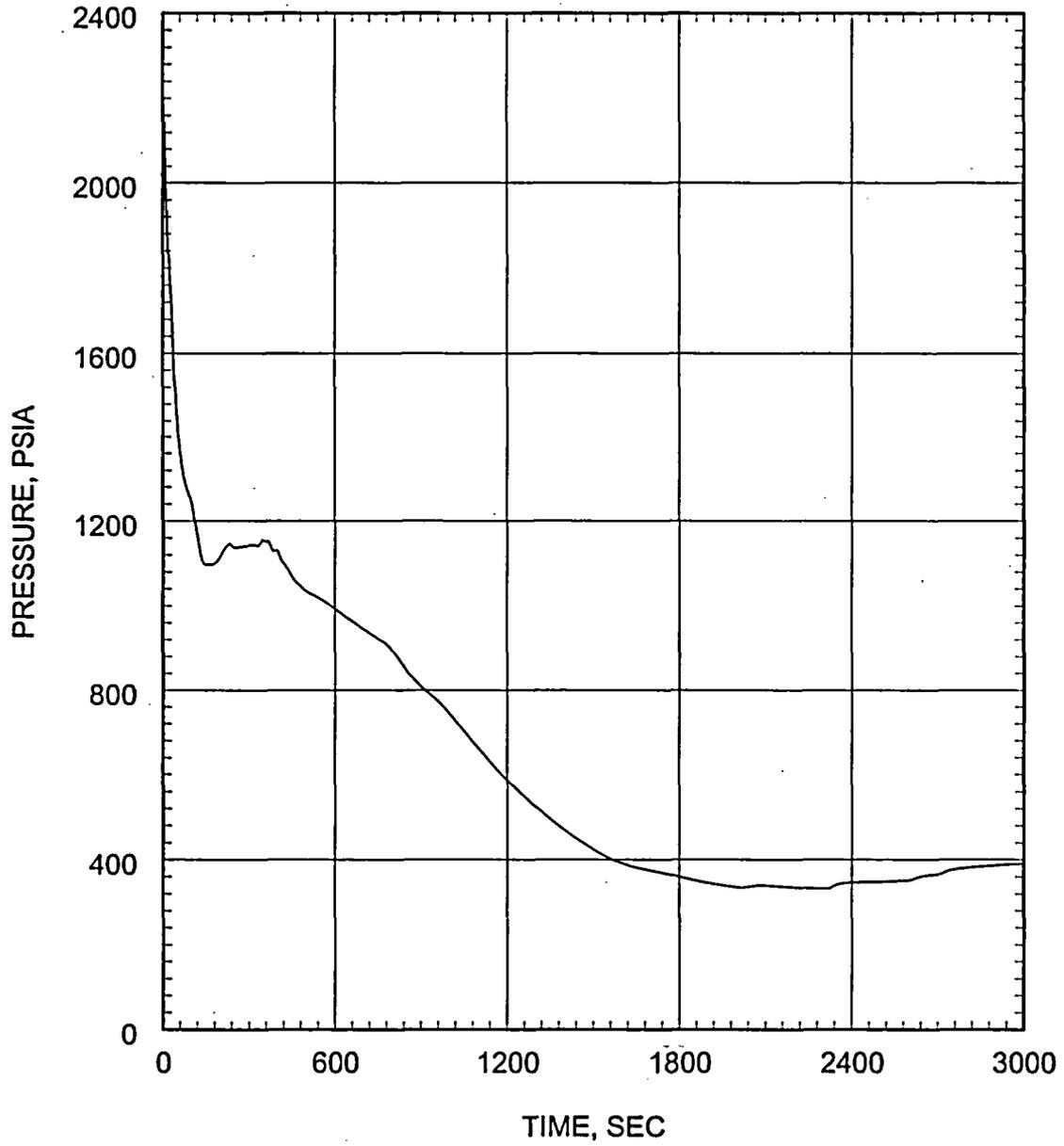
Figure 5.2.4.3-18 Small Break LOCA ECCS Performance Analysis 0.06 ft<sup>2</sup>/PD Break Inner Vessel Pressure
