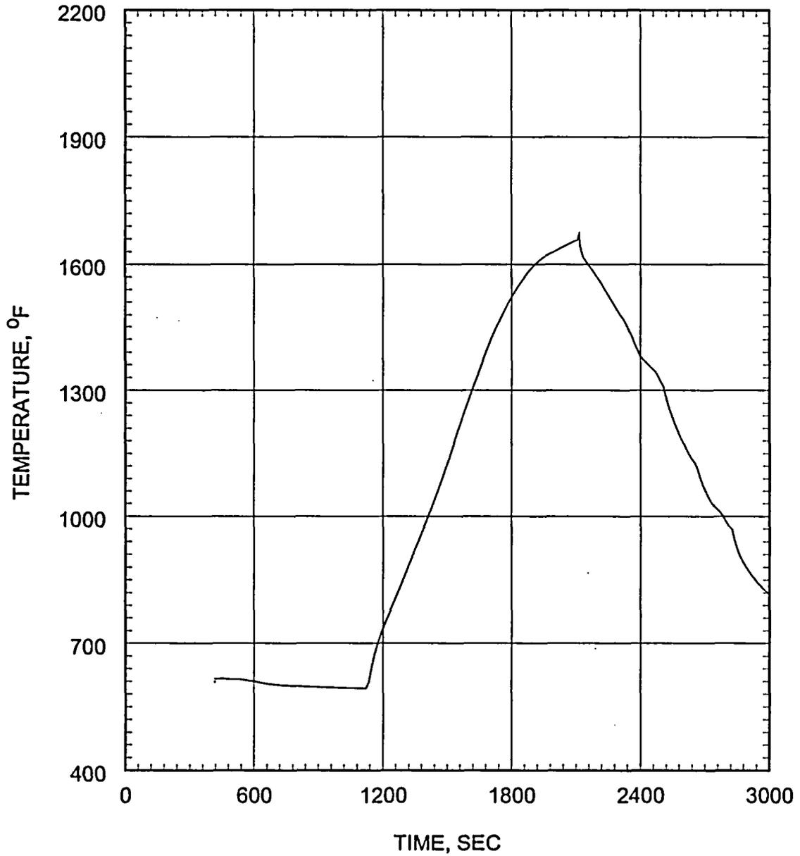
Figure 5.2.4.3-8 Small Break LOCA ECCS Performance Analysis 0.04 ft<sup>2</sup>/PD Break Cladding Temperature at Hot Spot
