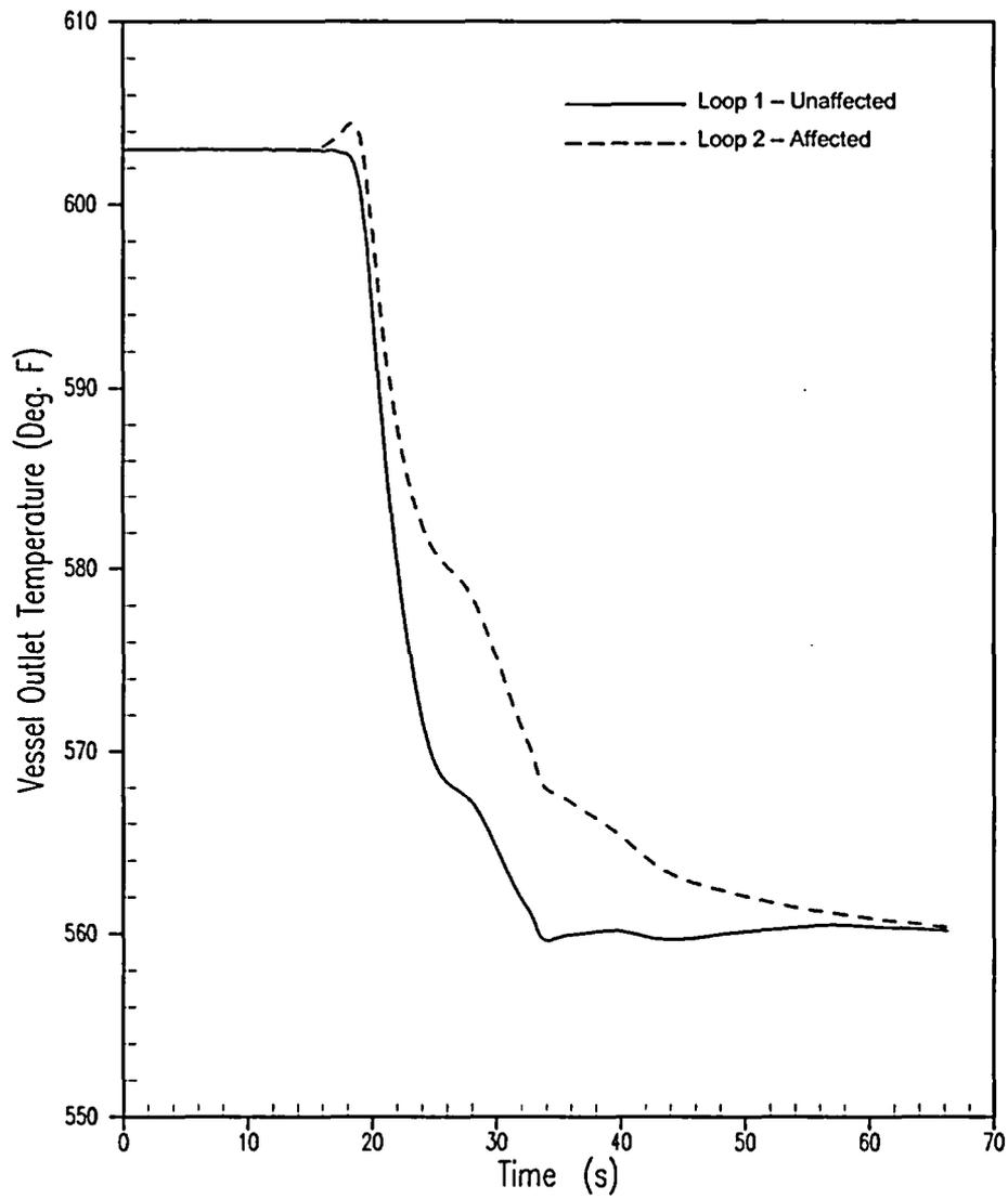
Figure 5.1.11-17 Vessel Outlet Temperature for Asymmetric Steam Generator Transient 30% Tube Plugging
