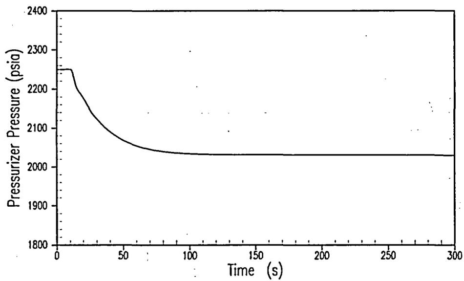
**Figure 5.1.18-7 Representative Transient Response to Dropped CEA Worth of 500 pcm at a Moderator Temperature Coefficient of  $-25$  pcm/ $^{\circ}$ F – Pressurizer Pressure versus Time**
