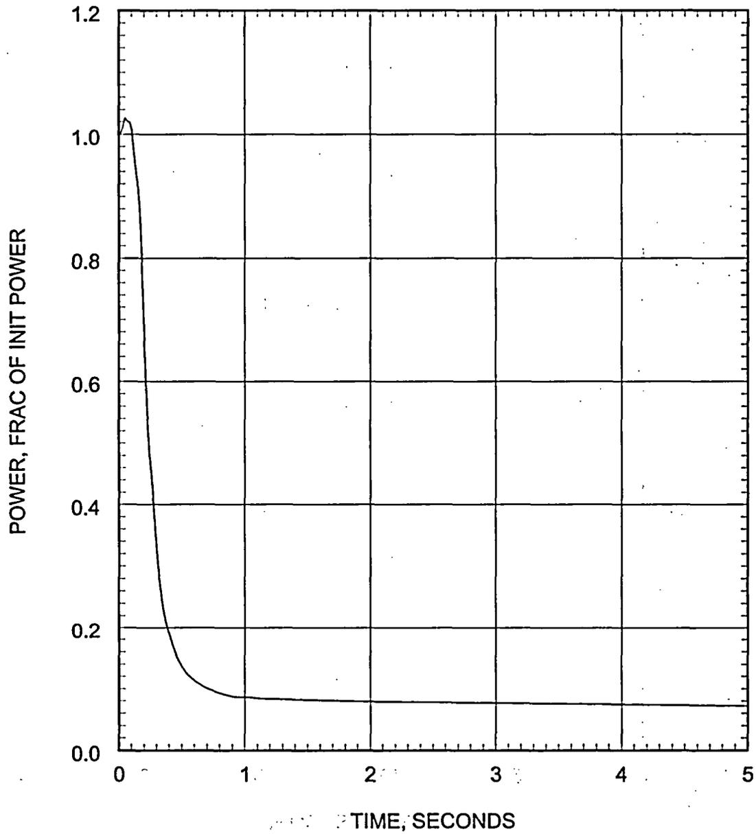
Figure 5.2.3.3-10 Large Break LOCA ECCS Performance Analysis 0.8 DEG/PD Break Core Power
