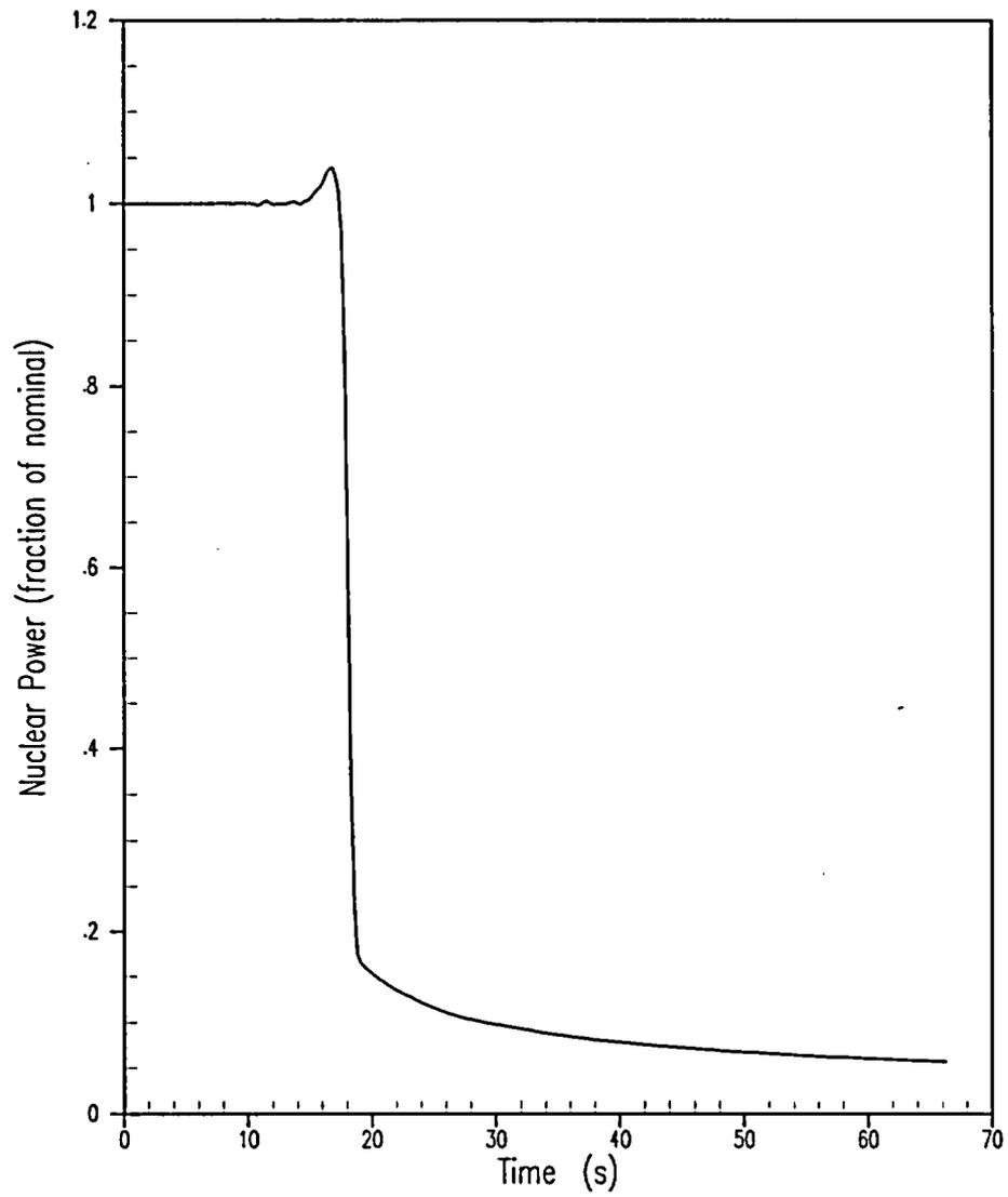
Figure 5.1.11-13 Nuclear Power for Asymmetric Steam Generator Transient 30% Tube Plugging
