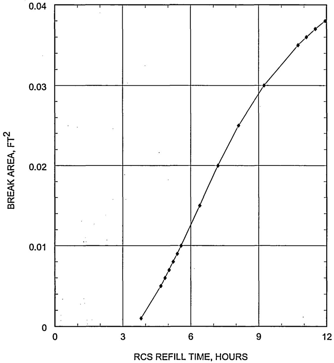
Figure 5.2.5.3-4 Long-Term Cooling Analysis Break Area Versus RCS Refill Time
