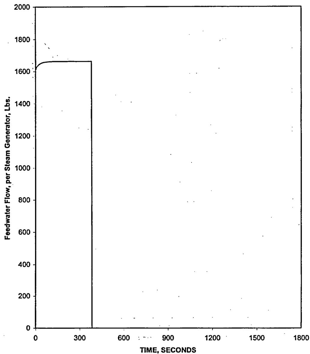
Figure 5.1.24-10 : Steam Generator Tube Rupture with Loss of Offsite Power – Feedwater Flow vs. Time
