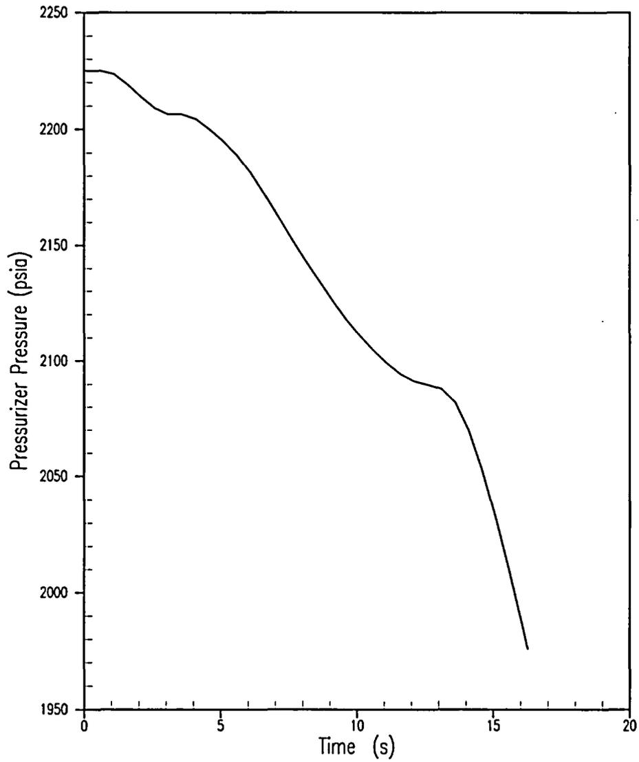
Figure 5.1.5-4 Pre-Trip Main Steamline Break – Pressurizer Pressure versus Time
