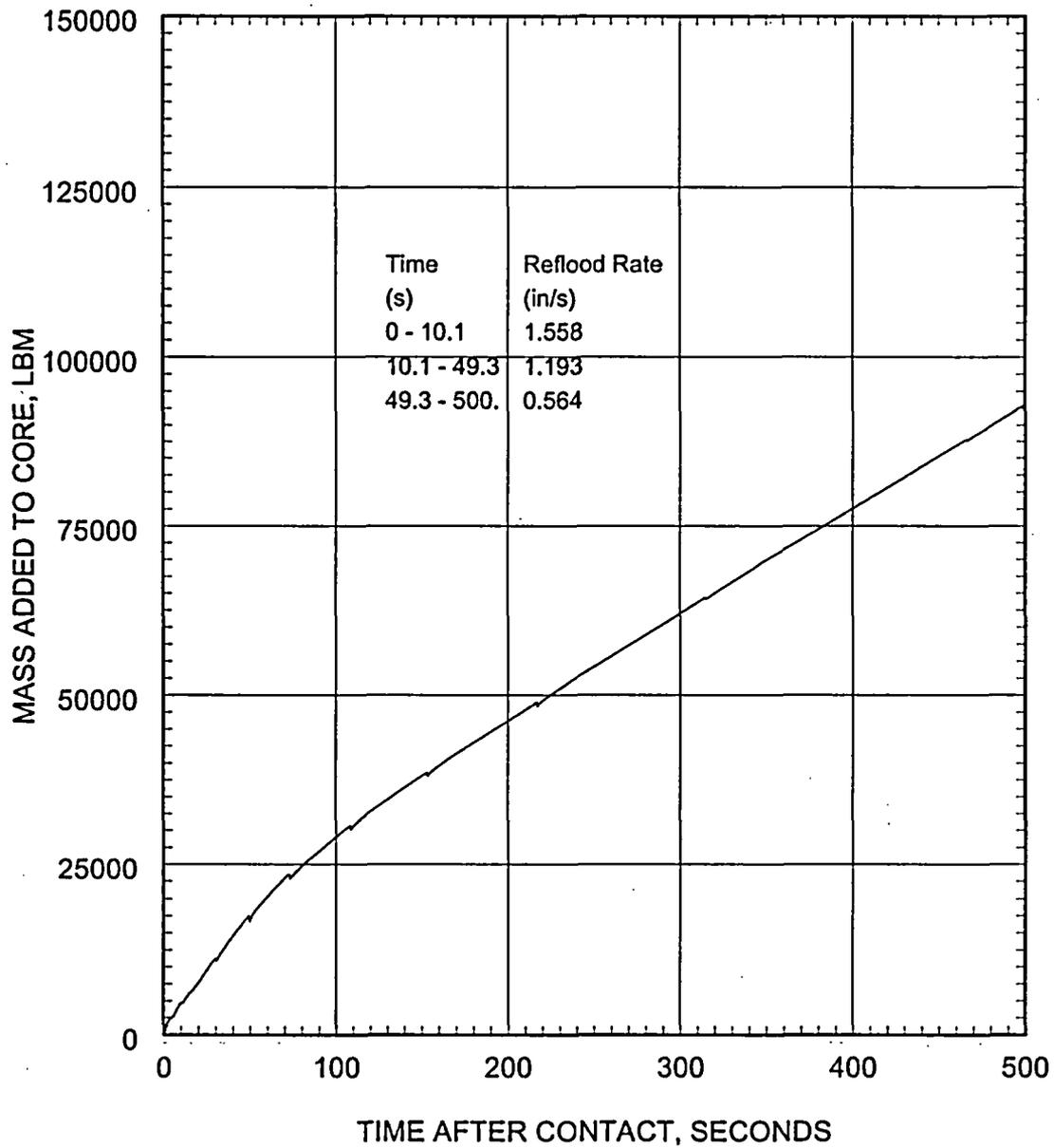
Figure 5.2.3.3-17 Large Break LOCA ECCS Performance Analysis 0.8 DEG/PD Break Mass Added to Core During Reflood
