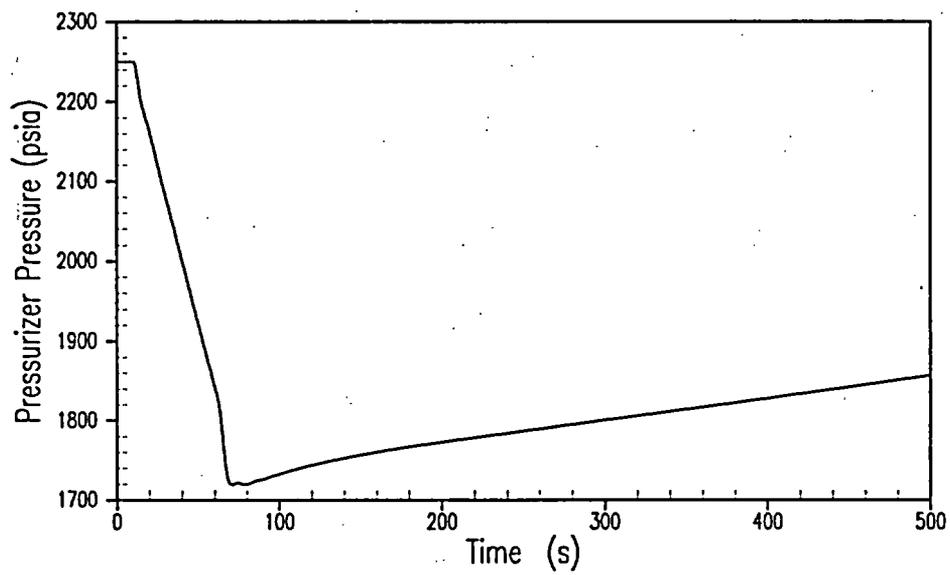
**Figure 5.1.18-3 Representative Transient Response to Dropped CEA Worth of 500 pcm at a Moderator Temperature Coefficient of 0 pcm/°F – Pressurizer Pressure versus Time**
