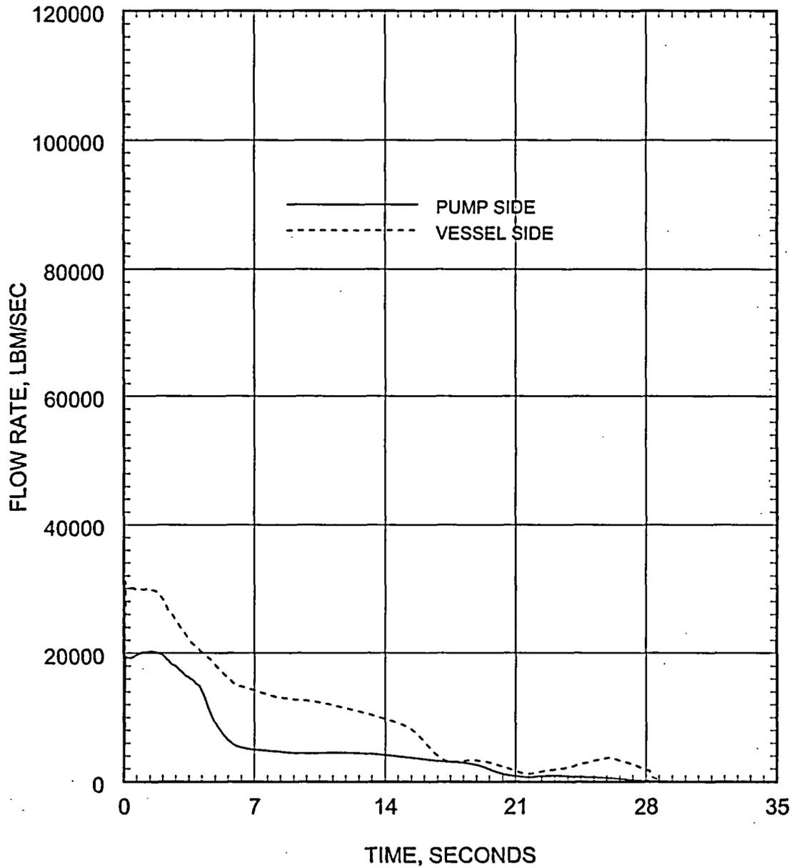
Figure 5.2.3.3-41 Large Break LOCA ECCS Performance Analysis 0.4 DEG/PD Break Leak Flow Rate
