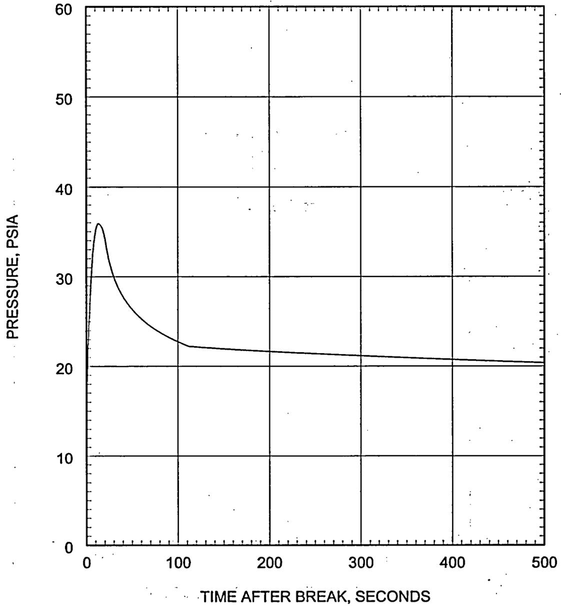
Figure 5.2.3.3-16 Large Break LOCA ECCS Performance Analysis 0.8 DEG/PD Break
