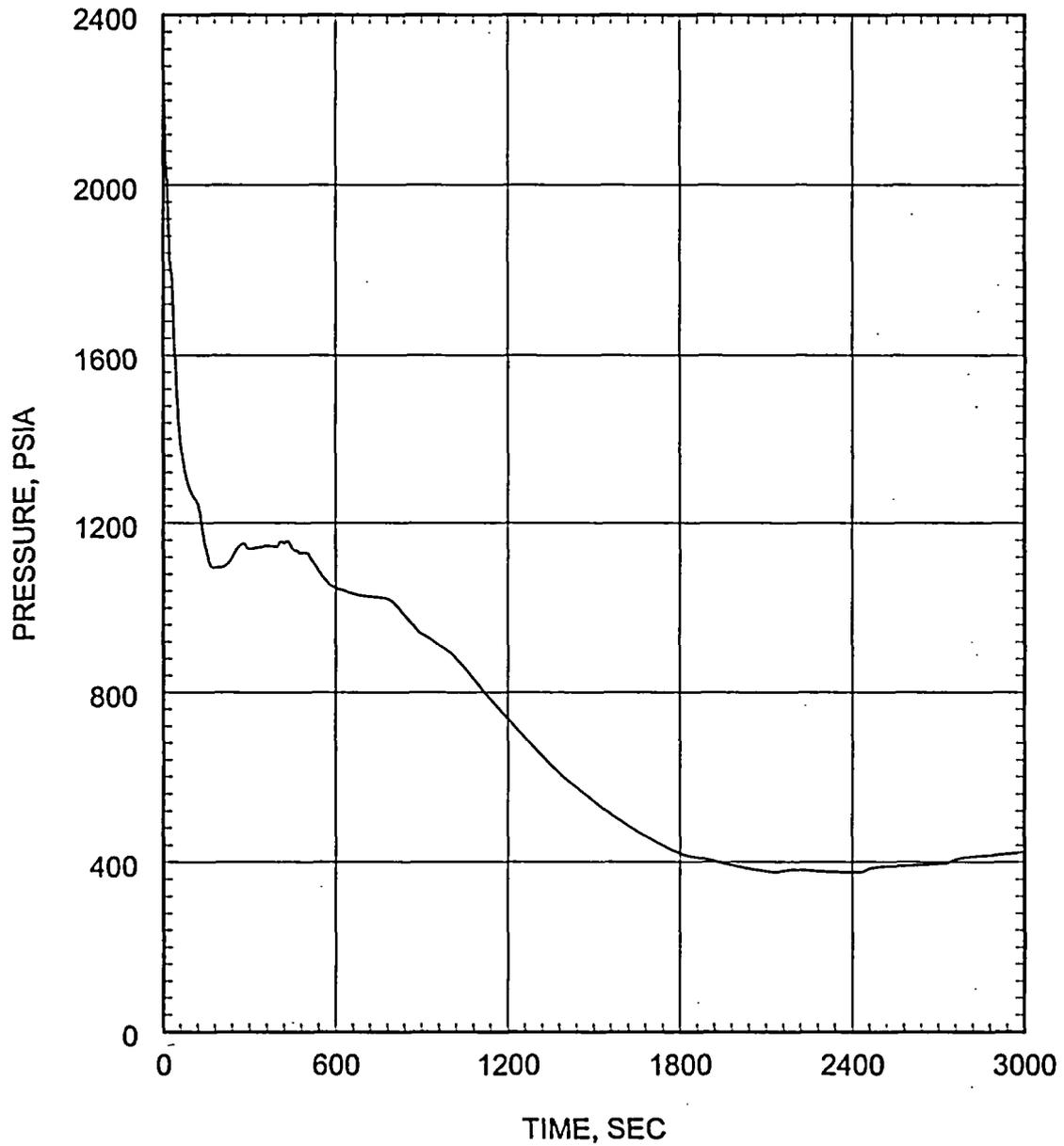
Figure 5.2.4.3-10 Small Break LOCA ECCS Performance Analysis 0.05 ft<sup>2</sup>/PD Break Inner Vessel
