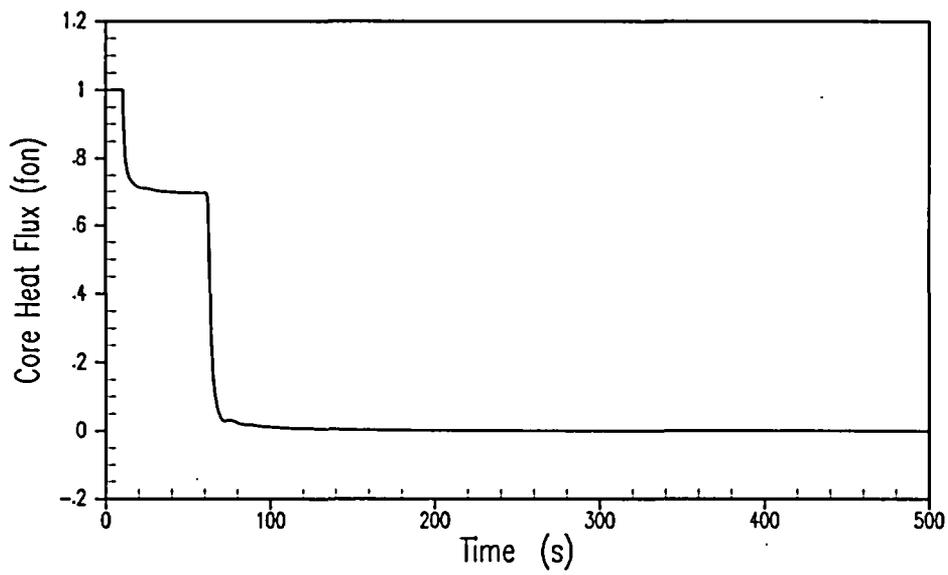
**Figure 5.1.18-2 Representative Transient Response to Dropped CEA Worth of 500 pcm at a Moderator Temperature Coefficient of 0 pcm/°F – Core Heat Flux versus Time**
