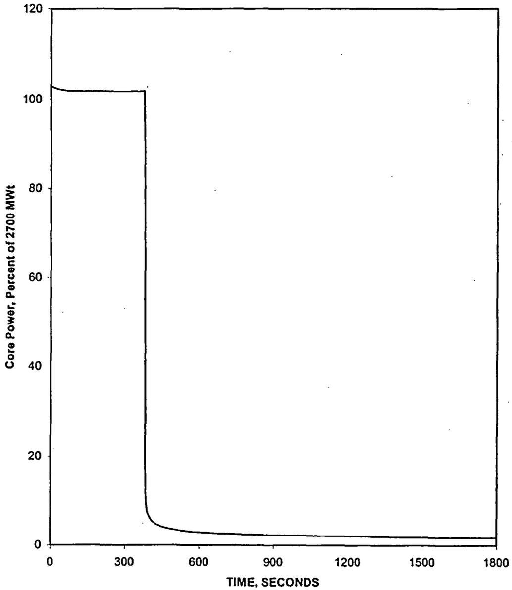
Figure 5.1.24-1 Steam Generator Tube Rupture with Loss of Offsite Power – Core Power vs. Time
