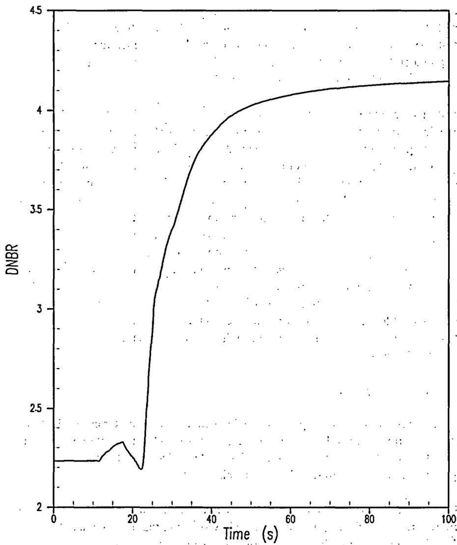
Figure 5.1.10-10 Loss of Condenser Vacuum (DNB Case) DNBR
