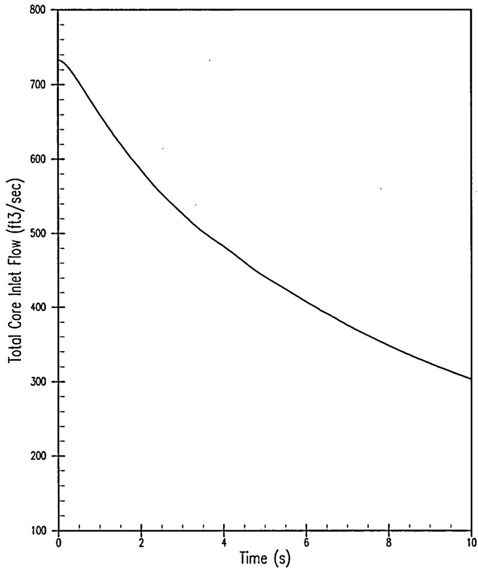
**Figure 5.1.14-1 Total Core Inlet Flow versus Time – Complete Loss of Flow – Four Pumps Coasting Down (CLOF)**
