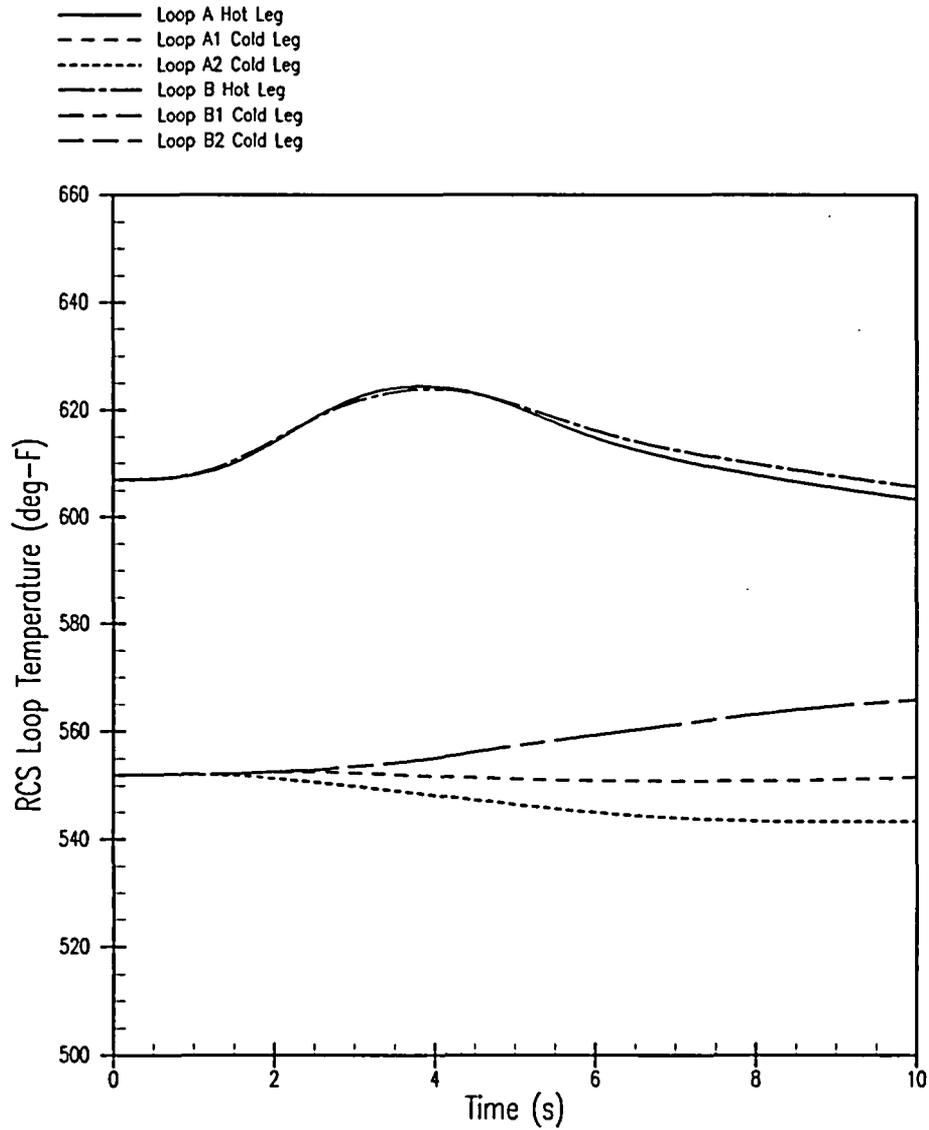
Figure 5.1.15-7 RCS Loop Temperature versus Time – Locked Rotor/Shaft Break
