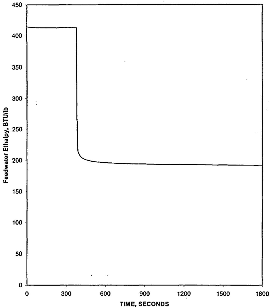
**Figure 5.1.24-13 Steam Generator Tube Rupture with Loss of Offsite Power – Feedwater Enthalpy vs. Time**
