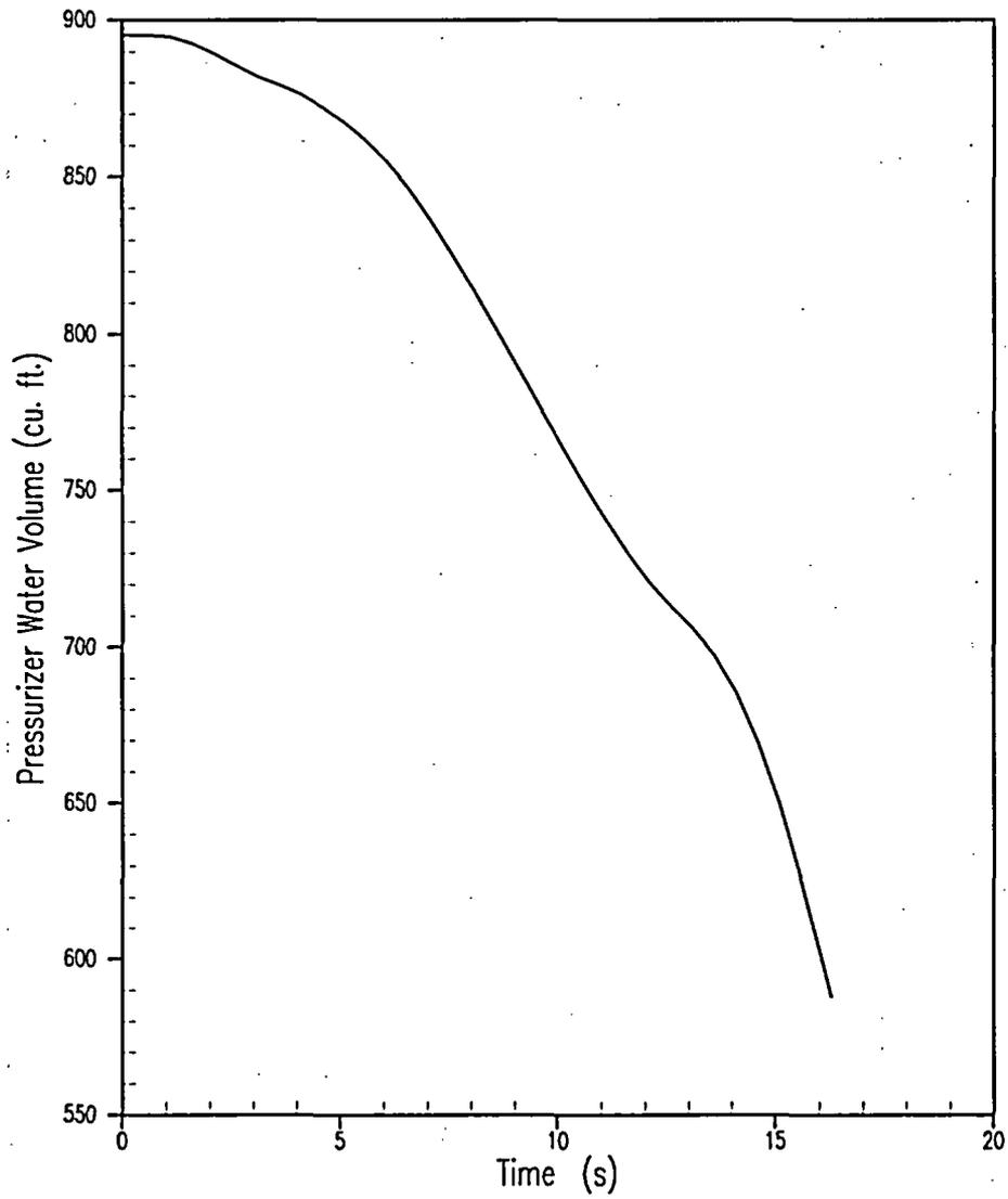
Figure 5.1.5-5 Pre-Trip Main Steamline Break – Pressurizer Water Volume versus Time
