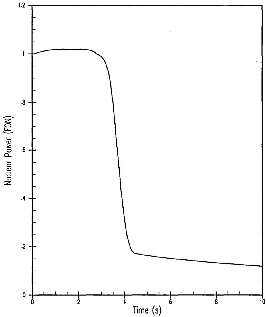
**Figure 5.1.14-3 Nuclear Power versus Time – Complete Loss of Flow – Four Pumps Coasting Down (CLOF)**
