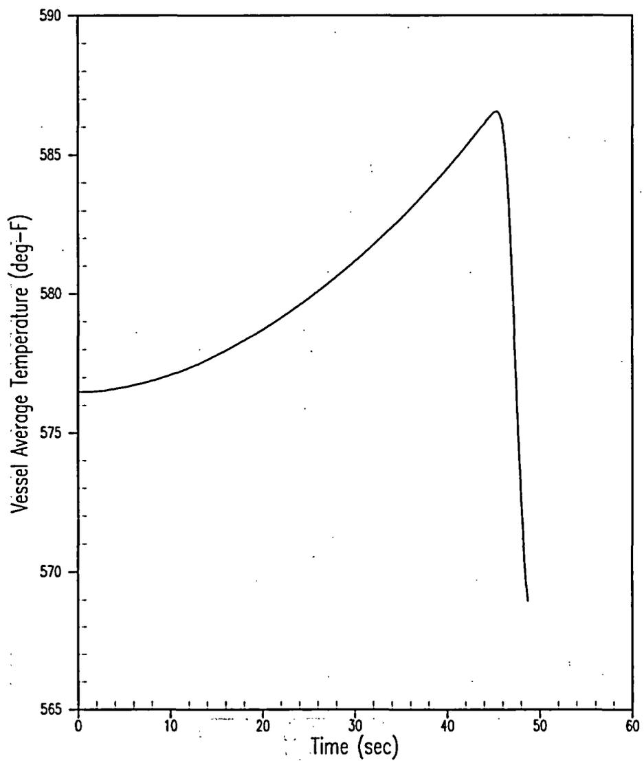
**Figure 5.1.16-2 Uncontrolled CEA Bank Withdrawal at Power 100% Power, 2pcm/sec Reactivity Insertion Rate & Minimum Feedback Variable High Power Trip & Maximum Nominal RCS Vessel  $T_{avg}$  (Sheet 3 of 4)**
