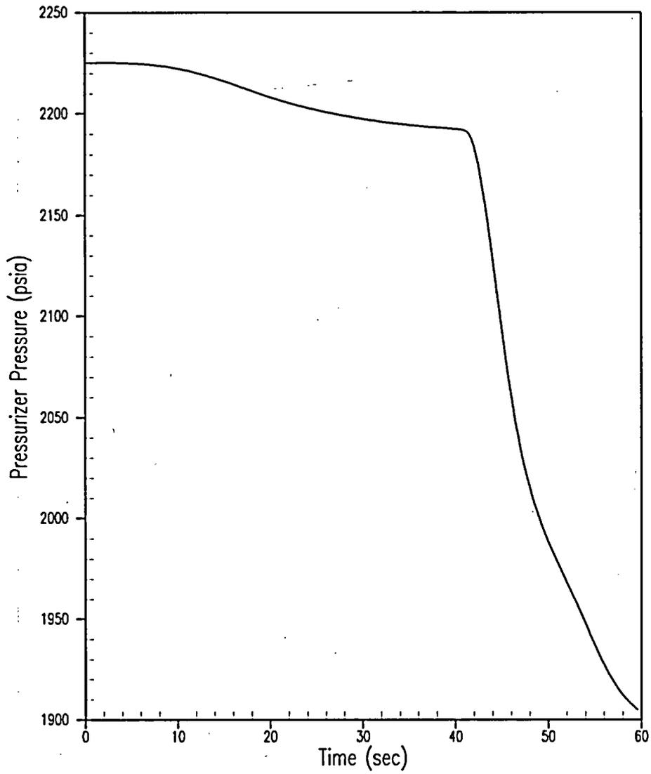
**Figure 5.1.1-4 Pressurizer Pressure for a Feedwater Malfunction Increased Feedwater Flow at HFP Initial Conditions**
