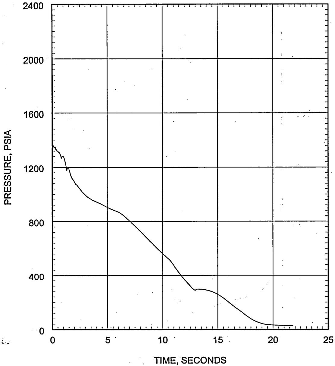
Figure 5.2.3.3-2 Large Break LOCA ECCS Performance Analysis 1.0 DEG/PD Break Pressure in Center Hot Assembly Node
