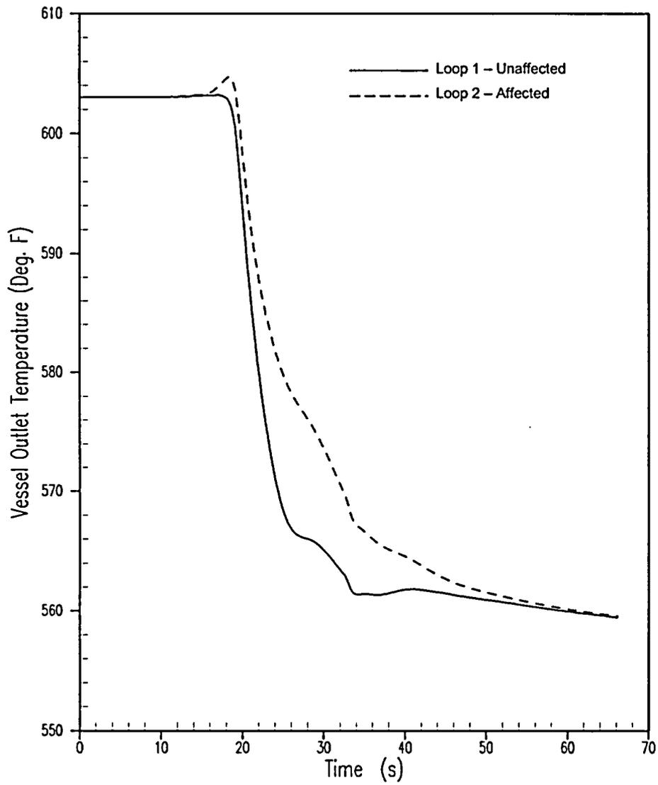
**Figure 5.1.11-5 Vessel Outlet Temperature for Asymmetric Steam Generator Transient 0% Tube Plugging**
