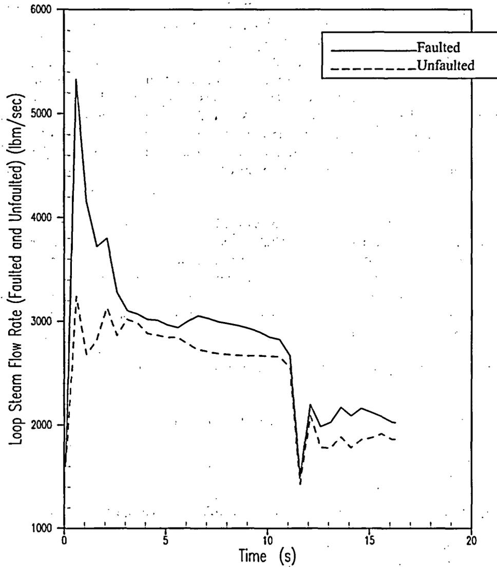
Figure 5.1.5-9 Pre-Trip Main Steamline Break – Loop Steam Flow Rate versus Time
