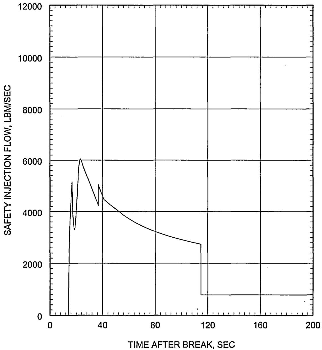
Figure 5.2.3.3-31 Large Break LOCA ECCS Performance Analysis 0.6 DEG/PD Break Safety Injection Flow Rate into Intact Discharge Legs
