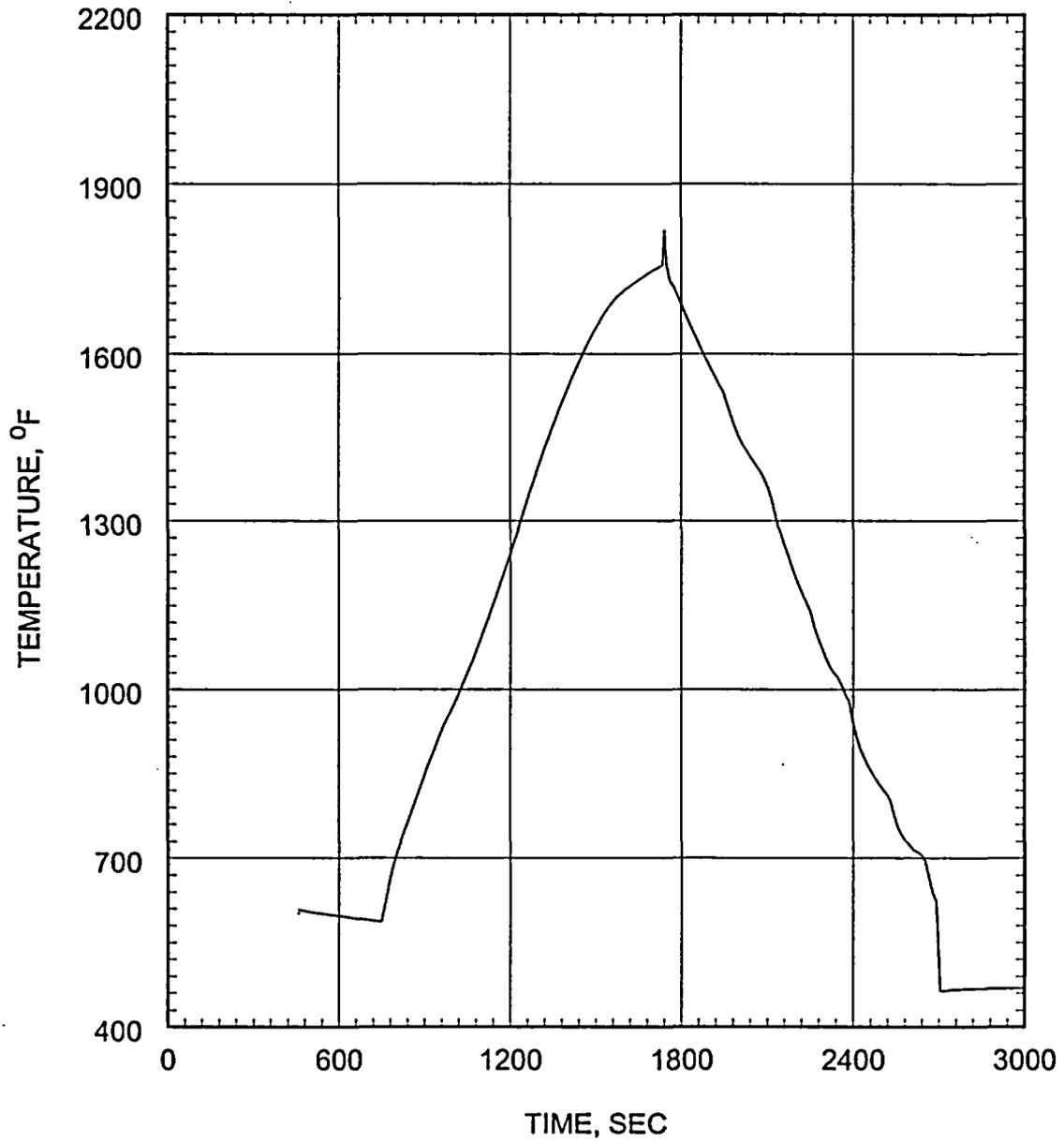
Figure 5.2.4.3-24 Small Break LOCA ECCS Performance Analysis 0.06 ft<sup>2</sup>/PD Break Cladding
