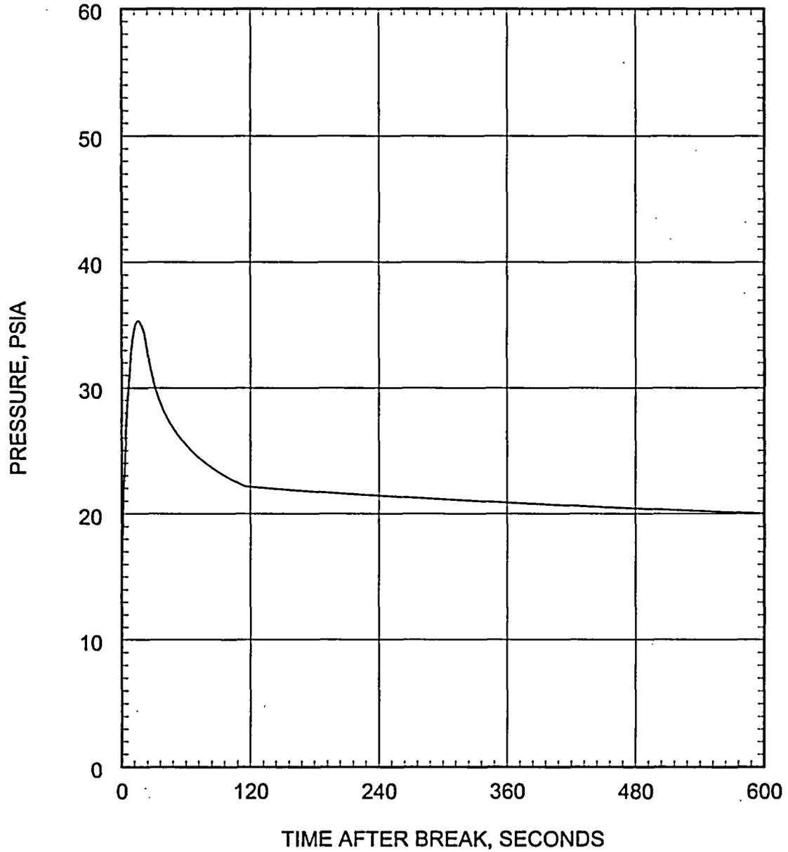
**Figure 5.2.3.3-25 Large Break LOCA ECCS Performance Analysis 0.6 DEG/PD Break
