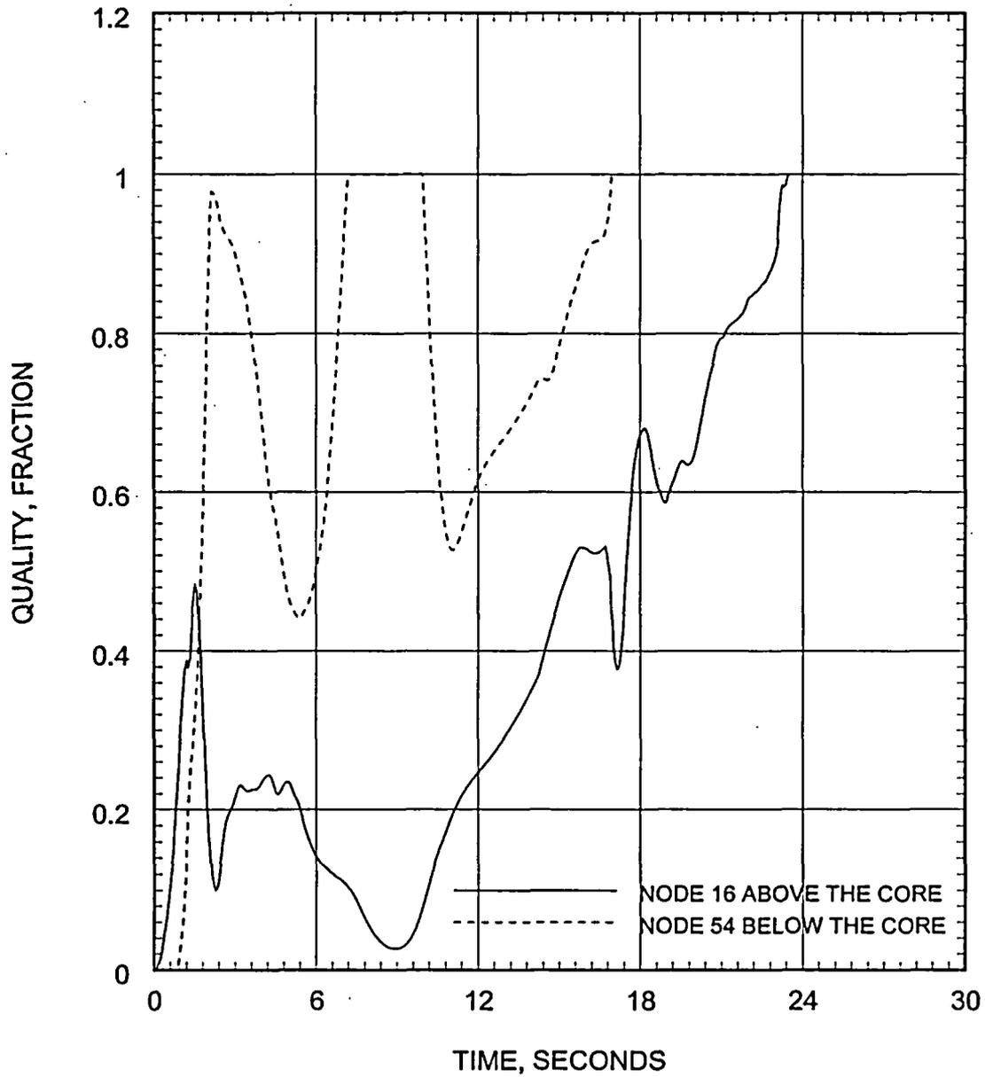
Figure 5.2.3.3-29 Large Break LOCA ECCS Performance Analysis 0.6 DEG/PD Break Quality Above and Below the Core
