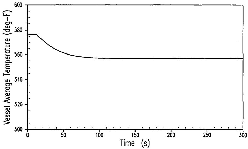
**Figure 5.1.18-8 Representative Transient Response to Dropped CEA Worth of 500 pcm at a Moderator Temperature Coefficient of  $-25 \text{ pcm}/^{\circ}\text{F}$  – Vessel Average Temperature versus Time**
