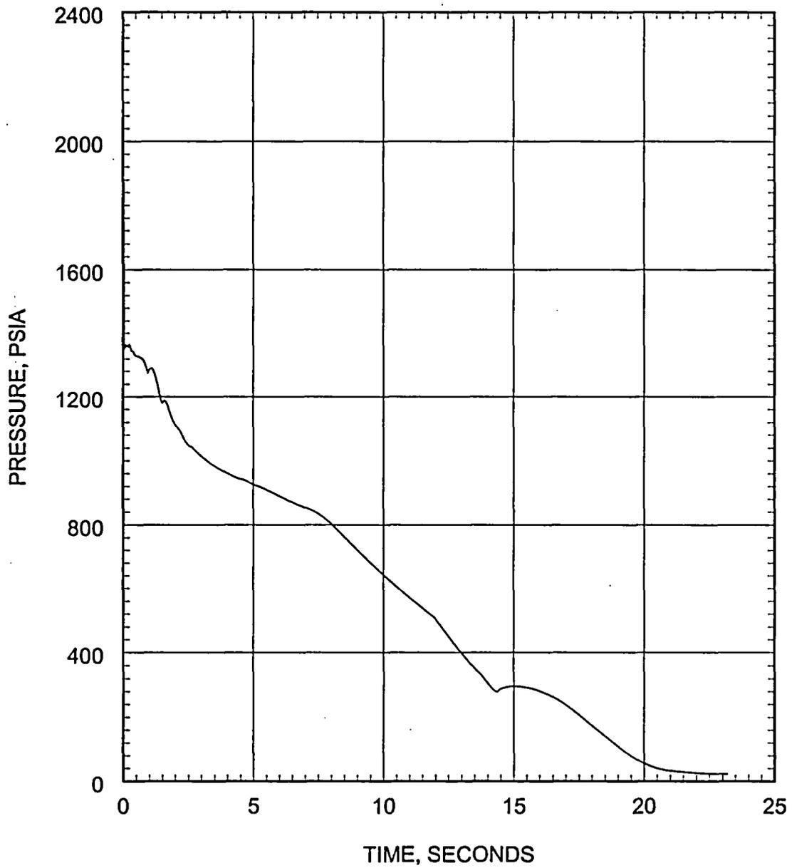
Figure 5.2.3.3-11 Large Break LOCA ECCS Performance Analysis 0.8 DEG/PD Break Pressure in Center Hot Assembly Node
