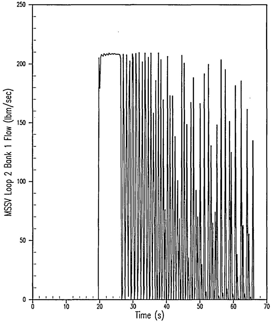
**Figure 5.1.11-21 Main Steam Safety Valve Flow (Loop 2 – Bank 1 Affected Steam Generator) for Asymmetric Steam Generator Transient 30% Tube Plugging**
