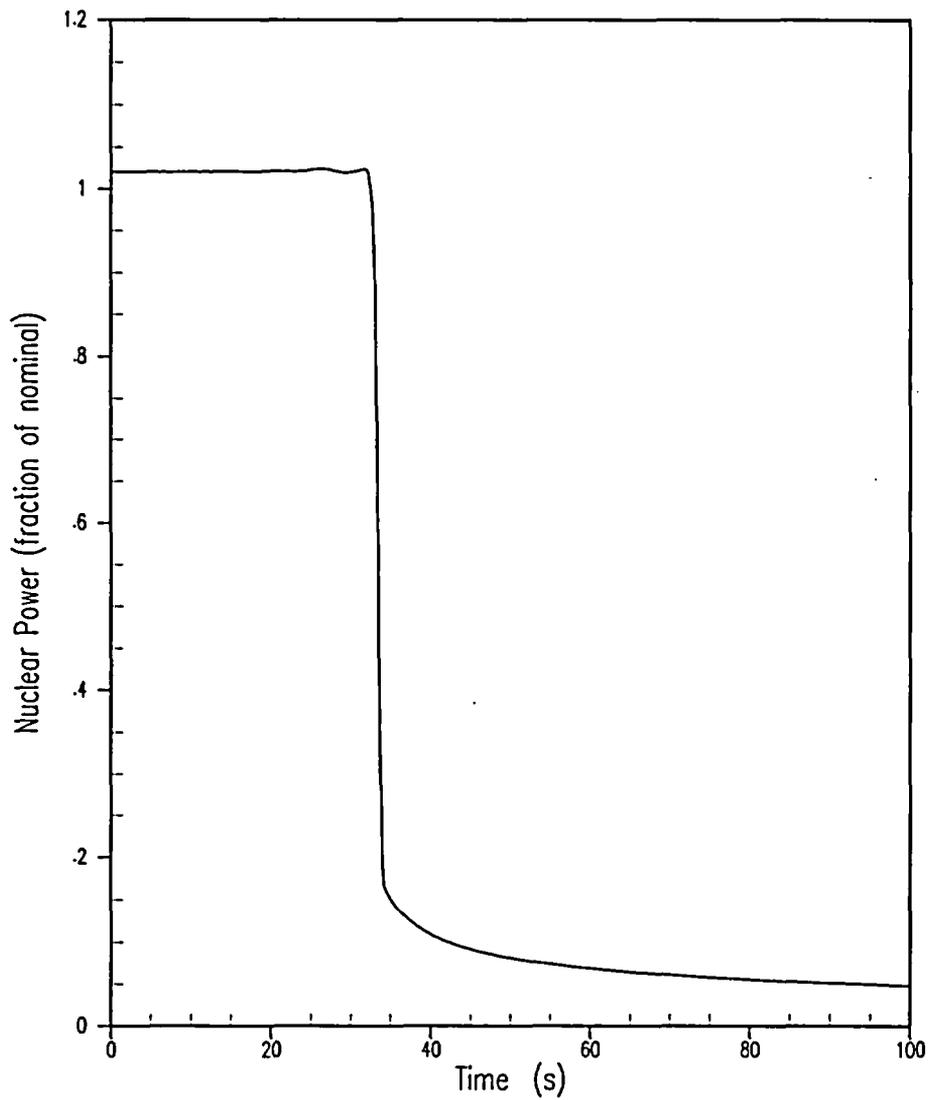
**Figure 5.1.12-1 Feedwater Line Break RCS Overpressure Case Limiting Break Size = 0.28 ft<sup>2</sup>
