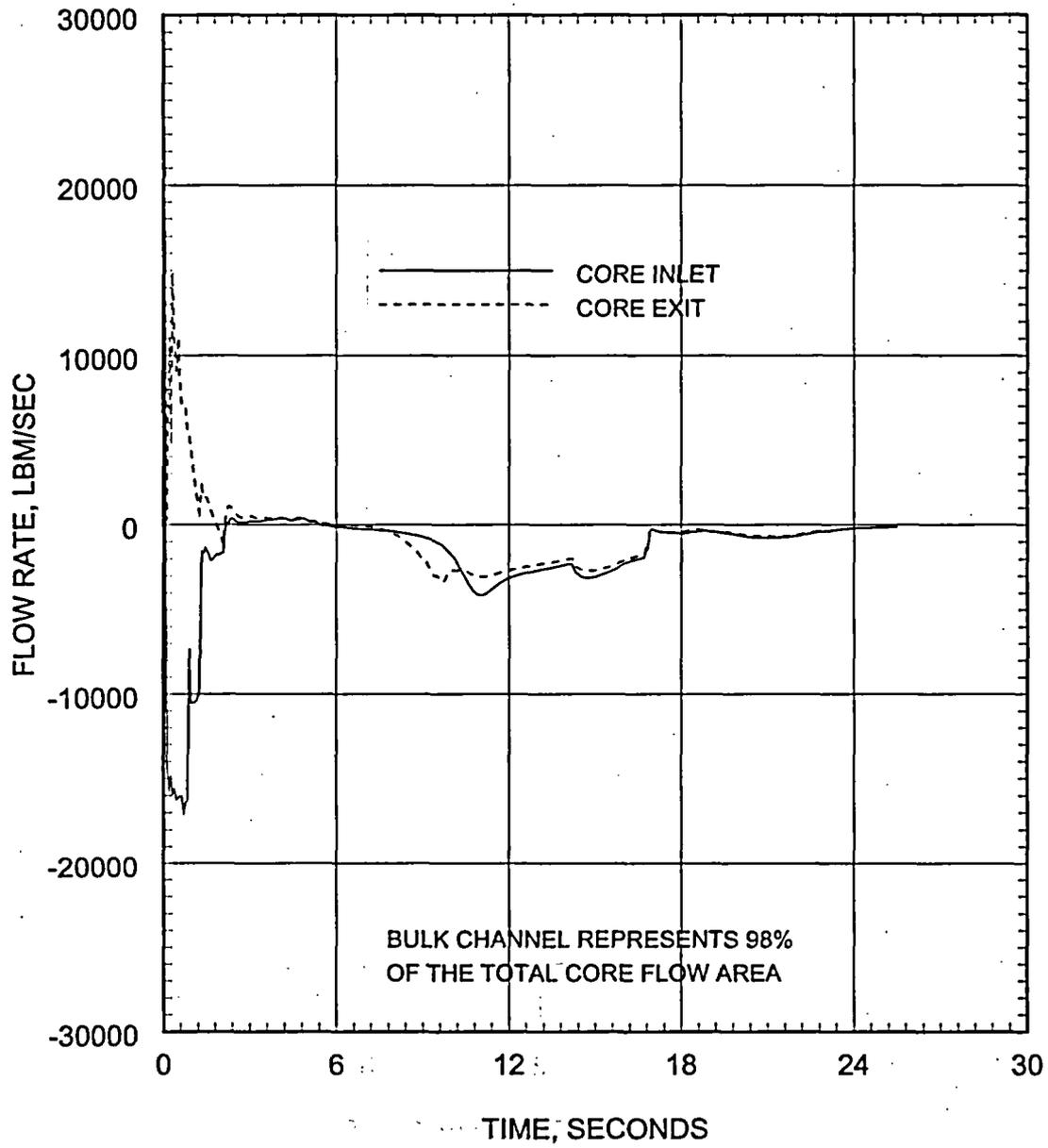
Figure 5.2.3.3-38 Large Break LOCA ECCS Performance Analysis 0.6 DEG/PD Break Core Bulk Channel Flow Rate
