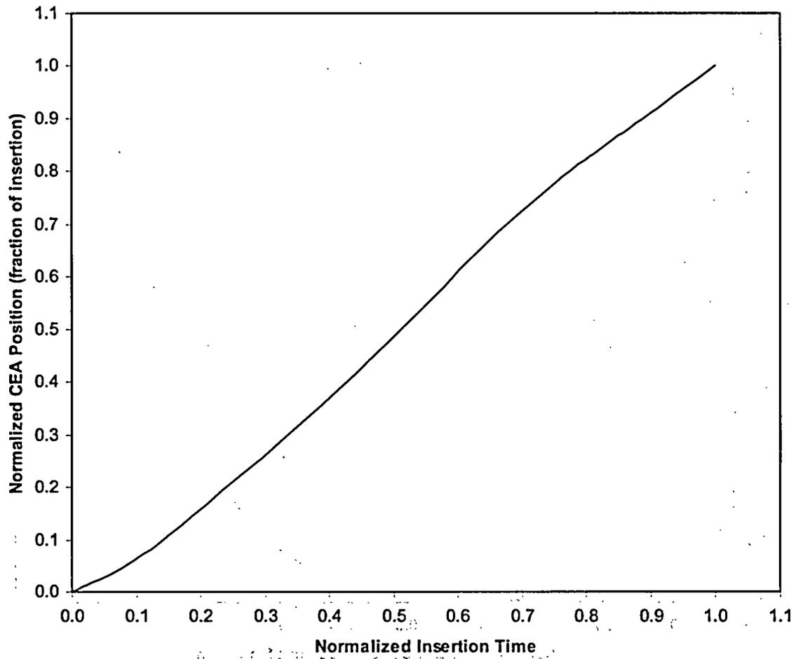
Figure 5.1.0-3 Normalized CEA Position vs. Time
