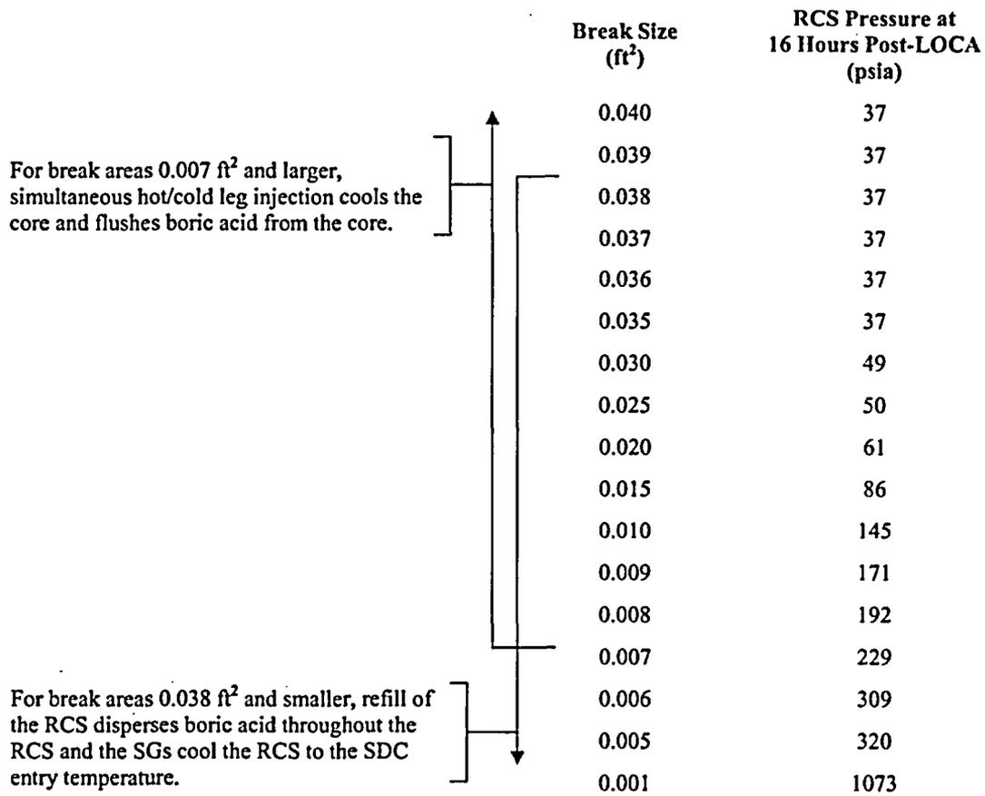
Figure 5.2.5.3-6 Long-Term Cooling Analysis Overlap of Acceptable Procedures in Terms of Break Size
