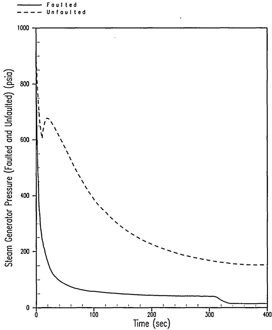
Figure 5.1.6-4 Post-Trip Main Steamline Break – Steam Generator Steam Pressure versus Time
