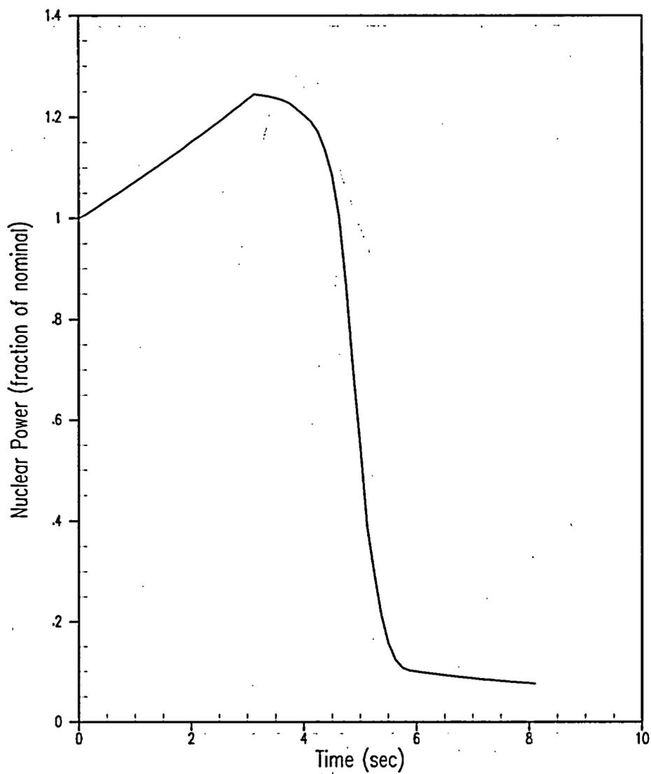
**Figure 5.1.16-1 Uncontrolled CEA Bank Withdrawal at Power 100% Power, 53 pcm/sec Reactivity Insertion Rate & Minimum Feedback Variable High Power Trip & Maximum Nominal RCS Vessel  $T_{avg}$  (Sheet 1 of 4)**
