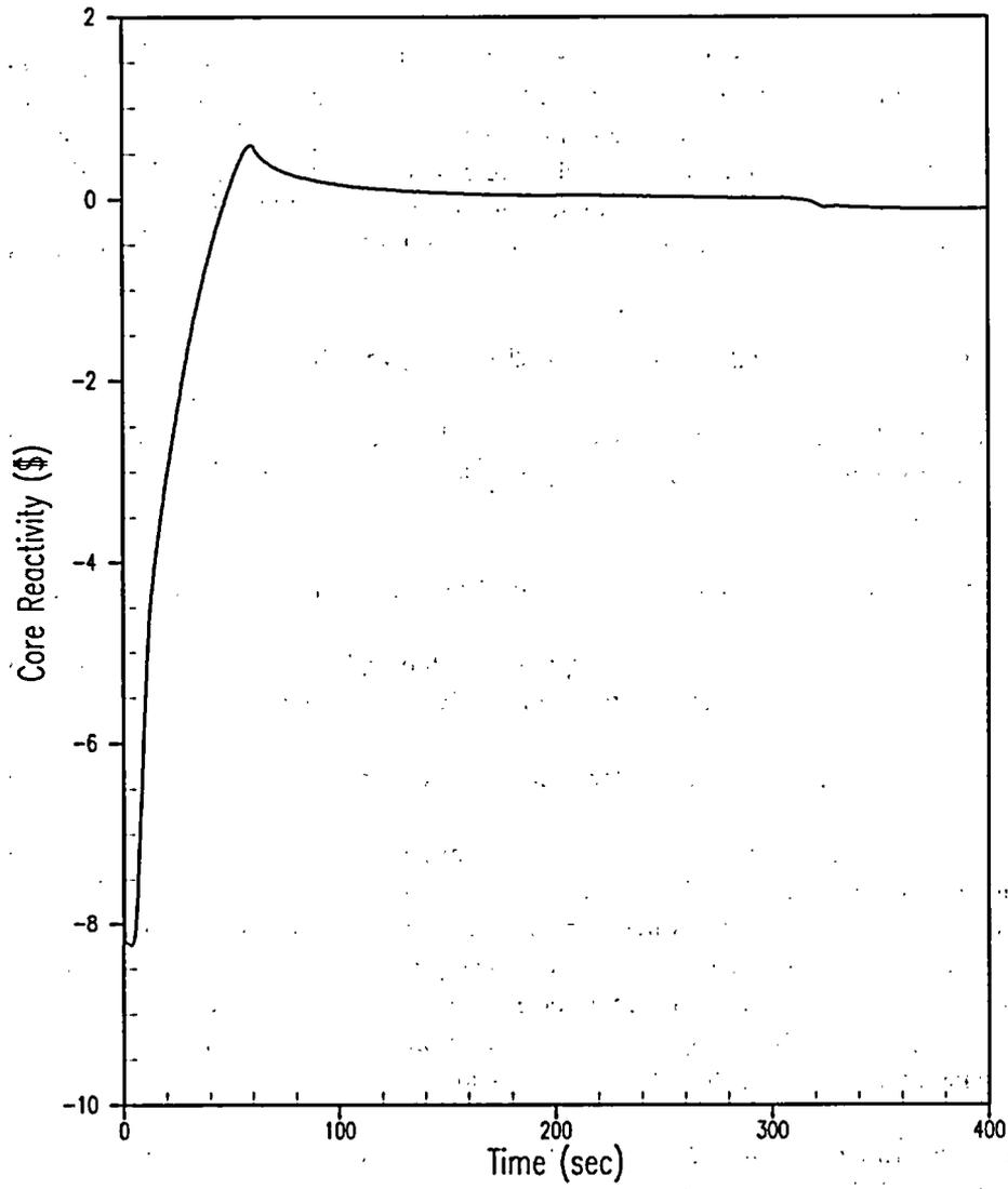
Figure 5.1.6-11 Post-Trip Main Steamline Break – Reactivity versus Time
