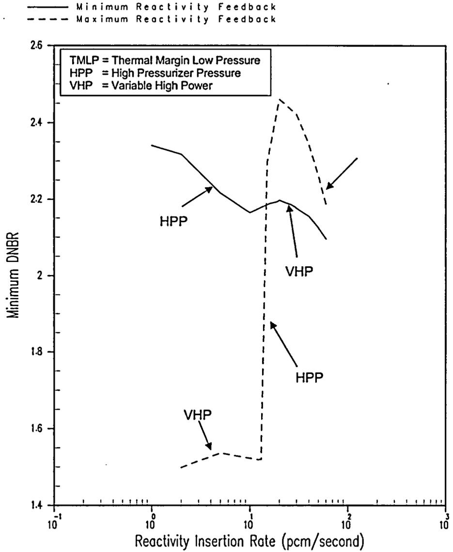
Figure 5.1.16-3 Uncontrolled CEA Bank Withdrawal at Power Initial Power Level of 65% (Sheet 2 of 4)
