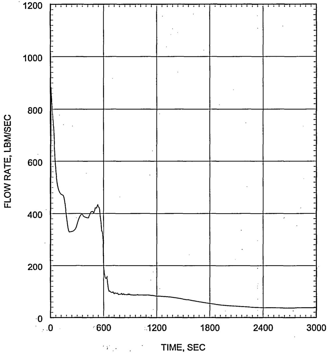
Figure 5.2.4.3-3 Small Break LOCA ECCS Performance Analysis 0.04 ft<sup>2</sup>/PD Break Break Flow Rate
