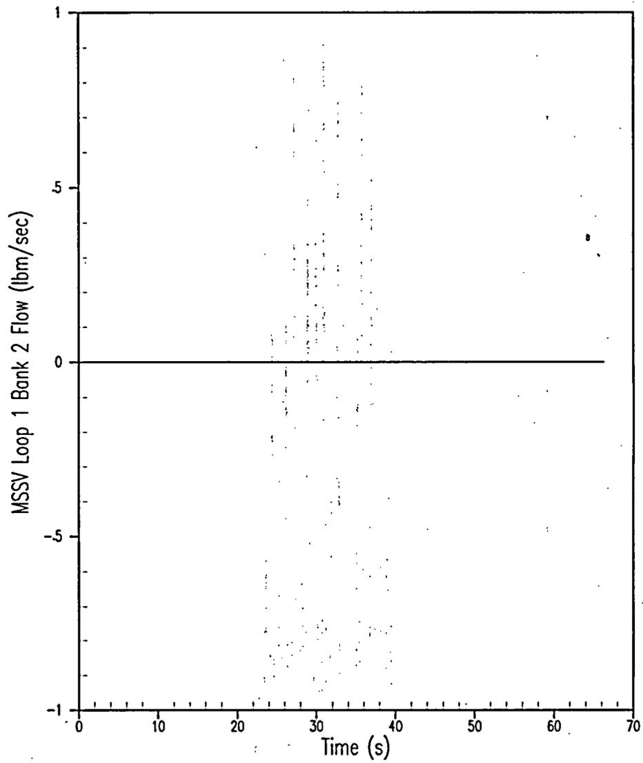
**Figure 5.1.11-22 Main Steam Safety Valve Flow (Loop 1 – Bank 2 Unaffected Steam Generator) for Asymmetric Steam Generator Transient 30% Tube Plugging**
