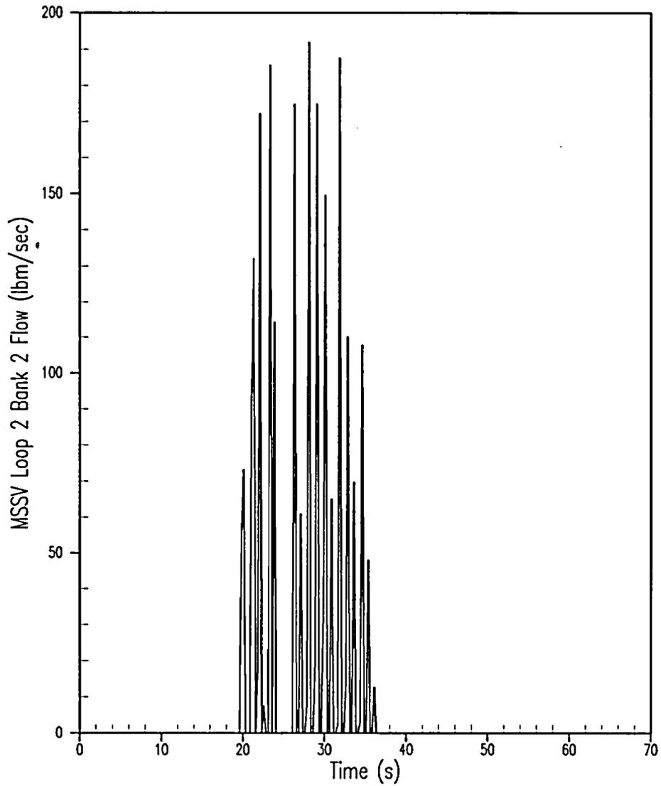
**Figure 5.1.11-23 Main Steam Safety Valve Flow (Loop 2 – Bank 2 Affected Steam Generator) for Asymmetric Steam Generator Transient 30% Tube Plugging**
