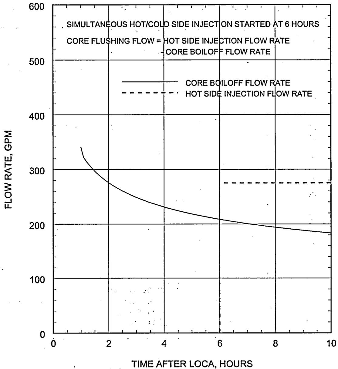
Figure 5.2.5.3-1 Long-Term Cooling Analysis Comparison of Core Boiloff Rate and the Minimum Simultaneous Hot and Cold Side Injection Flow Rate
