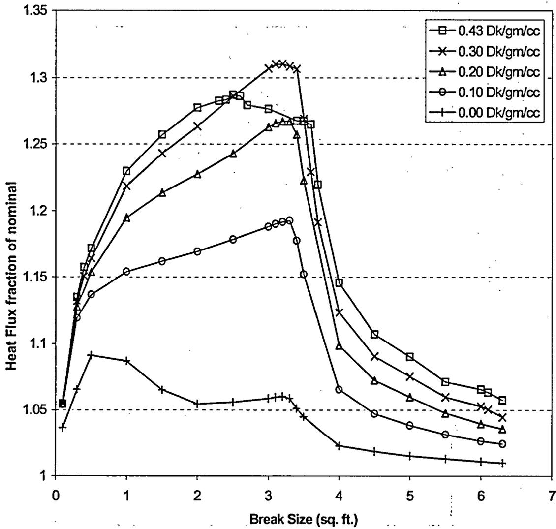
Figure 5.1.5-1 Summary of Peak Core Heat Flux vs. Break Size for a Spectrum of MDCs (0.0 to 0.43  $\Delta k/gm/cc$ )
