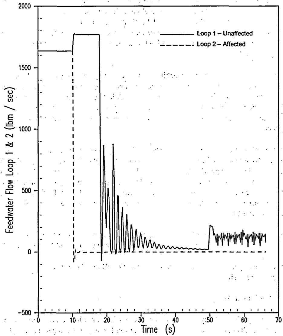
Figure 5.1.11-24 Feedwater Flow for Asymmetric Steam Generator Transient 30% Tube Plugging
