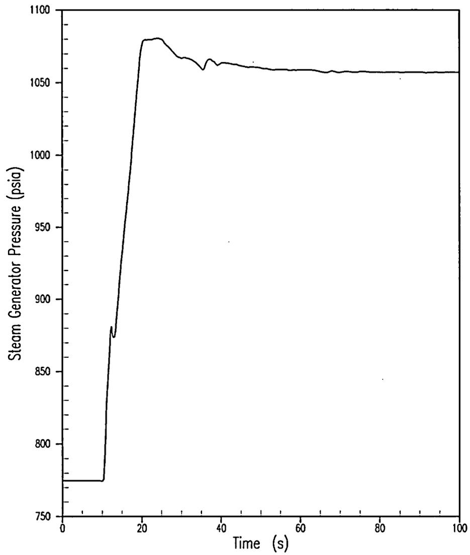
Figure 5.1.10-5 Loss of Condenser Vacuum (RCS Overpressure Case) Steam Generator Pressure
