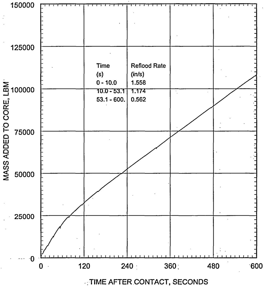
Figure 5.2.3.3-26 Large Break LOCA ECCS Performance Analysis 0.6 DEG/PD Break Mass Added to Core During Reflood
