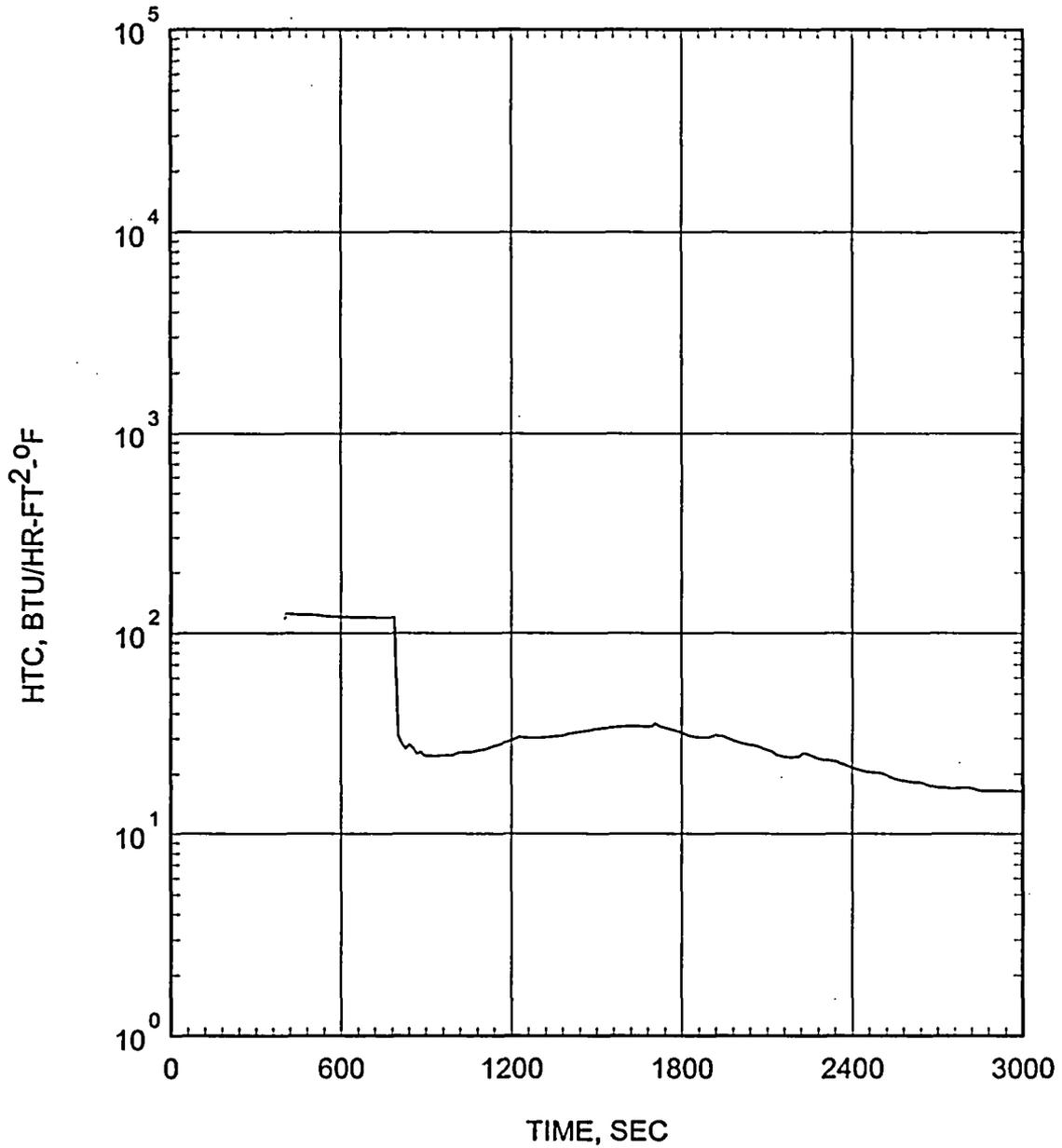
Figure 5.2.4.3-14 Small Break LOCA ECCS Performance Analysis 0.05 ft<sup>2</sup>/PD Break Heat Transfer Coefficient at Hot Spot
