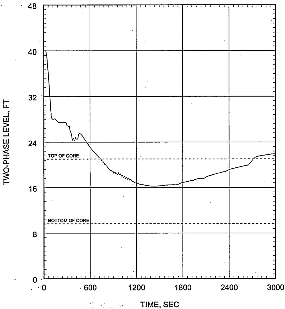
Figure 5.2.4.3-21 Small Break LOCA ECCS Performance Analysis 0.06 ft<sup>2</sup>/PD Break Inner Vessel Two-Phase Mixture Level
