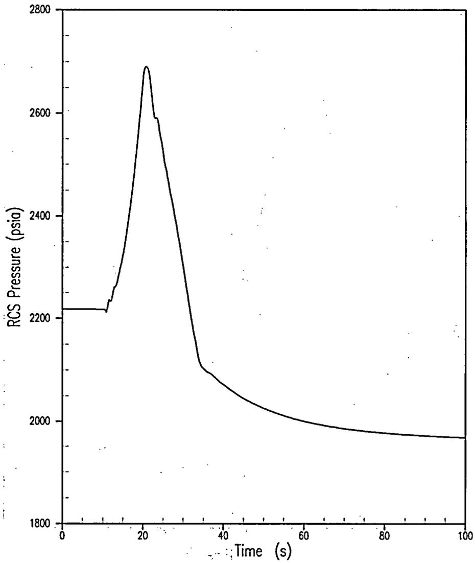
**Figure 5.1.10-2 Loss of Condenser Vacuum (RCS Overpressure Case) RCS Pressure (RCP Outlet Pressure)**
