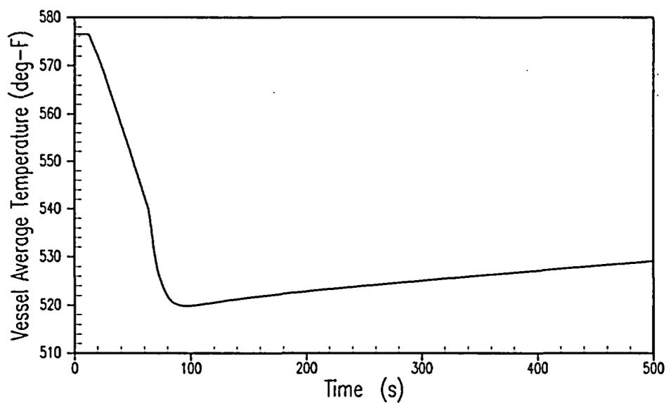
**Figure 5.1.18-4 Representative Transient Response to Dropped CEA Worth of 500 pcm at a Moderator Temperature Coefficient of 0 pcm/°F – Vessel Average Temperature versus Time**
