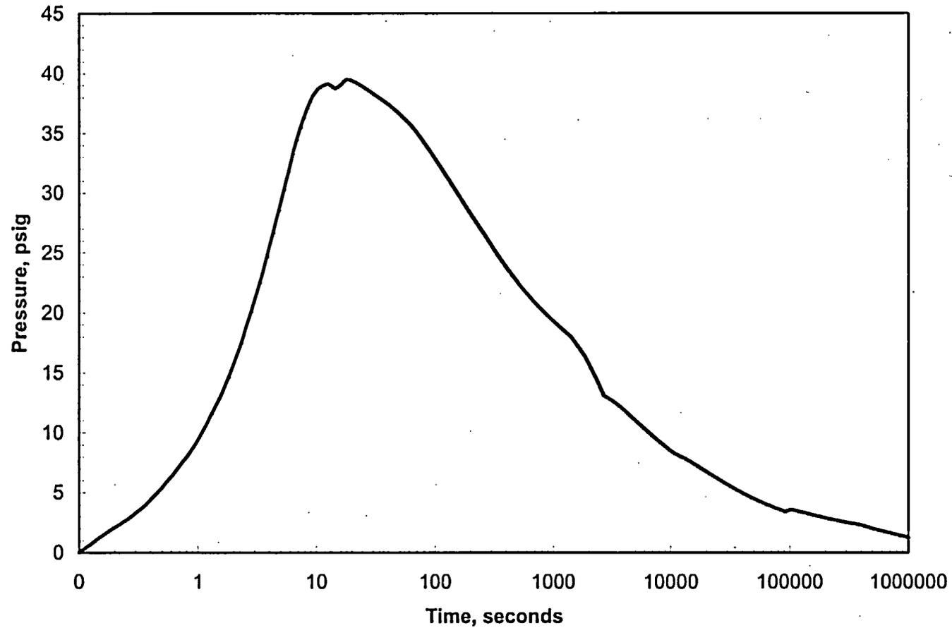
Figure 5.5-1 St. Lucie 2 LOCA Containment Analysis – Pressure vs. Time – 19.24 ft<sup>2</sup> DEHLS, Min SI
