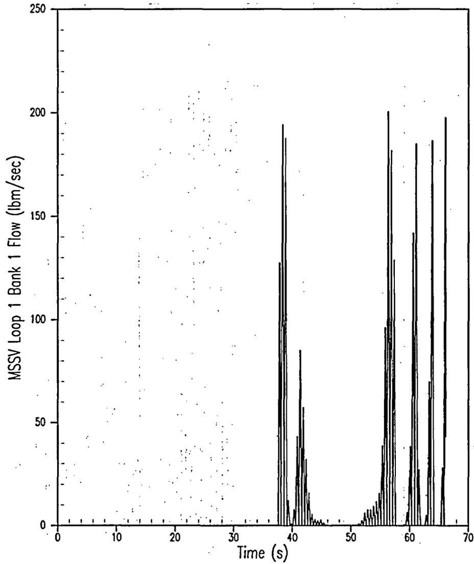
**Figure 5.1.11-8 Main Steam Safety Valve Flow (Loop 1 – Bank 1 Unaffected Steam Generator) for Asymmetric Steam Generator Transient 0% Tube Plugging**
