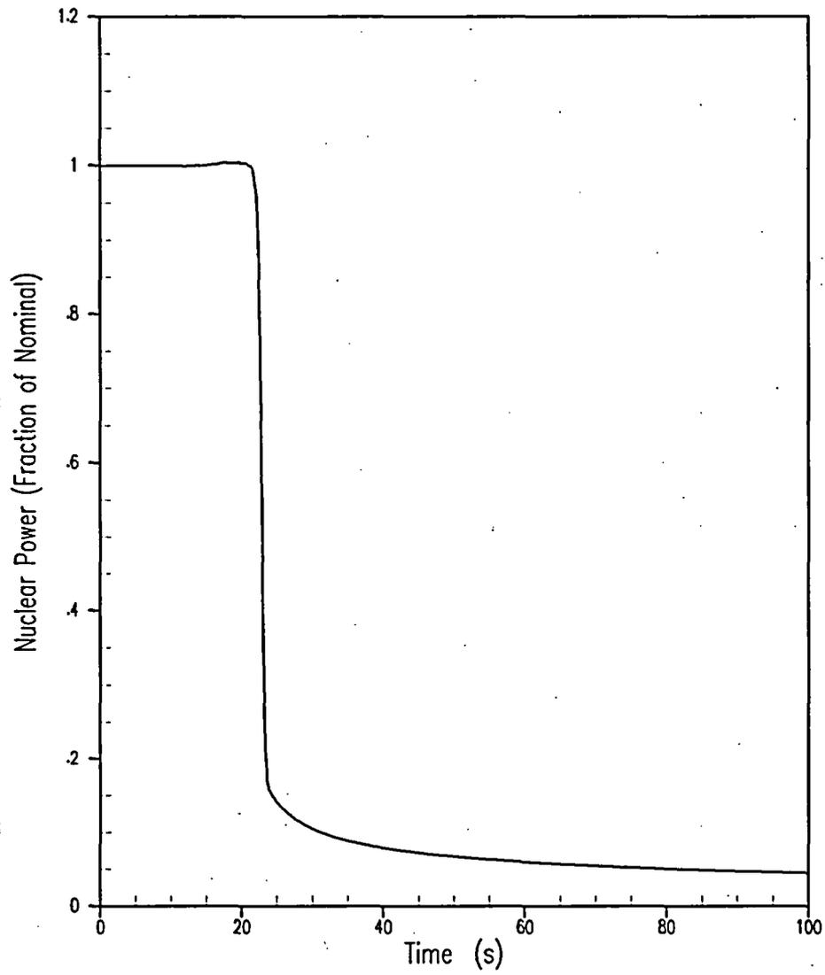
Figure 5.1.10-6 Loss of Condenser Vacuum (DNB Case) Nuclear Power
