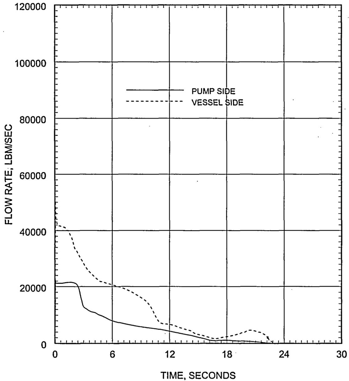
Figure 5.2.3.3-21 Large Break LOCA ECCS Performance Analysis 0.6 DEG/PD Break Leak Flow Rate
