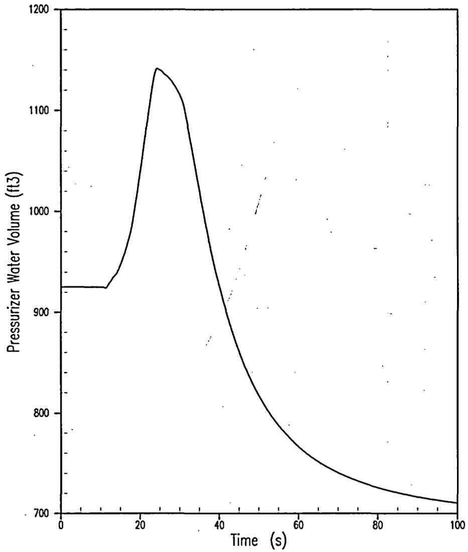
Figure 5.1.10-8 Loss of Condenser Vacuum (DNB Case) Pressurizer Water Volume
