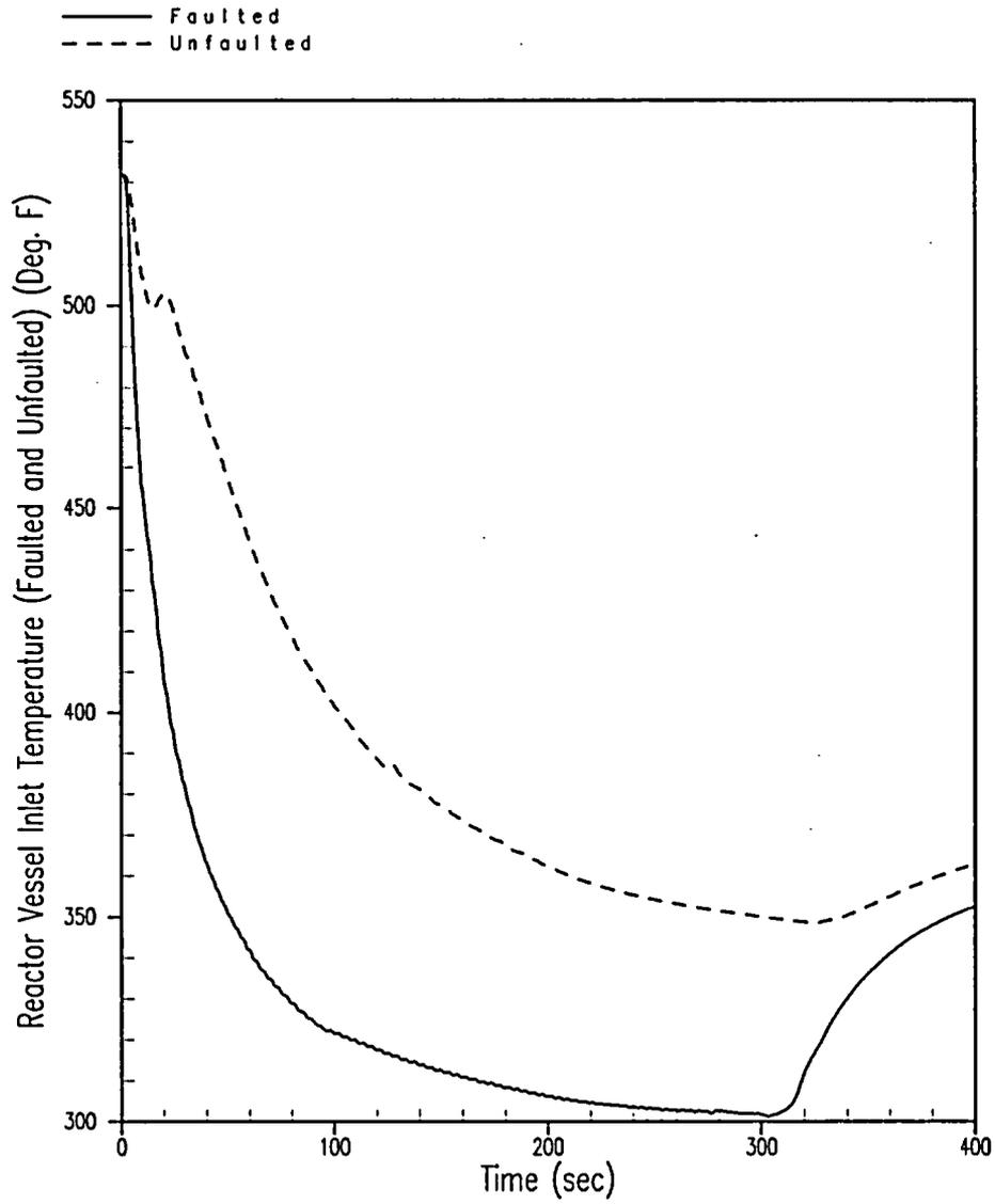
Figure 5.1.6-8 Post-Trip Main Steamline Break – Reactor Vessel Inlet Temperature versus Time
