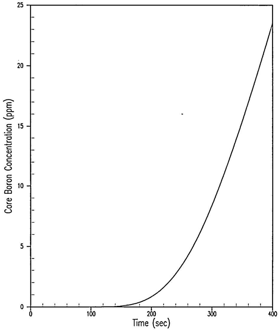
**Figure 5.1.6-10 Post-Trip Main Steamline Break – Core Averaged Boron Concentration versus Time**
