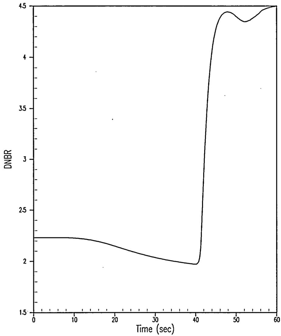
**Figure 5.1.1-7 DNBR for a Feedwater Malfunction Increased Feedwater Flow at HFP Initial Conditions**
