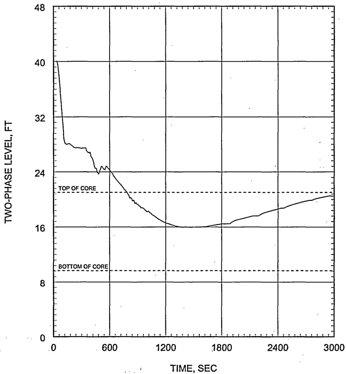
Figure 5.2.4.3-13 Small Break LOCA ECCS Performance Analysis 0.05 ft<sup>2</sup>/PD Break Inner Vessel
