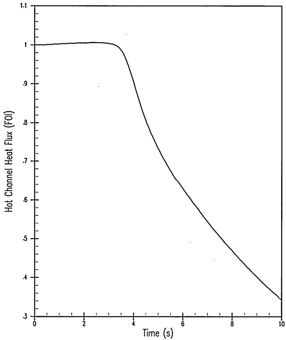
**Figure 5.1.14-7 Hot Channel Heat Flux versus Time – Complete Loss of Flow, Four Pumps Coasting Down (CLOF)**
