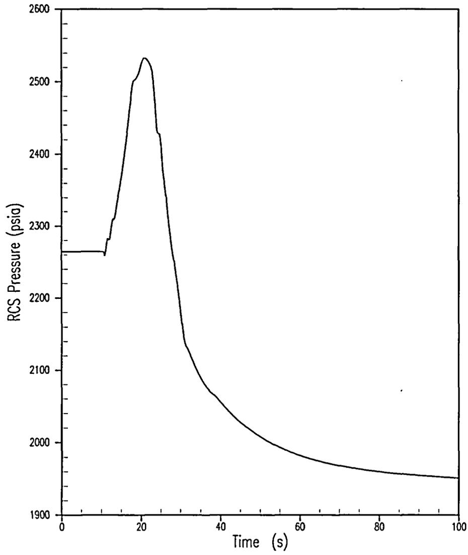
Figure 5.1.10-7 Loss of Condenser Vacuum (DNB Case) RCS Pressure (RCP Outlet Pressure)
