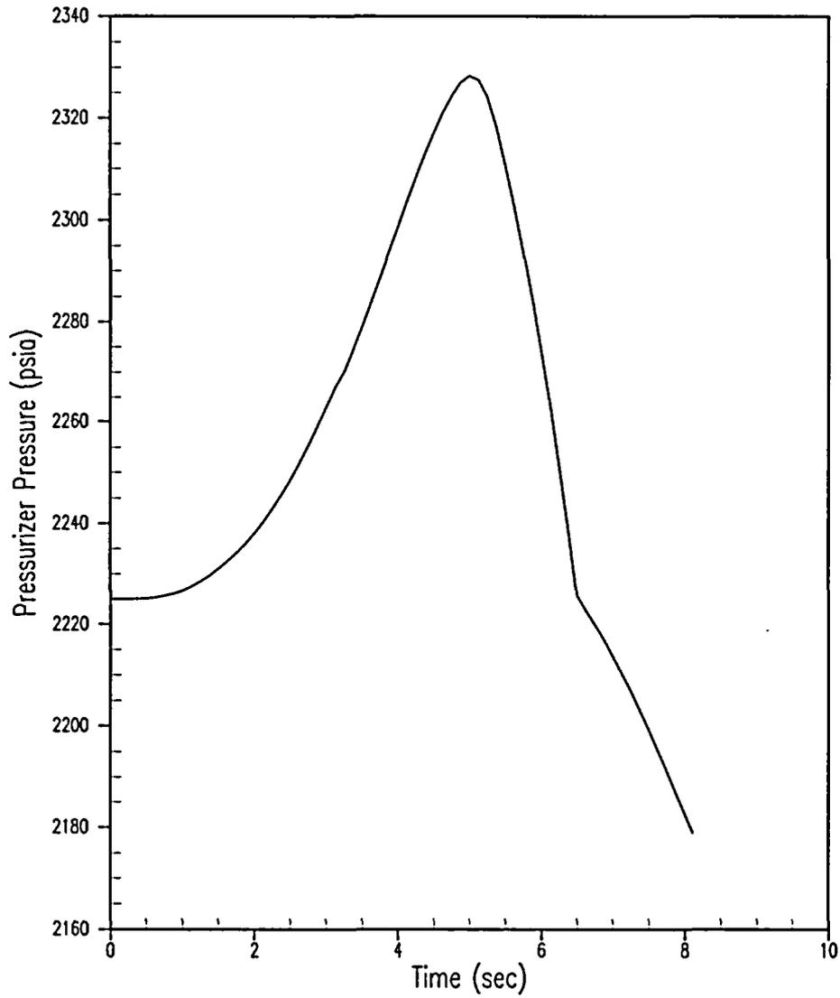
**Figure 5.1.16-1 Uncontrolled CEA Bank Withdrawal at Power 100% Power, 53 pcm/sec Reactivity Insertion Rate & Minimum Feedback Variable High Power Trip & Maximum Nominal RCS Vessel  $T_{avg}$  (Sheet 2 of 4)**
