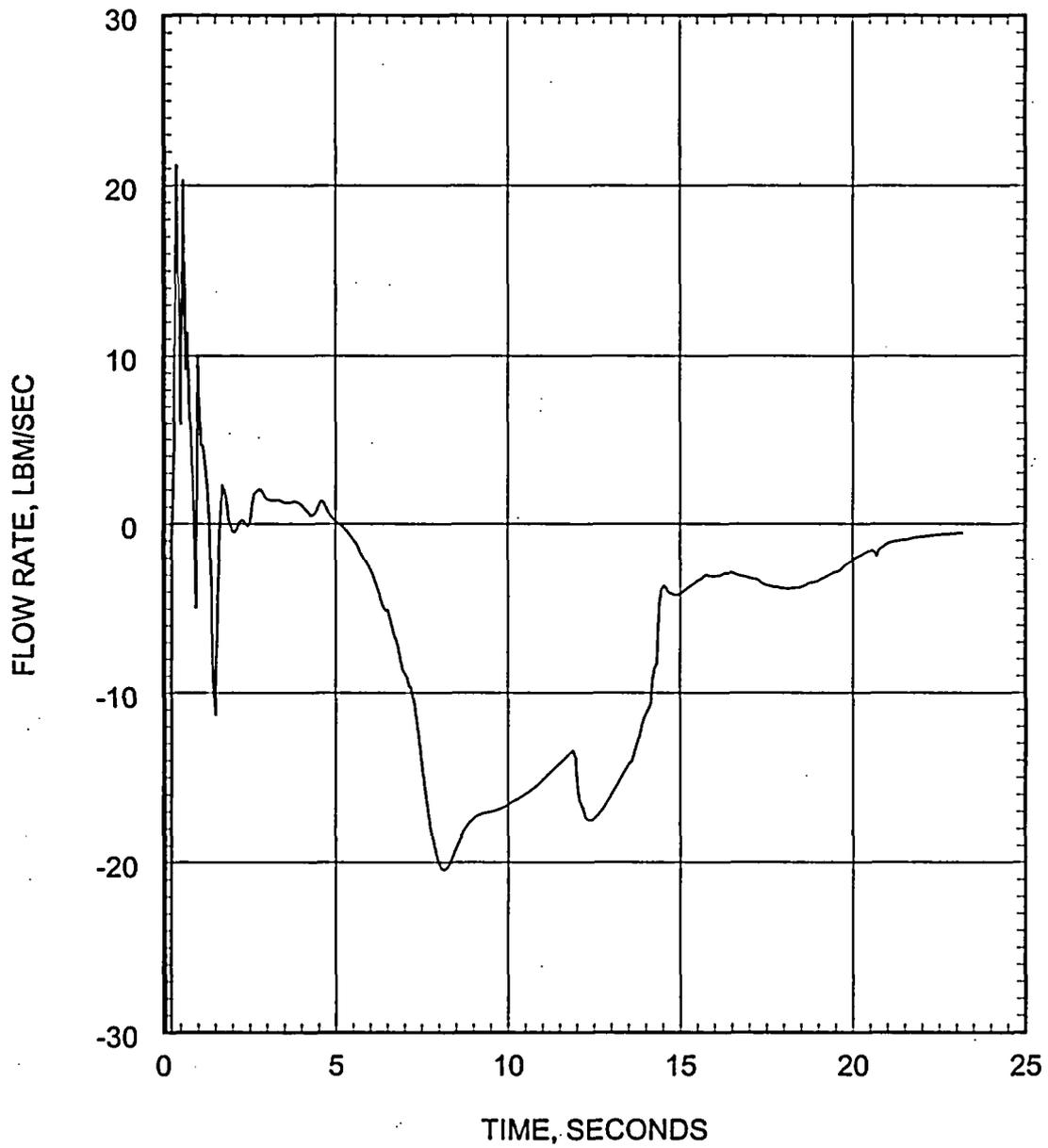
Figure 5.2.3.3-13 Large Break LOCA ECCS Performance Analysis 0.8 DEG/PD Break Hot
