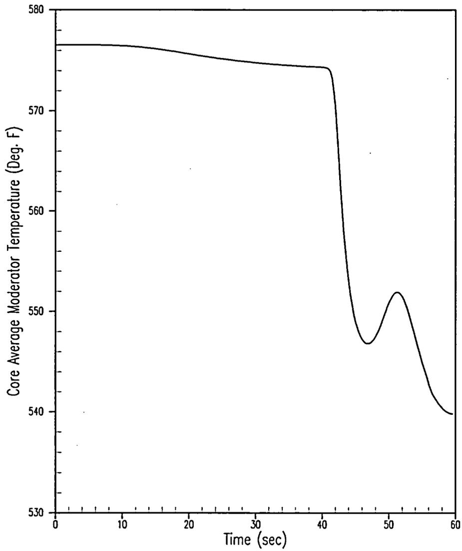
**Figure 5.1.1-5 Core Average Moderator Temperature for a Feedwater Malfunction Increased Feedwater Flow at HFP Initial Conditions**
