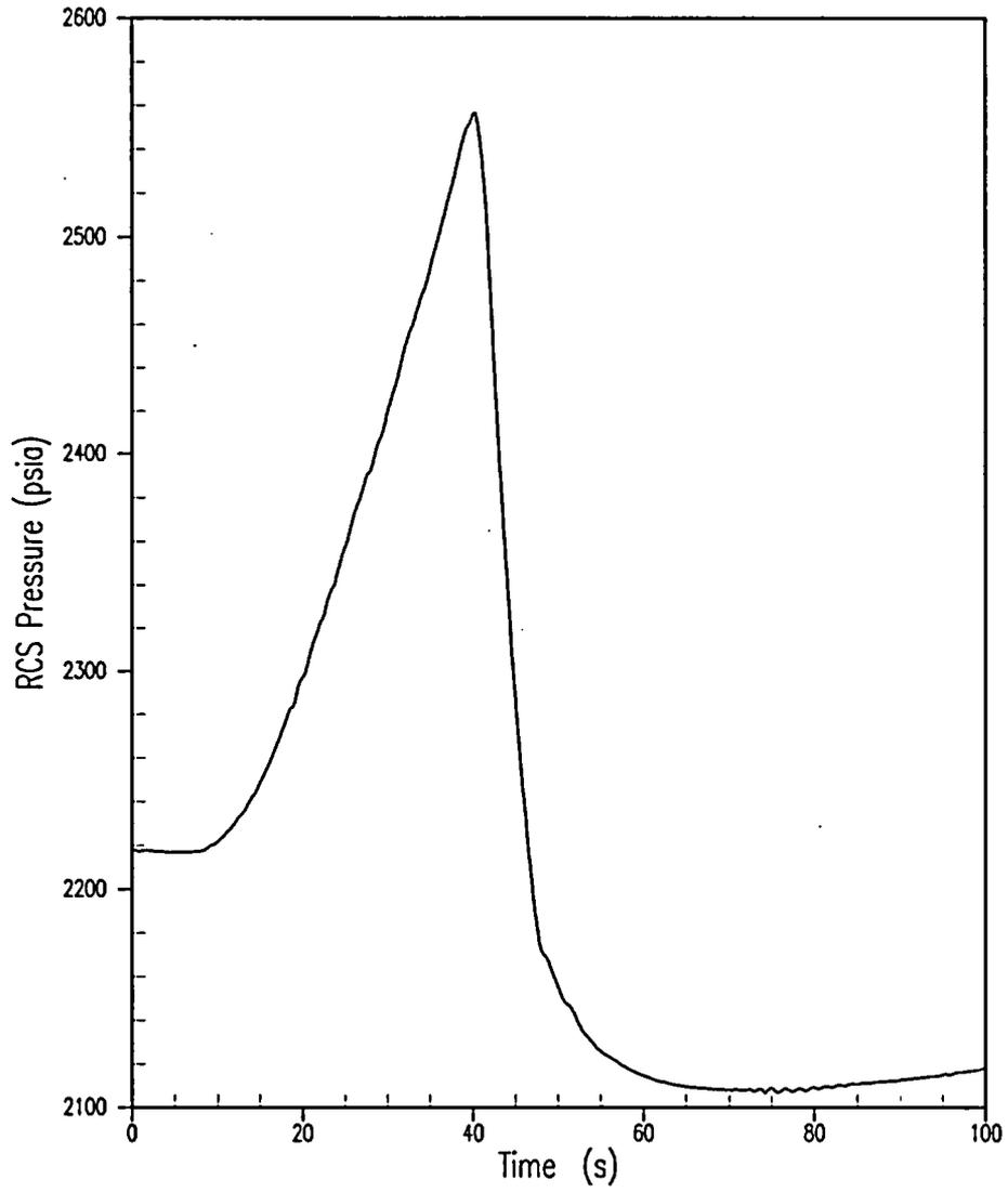
Figure 5.1.12-9 Feedwater Line Break MSS Overpressure Case Limiting Break Size = 0.05 ft<sup>2</sup> RCS Pressure
