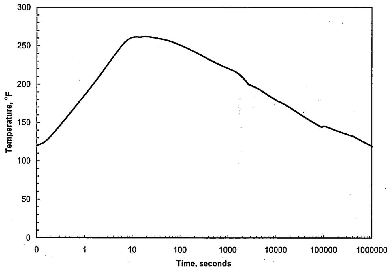
Figure 5.5-2 St. Lucie 2 LOCA Containment Analysis – Temperature vs. Time – 19.24 ft<sup>2</sup> DEHLS, Min SI
