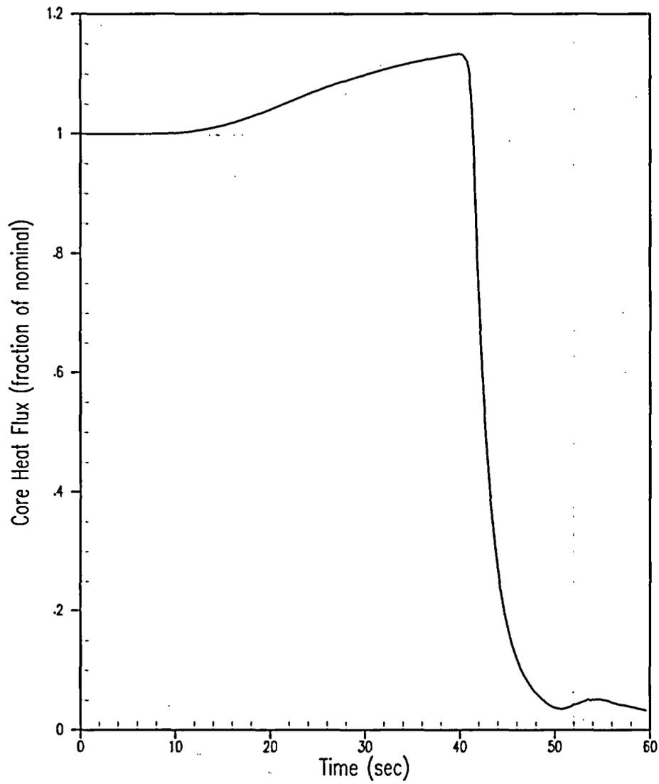
**Figure 5.1.1-2 Core Heat Flux for a Feedwater Malfunction Increased Feedwater Flow at HFP Initial Conditions**
