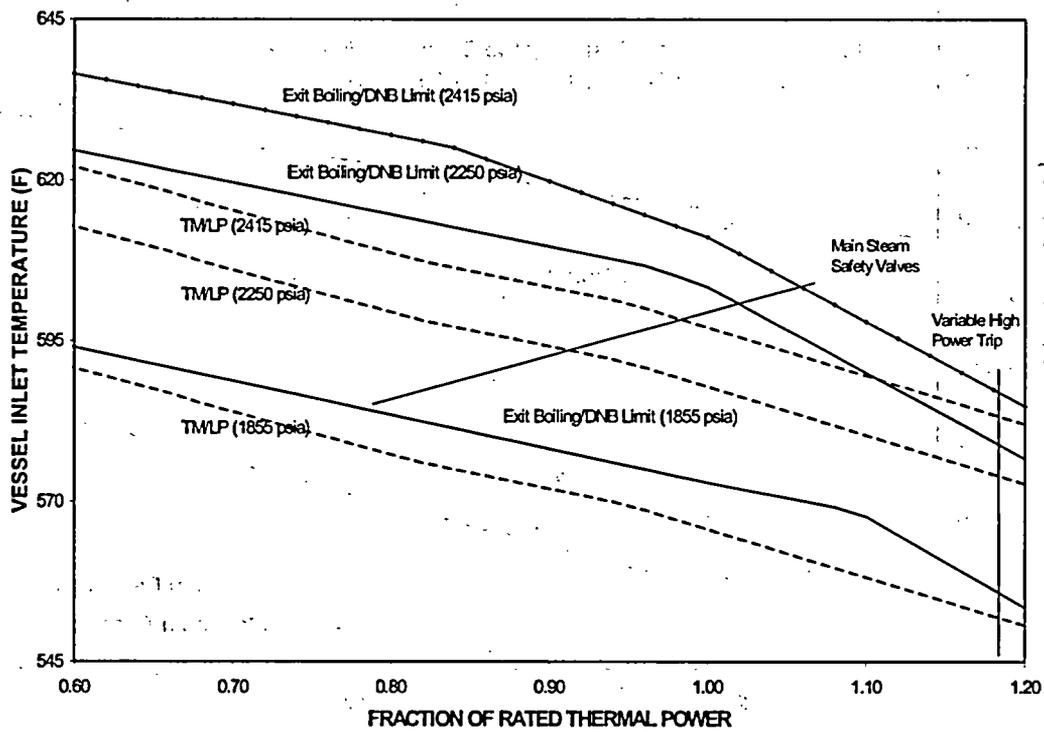
Figure 5.1.0-5 Illustration of the Thermal Margin/Low Pressure Reactor Trip Function and the Reference Core Thermal Limits
