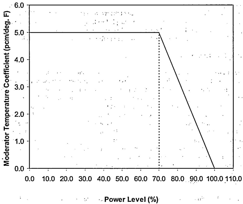
Figure 5.1.0-7 Moderator Temperature Coefficient Used in Accident Analyses
