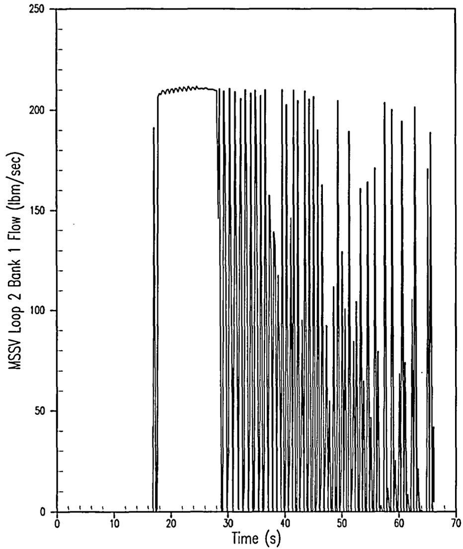
**Figure 5.1.11-9 Main Steam Safety Valve Flow (Loop 2 – Bank 1 Affected Steam Generator) for Asymmetric Steam Generator Transient 0% Tube Plugging**
