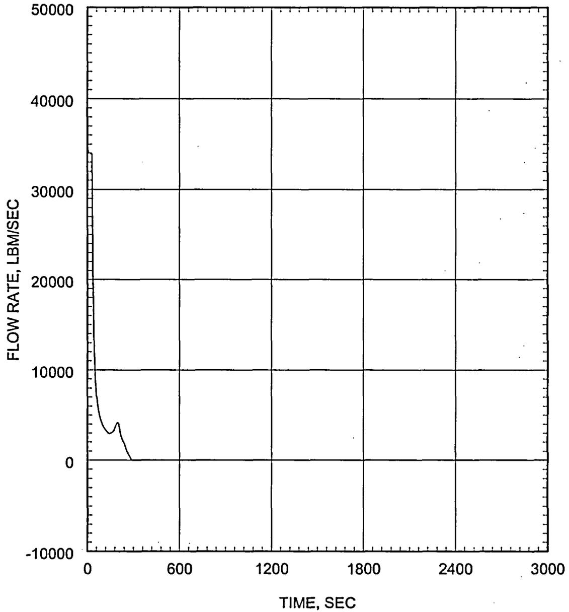
Figure 5.2.4.3-4. Small Break LOCA ECCS Performance Analysis 0.04 ft<sup>2</sup>/PD Break Inner Vessel Inlet Flow Rate
