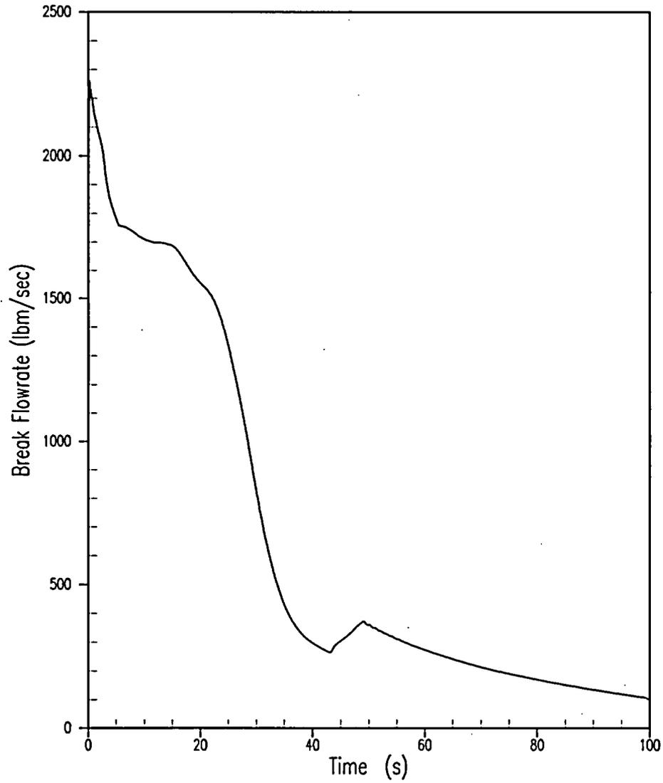
Figure 5.1.12-21 Feedwater Line Break DNB Case Limiting Break Size = 0.25 ft<sup>2</sup> Break Flowrate
