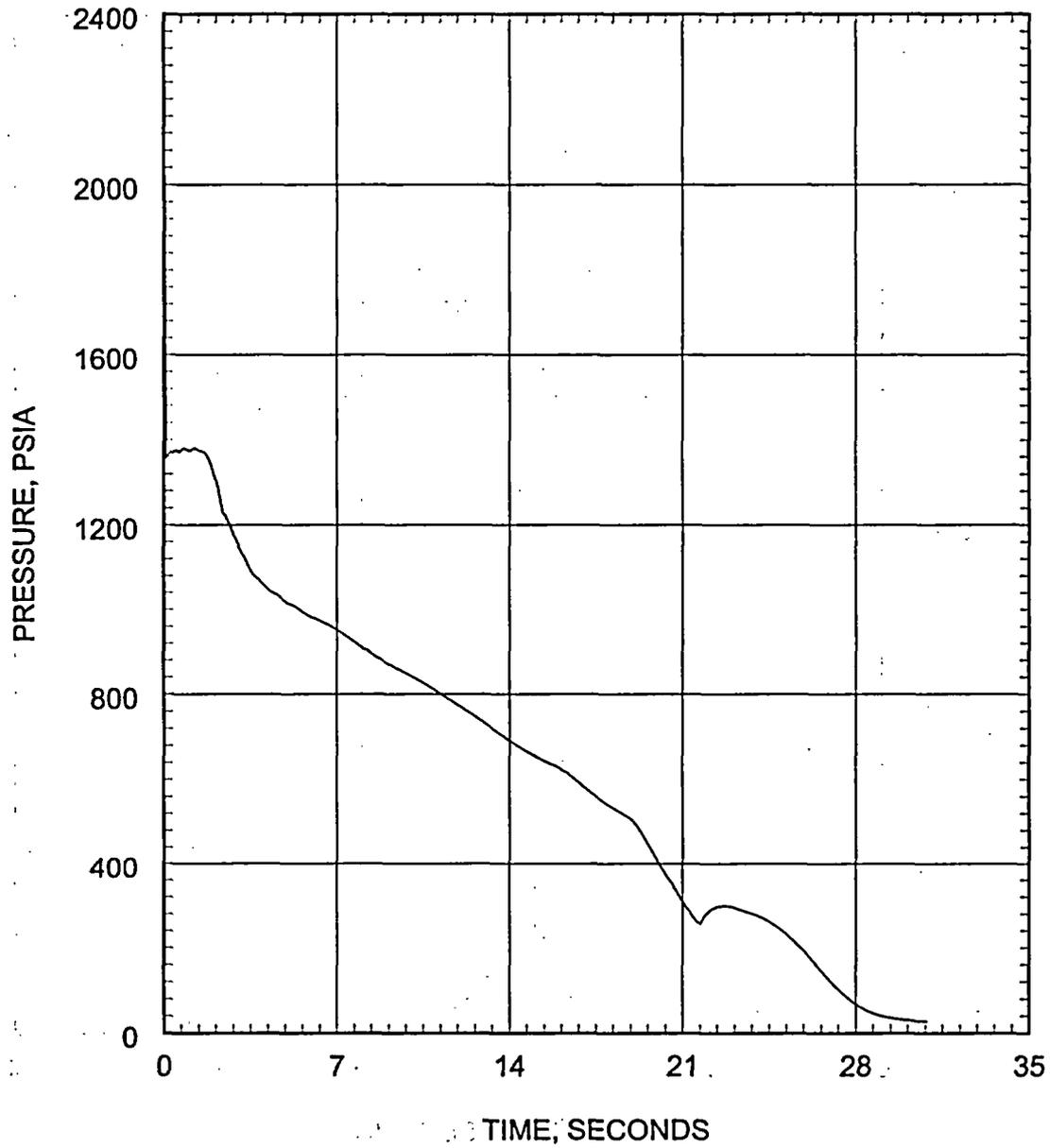
Figure 5.2.3.3-40 Large Break LOCA ECCS Performance Analysis 0.4 DEG/PD Break Pressure in Center Hot Assembly Node
