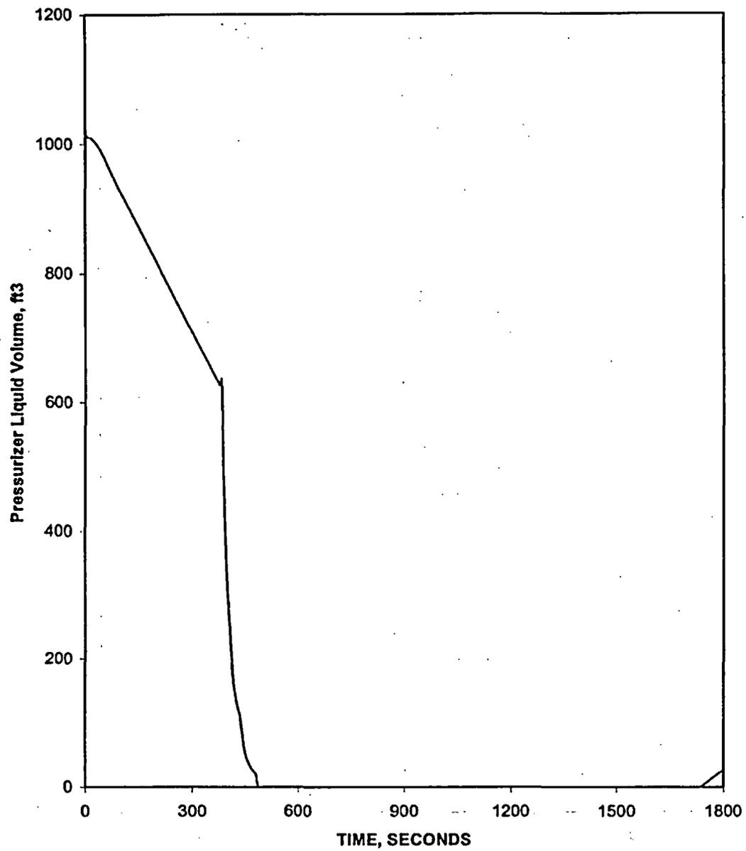
**Figure 5.1.24-12 Steam Generator Tube Rupture with Loss of Offsite Power –PZR Water Volume vs. Time**
