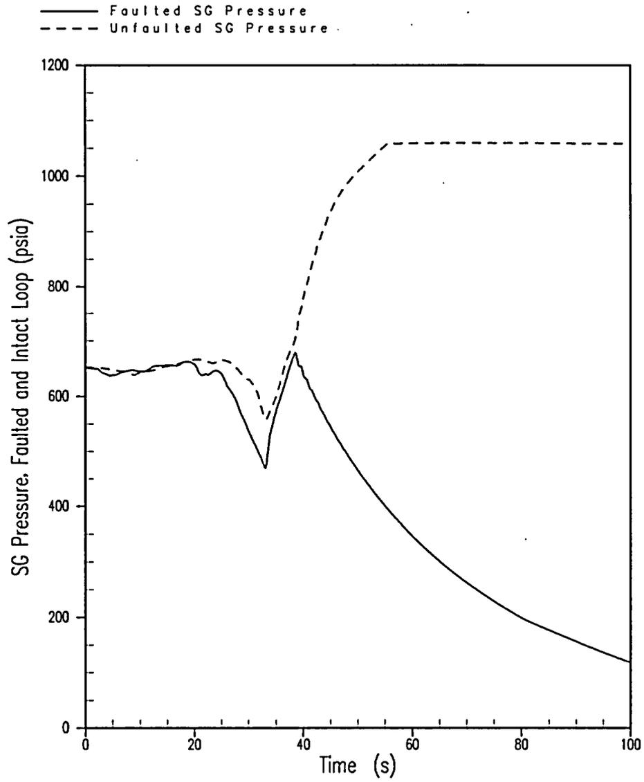
Figure 5.1.12-5 Feedwater Line Break RCS Overpressure Case Limiting Break Size = 0.28 ft<sup>2</sup> SG Pressure, Faulted and Intact Loop
