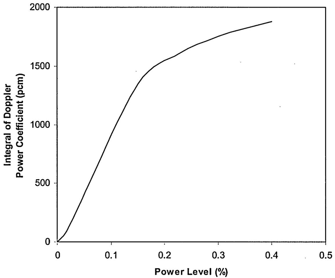
Figure 5.1.6-2 Stuck CEA Doppler Power Feedback
