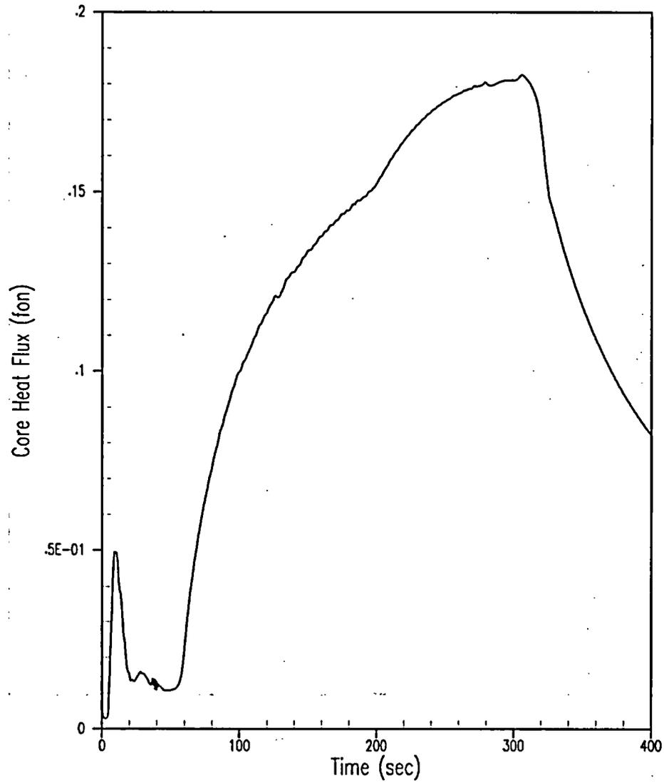
Figure 5.1.6-9 Post-Trip Main Steamline Break – Core Heat Flux versus Time
