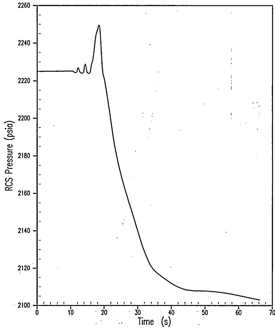
Figure 5.1.11-14 RCS Pressure for Asymmetric Steam Generator Transient 30% Tube Plugging
