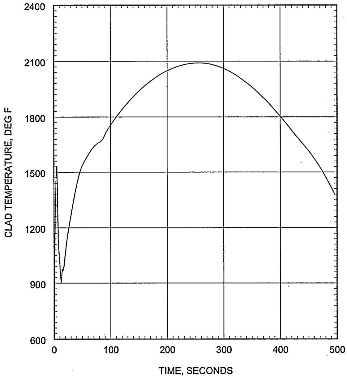
**Figure 5.2.3.3-9 Large Break LOCA ECCS Performance Analysis 1.0 DEG/PD Break Peak Cladding Temperature**
