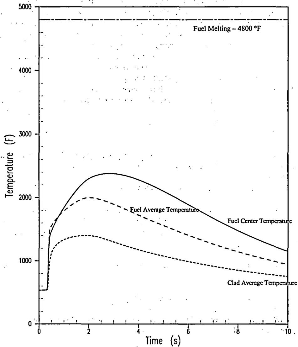
Figure 5.1.20-8 CEA Ejection Accident from Zero Power End of Cycle – Fuel and Cladding Temperatures versus Time
