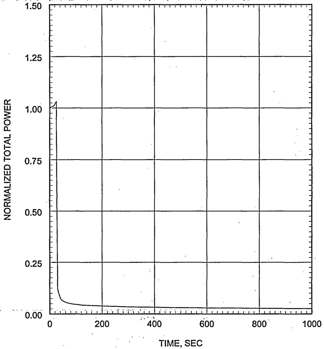
Figure 5.2.4.3-9 Small Break LOCA ECCS Performance Analysis 0.05 ft<sup>2</sup>/PD Break Core Power
