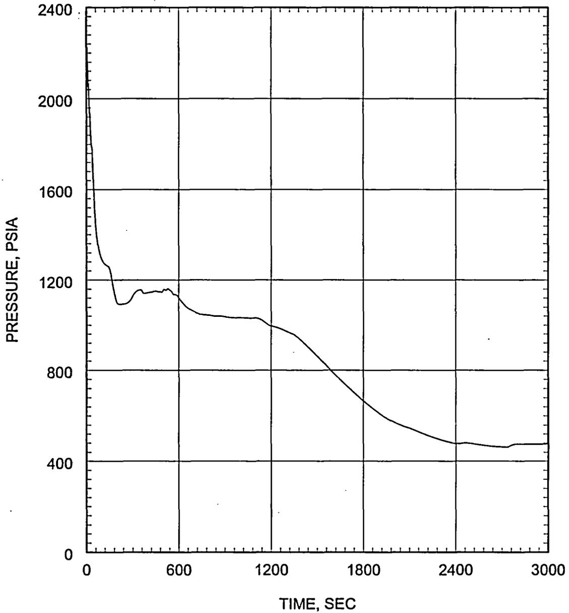
Figure 5.2.4.3-2 Small Break LOCA ECCS Performance Analysis 0.04 ft<sup>2</sup>/PD Break Inner Vessel Pressure
