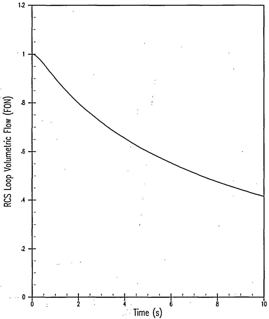
**Figure 5.1.14-2 RCS Loop Flow versus Time – Complete Loss of Flow – Four Pumps Coasting Down (CLOF)**
