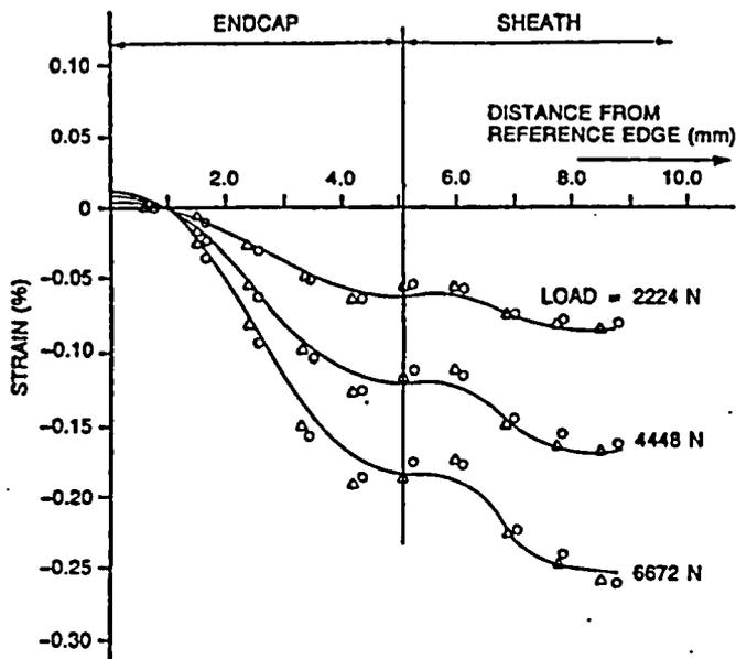
Figure 4 End cap strain: finite element vs measurements
