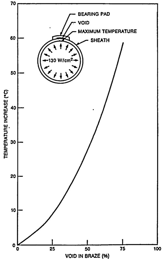
Figure 12 Increase in maximum sheath temperature due to void in braze
