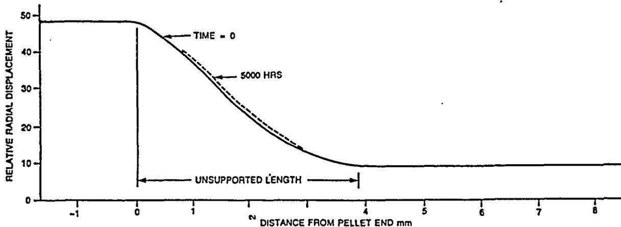
Figure 8 Creep of sheath on a pellet of reduced diameter
