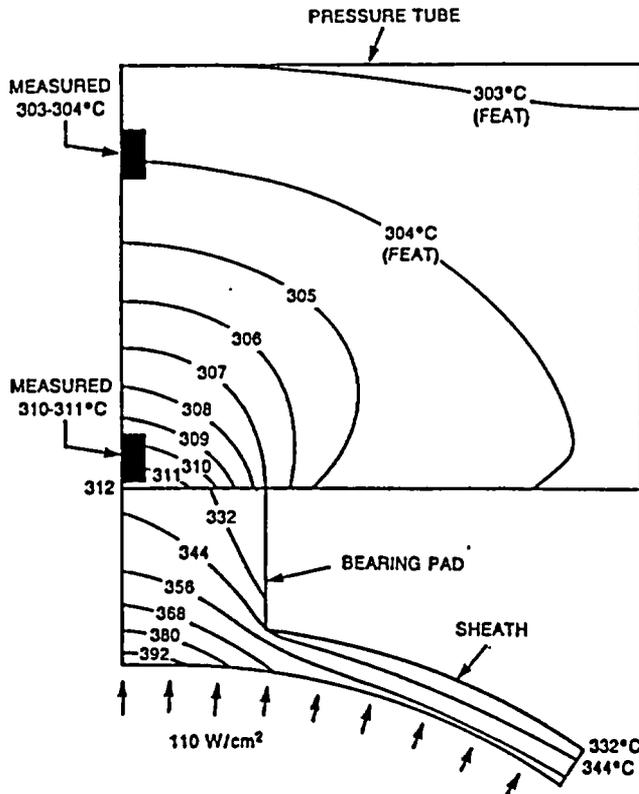
Figure 10 Isotherms ( $^{\circ}\text{C}$ ) near a bearing pad: Thermocouple measurements vs FEAT predictions
