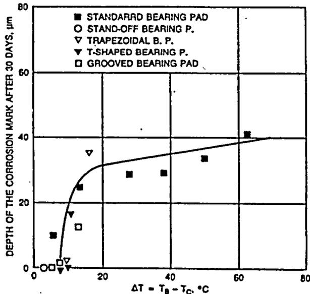
Figure 11 FEAT predictions for temperatures helped correlate corrosion rates in bearing pads of different designs
