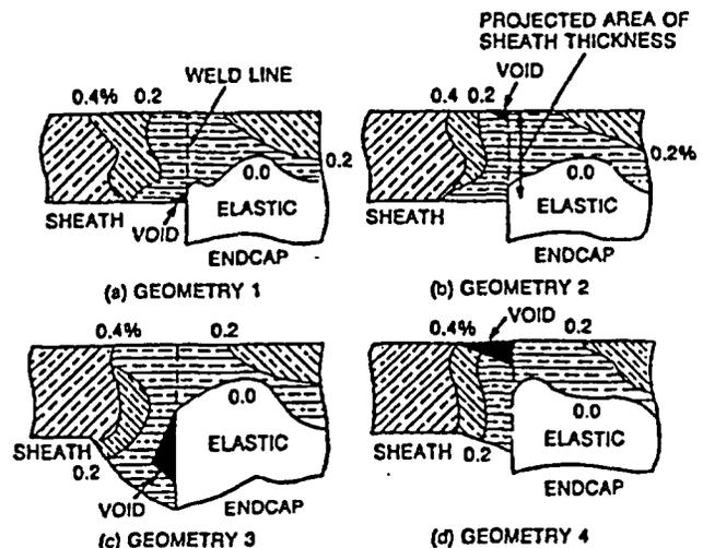
Figure 6 Plastic strains: Effect of discontinuity in the sheath/endcap weld
