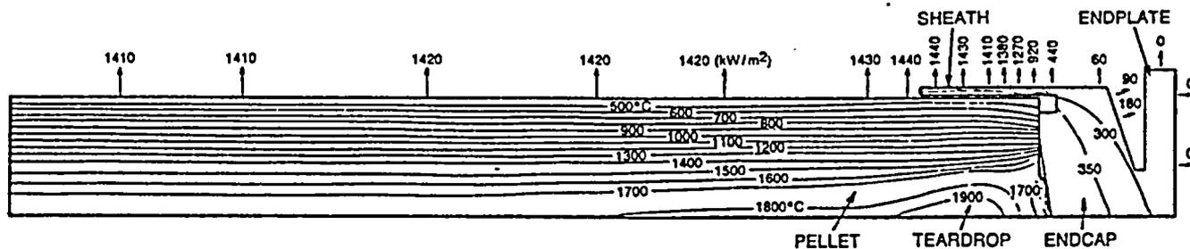
Figure 13 Isotherms (°C), heat flux (kW/m<sup>2</sup>), and tear drop near the end of a fuel stack
