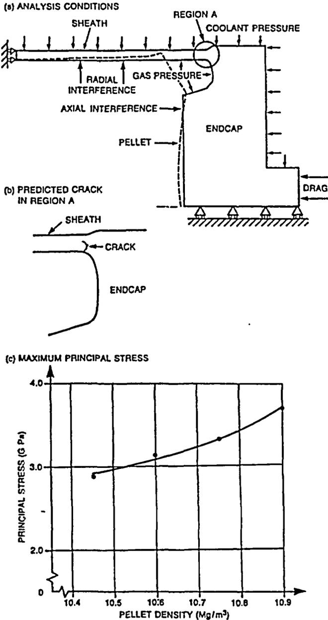
Figure 5 Higher pellet density gives larger weld stress
