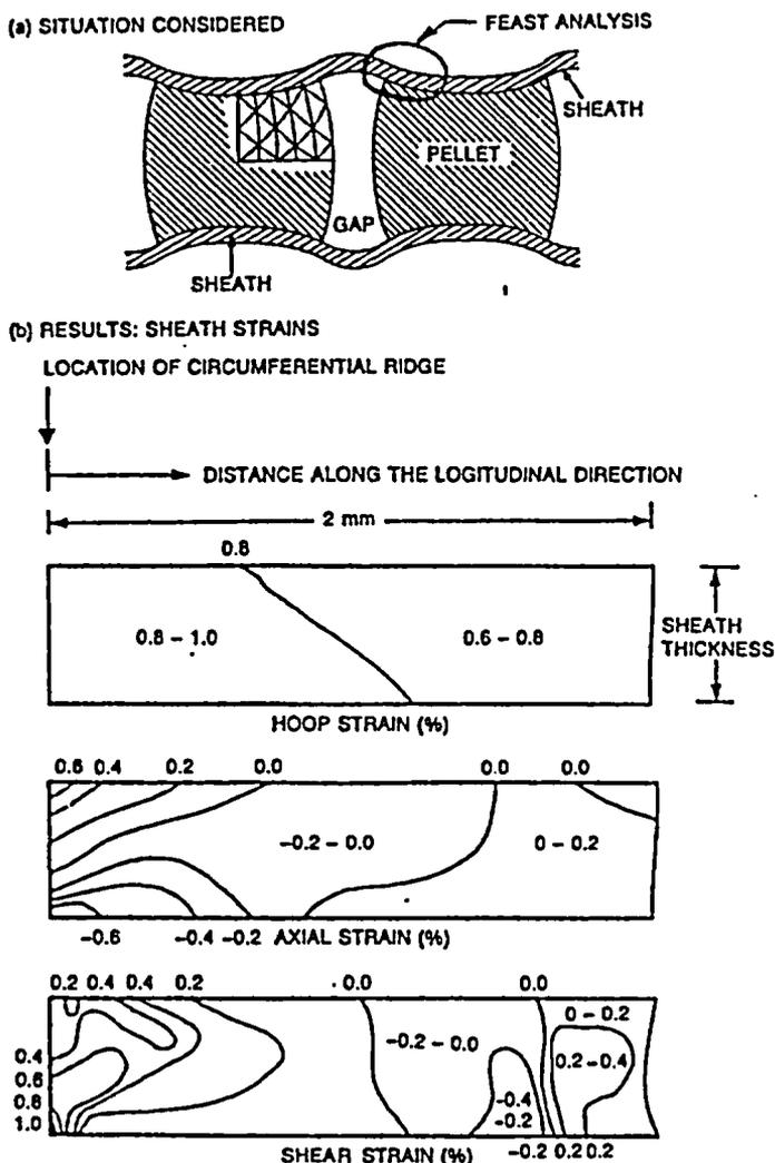
Figure 7 Multiaxial sheath strains near the circumferential ridge
