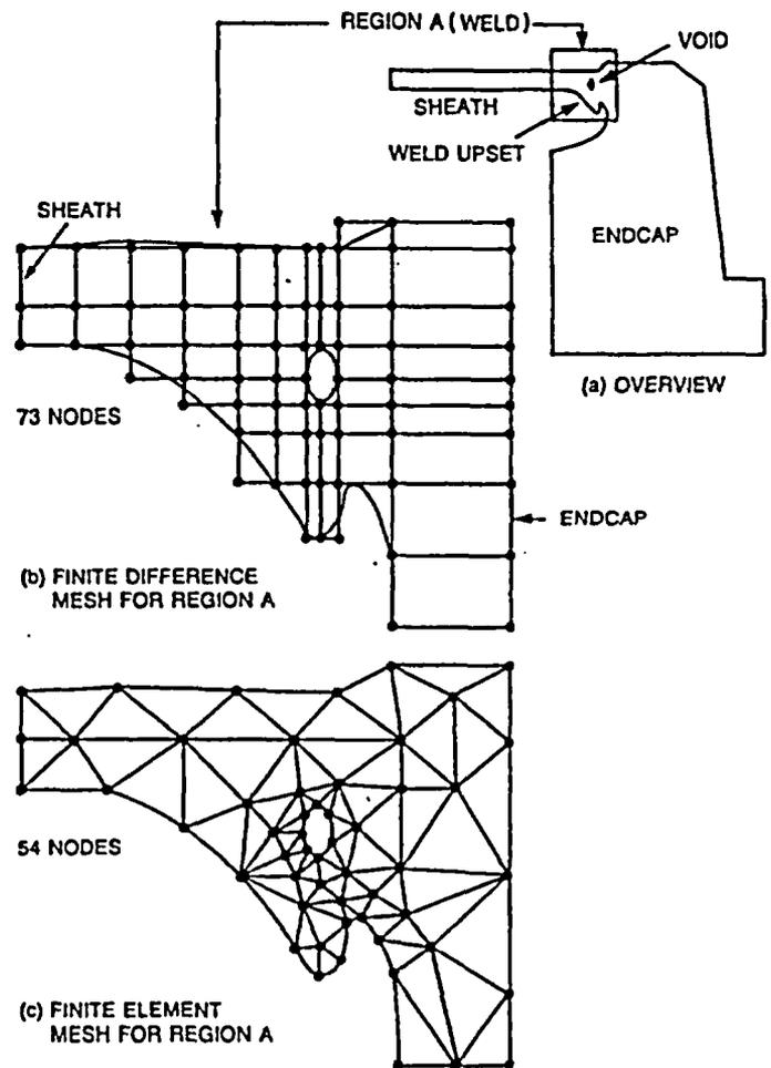
Figure 1 Finite difference and finite element idealizations of a hypothetical joint between the sheath and the endcap
