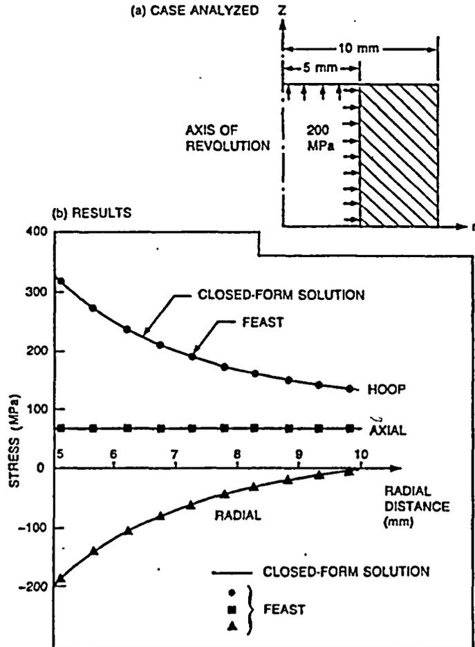
Figure 3 Creep stresses: FEAST vs closed-form solution
