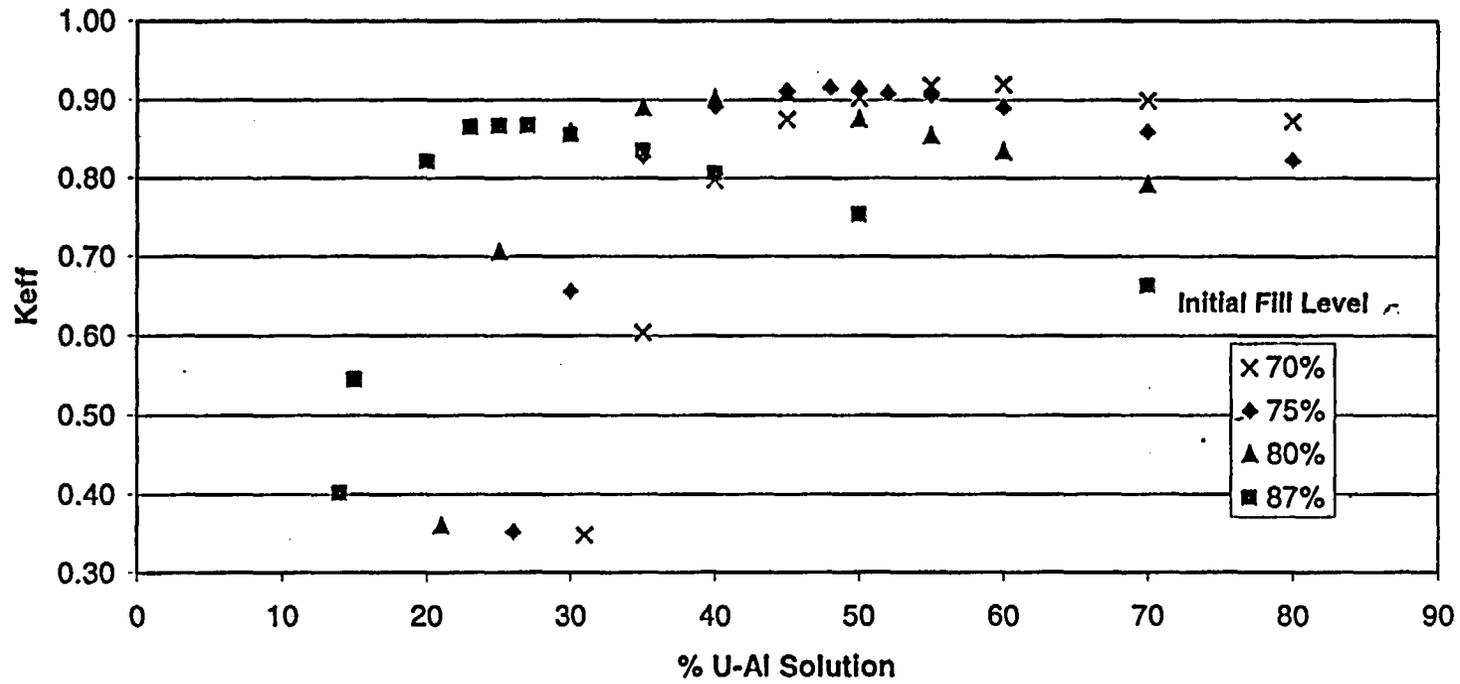
Figure 5.2.2b. Codisposal Canister Calculations – 15 % U-235
