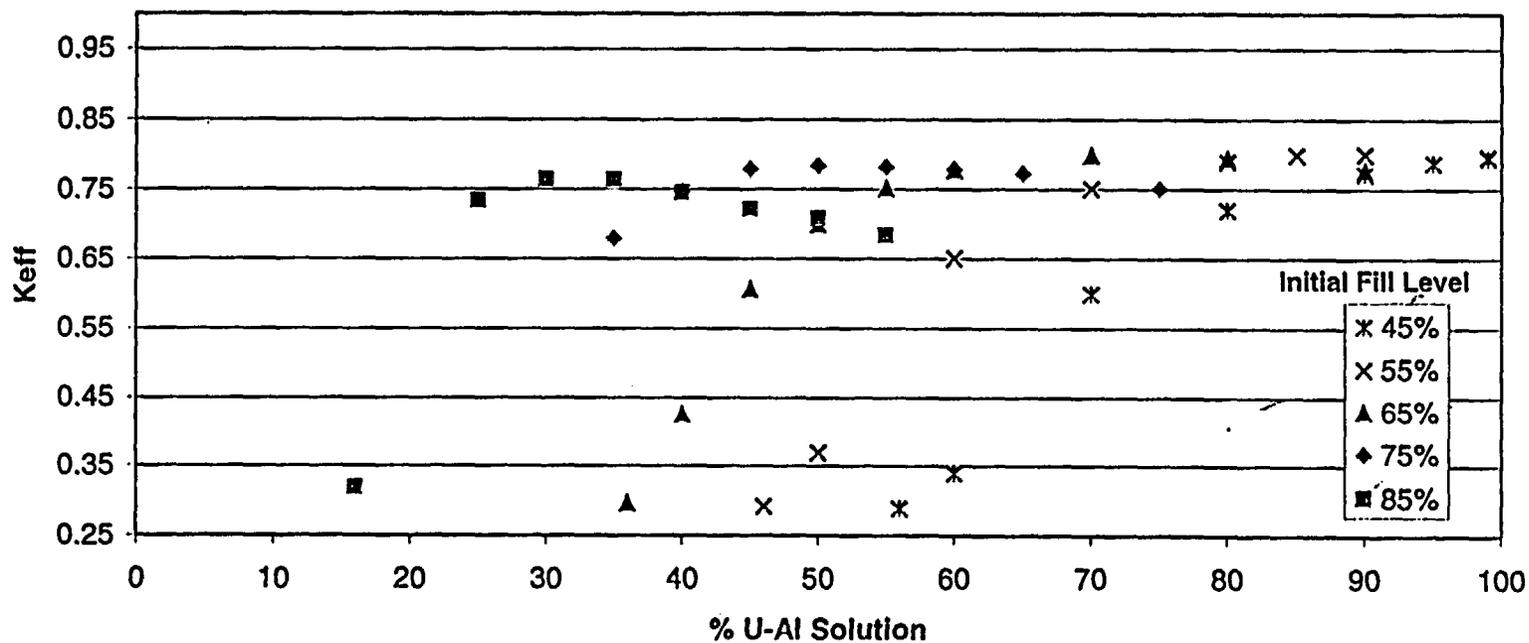
Table 5.2.2 summarizes the criticality calculations for the various configurations. The  $k_{eff}$  results in Table 5.2.2 have been adjusted by +0.018 (Code Bias) to account for code and cross section uncertainties (Section 4.2). The  $k_{eff} + 2*\sigma + \text{bias}$  values represents the bounding reactivity value for each configuration. These values should be used in the preliminary design process for the melt dilute option.
