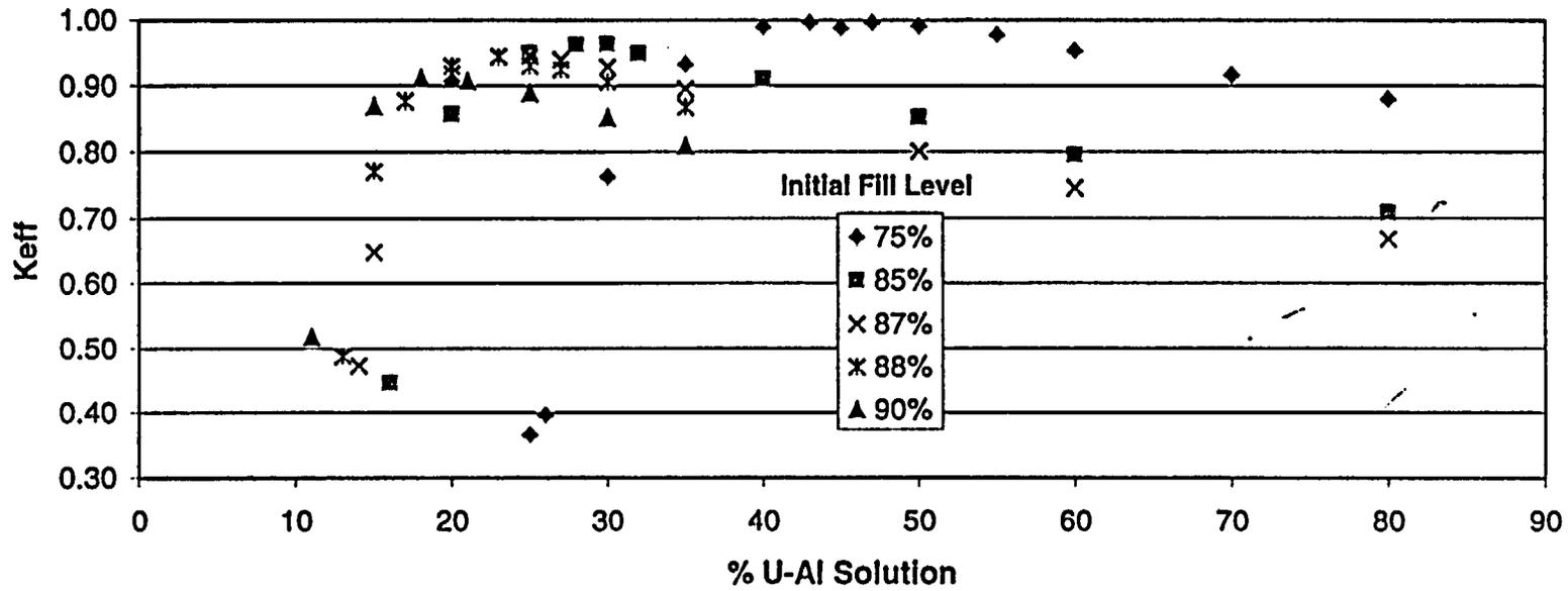
Figure 5.2.2a. Codisposal Canister Calculations – 15 % U-235
