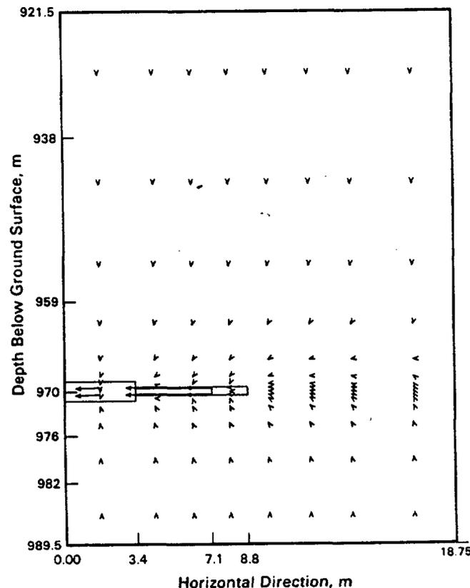
FIGURE 4. Velocity Vectors, 1.3 Years after Waste Package Emplacement
