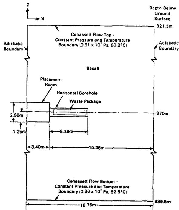
FIGURE 2. Detailed XZ Plane Dimensions of the Two-Dimensional Cartesian Model
