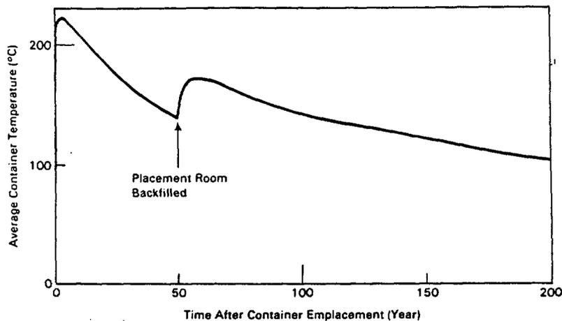
FIGURE 6. Container Temperature Versus Time
