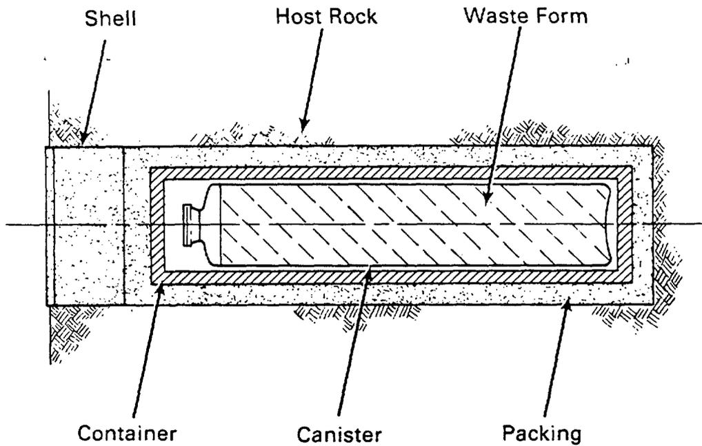
FIGURE 1. BWIP Waste Package Design
