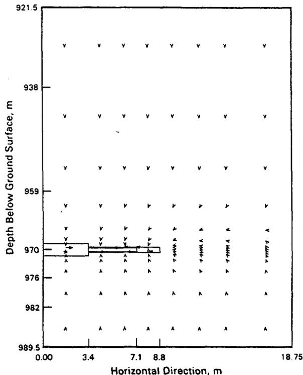
FIGURE 5. Velocity Vectors, 60 Years after Waste Package Emplacement
