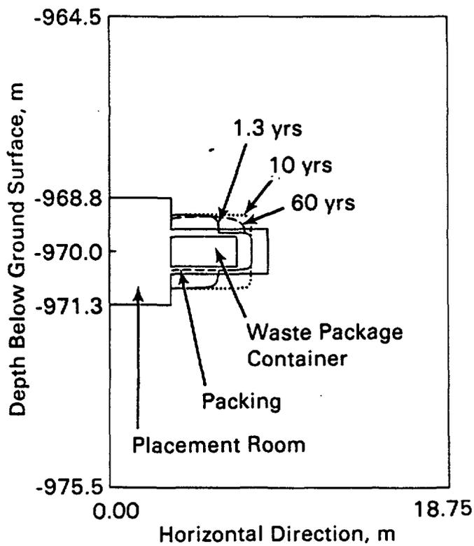
FIGURE 3. Contour of Groundwater Saturation
