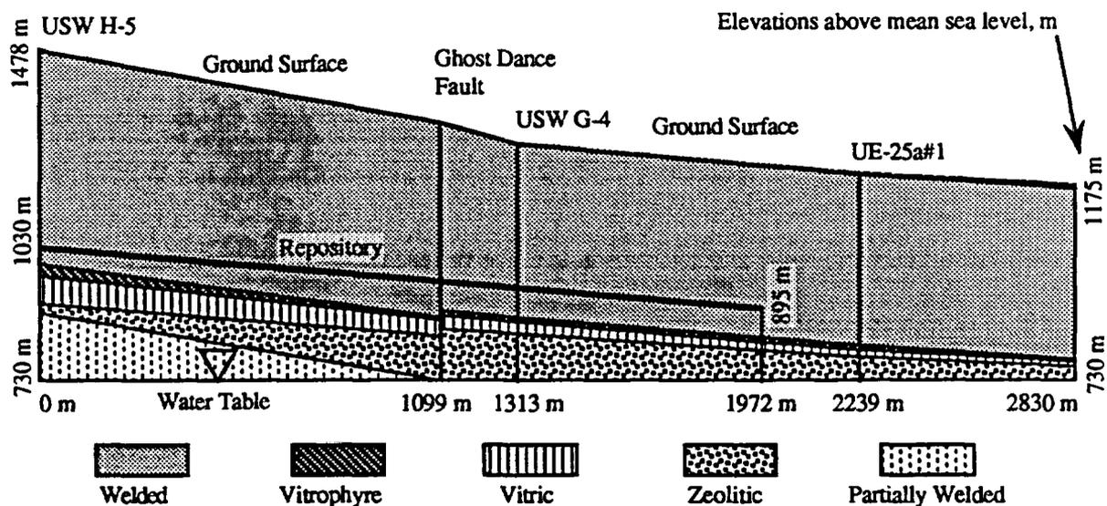
FIGURE 1. East-West Cross Section: Physical and Hydrogeologic System
