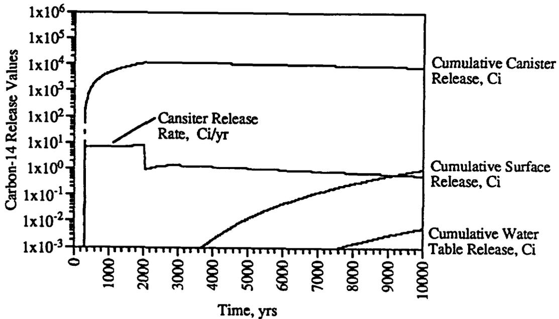
FIGURE 9. C<sup>14</sup> Release Histories, 0.01 mm/yr recharge case.
