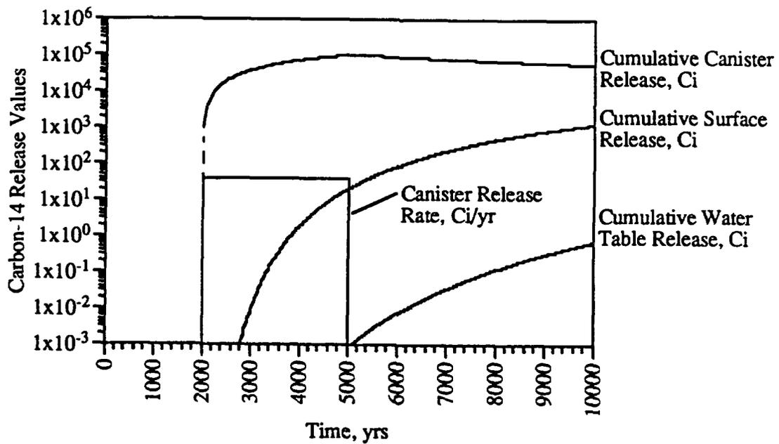
FIGURE 8. C<sup>14</sup> Release Histories, 0.0 mm/yr Recharge Case.
