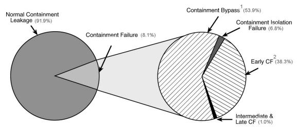
Total Core Damage Frequency = 2.4 E-7/y
