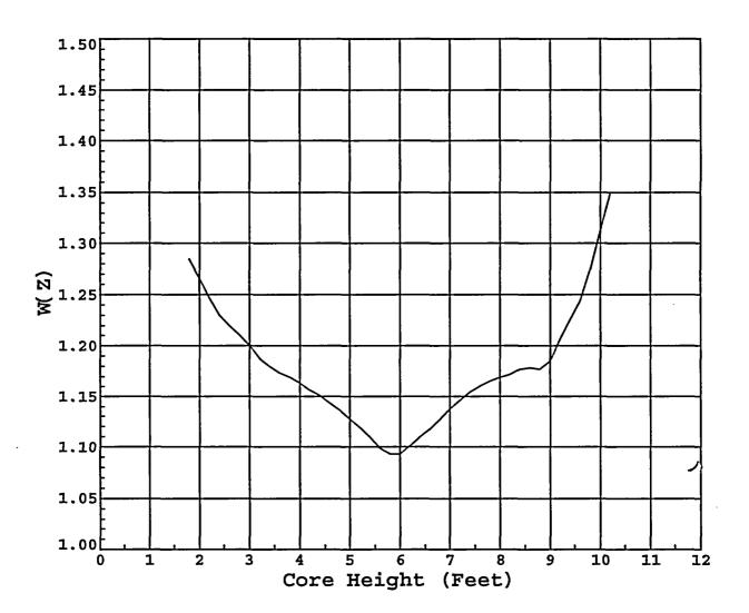
Figure 4.4 W(Z) Versus Core Height 10,000 MWD/MTU
