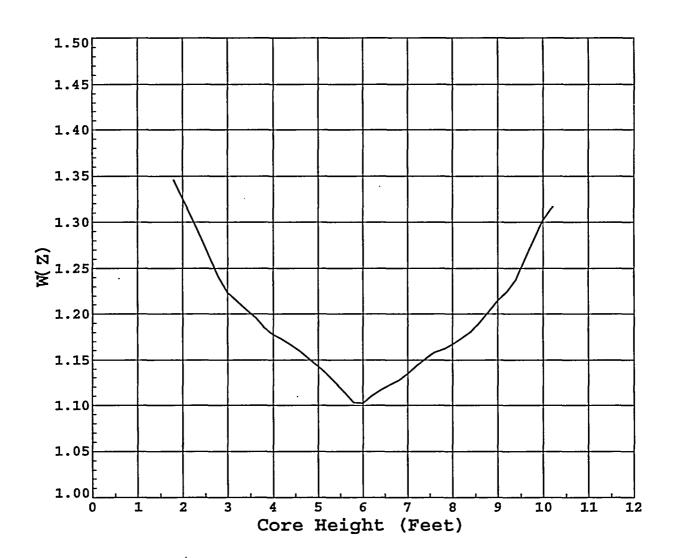
Figure 4.2 W(Z) Versus Core Height 2,000 MWD/MTU
