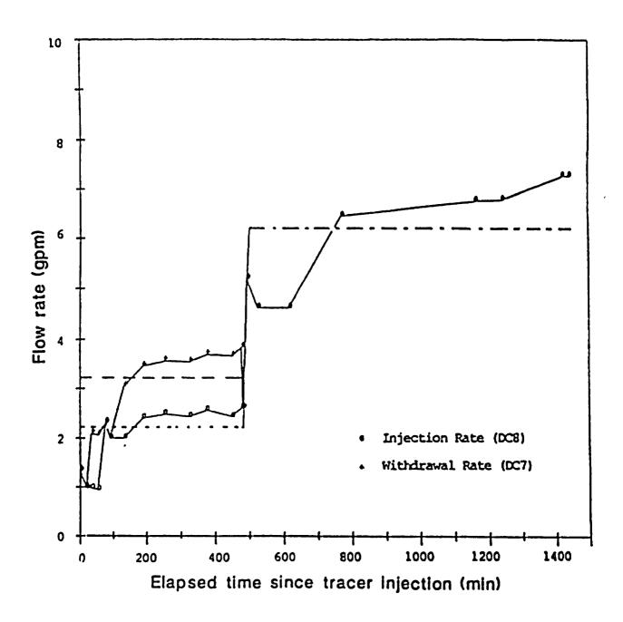
Figure 4.7. Plot of reported pumping and injection rates for Hanford Test 1, with averages assumed for initial numerical modeling.
