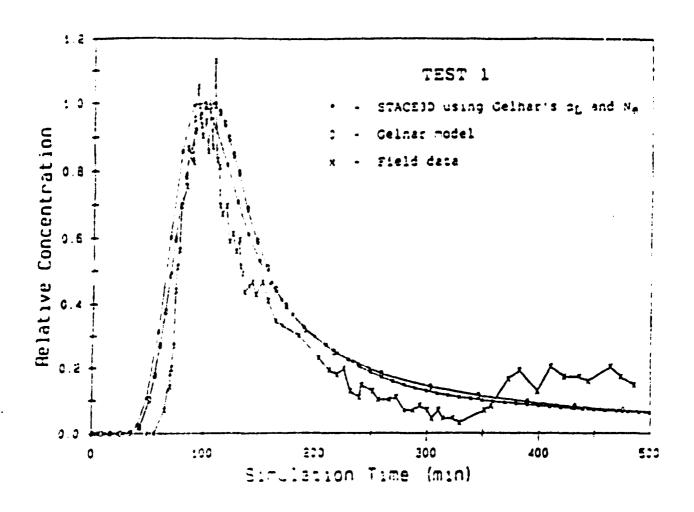
Figure 4.10. Comparison of STACE3D (without pipe-flow component) and Gelhar analytical model simulation with field data for Hanford Test 1, using values of  $\alpha_L$  and  $n_e$  reported by Gelhar (1982).
