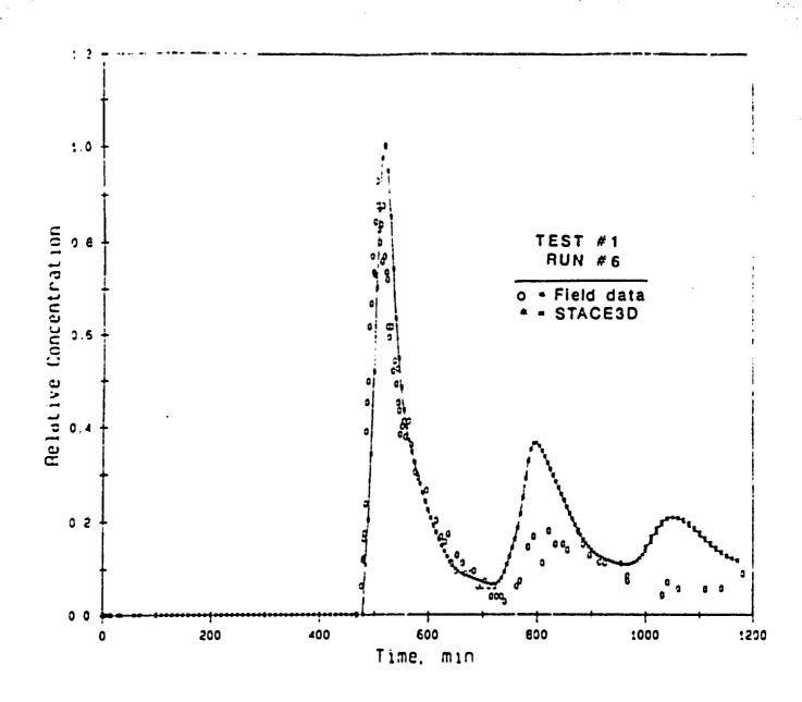
Figure 4.8. Comparison of best-fit simulation to field data using composite STACE3D model for Hanford Test 1.
