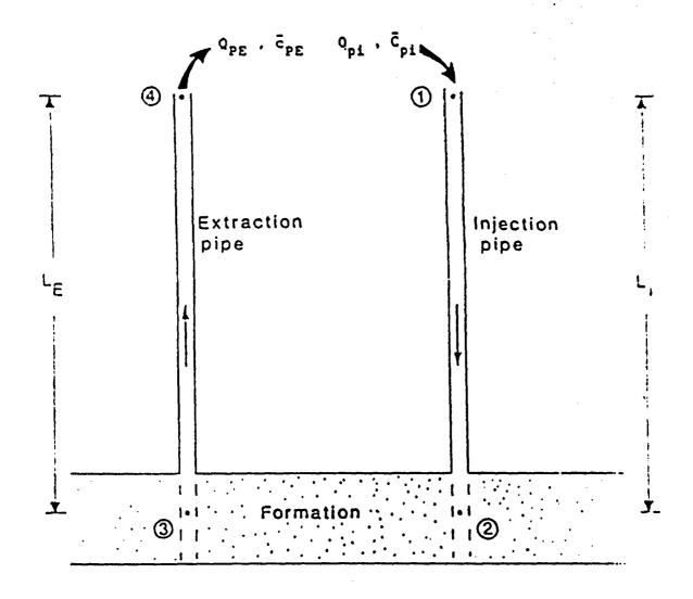
Figure 3.1. Schematic diagram illustrating three main components of STACE3D model for deep two-well tracer tests (injection pipe, extraction pipe, and geologic formation) and four component interfaces (labeled 1, 2, 3, and 4). L is pipe length, Q is flow rate, and c is average tracer concentration.
