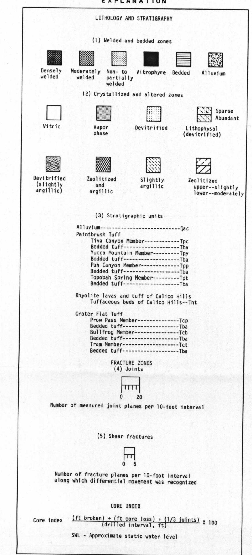
Graphic log showing lithologic, structural, and geophysical features of USW G-4
