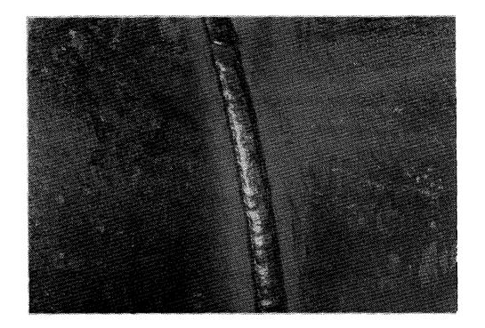
Figure 7. Illustration of Final or Cap Weld, Average External Protrusion of 1/16 In.
