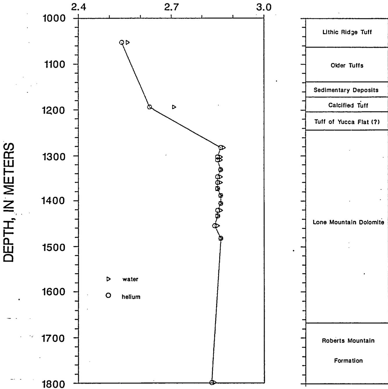
Figure 11. Plot of grain density values for the UE25p#1 borehole core samples using rock volumes determined by both helium and water displacement methods.
