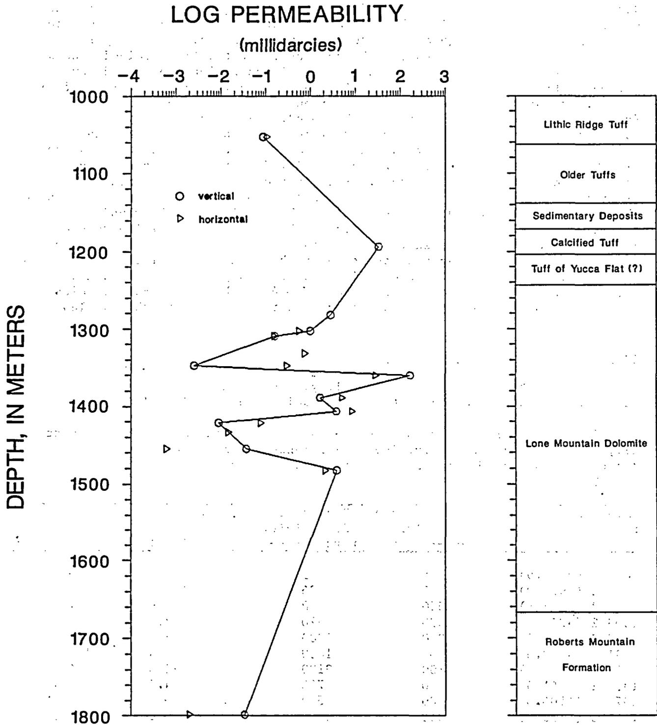
Figure 13. Plot of permeability values determined for vertical and horizontal flow directions on samples taken from the UE25p#1 borehole.
