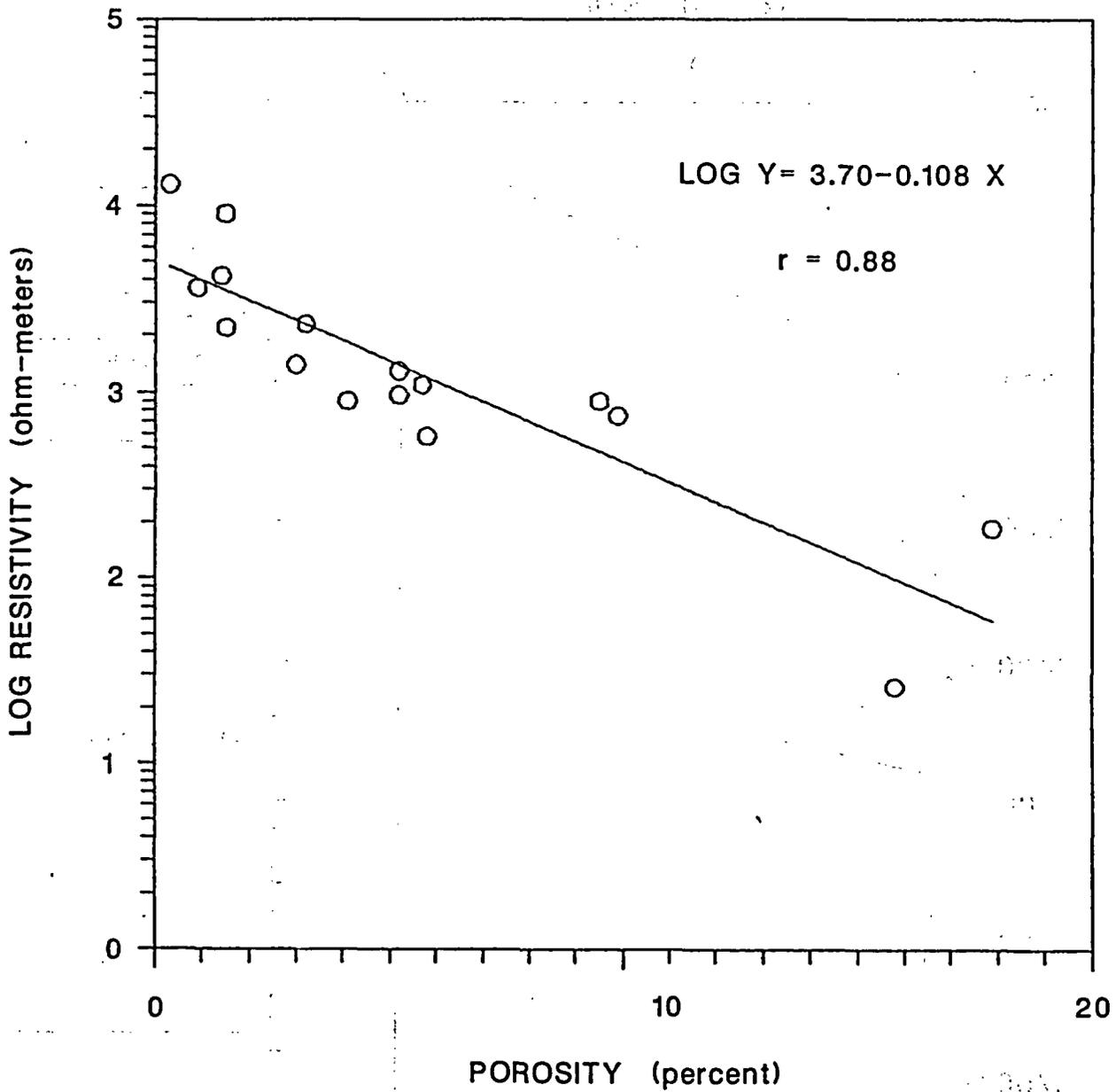
Figure 17. Correlation between resistivity and porosity data determined for the UE25p#1 borehole samples based on a least squares fit. The equation for the line of regression and the correlation coefficient,  $r$ , is indicated on the plot.
