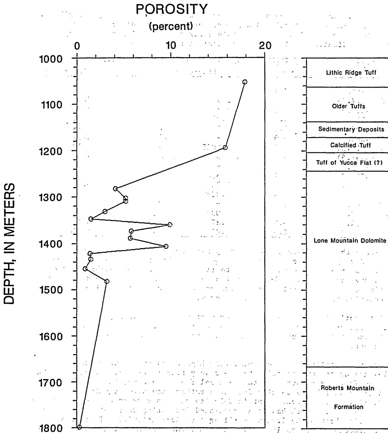
Figure 12. Plot of porosity values determined for the UE25p#1 borehole samples.
