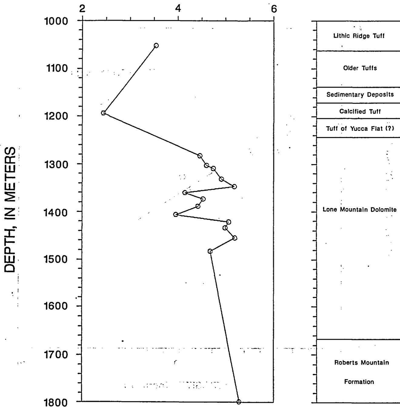
Figure 14. Plot of sonic velocity data obtained on core samples from the UE25p#1 borehole.
