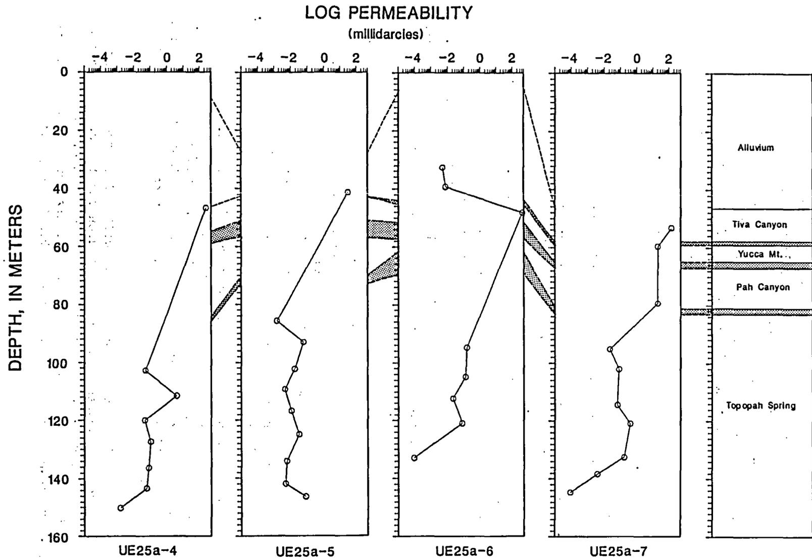
Figure 5. Plots of permeability or hydraulic conductivity values obtained on core samples from the Yucca Mountain UE25a-4, -5, -6, and -7 boreholes.
