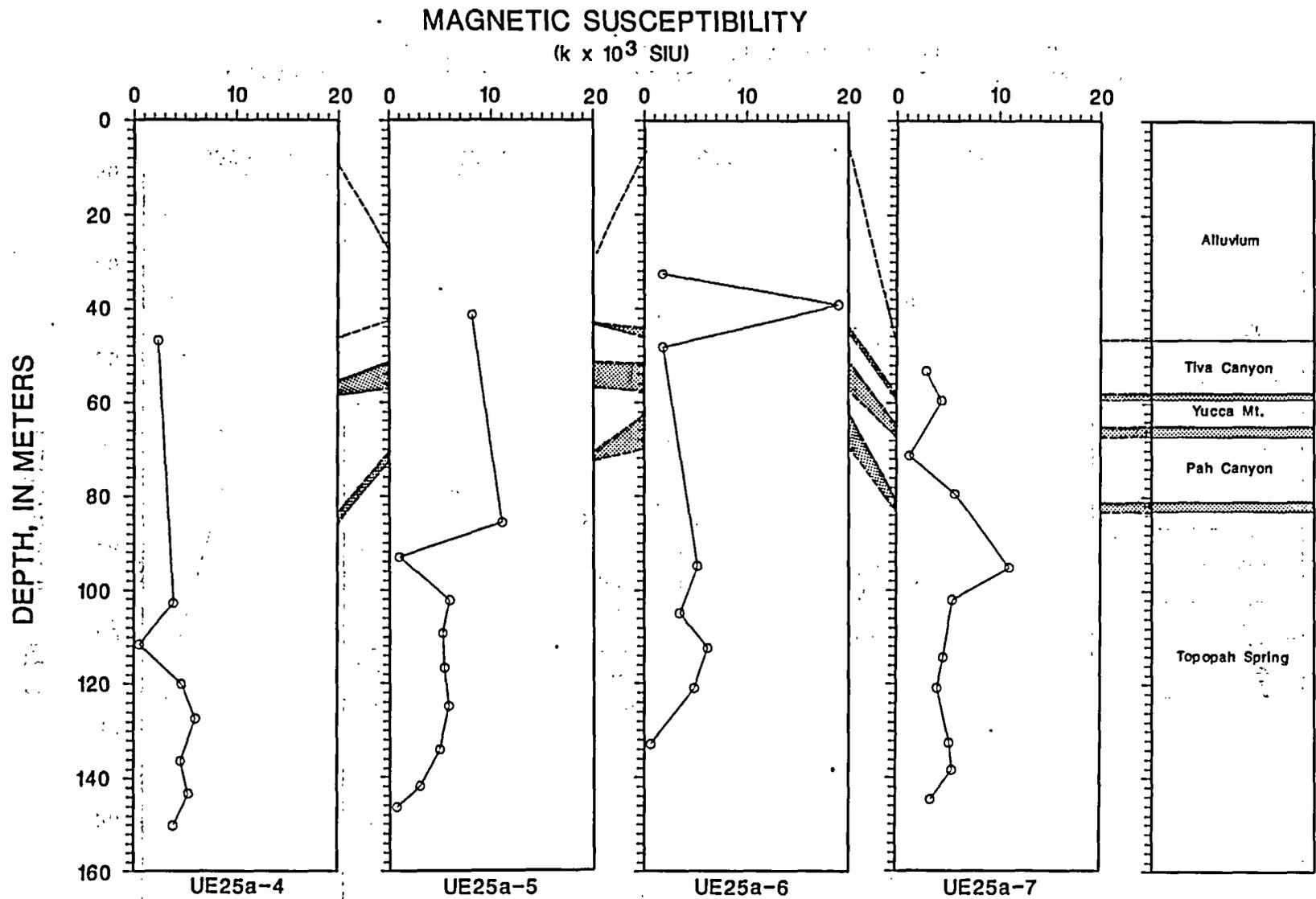
Figure 8. Plots of magnetic susceptibility values obtained on core samples taken from the Yucca Mt. UE25a-4, -5, -6, and -7 boreholes.
