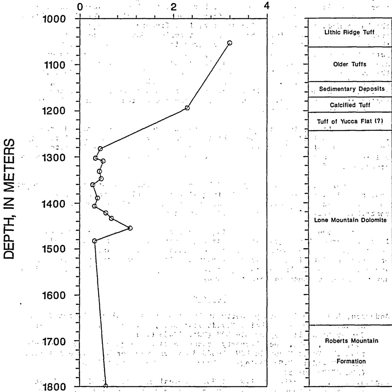
Figure 19. Plot of remanent magnetization values measured on core samples from the UE25p#1 borehole.
