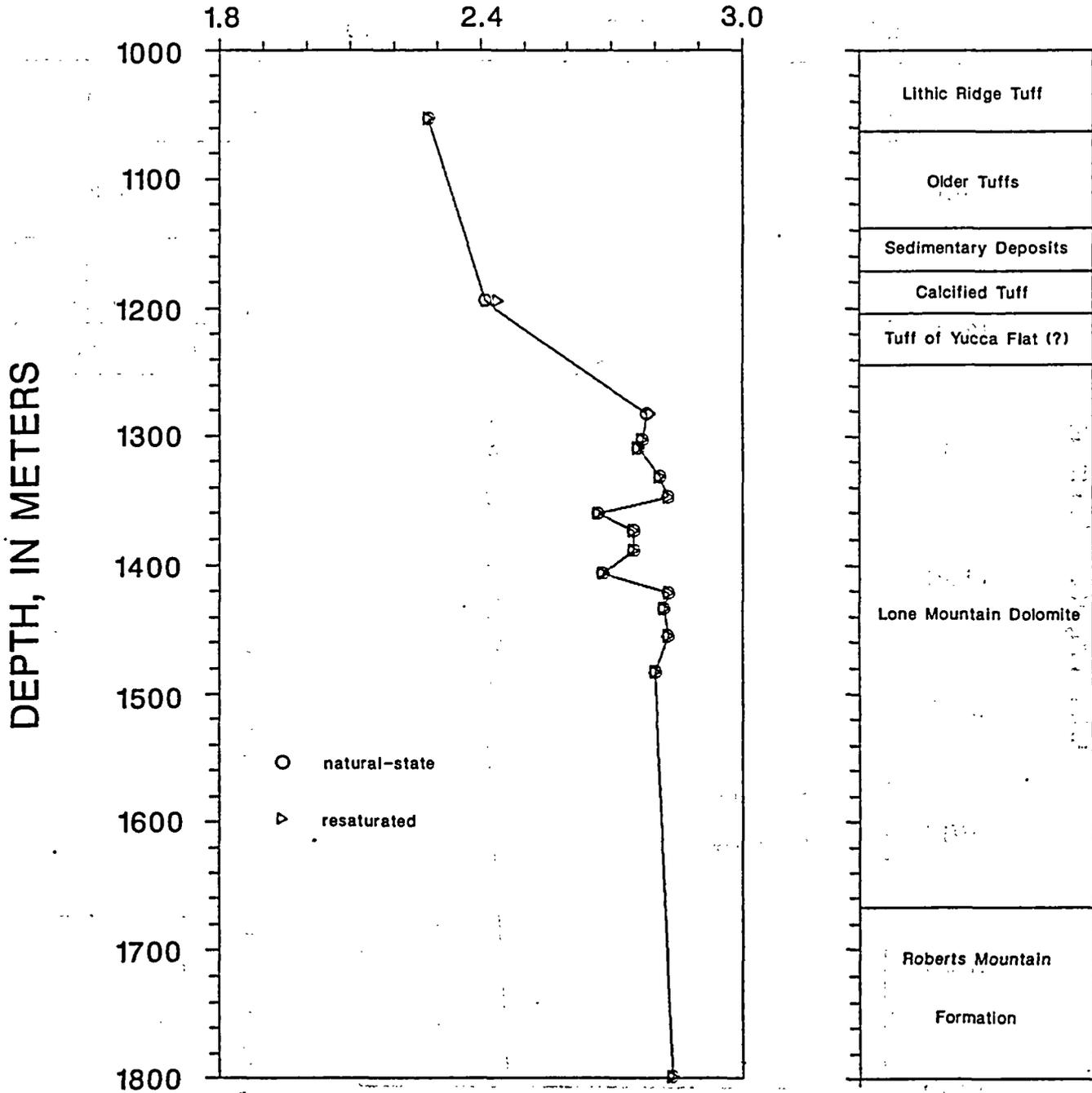
Figure 10. Plot of bulk density values determined for core samples from the UE25p#1 borehole. Circles designate in place levels of pore water within the rock and the triangles indicate values obtained following resaturation with local tap water. The stratigraphic section as presented by Carr and Others, 1986, is shown on the right-hand side of the figure.
