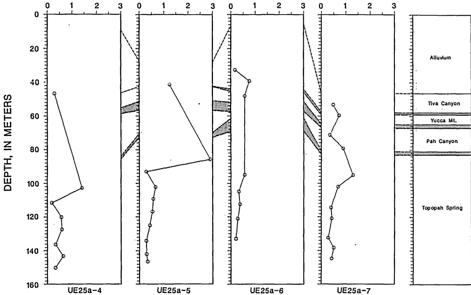
Figure 9. Plots of remanent magnetization values obtained on core samples taken from the Yucca Mt. UE25a-4, -5, -6, and -7 boreholes.
