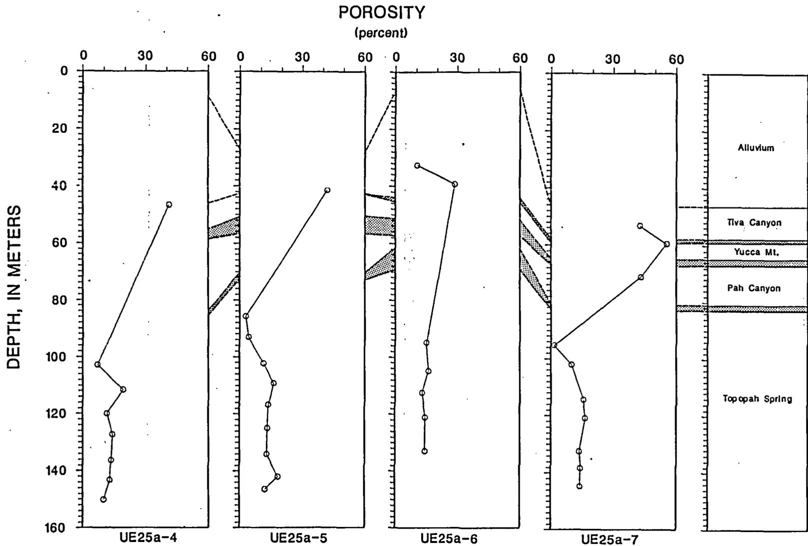
Figure 4. Porosity plots of sample data obtained on core from the Yucca Mt. UE25a-4, -5, -6, and -7 boreholes.
