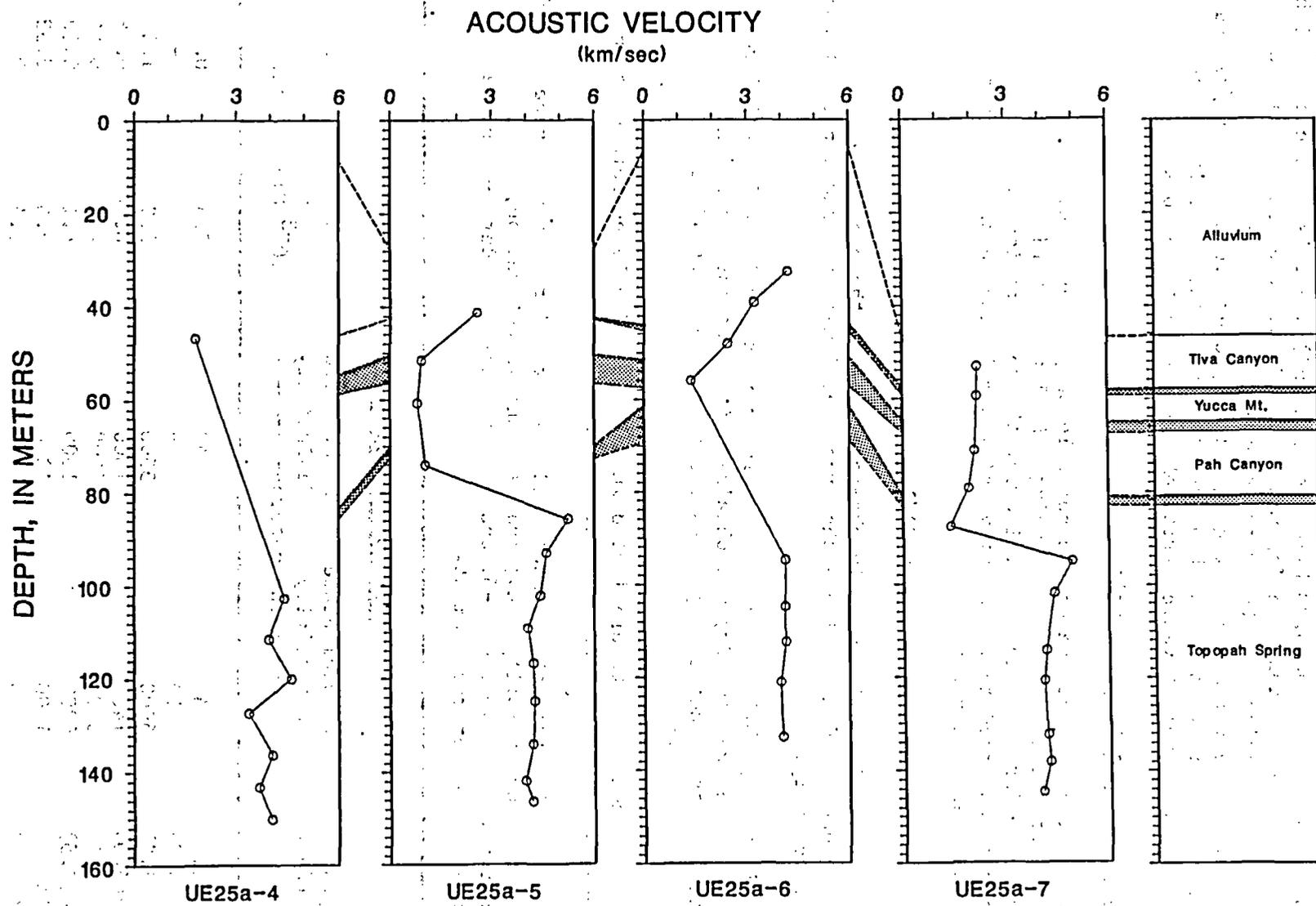
Figure 6. Acoustic velocity plots of sample data obtained on core from the Yucca Mt. UE25a-4, -5, -6, and -7 boreholes.
