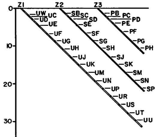
Figure 4: Core sample locations in inclined boreholes at the Apache Leap Tuff Site.
