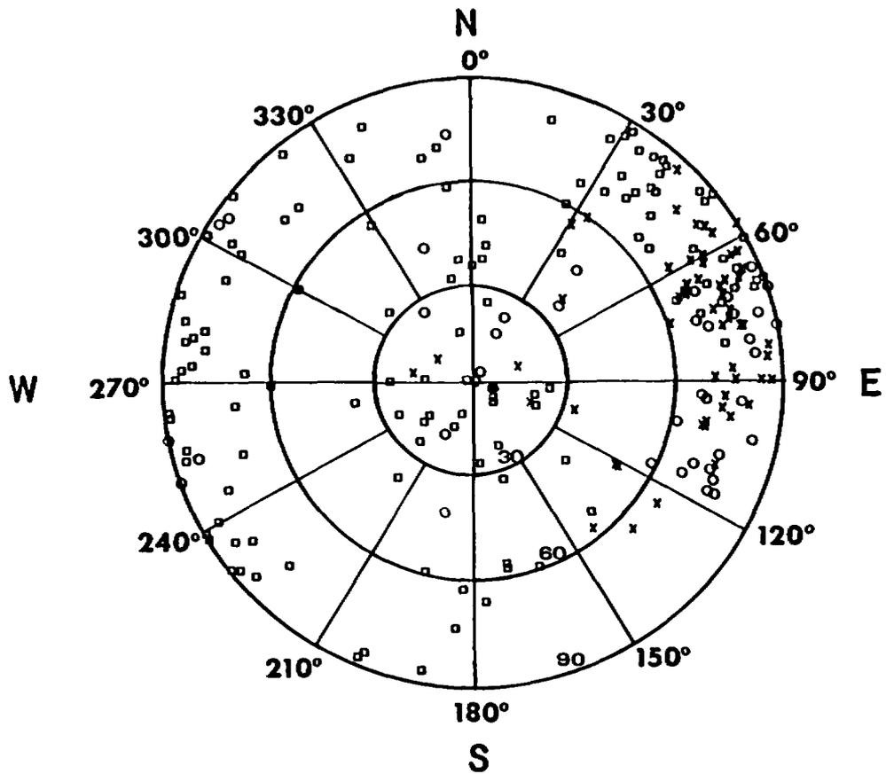
Figure 8: Lower stereonet projection of fracture orientations observed at Apache Leap Tuff Site, from X-series boreholes (crosses), Y-series boreholes (circles) and Z-series boreholes (squares).
