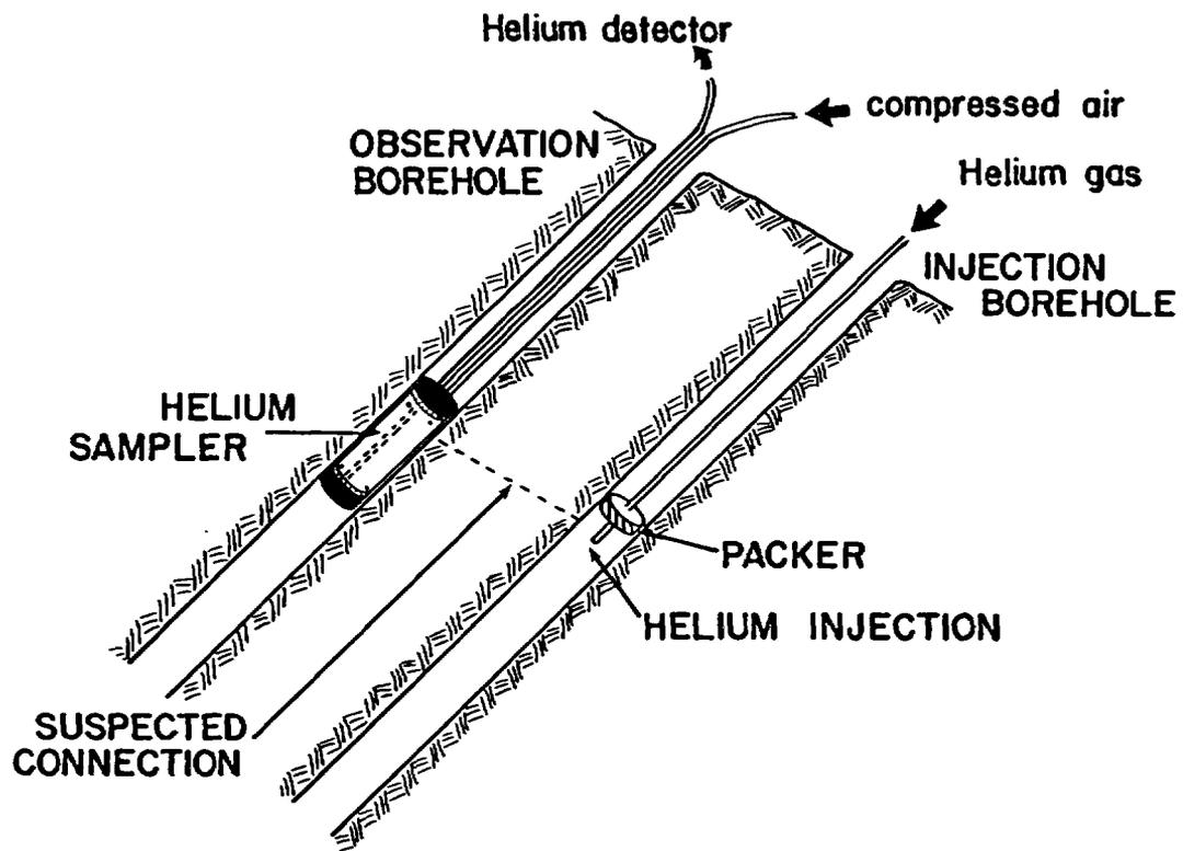
Figure 9: Cross-borehole helium tracer detection setup used at the Apache Leap Tuff Site.
