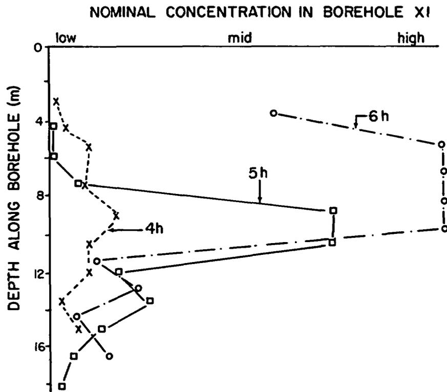
Figure 10: Cross-borehole helium tracer test data obtained from Apache Leap Tuff Site.
