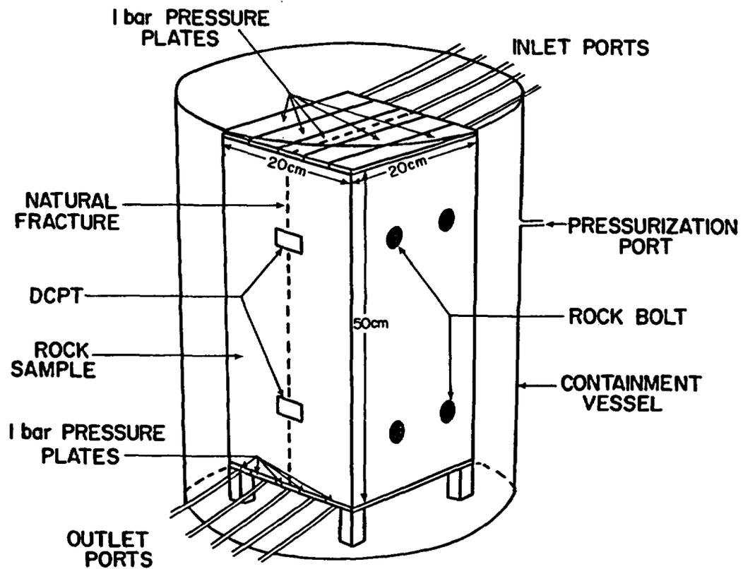
Figure 11: Experimental setup for unsaturated fracture-matrix flow studies.
