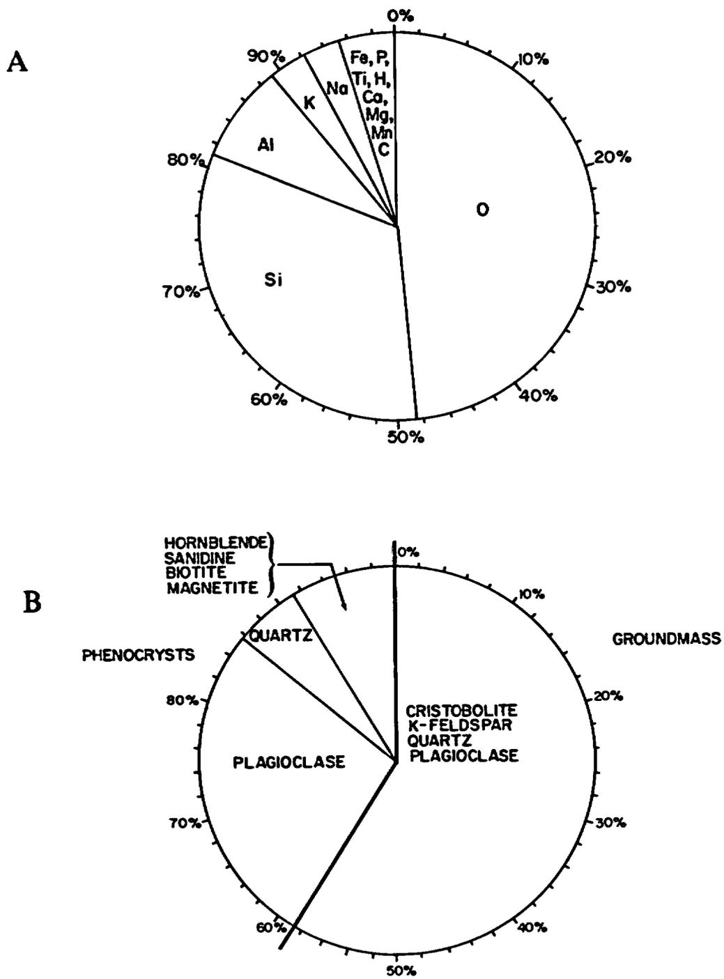
Figure 2: Whole rock elemental composition (A) and mineralogical composition of tuff groundmass and phenocrysts (B) at the Apache Leap Tuff Site.
