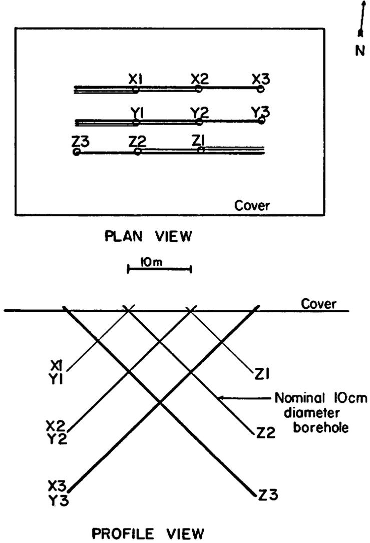
Figure 1: Borehole configuration at the Apache Leap Tuff Site showing inclined boreholes and 30 x 50 m plastic cover.
