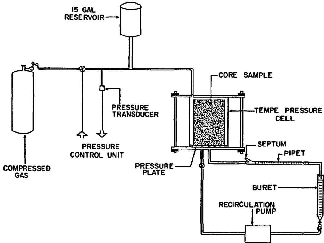
Figure 6: Outflow method experimental setup for determining unsaturated hydraulic conductivity and characteristic curves for rock core samples obtained from the Apache Leap Tuff Site.
