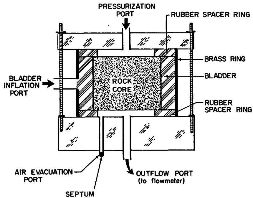
Figure 5: Permeameter used to obtain saturated hydraulic conductivity and unsaturated pneumatic permeabilities for rock core samples obtained from the Apache Leap Tuff Site.
