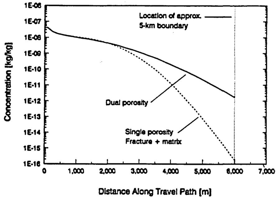
**Figure 4.** Contaminant concentration profiles along the transport pathway at approximately 5500 years. Curves depict single-porosity, fracture-plus-matrix transport and dual-porosity transport.
