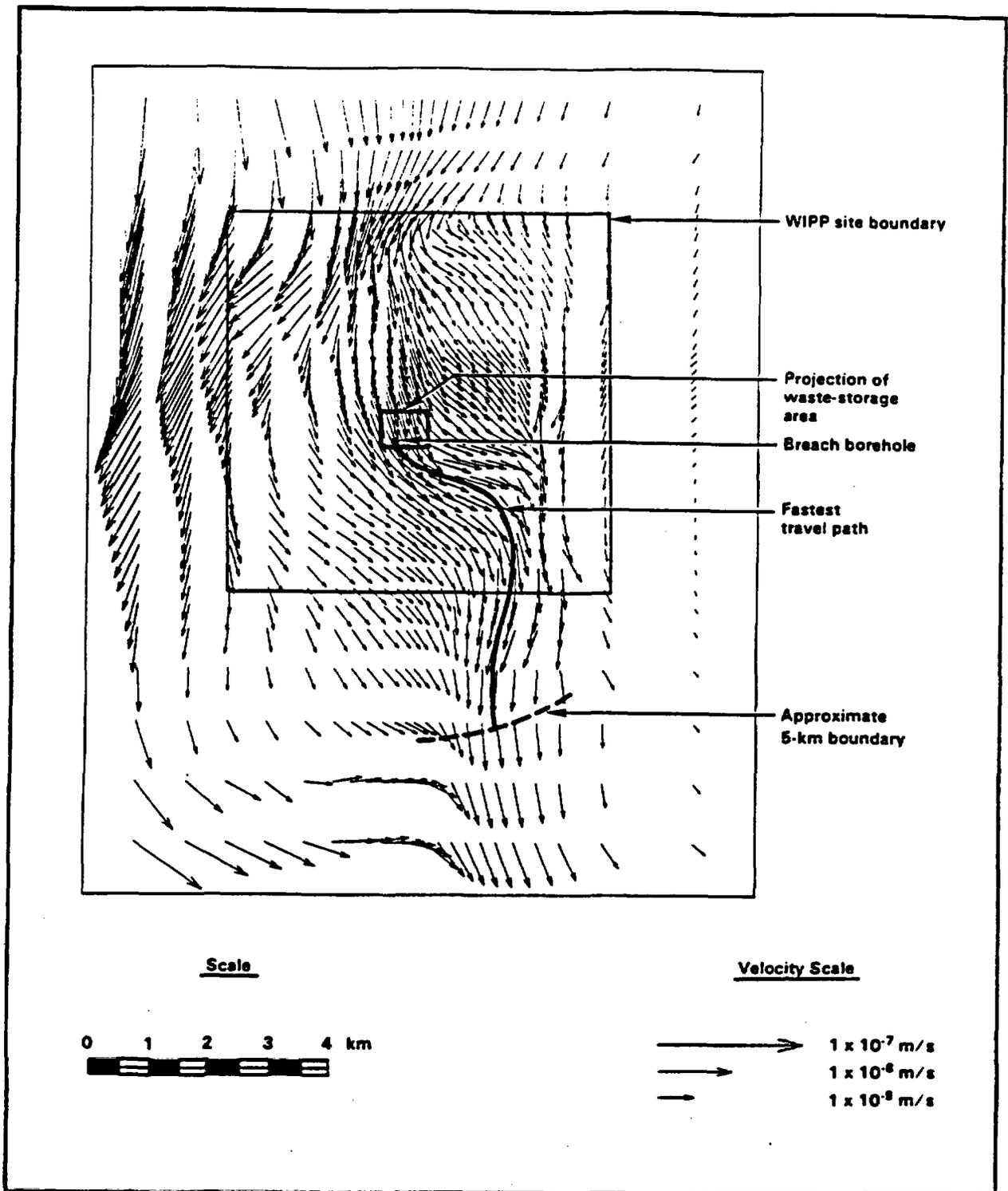
**Figure 2.** Simulated flow field (Darcy velocities) for the Culebra dolomite under undisturbed conditions [7]. Fastest transport pathway from a breach borehole to the approximate 5-kilometer boundary is also shown.
