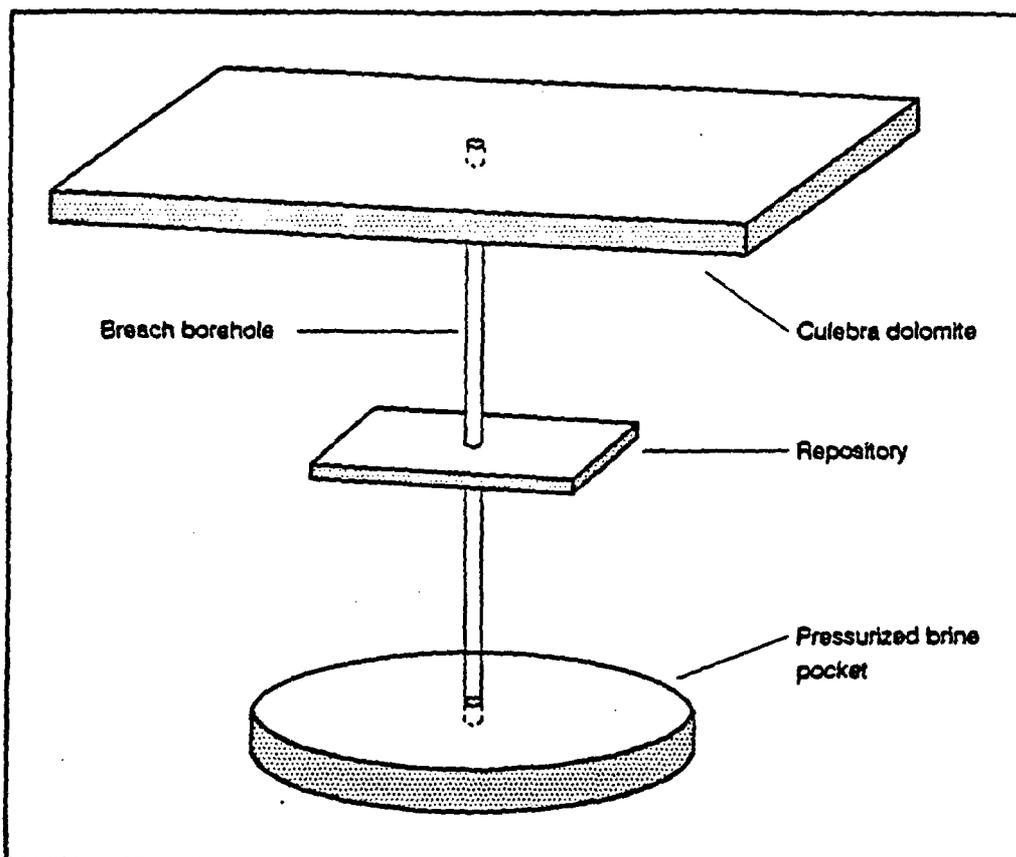
**Figure 1.** Schematic diagram of flow system considered for breach simulation. This system consists of a borehole penetrating both the repository and an underlying pressurized brine pocket, with contaminant release and offsite transport in the Culebra dolomite.
