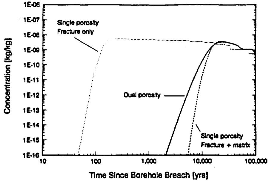
**Figure 3.** Contaminant concentration versus time at the 5-kilometer boundary for a conservative, nonretarded solute. Curves depict single-porosity, fracture-only transport; single-porosity, fracture-plus-matrix transport; and dual-porosity transport.
