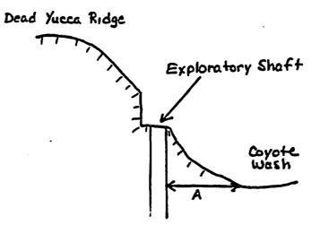
The potential for erosion along line A at this location is highly probable in the future as the area continues to erode. Careful remedial actions should be used in these areas. Appropriate construction should be more than adequate to prevent or at least minimize the potential lateral erosion.
