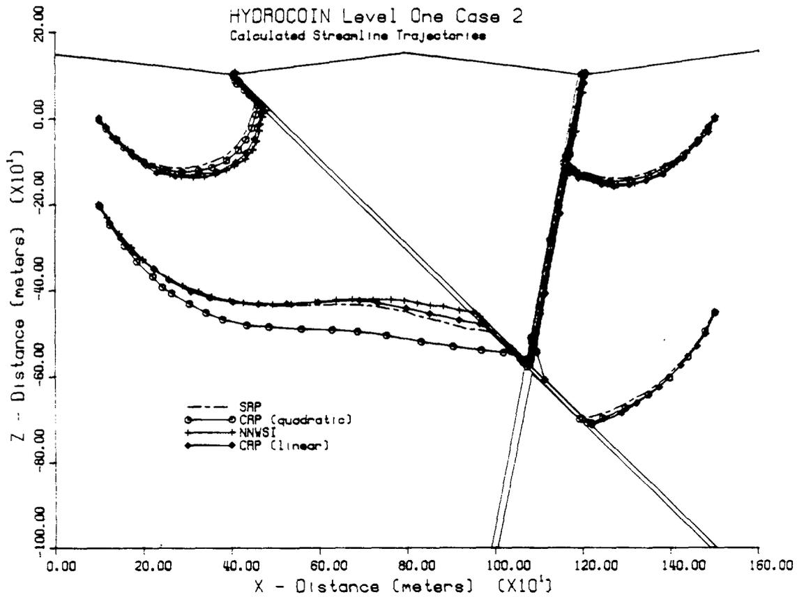
FIGURE 9. Comparison of Streamline Trajectories for the Finest Grids Calculated by CRP (using two different interpolation schemes), NNWSI, and SRP
