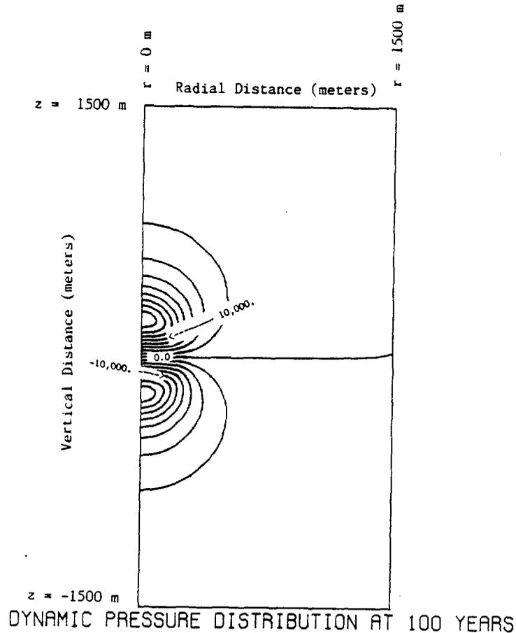
**FIGURE 15.** Contour Map of Dynamic Pressure Results for Case 4 at a Time of 100 Years With Dynamic Pressure Contour Spacing of 2000 Pascals. This figure taken from SRP results presented at the fourth HYDROCOIN workshop.
