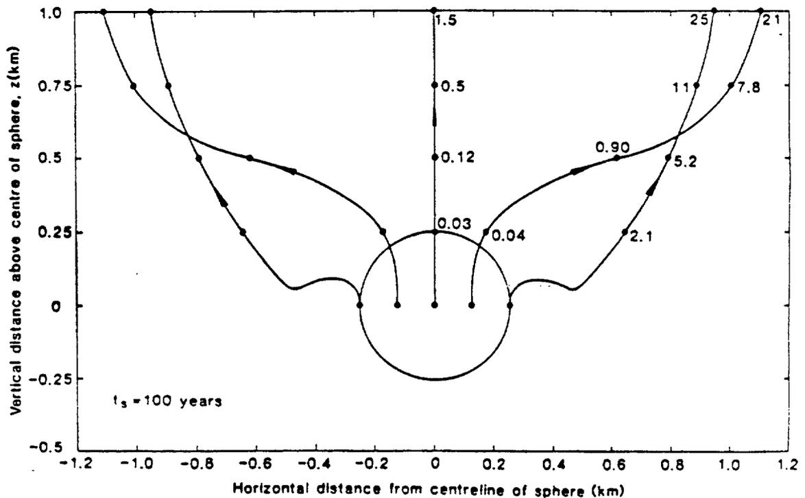
Fig. 4 Representation of the spherical heat source. Shown are also some pathlines starting after 100 years. The numbers represent approximate travel times in thousands of years.
