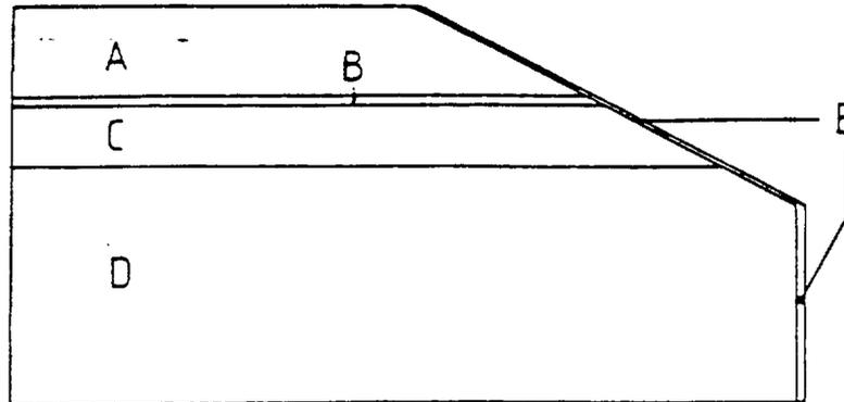
Fig. 3 The geometry assumed for Case 3. The media A and C represent pervious formations whereas media B and D are regarded as relatively impervious. Medium E is used to simulate the seepage face.
