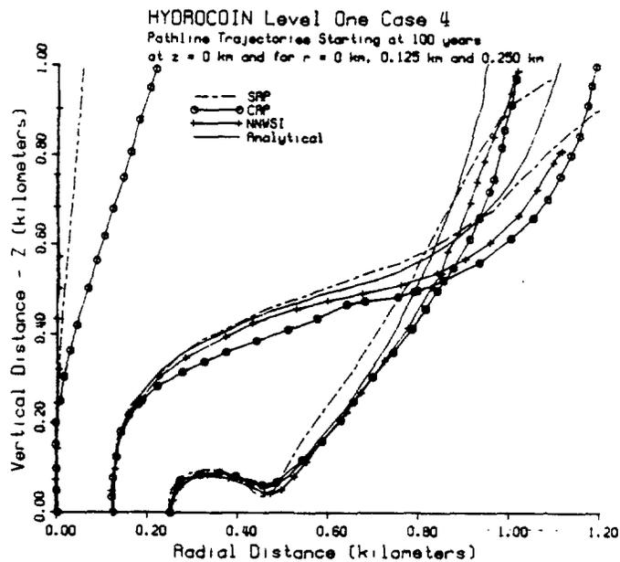
FIGURE 22. CRP, NNWSI, and SRP Calculated Pathline Trajectories and the Analytical Solution for Three Pathlines Initiated at a Time of 100 Years from Locations  $r = 0$  m and for  $z = 0, 125, \text{ and } 250$  m
