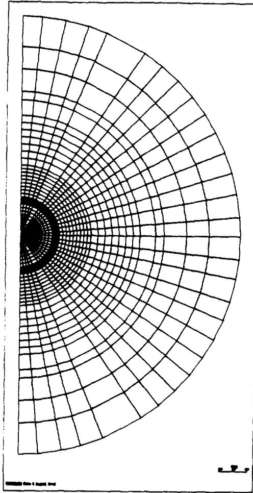
FIGURE 13. The Radial (r-z) Grid Utilized by SRP for Case 4. This figure was taken from their presentation at the fourth HYDROCOIN workshop.
