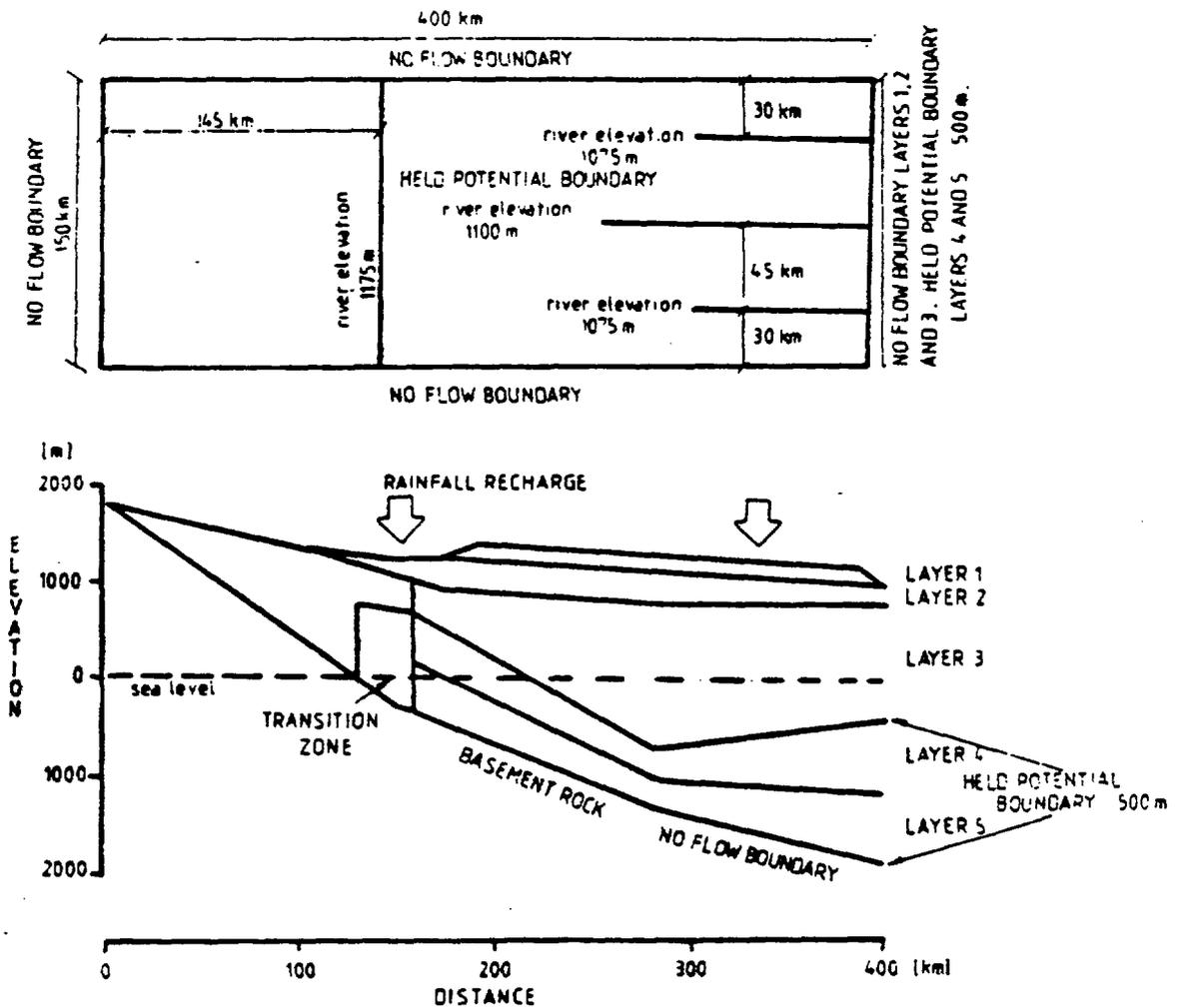
Fig. 6 Horizontal (top) and vertical (bottom) view of the modelled domain for Case 6.
