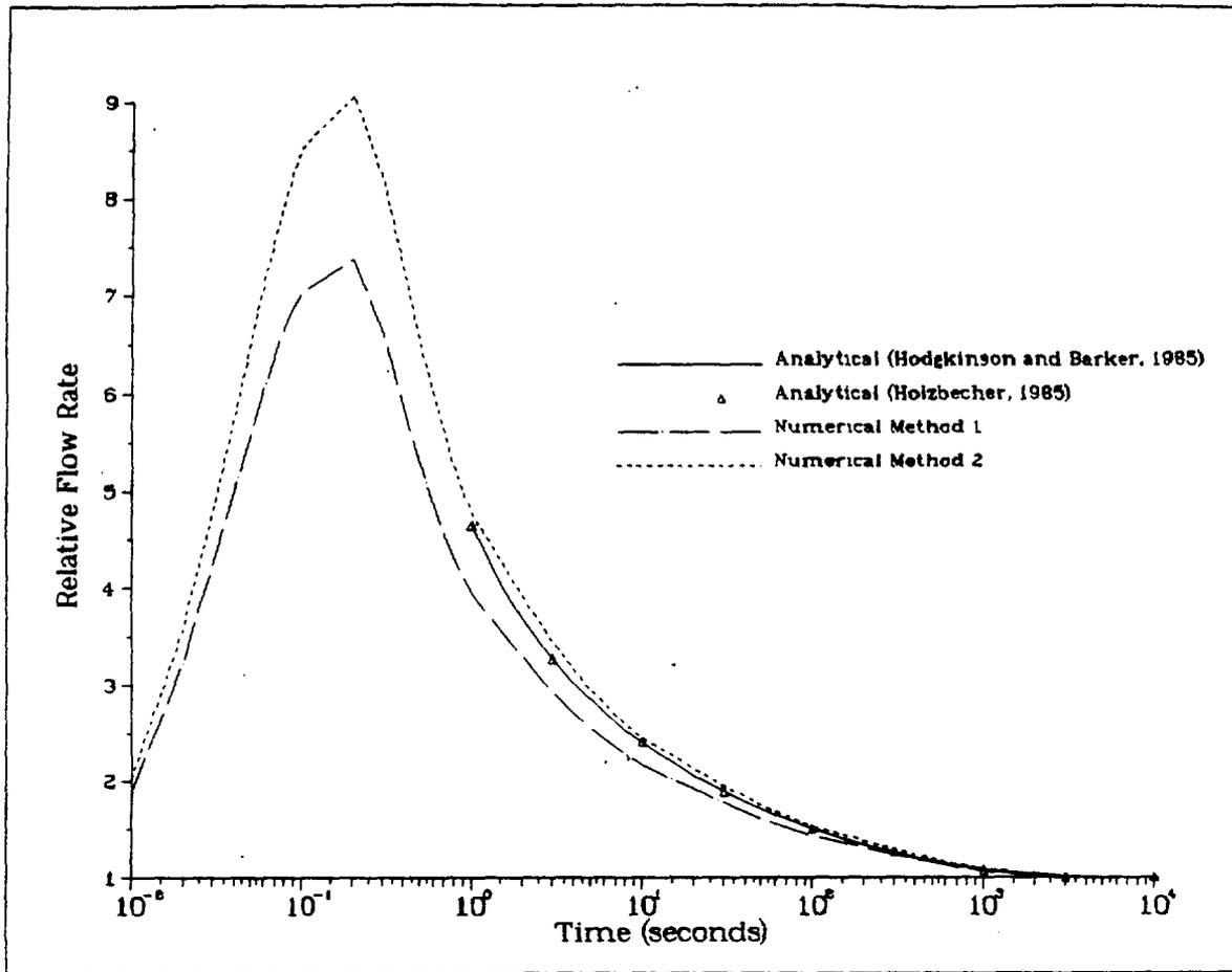
**FIGURE 4.** CRP Results for Time-Dependent Relative Flow Rate from the Borehole into the Rock Matrix as a Function of Time. This graph was taken from a CRP presentation at the third HYDROCOIN workshop. Results for two different numerical methods and two different analytical solution methods are shown.
