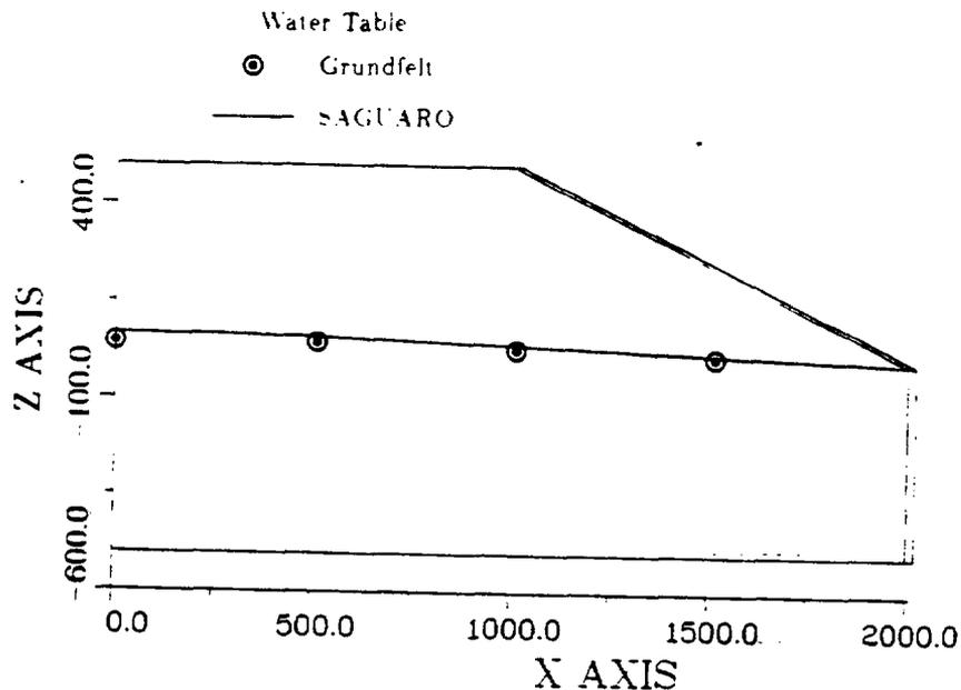
FIGURE 12. A Comparison of NNWSI Calculated Steady-State Water Table Location With Results Presented by Grundfelt (1984). This figure was taken from the January 10, 1986, NNWSI status report submitted to the HYDROCOIN secretariat.
