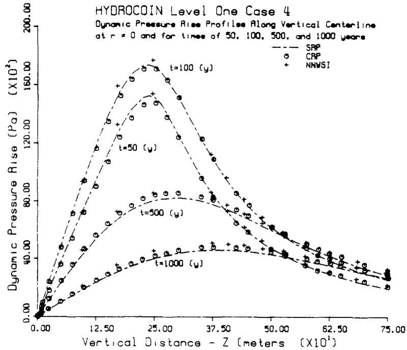
FIGURE 19. Closer Comparison Between CRP, NNWSI, and SRP Calculations for Dynamic Pressure Versus Vertical Distance at a Radius of 0 m and at Times of 50, 100, 500, and 1000 Years
