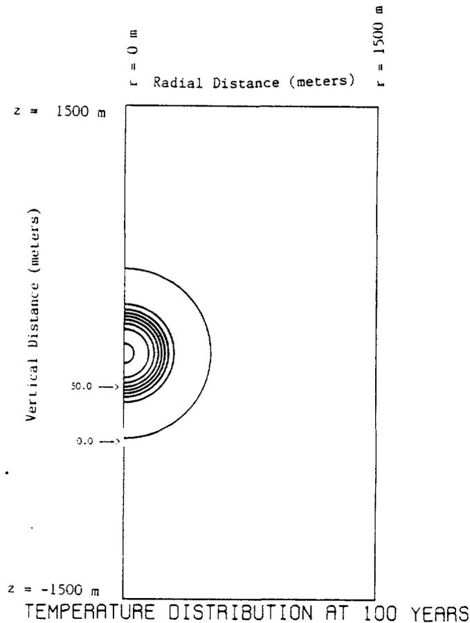
FIGURE 14. Contour Maps of SRP Temperature Results for Case 4 at a Time of 100 Years With Equally Spaced Temperature Contours of 10°C. This figure was taken from SRP results presented at the fourth HYDROCOIN workshop.
