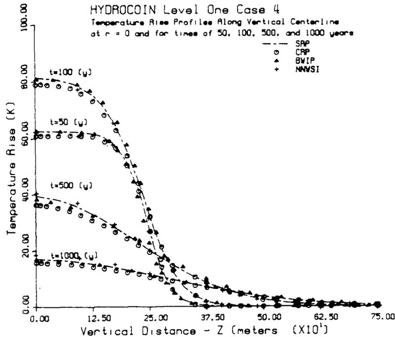
FIGURE 15. Comparison Between BWIP, CRP, NNWSI, and SRP Calculations for Temperature Versus Vertical Distance at a Radius of 0 m and at Times of 50, 100, 500, and 1000 Years
