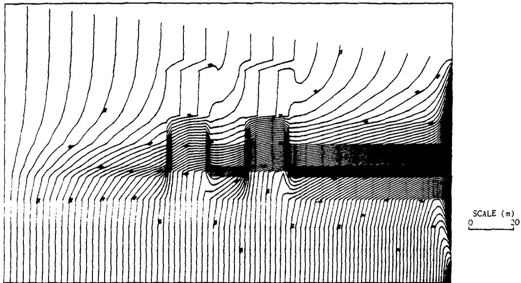
FIGURE 29. Contour Map of Calculated Potentials for the Low-Permeability Concrete Variation. The contour interval is 0.25 m. This figure was taken from SRP results presented at the second HYDROCOIN workshop.
