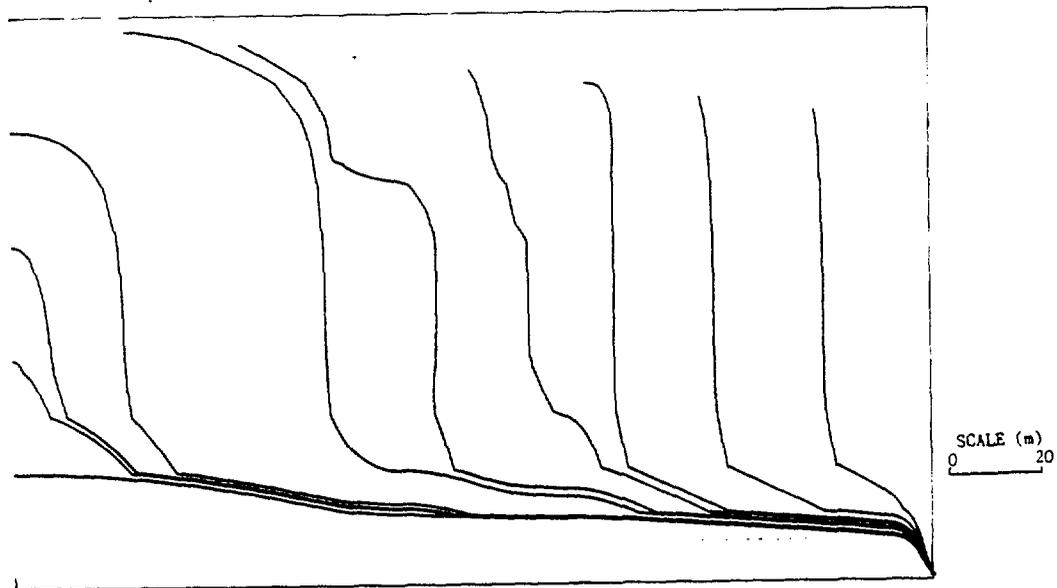
FIGURE 30. Calculated Streamline Trajectories for the Twelve Streamlines Specified in the Case 7 Problem Definition. This figure was taken from SRP results presented at the second HYDROCOIN workshop.
