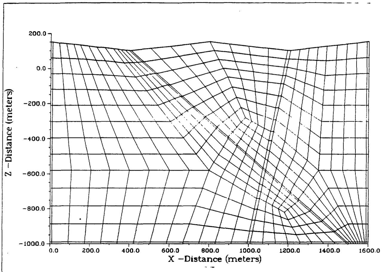
FIGURE 10. CRP's Finest Finite Element Grid, Illustrating the Use of Narrow Elements for Boundary Condition Implementation. This plot was taken from the CRP presentation at the third HYDROCOIN workshop.
