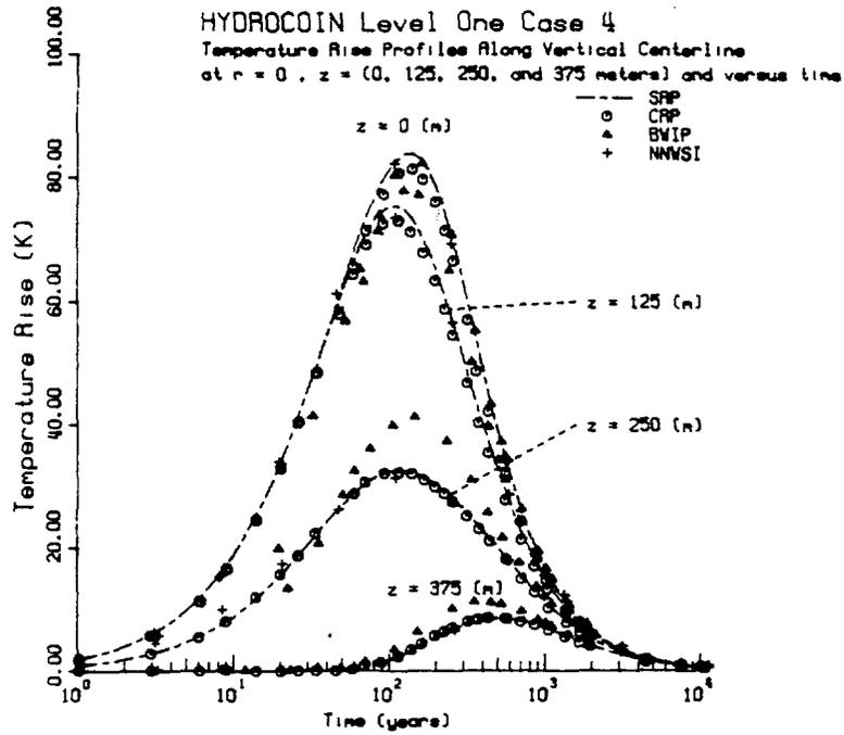
FIGURE 17. Comparison of BWIP, CRP, NNWSI, and SRP Calculations for Temperature Versus Time at Vertical Distances of 0, 125, 250, and 375 m and at a Radius of 0 m
