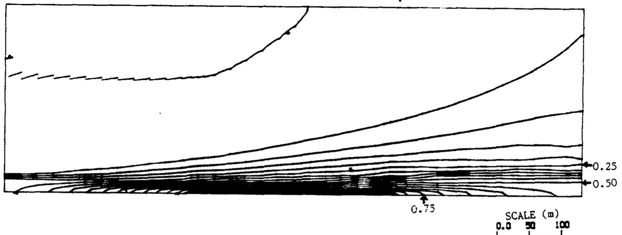
**FIGURE 23.** SRP-Calculated Steady-State, Salt Concentration Contours for Level One, Case 5. The contour interval is 0.05 and concentration is normalized (0-1.0). This figure is taken from SRP results presented at the fourth HYDROCOIN workshop.
