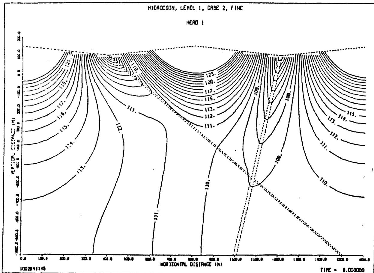
STEADY STATE HYDRAULIC HEAD FIELD, FINE FINITE ELEMENT MESH
