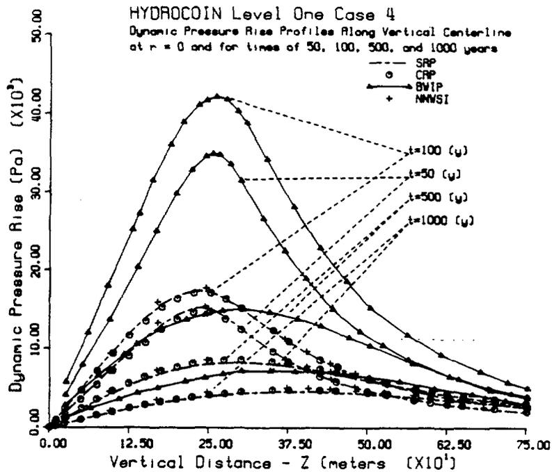
FIGURE 18. Comparison Between BWIP, CRP, NNWSI, and SRP Calculations for Dynamic Pressure Versus Vertical Distance at a Radius of 0 m and at Times of 50, 100, 500, and 1000 Years.
