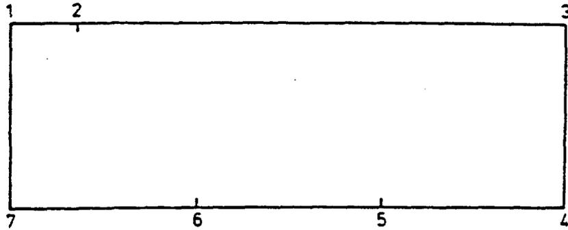
Fig. 5 Geometry of the modelled domain. The bottom boundary between the points 5 and 6 is held at a constant salt concentration.
