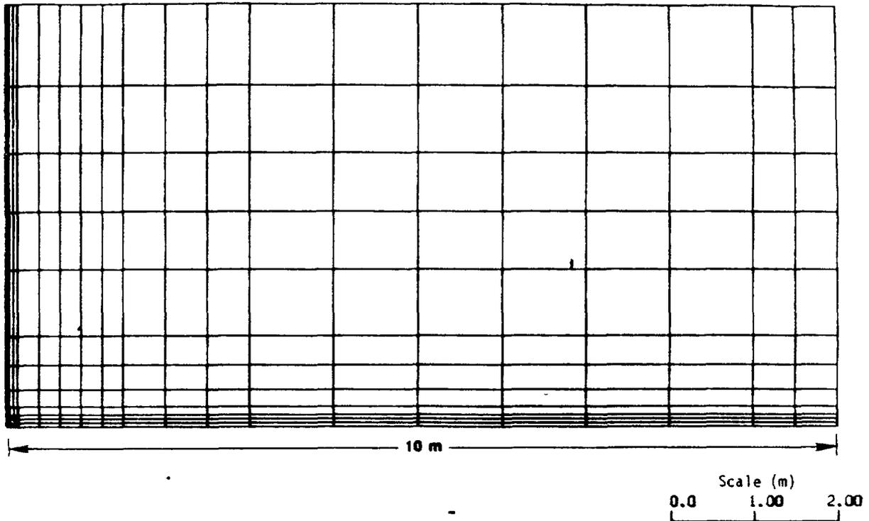
FIGURE 3. A Typical Case 1 Finite Element Grid Mesh. This figure was taken from an SRP presentation at the second HYDROCOIN workshop.
