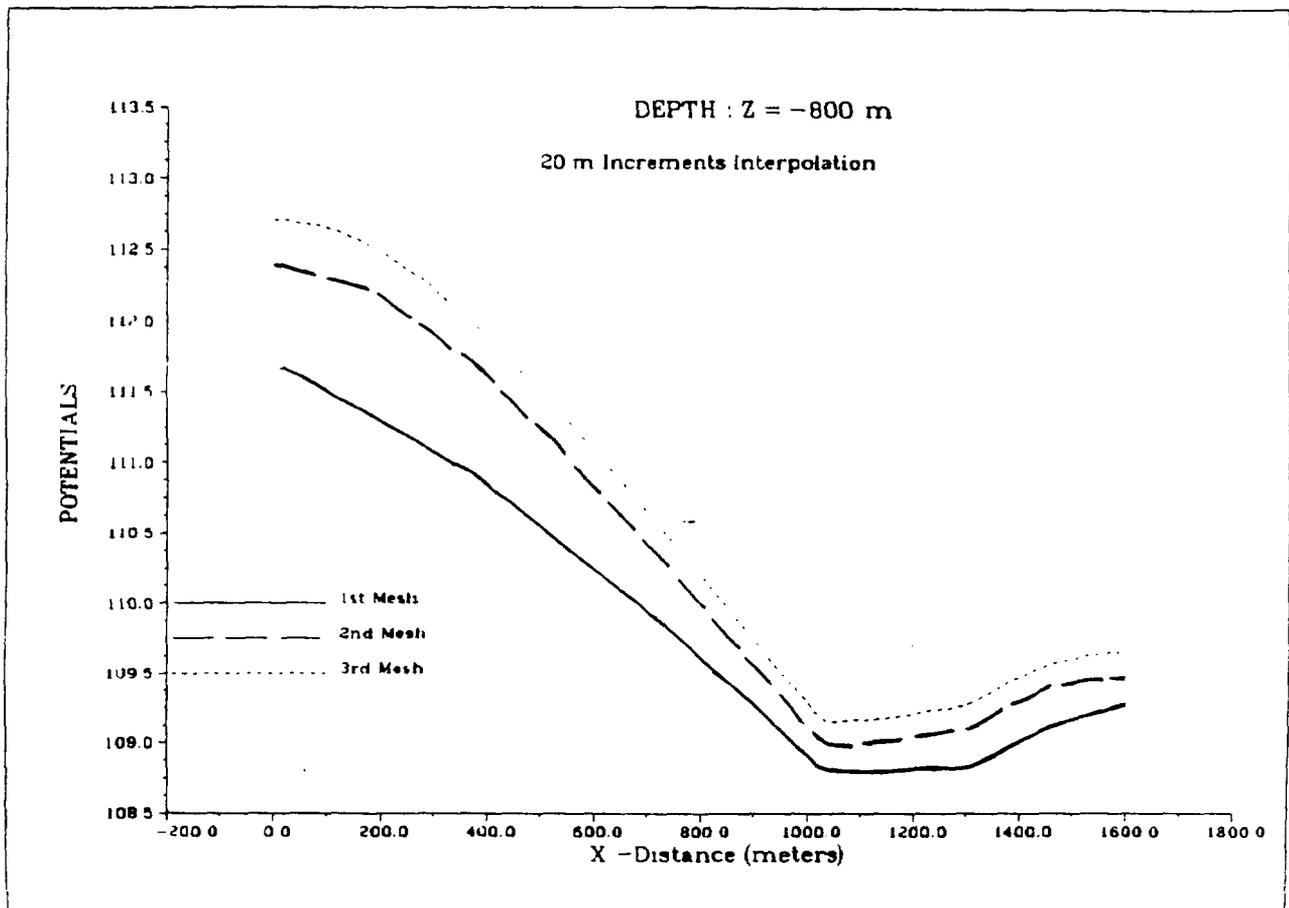
FIGURE 11. CRP Results (presented at the third HYDROCOIN workshop) Illustrating Solution Convergence as a Function of Increased Spatial Resolution. This is a plot of calculated potential versus x-location at an elevation of -800 m for three different grid meshes and linear interpolation.
