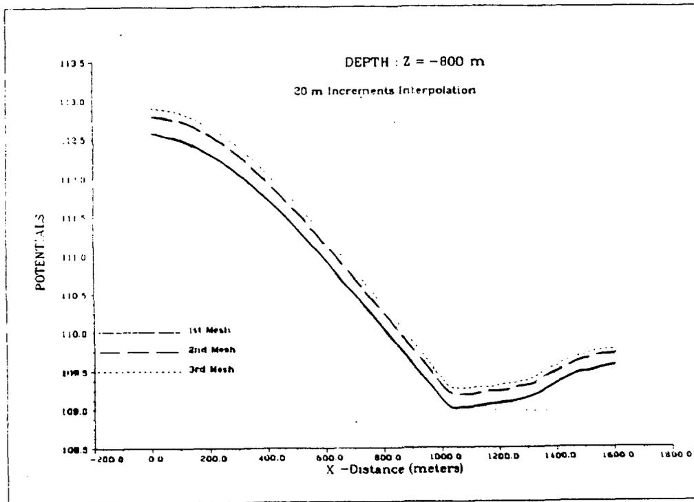
FIGURE 7. CRP Results (presented at the third HYDROCOIN workshop) Illustrating Solution Convergence as a Function of Increased Spatial Resolution. This is a plot of calculated potential versus x-location at an elevation of -800 m for three different grid meshes and quadratic interpolation.
