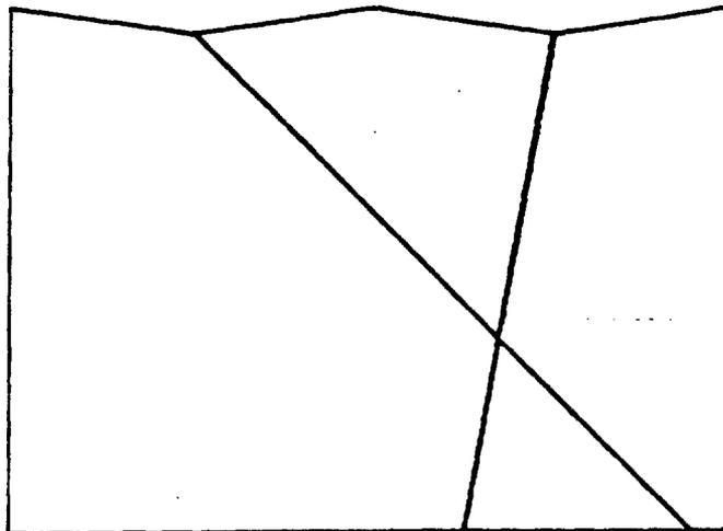
Fig. 2 The geometry of the modelled domain in Case 2. The thick inclined lines represent fracture zones with higher permeability than the rest of the domain.
