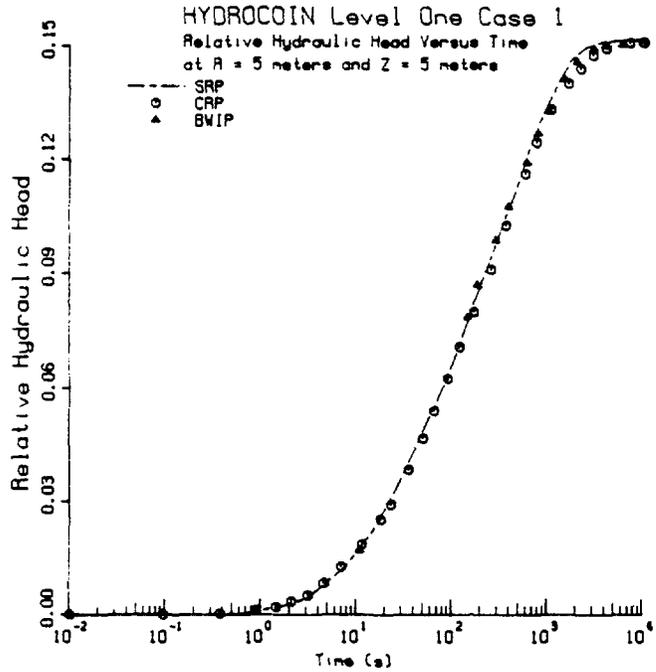
FIGURE 1. A Comparison of BWIP, CRP, and SRP Results for Relative Head as a Function of Time at the Interface Between the Rock Matrix and Fracture
