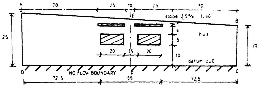
Fig. 7 Schematic diagram of the domain modelled in Case 7. The striped rectangles represent the repository and anti-intervention lids of concrete.
