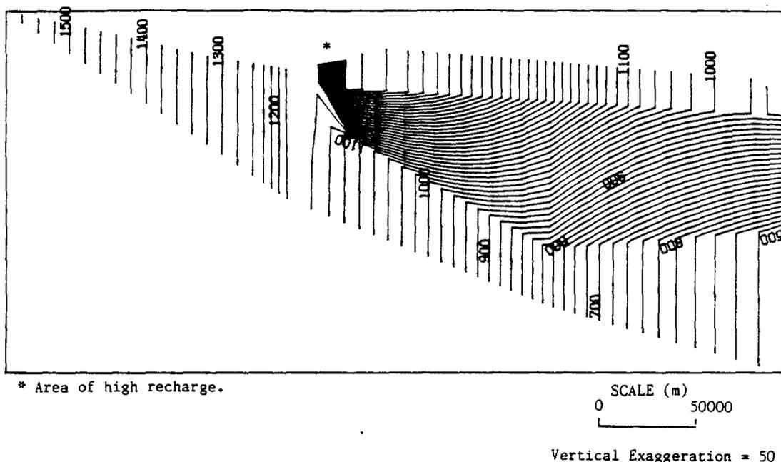
**FIGURE 28.** Contour Map of the Level One, Case 6 Potentials Calculated by SRP with the FE3DGW Code Along a Vertical Cross-Section on the Southern Problem Boundary. The contour interval is 25 m. This figure was taken from SRP results presented at the second HYDROCOIN workshop.
