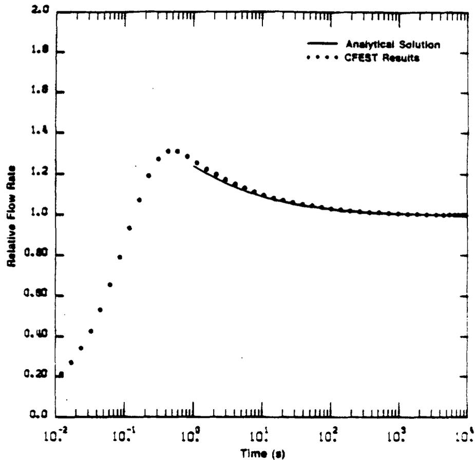
FIGURE 5. SRP Results for Time-Dependent Relative Flow Rate from the Borehole into the Fracture as a Function of Time for the High Transmissivity Optional Calculations. This graph was taken from an SRP presentation at the second HYDROCOIN workshop.
