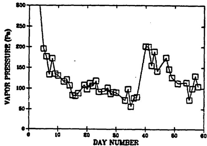
Figure 3 Maximum Vapor Pressure at the Lower End of the Core
