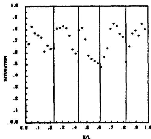
Figure 10 Core Saturation Profile from Gamma-Beam Measurements after 29 days
