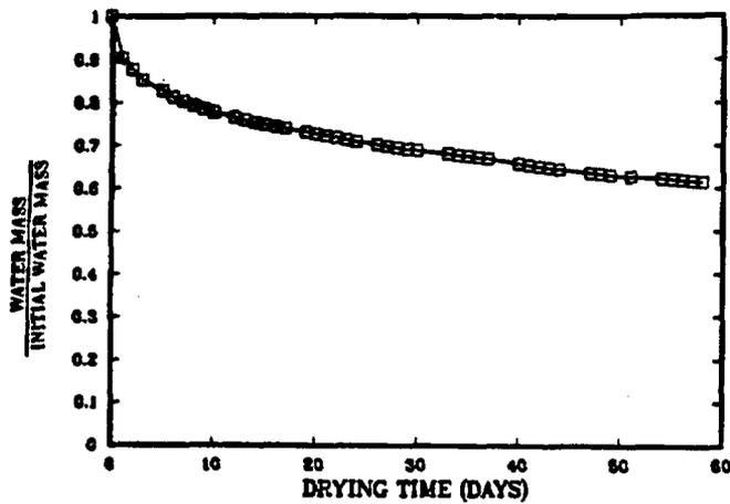
Figure 8 Average Core Saturation from Weight Loss Measurements
