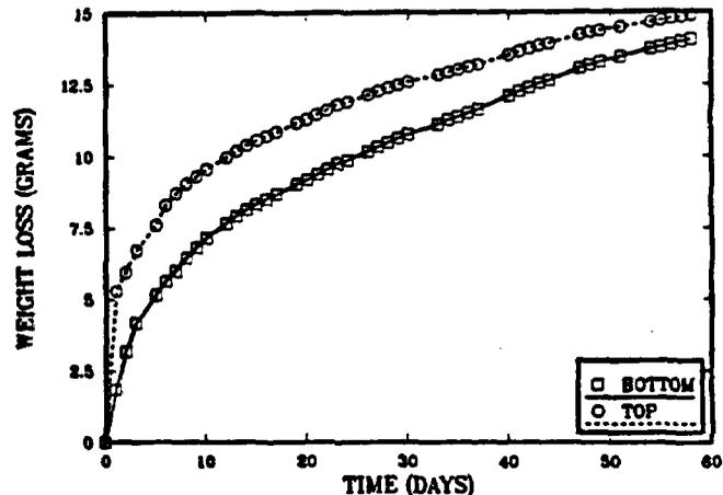
Figure 7 Rate of Water Removal from Each End of the Core
