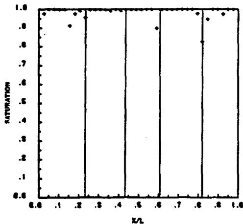
Figure 9 Core Saturation Profile from Gamma-Beam Measurements after 2 days
