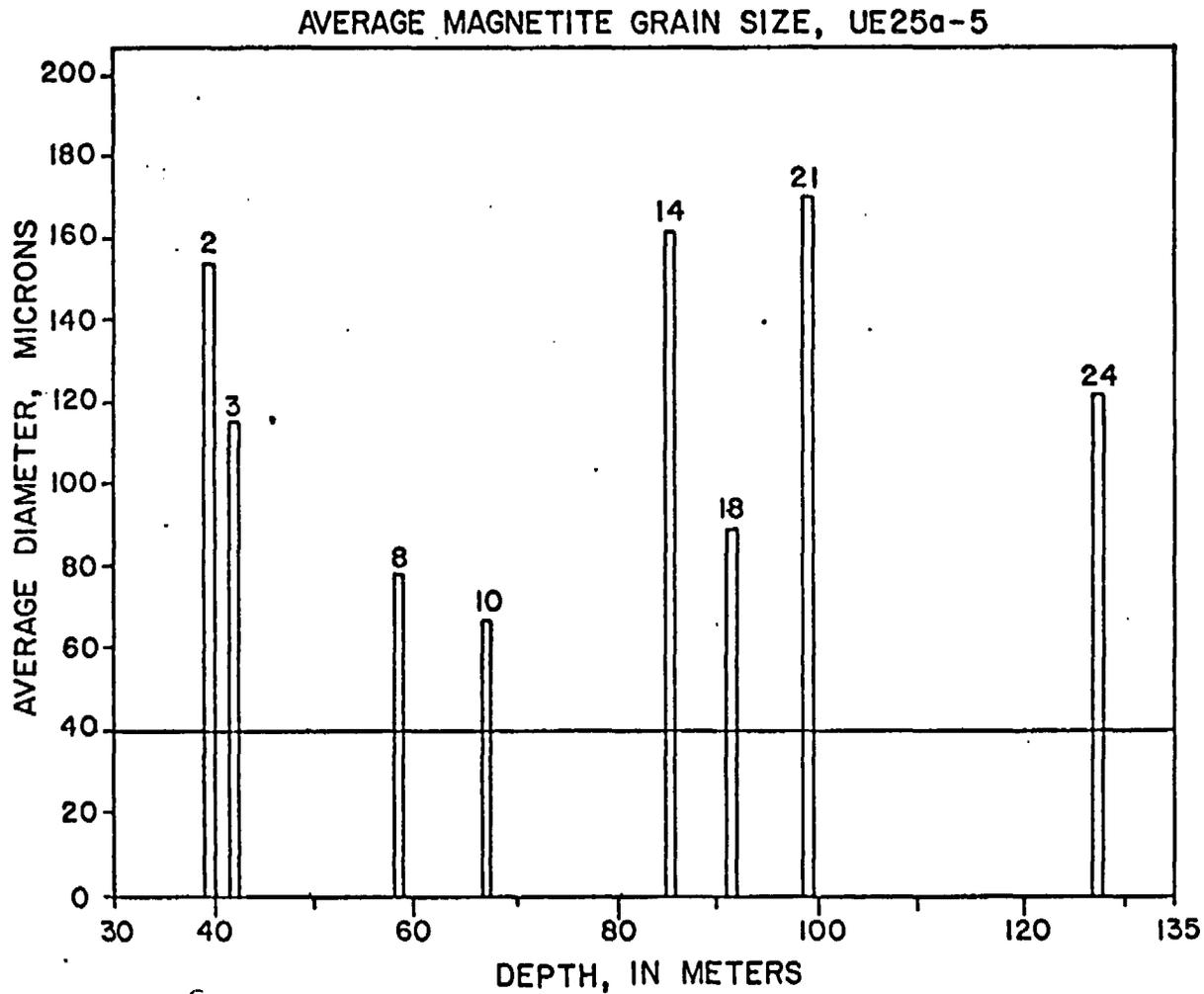
Figure 6.--Average magnetite grain diameters for samples, determined from thin-section observations, from drill hole UE25a-5, Nevada Test Site. The line at 40 microns represents an experimental cutoff below which the magnetic susceptibility of magnetite grains was observed to sharply decrease (figure 7).
