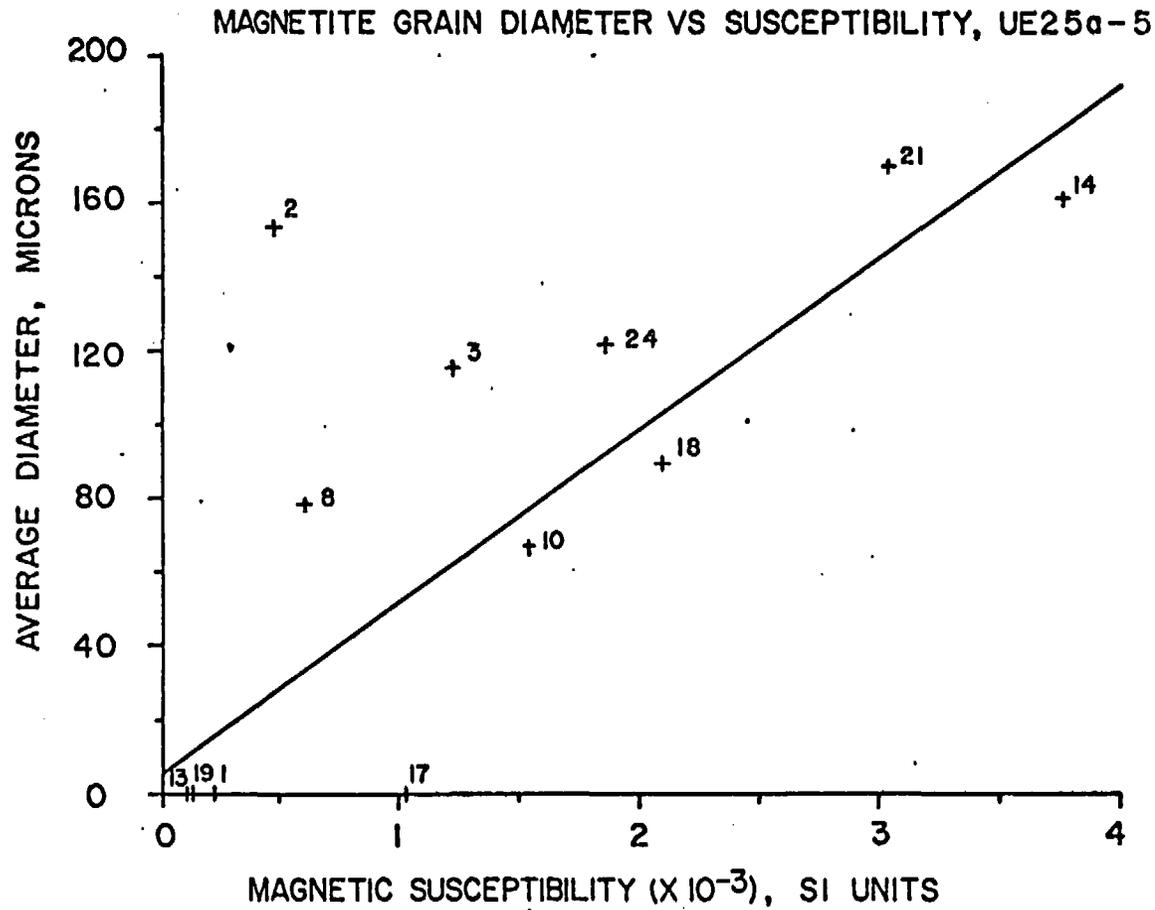
Figure 7.--Average magnetite grain diameter of samples from drill hole UE25a-5, Nevada Test Site, plotted against borehole magnetic susceptibility measurements from corresponding depths. The line represents a least-squares fit of all but one point representing sample 2 (see text).
