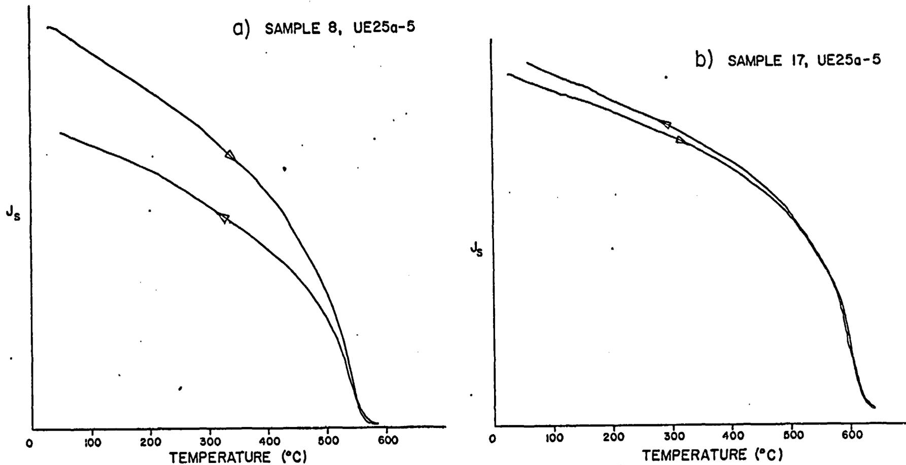
Figure 5.--Curie-balance experiments on heavy separate minerals from samples 8 and 17 from drill hole UE25a-5, Nevada Test Site. Sample 8 exhibits representative behavior for those samples that contained magnetite, and sample 17 shows no magnetite present, demonstrating behavior typical of hematite.
