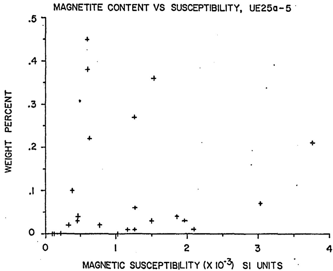
Figure 4.—Weight percent magnetite of samples from drill hole UE25a-5, Nevada Test Site, plotted against borehole magnetic susceptibility measurements from corresponding depths.
