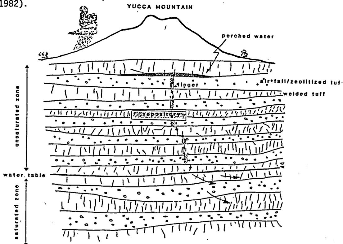
Figure 5. Diagram of NTS Fingering Scenario.
