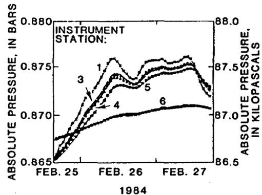
Fig. 6. Adjusted downhole-pressure variations in test borehole USW UZ-1. Differential pressures, measured with land surface transducers, were added to the calculated pneumatic-gravitational potential.
