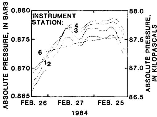
Fig. 5. Downhole-pressure variations at test borehole USW UZ-1, as measured with downhole-pressure transducers.
