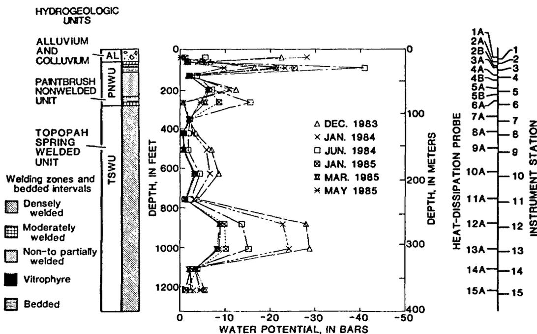
Fig. 8. Water potential in test borehole USW UZ-1 based on data from thermocouple psychrometers.
