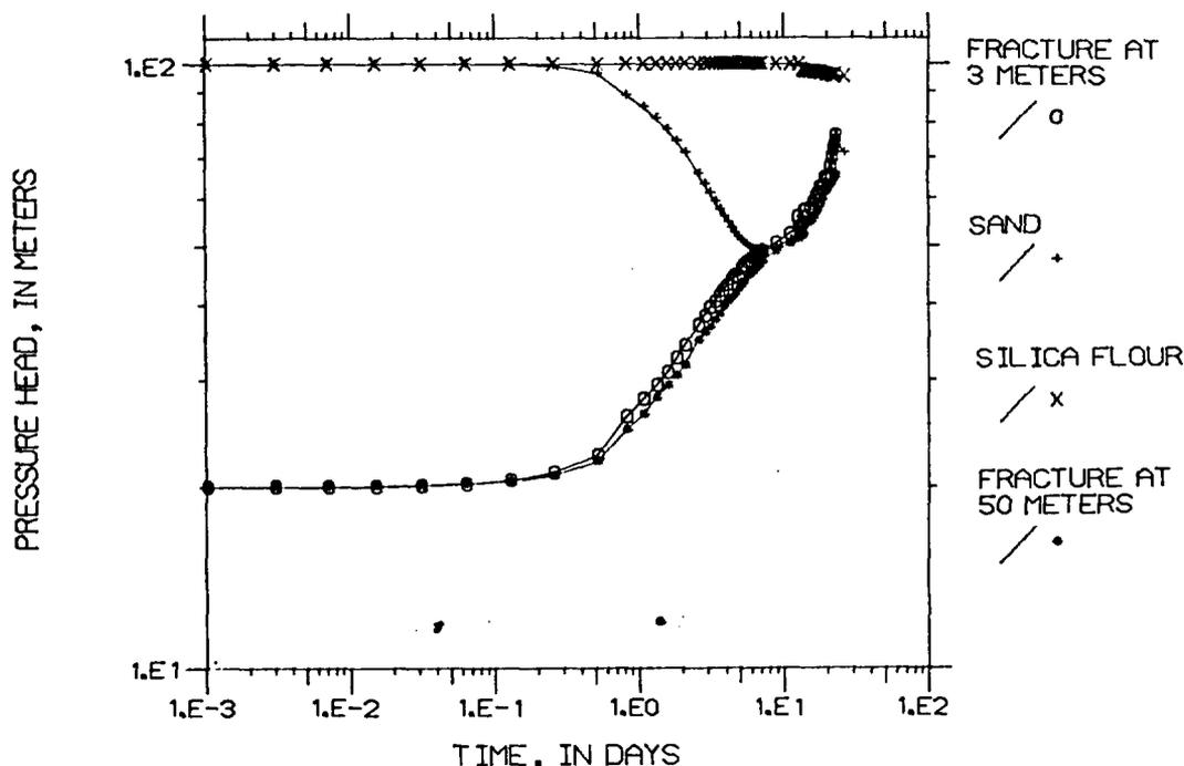
Fig. 13. Variation of pressure head with time at points in the fracture 3 and 50 meters away from the borehole compared with variations in pressurehead of points at the center of the sand column and at a point in the silica flour 7.5 meters above the fracture.
