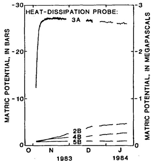
Fig. 3. Variations of matric potential with time in test borehole USW UZ-1 as measured with heat-dissipation probes.
