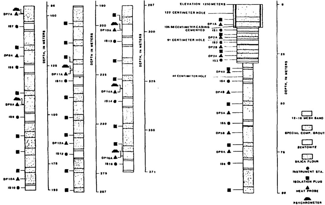
Fig. 2. Details of the stemming of test borehole USW UZ-1.
