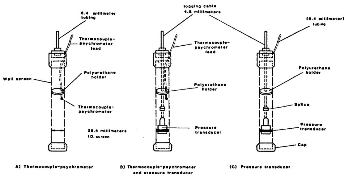
Fig. 1. Schematic diagrams of the well screens and the types of instruments installed in screens A, B, and C, test borehole USW UZ-1.
