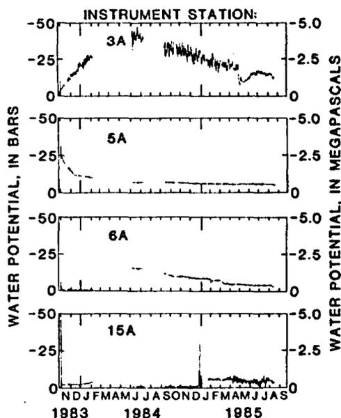
Fig. 10. Variations of water potential with time for selected instrument stations in test borehole USW UZ-1.
