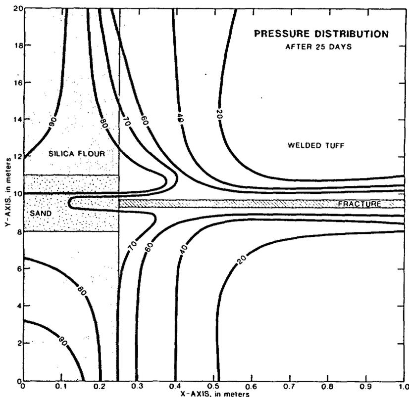
Fig. 14. Contour diagram of the pressure head distribution in the vicinity of the borehole after 25 days; slight wetting of the sand column and severe drying of the fracture are evident.
