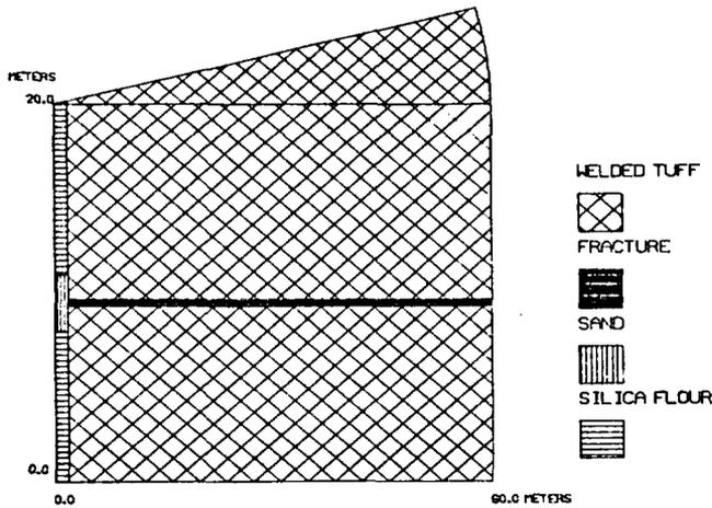
Fig. 11. A slice of the region simulated, 20 meters thick and 100 meters in radius; horizontal fracture is 0.3 meter thick.
