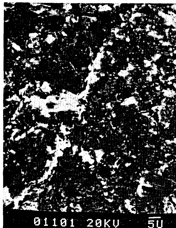
Figure 19. SEM Photograph of Matrix in Sample RMD-11 of Transition Zone (Scale bar is 5 \mu\text{m} .)
