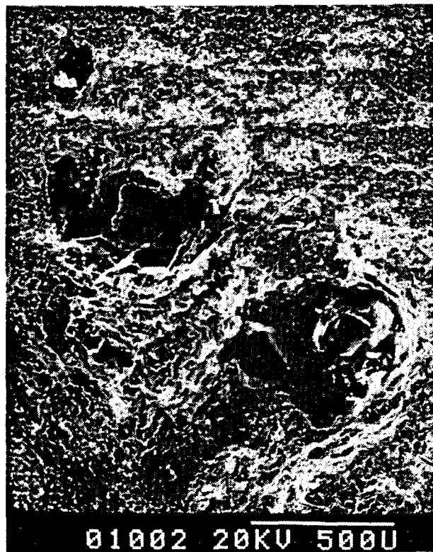
Figure 20. SEM Photograph of Vuggy Pores in Sample RMD-10 of Unit C (Note vapor-phase quartz in pore. Scale bar is 500 \mu\text{m} .)
