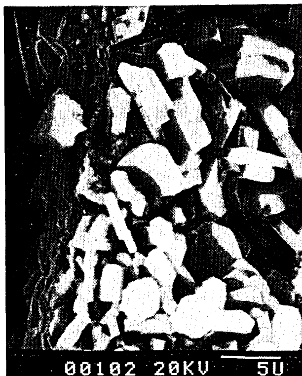
Figure 22. SEM Photograph of Clinoptilolite Crystals in Pore Within Pumice Fragment in Sample RMD-1 of Tunnel Bed 5 (Scale bar is 5 \mu\text{m} .)
