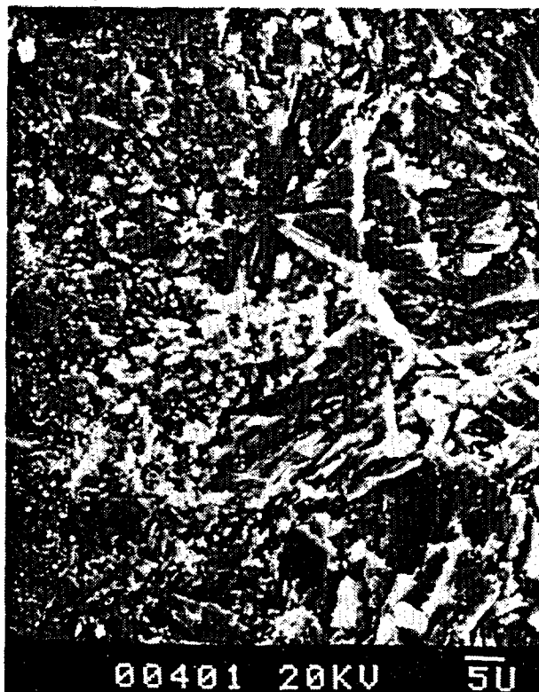
Figure 16. SEM Photograph of Matrix in Sample RMD-4 of Lower Part of Unit B (Scale bar is 5 \mu\text{m} .)
