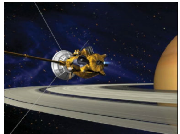
Plutonium-238 powers the Cassini spacecraft orbiting Saturn (NASA)
