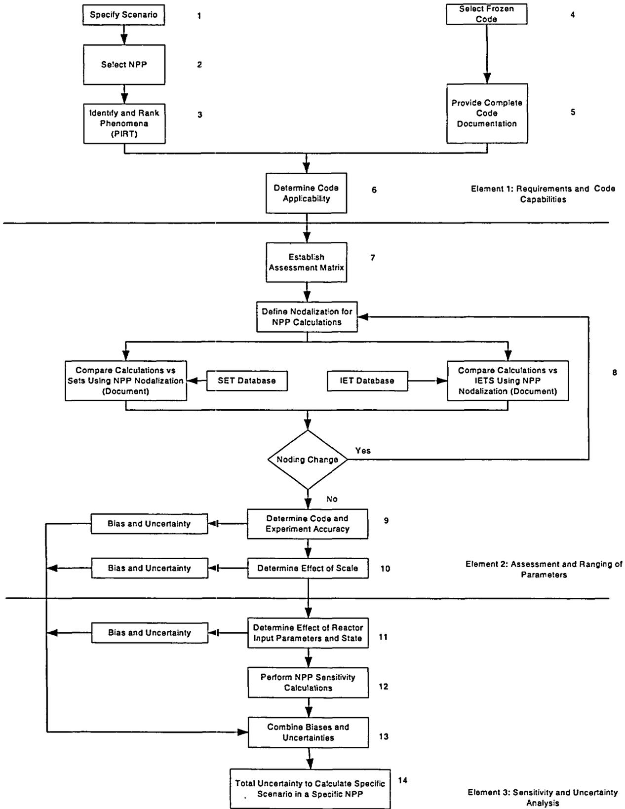
Figure II.5 Illustration of the CSAU Methodology
