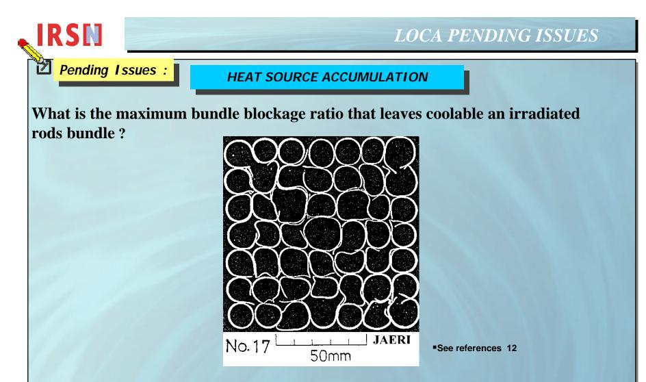
The 90% value derived from results of flooding experiments (FLECHT-SEASET-SEFLEX-FEBA et al) on unirradiated rods arrays is questionable since these experiments did not take account of any fuel relocation and associated effects (lineic and surfacic power increase, gap reduction)
