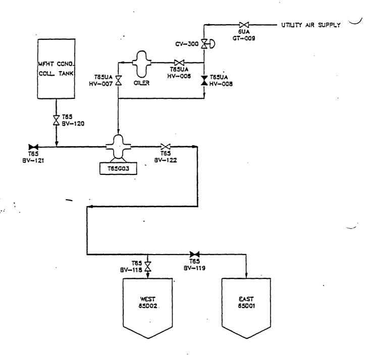
MFHT CONDENSATE COLLECTION TANK TRANSFER TO WEST TANK 65-DO: FIGURE 3
