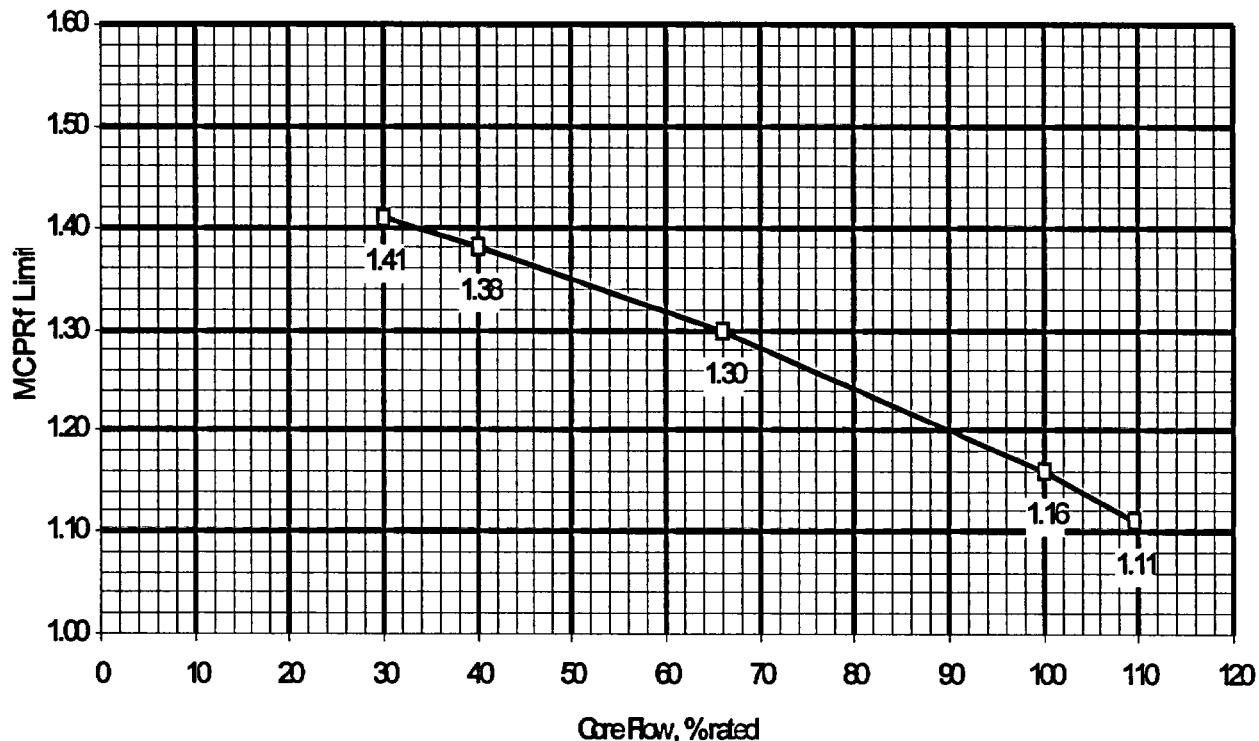
**FIGURE 12. OPERATING LIMIT MCPR (MCPR<sub>F</sub>) VERSUS CORE FLOW FOR GE-11 FOR RECIRCULATION SYSTEM IN LOOP AUTO CONTROL, ALL EXPOSURES**
