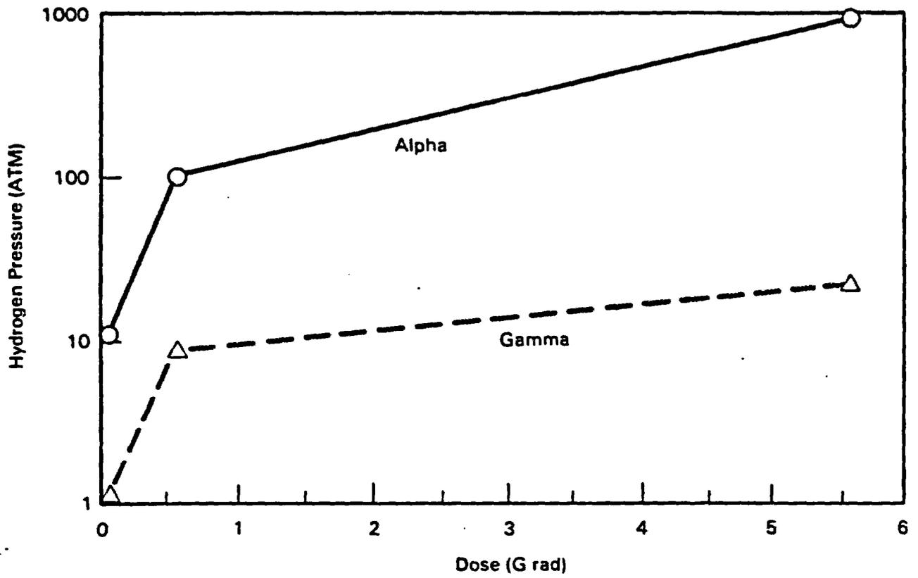
CALCULATED HYDROGEN PRESSURE GENERATED BY GAMMA OR ALPHA
