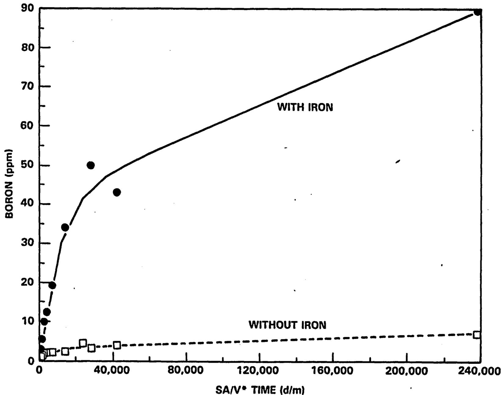
Boron Release From 76-68 Glass vs. SA/V\* Time in Permian Basin brine No. 1 at a Temperature of 70°C, With and Without Iron
