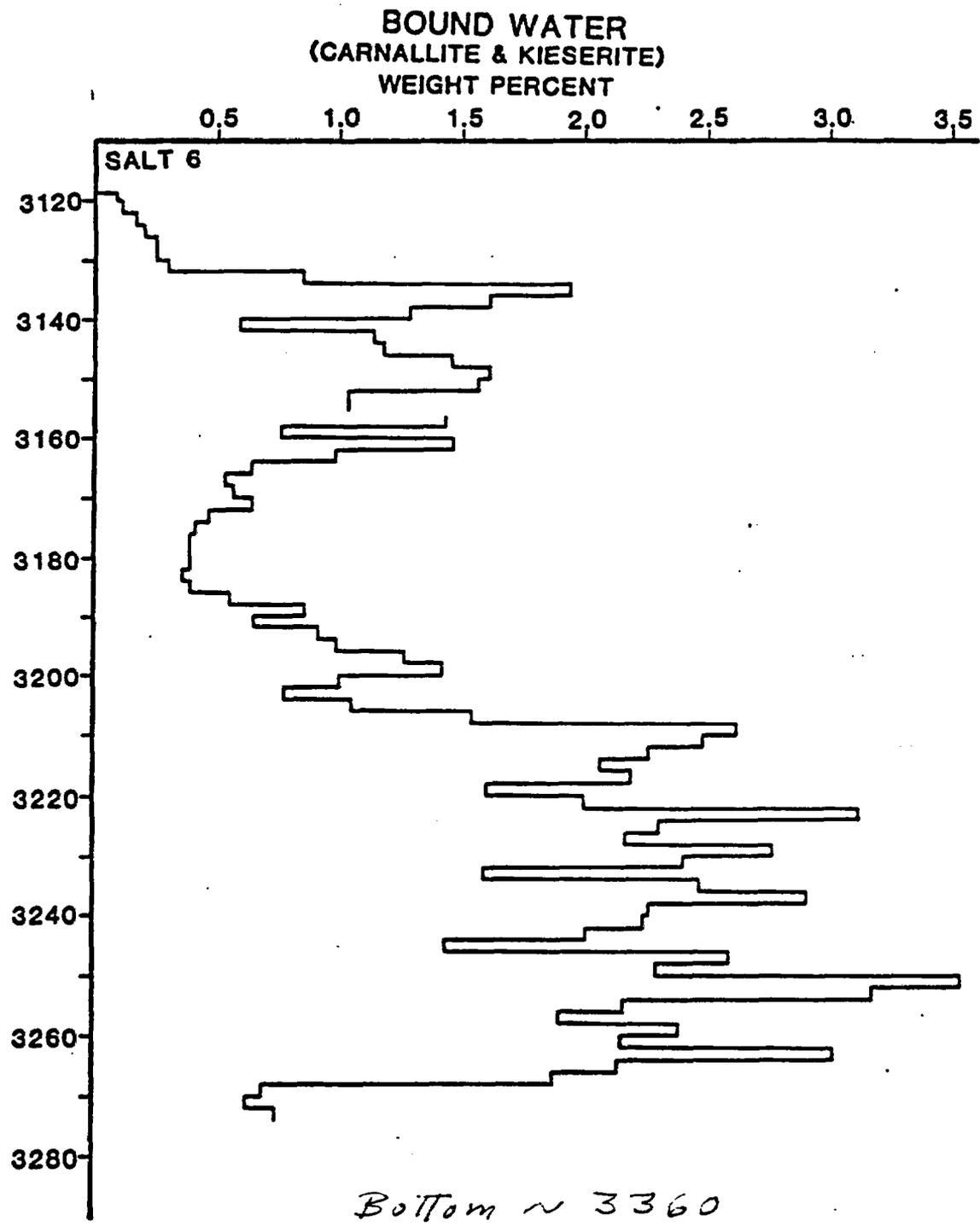
Figure 46.-- Total bound water in the "carnallite marker" of Salt 6 of the Paradox Member, GD-1 core hole. Includes water of crystallization from carnallite ( $KCl \cdot MgCl_2 \cdot 6H_2O$ ) and kieserite ( $MgSO_4 \cdot H_2O$ ).
