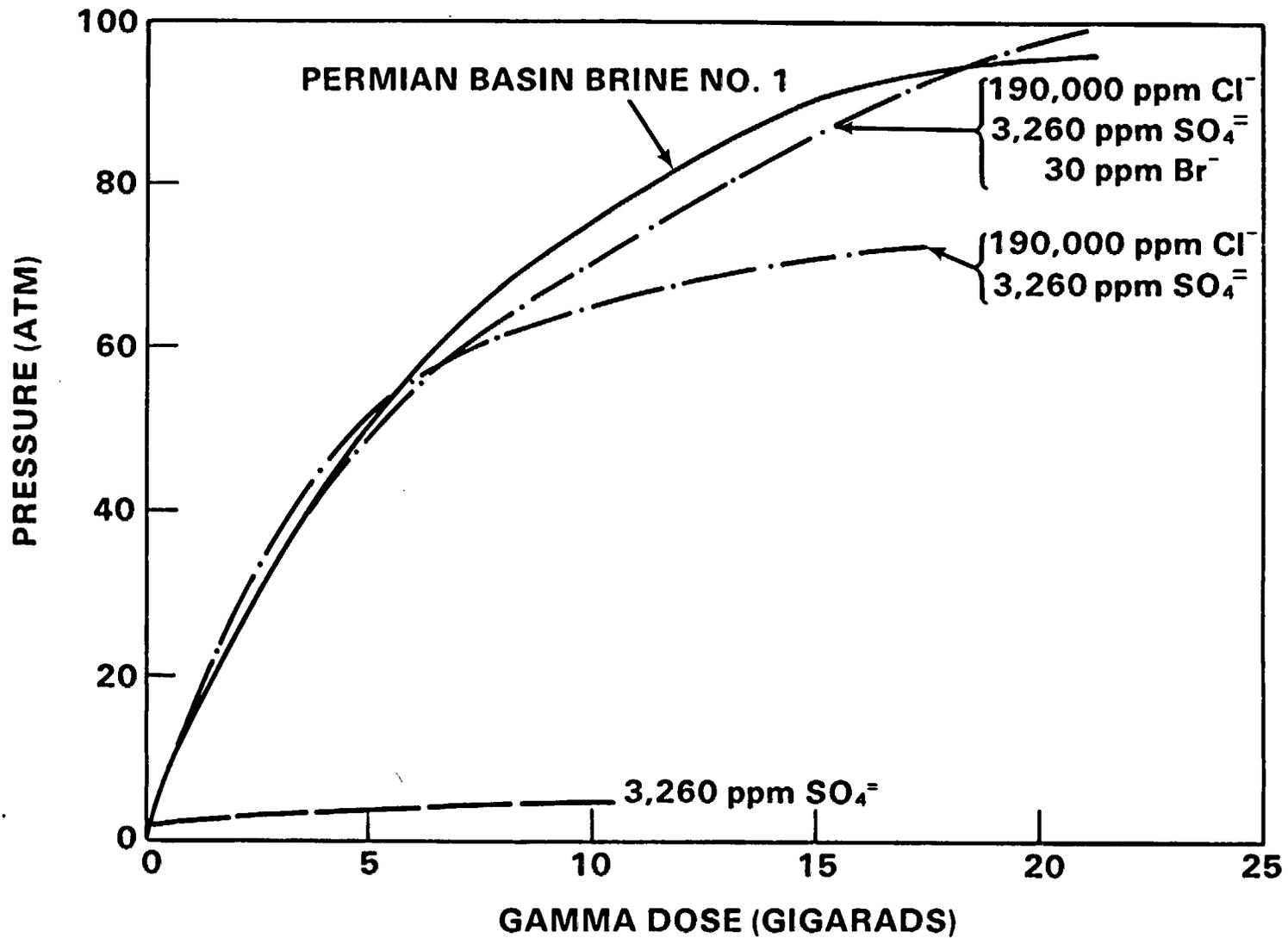
**Gamma Radiolysis Gas Pressure Generation From Various Salt Solutions as a Function of Dose**
