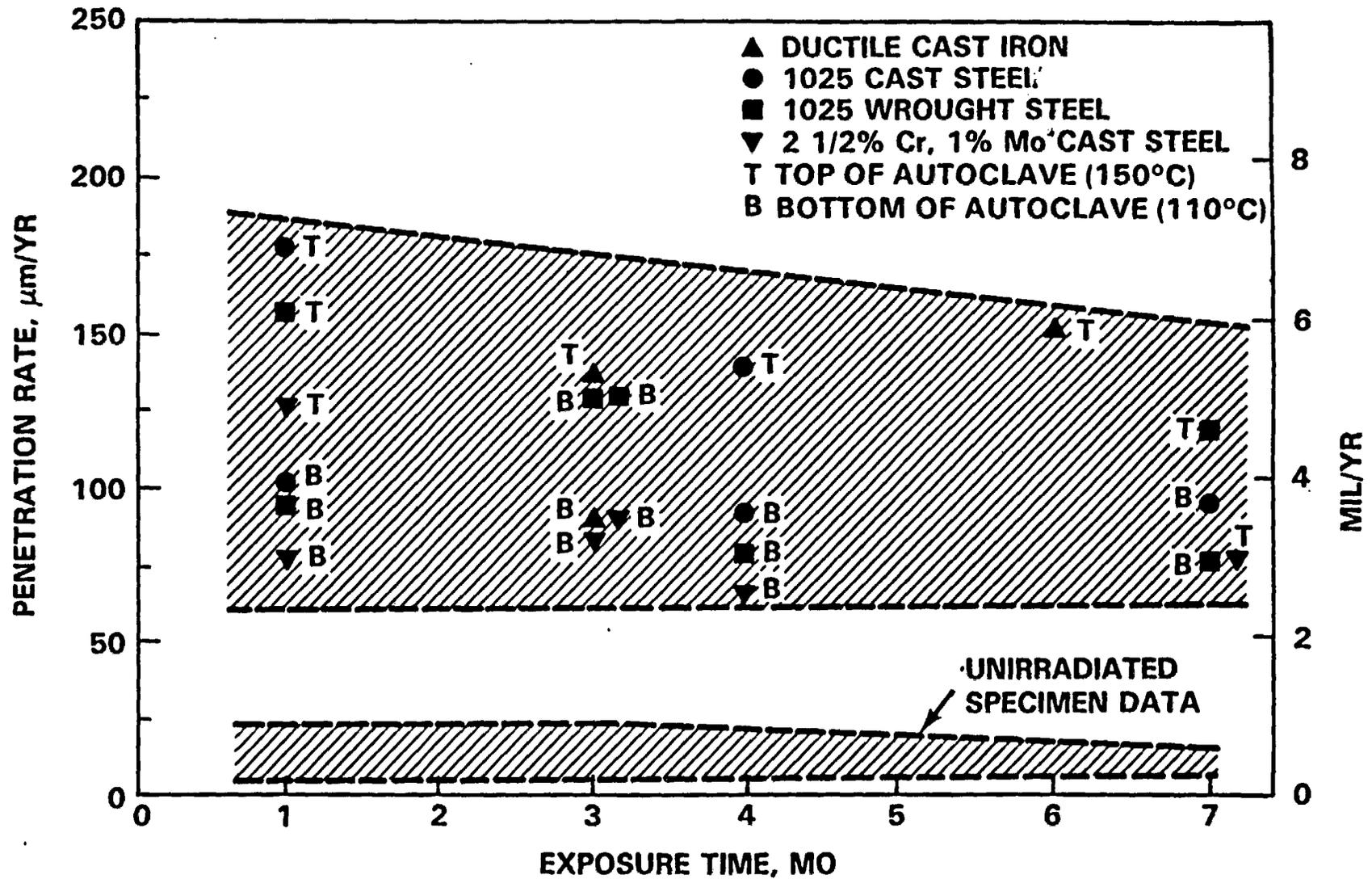
**Irradiation-Corrosion of Ferrous Materials in Permian Basin Brine No. 2 at  $1 \times 10^5$  rad/hr and a Maximum Temperature of 150°C**
