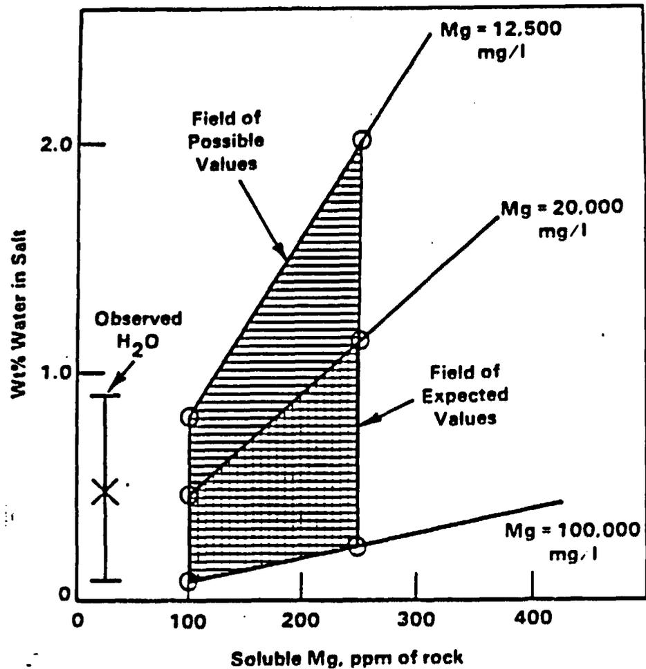
Figure 17. This figure shows the expected content and Mg concentration of fluid inclusions in the Lower San Andres salt beds in depositional cycle 4. The fields of possible and expected values are derived from a sample model of sea water evaporation discussed in the text.
