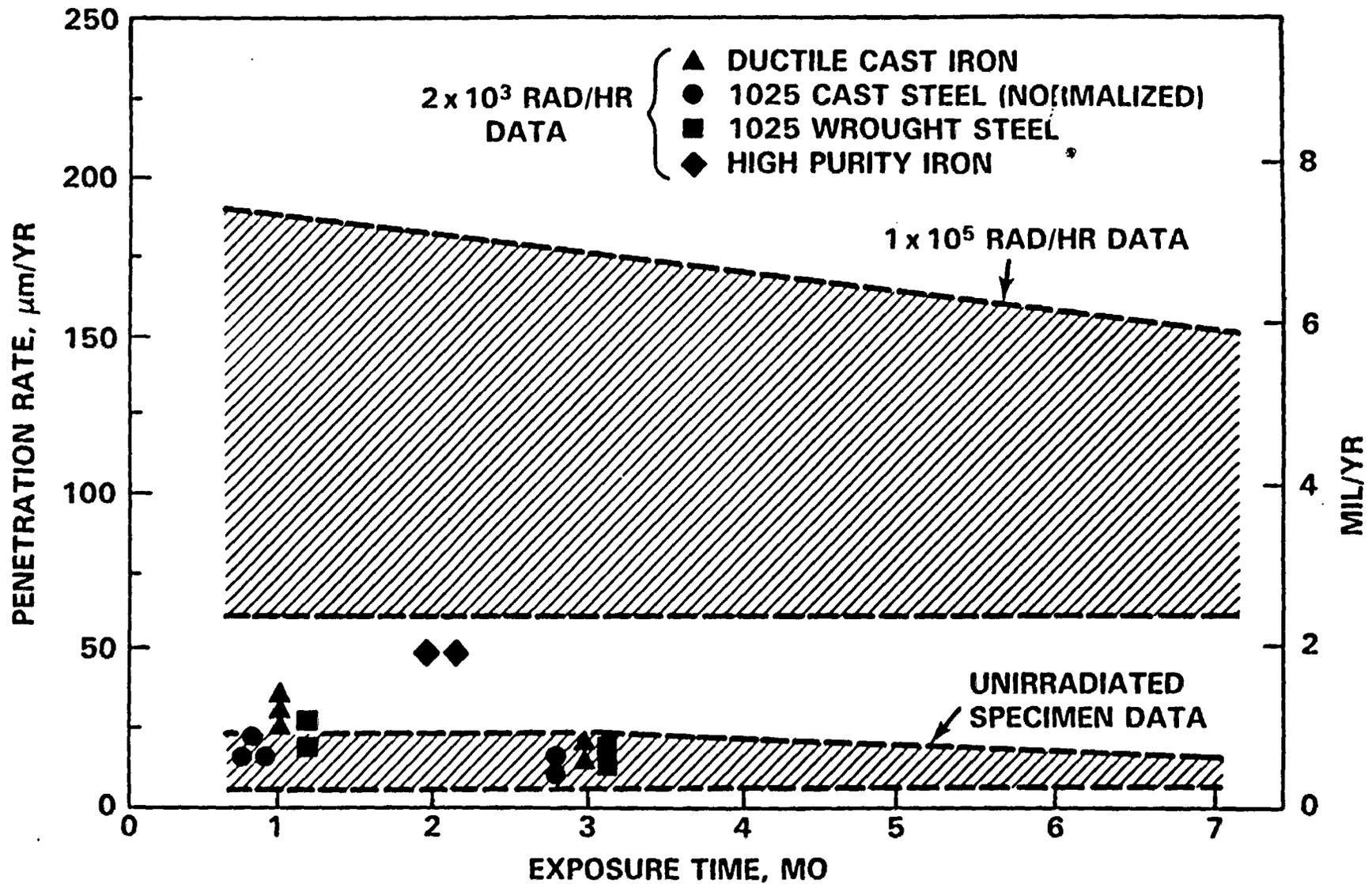
**Irradiation-Corrosion of Ferrous Materials in Permian Basin Brine No. 2 at  $2 \times 10^3$  rad/hr and a Maximum Temperature of  $150^\circ\text{C}$**
