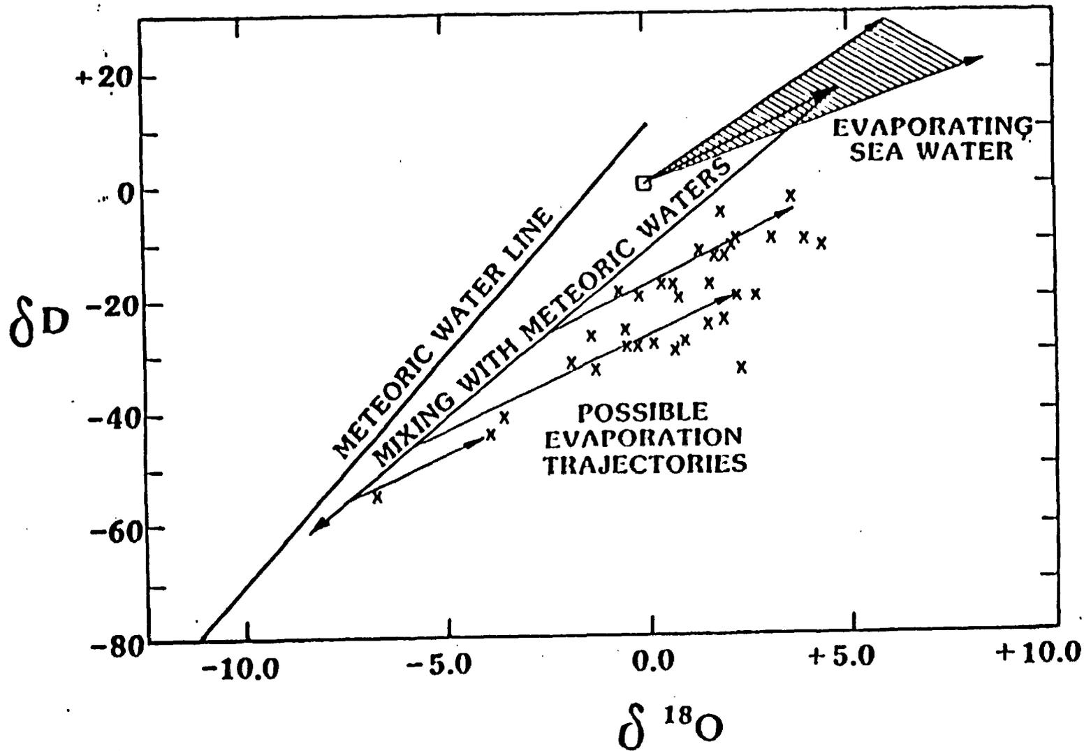
FIGURE 2. POSSIBLE EVAPORATION TRAJECTORIES THAT OVERLAP THE OBSERVED FLUID INCLUSION DATA
