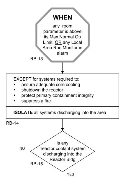
The "**NO**" response based on a leak from the CST (Non Reactor Coolant System) leaking in the Reactor Building directs actions per RB-21.
