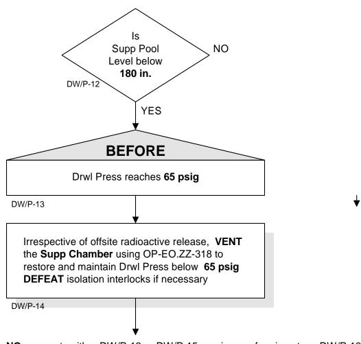
The **NO** answer to either DW/P-12 or DW/P-15 requires performing steps DW/P-16 and DW/P-17, a less desirable vent path using the Drywell (**see below**).
