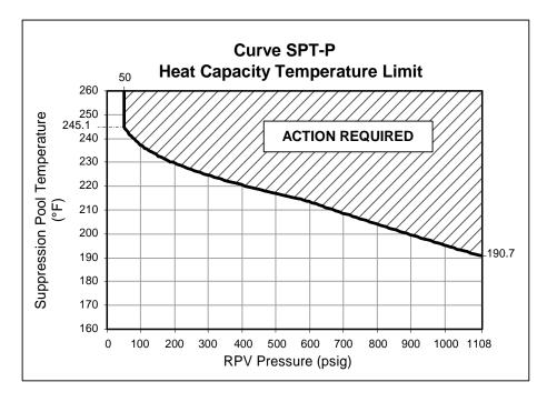
we see that to be on the curve approaching the limit, we are well above the 150 °F required for Boron Injection Initiation temperature requirement of step RQ/Q-10. Therefore Choice "b" is also correct.
