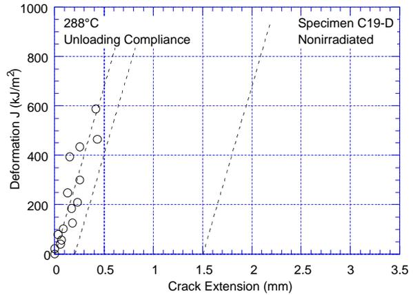
Figure 16. Fracture toughness J-R curve obtained by DC potential and unloading compliance methods for nonirradiated specimen C19-D of Heat C19 of Type 304 SS at 288°C.
