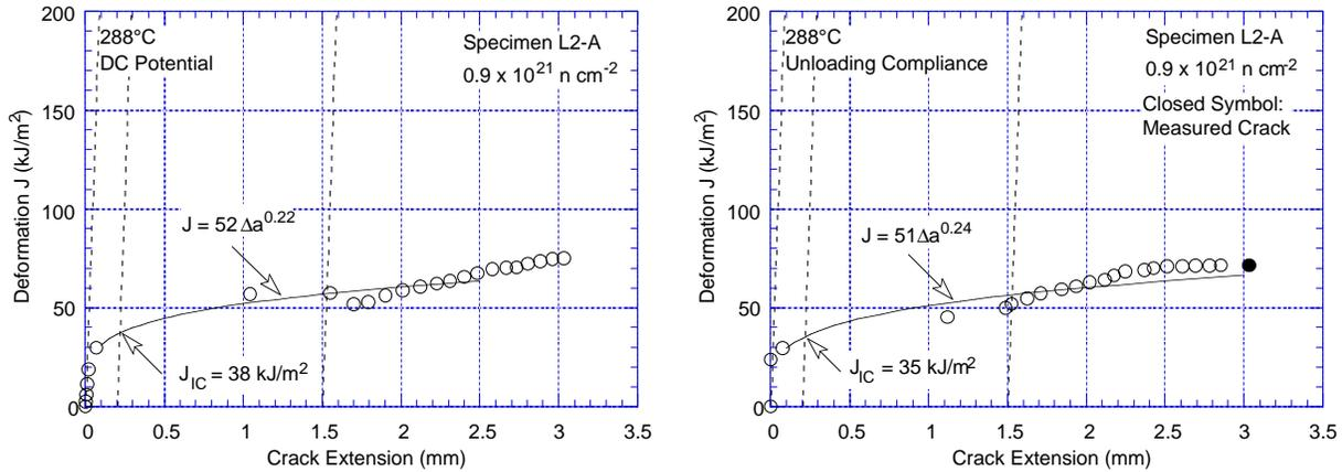
Figure 24. Fracture toughness J-R curve obtained by DC potential and unloading compliance methods at 288°C for Heat L2 of Type 304 SS irradiated to a fluence level of  $0.9 \times 10^{21} \text{ n/cm}^2$ .
