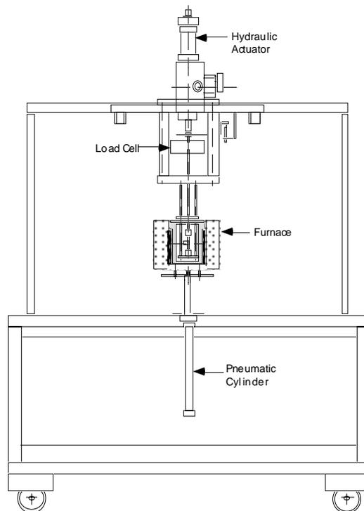
Figure 3. Schematic representation of hot-cell J-R test facility
