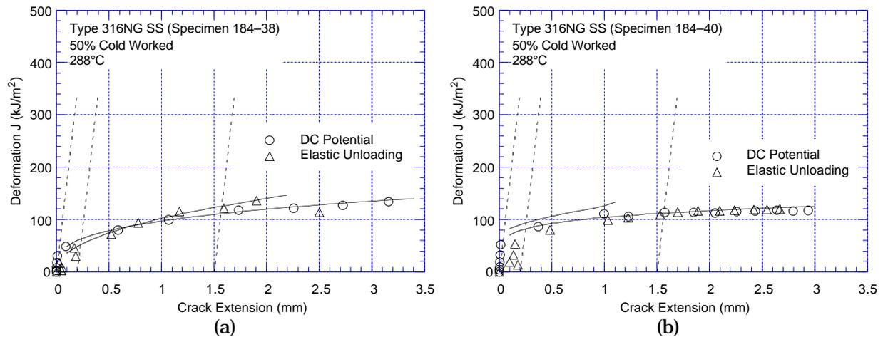
Figure 9. Fracture toughness J-R curves obtained from DC potential and elastic unloading compliance methods for 50% cold-worked Type 316NG; specimen (a) 184-38 and (b) 184-40
