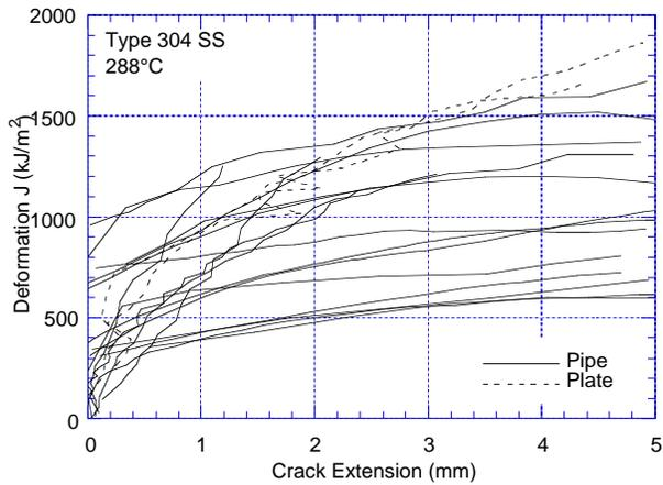
Figure 17. Fracture toughness J-R curves for nonirradiated Type 304 stainless steels at 288°C.
