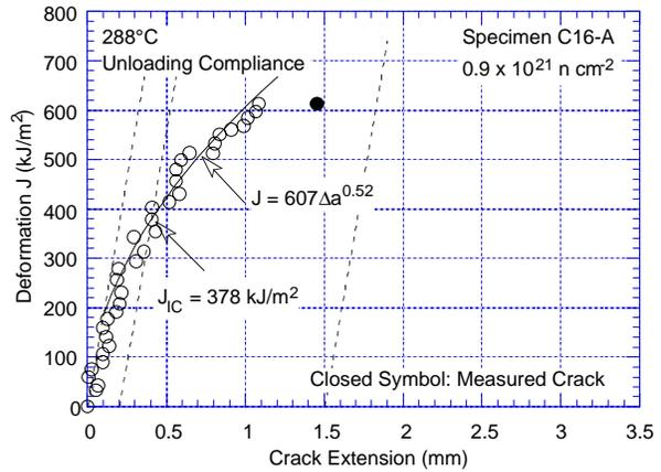
Figure 22. Fracture toughness J-R curve obtained by DC potential and unloading compliance methods at 288°C for Heat C16 of Type 316 SS irradiated to a fluence level of  $0.9 \times 10^{21}$  n/cm<sup>2</sup>.
