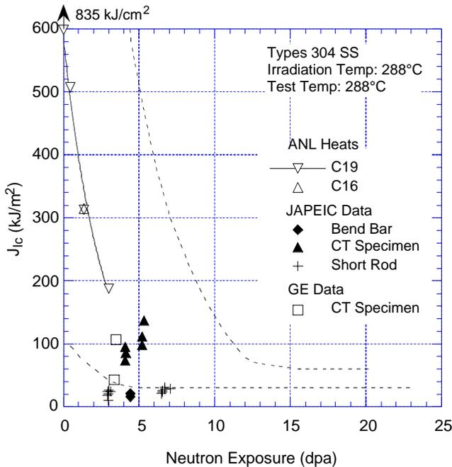
Figure 25. Fracture toughness  $J_{IC}$  of austenitic stainless steels as a function of neutron exposure at 288°C. Dashed lines represent upper and lower bounds for change in  $J_{IC}$  for austenitic SSs irradiated at 350–450°C. JAPEIC = Japan Power Engineering and Inspection Corporation, GE = General Electric Nuclear Energy
