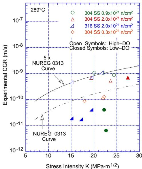
Figure 38. CGR data under constant load with periodic partial unloads for irradiated austenitic SSs in high-purity water at 289°C
