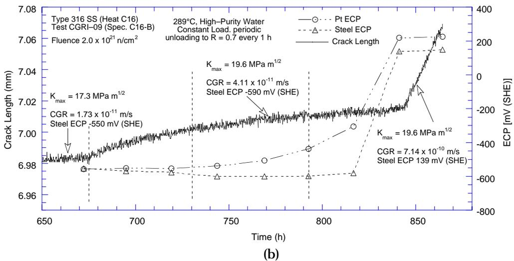
Figure 32. Change in crack length and ECP of Pt and SS electrodes when the DO level in feedwater was (a) decreased from  $\approx 300$  to  $<40$  ppb and (b) increased from  $<40$  to  $\approx 300$  ppb.
