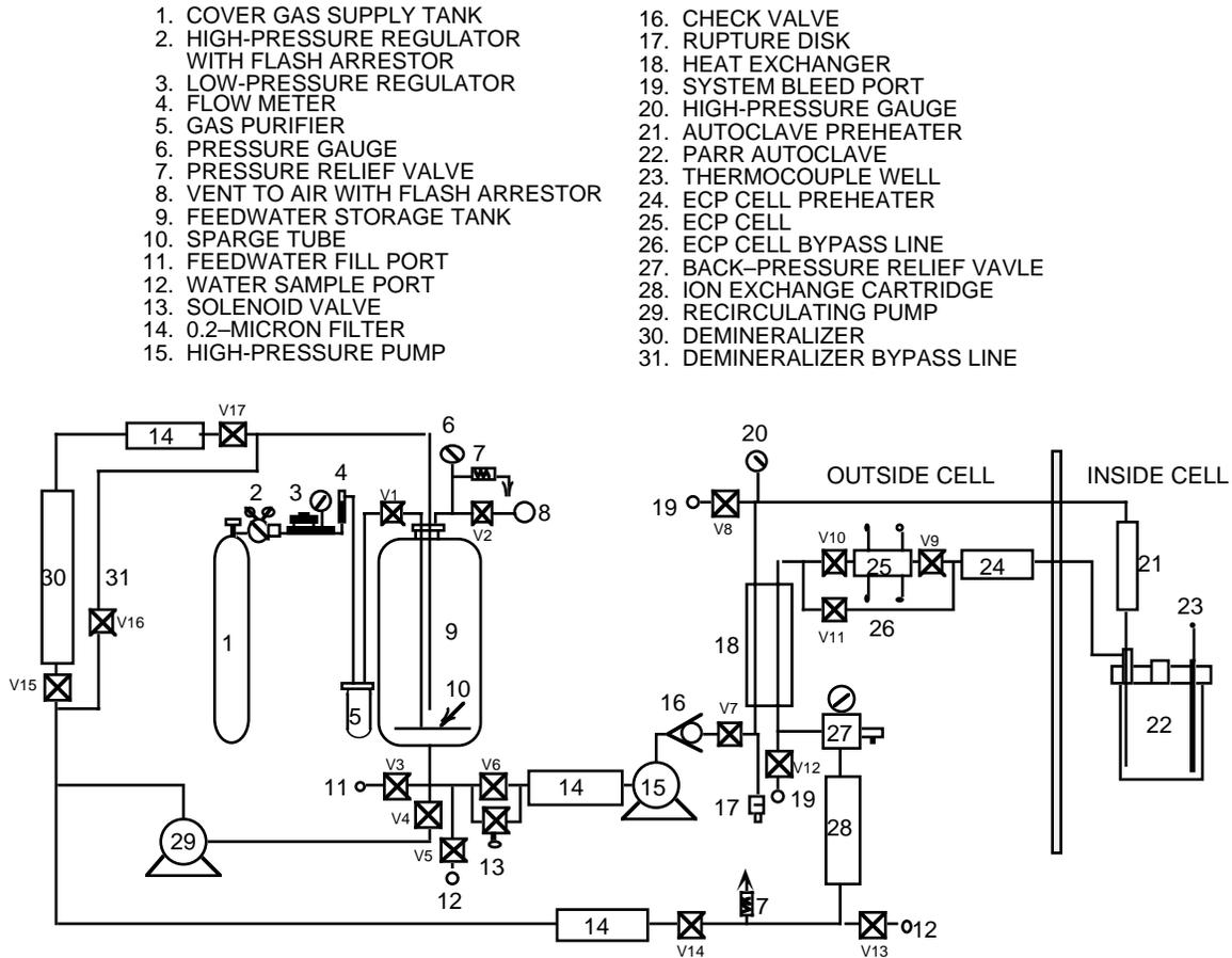
Figure 5. Schematic diagram of recirculating water system
