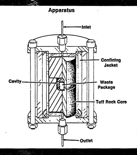
In a 13 week analog test, (NL)<sub>wt</sub> was 0.1 glm<sup>2</sup>
