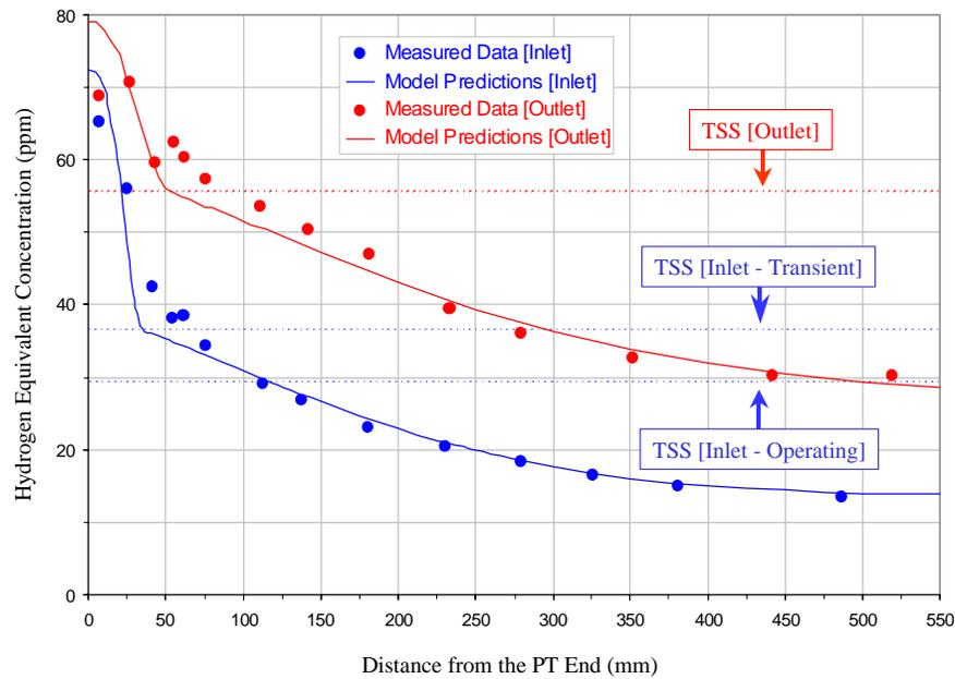
**Figure 9-12 Hydrogen Equivalent Concentration at the Inlet End and Outlet End of a Pressure Tube after 17 Hot Years of Operation. The model incorporates a postulated transient temperature increase at the inlet end during reactor startup.**
