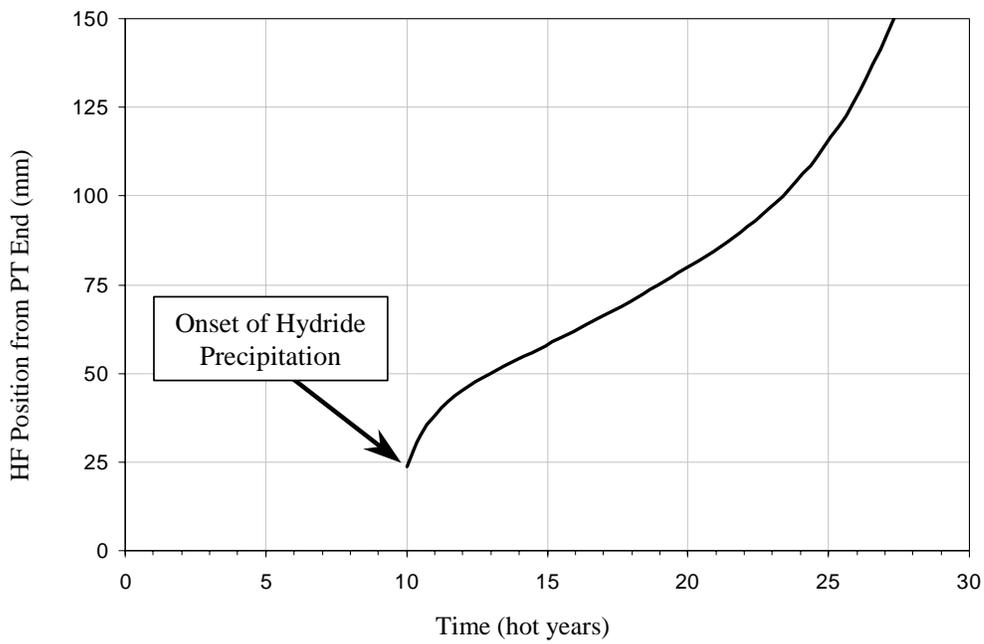
**Figure 9-15 Hydride Front Propagation along the Outlet End of a CANDU 6 Pressure Tube**
