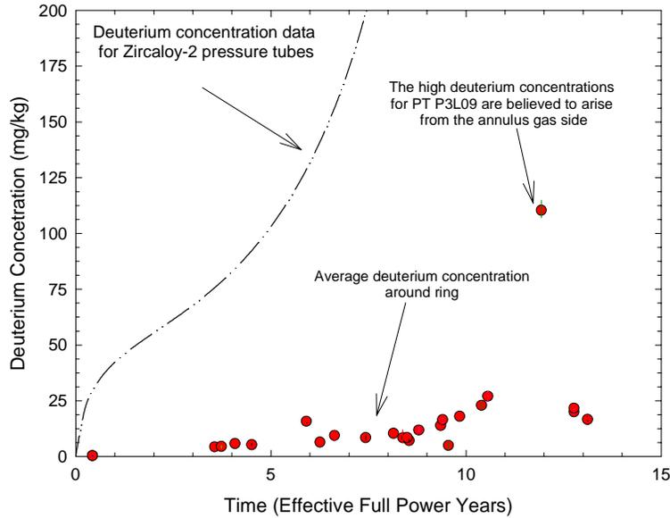
**Figure 9-3 The Measured Deuterium Concentration in Zr-2.5Nb Surveillance Pressure Tubes near the Outlet of the Fuel Channel as a Function of Time<sup>14</sup>**
