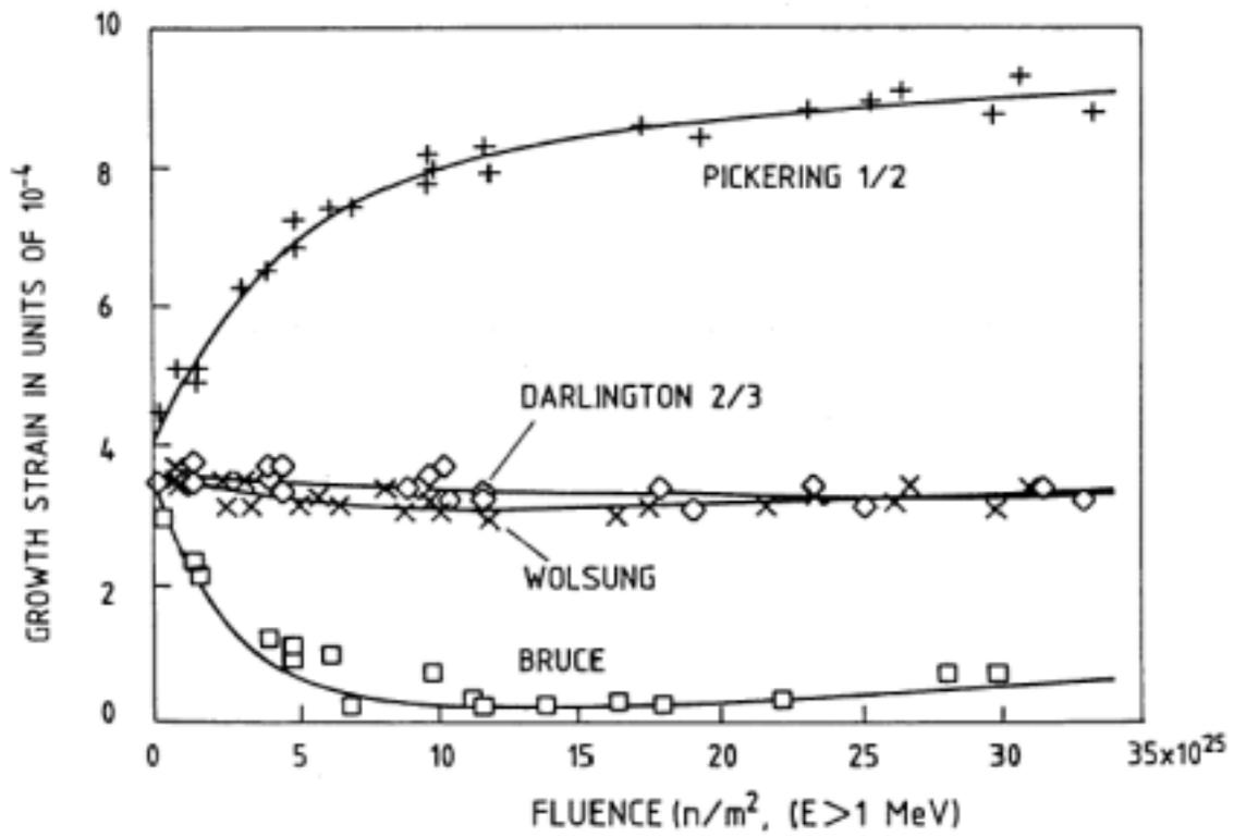
**Figure 16-6 The Irradiation Growth Behavior in the Longitudinal Direction at 60°C of Specimens taken from Different Production Runs of Calandria Tubes and Irradiated in the High-Flux ATR**
