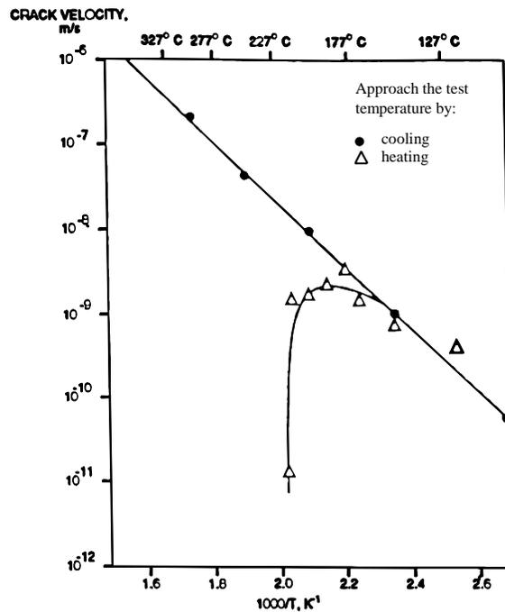
Figure 12-6 Effect of Approaching the Test Temperature by Heating or by Cooling on DHCV [12.9]
