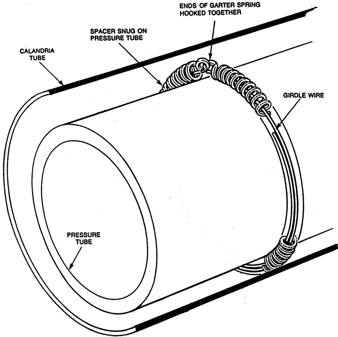
**Figure 17-1 The Current Design for CANDU Fuel Channel Annulus Spacers**
