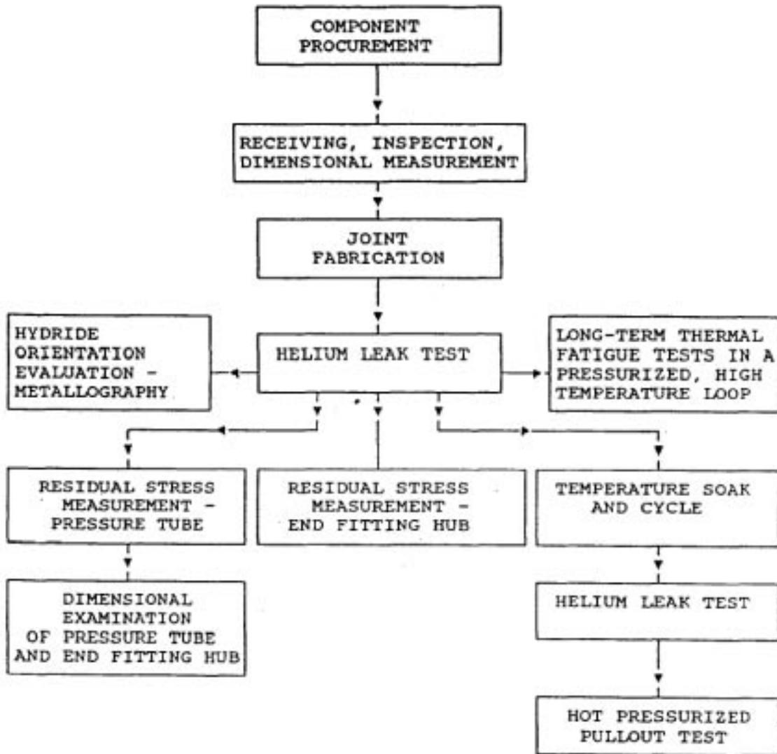
Figure 7-5 Primary Constituents of a Rolled Joint Test Program
