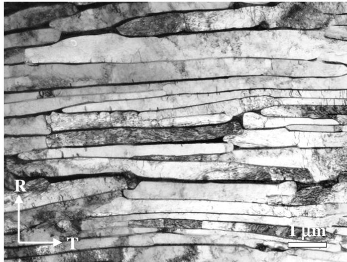
**Figure 10-1 Typical Grain Structure in Zr-2.5Nb Pressure Tube. The light colored  $\alpha$ -phase platelets are interspersed with dark-colored  $\beta$ -phase filaments.**
