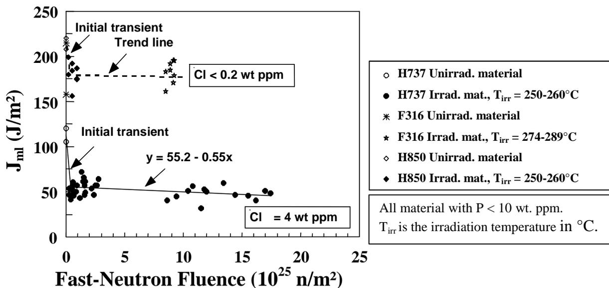
Figure 10-16  $J$  at Maximum Load,  $J_{ml}$ , from Curved Compact Specimens of Irradiated Material Tested at 240/250°C Versus Fast Neutron Fluence [10.9]
