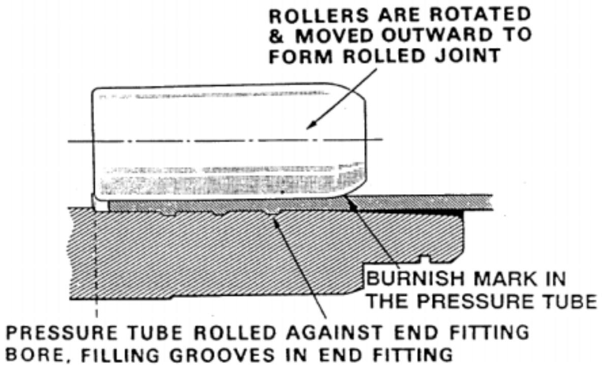
**Figure 7-1 Typical Pressure Tube to End Fitting Rolled Joint**
