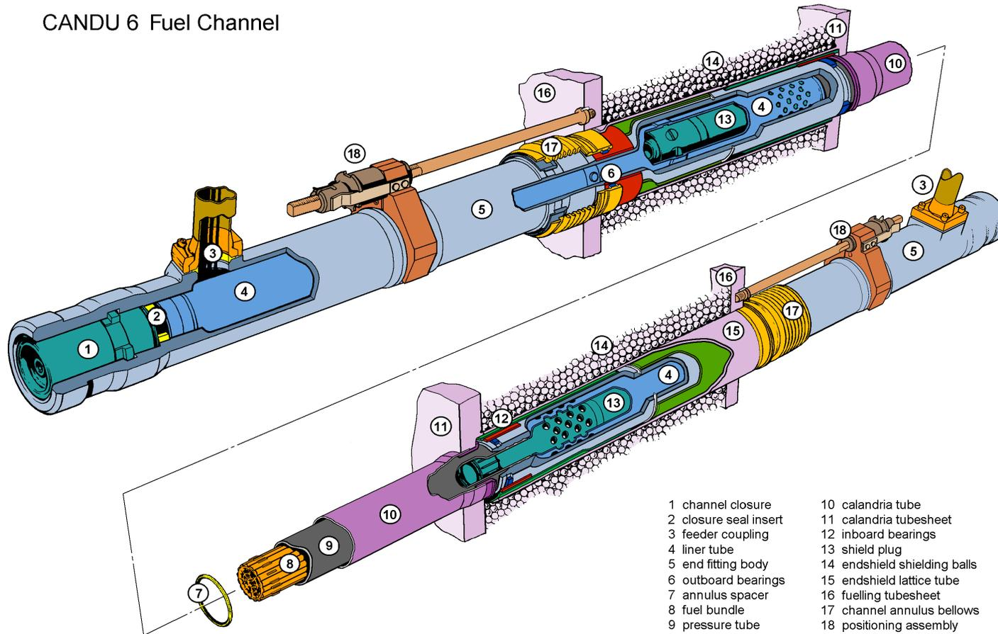
Figure 1-6 Details of the CANDU-6 Fuel Channel
