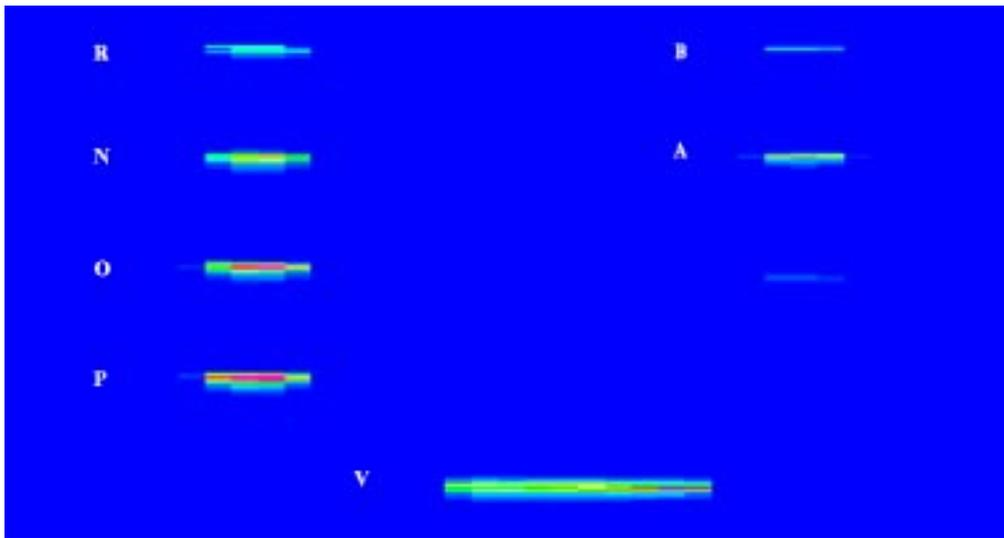
**Figure 11-1 Ultrasonic C-Scan Display Showing Response from Calibration Artifacts with a Circumferentially-Directed, 45° Shear Wave. Notches A and B are 6 mm long by 0.15 mm and 0.075 mm deep respectively. Notch A is a reference calibration for ultrasonic testing.**
