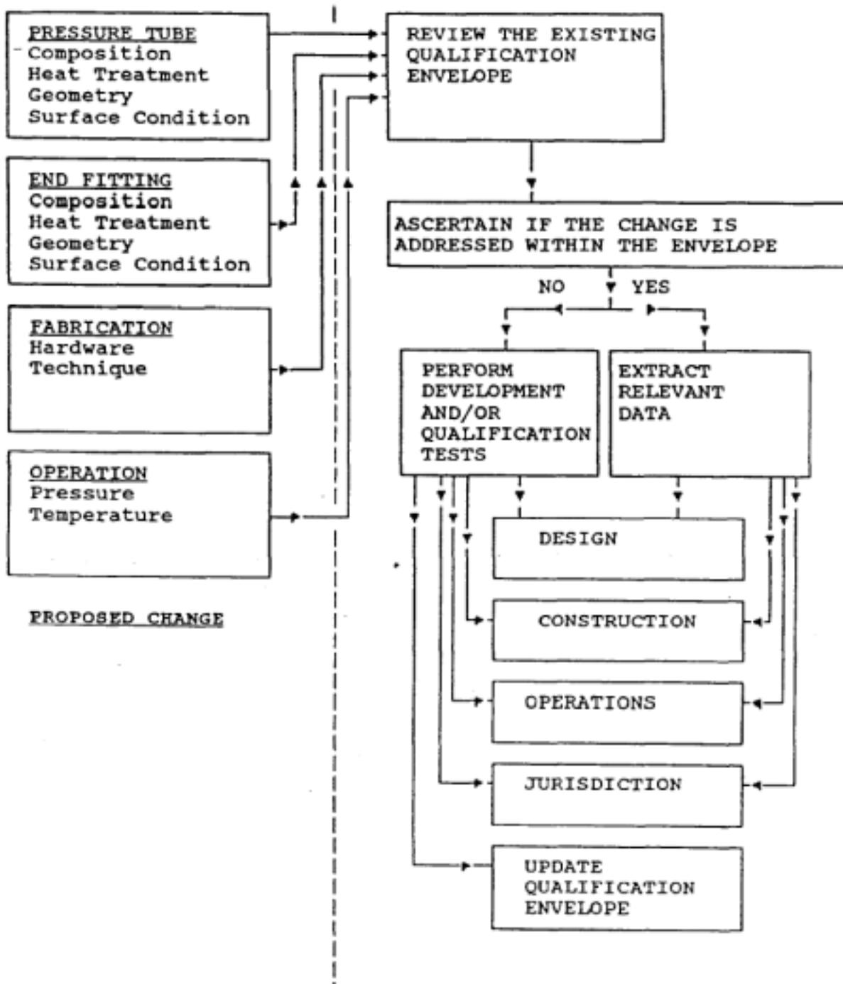
Figure 7-2 Qualification Process for Changes to Rolled Joint
