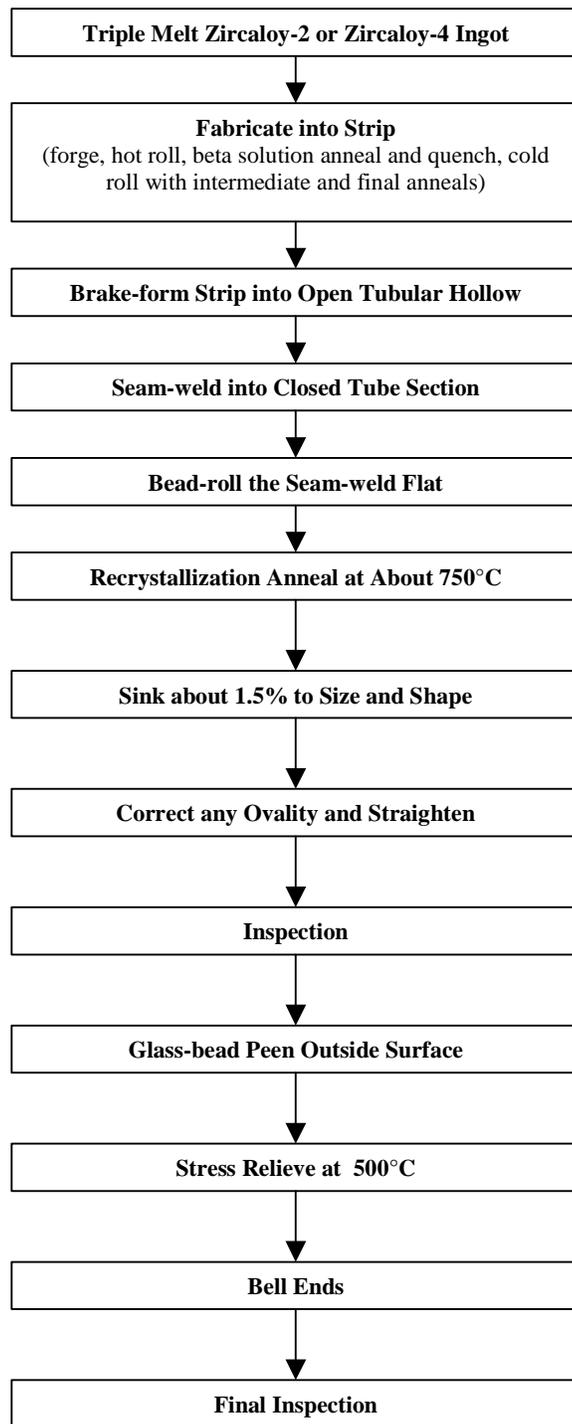
**Figure 16-1 Simplified Seam Welded Calandria Tube Fabrication Flow Chart**
