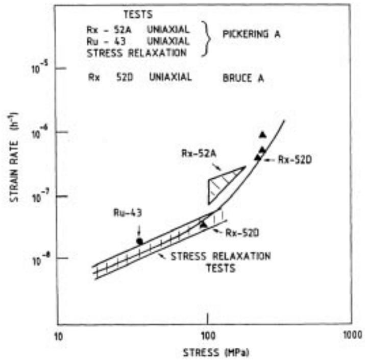
Figure 16-5 The In-Reactor Creep of Calandria Tube Material (Longitudinal Direction) at 50°C, and Neutron Flux of  $2 \times 10^{17} \text{ n/m}^2\cdot\text{s}$   $E > 1.0 \text{ MeV}$ , as a Function of Stress
