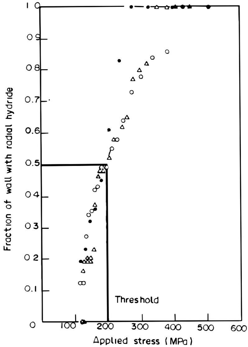
Figure 10-13 Hydride Morphology and Applied Stress for Zr-2.5Nb Material [10.21]
