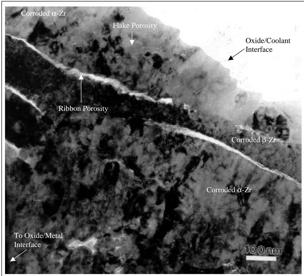
**Figure 9-10 Oxide Cross-Section Showing Flake Porosity along Edge of Columnar Oxide Grain Boundary and Ribbon Porosity along a Corroded  $\alpha/\beta$  Zr-Grain Boundary**
