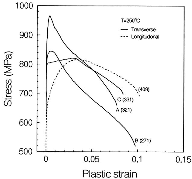
(Values in parentheses indicate the tube number of a particular specimen.)
