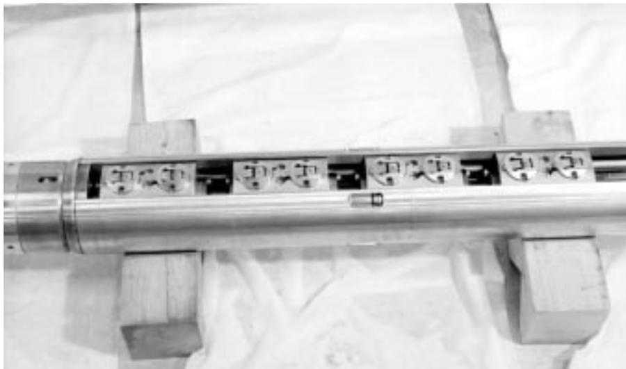
**Figure 11-7 The AECL Multi-Head Sampling Tool Showing the Four Sampling Heads in the Main Module at the End of the Tool. The module to the left houses the actuator, control mechanisms and connectors.**
