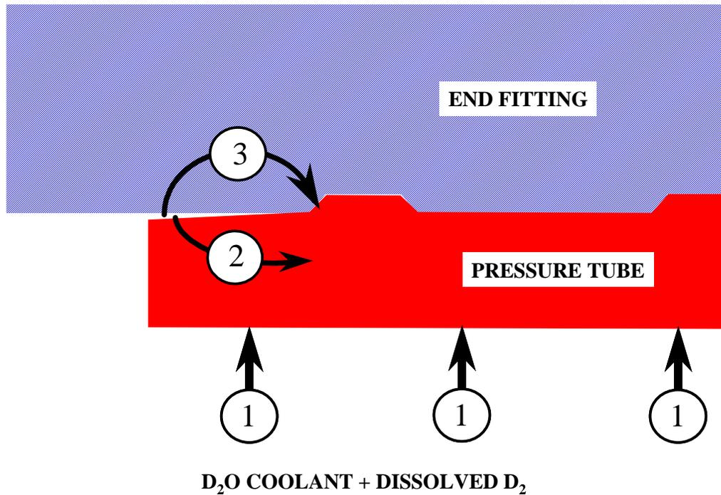
**Figure 9-11 A Schematic of the Pressure Tube Rolled Joint Showing the Main Routes of Deuterium Ingress into the Pressure Tube**
