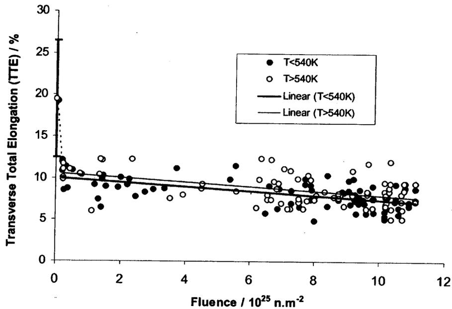
(Tested at 250°C at a strain rate of 10<sup>-3</sup>/s)
