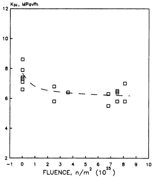
Figure 12-4 Effect of Irradiation Fluence on  $K_{IH}$  [12.8]
