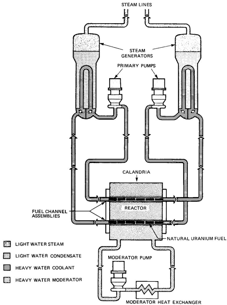
**Figure 1-4 CANDU Reactor Simplified Flow Diagram. In ACR the coolant is light water and the fuel is SEU.**
