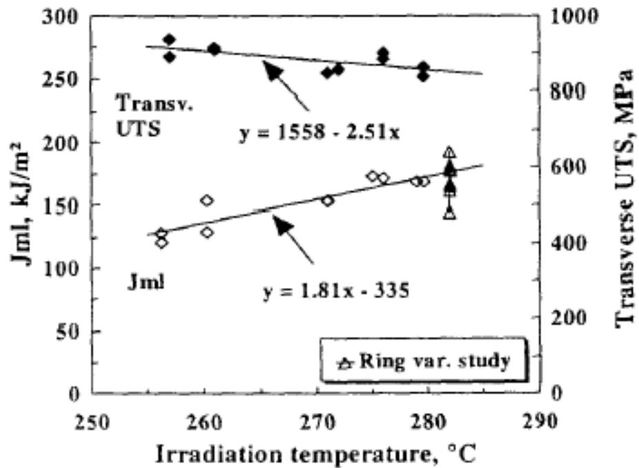
Figure 10-8 Variation in Transverse UTS and  $J_{ml}$  at 250°C with Irradiation Temperature [10.9]
