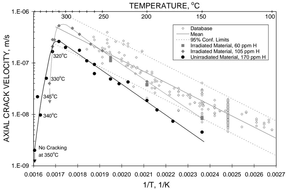
**Figure 12-7 Effect of Test Temperature on DHCV for Irradiated Material [12.4]**
