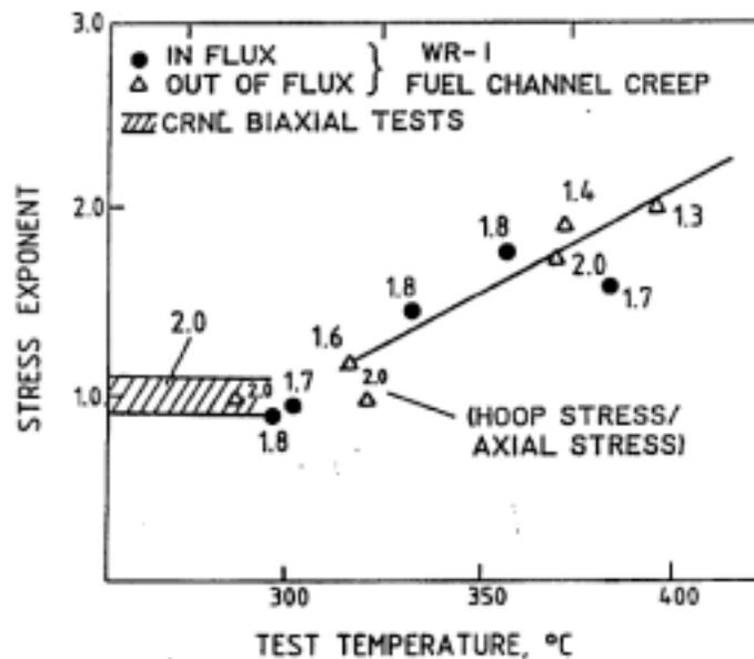
Figure 8-6 Effect of Temperature on the Stress Dependence of Creep of Cold-worked Zr-2.5Nb Pressure Tubes (from [8.10])
