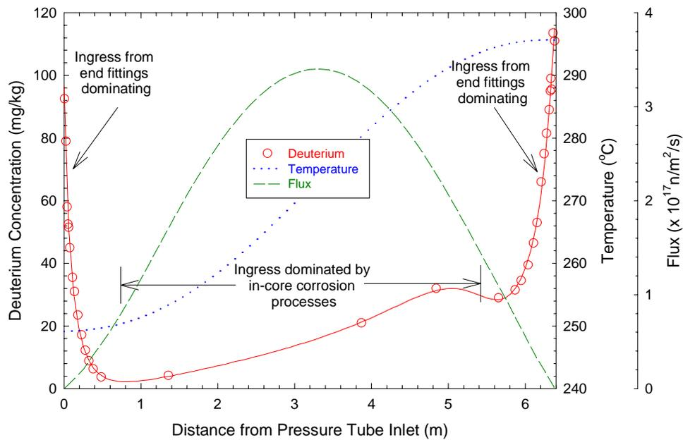
**Figure 9-2 A Typical Deuterium Concentration Profile along a Pressure Tube in a CANDU Reactor (after 14 EFPY of Operation). The flux and temperature profiles along the pressure tube are also shown.**
