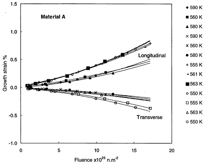
**Figure 8-13 Irradiation Growth of Longitudinal and Transverse Specimens of a Darlington Tube Irradiated in Trillium 2 and 3 in Osiris**
