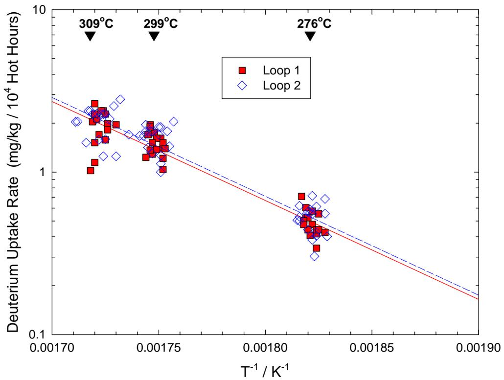
**Figure 9-5 An Arrhenius Plot of the Deuterium Uptake for Pressure Tubes in a CANDU 6 Reactor**
