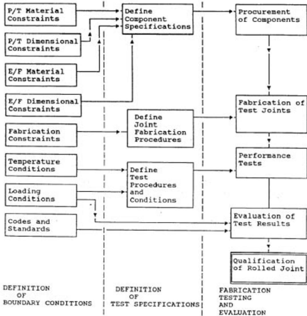
Figure 7-3 Stages in a Rolled Joint Test Program
