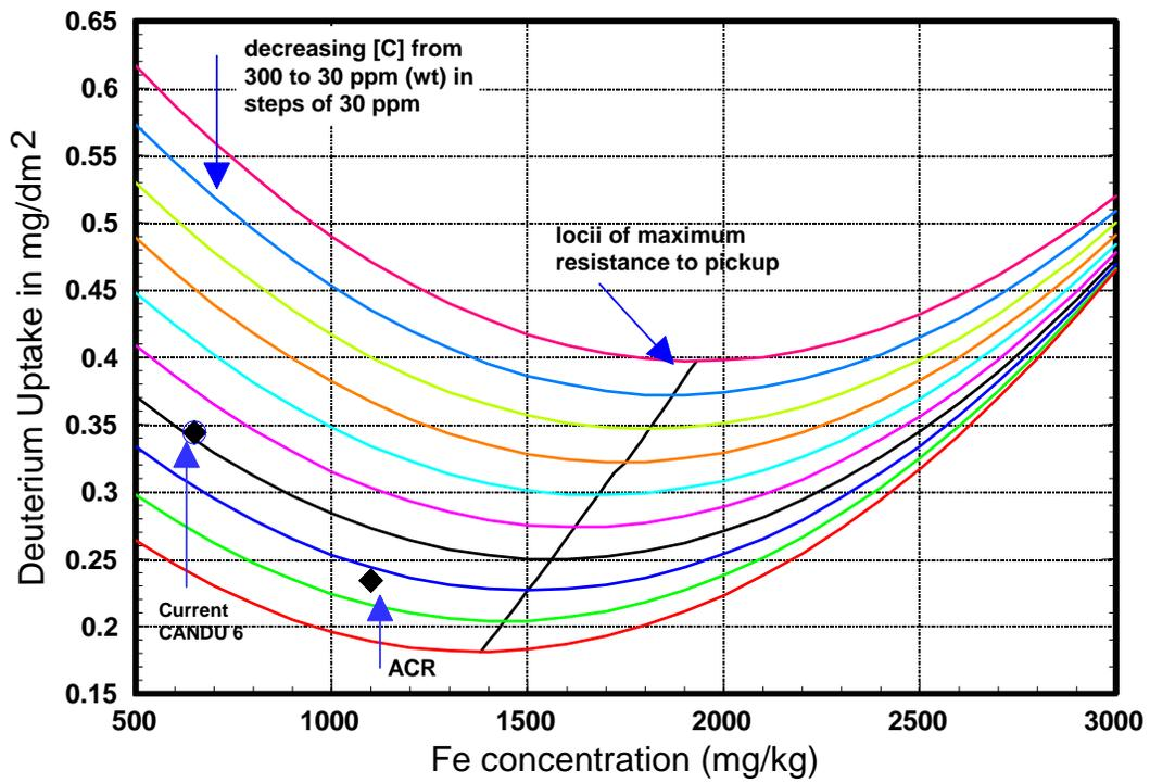
**Figure 9-9 Deuterium Uptake Curves as a Function of Iron and Carbon Concentrations in Zr-2.5Nb Drop Castings Corroded In-flux for 450 Days at 325°C in D<sub>2</sub>O**
