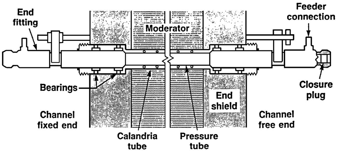
Figure 3-1 Schematic of a Fuel Channel in a CANDU Reactor
