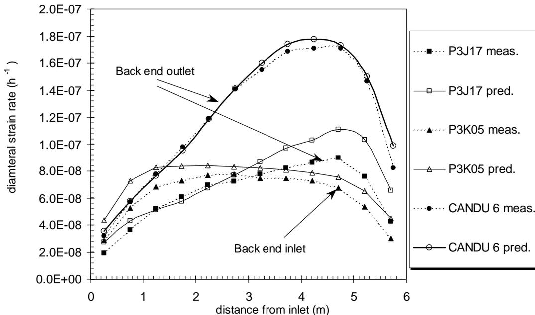
**Figure 8-16 Comparison of Measured and Predicted Transverse Strain Rates for the Axial Profiles of Pressure Tubes in Pickering Unit 3 and a CANDU 6 Reactor. Note that one of the Pickering 3 tubes and the CANDU 6 tubes have the back in the outlet, while the other Pickering 3 tube has the back end in the inlet.**
