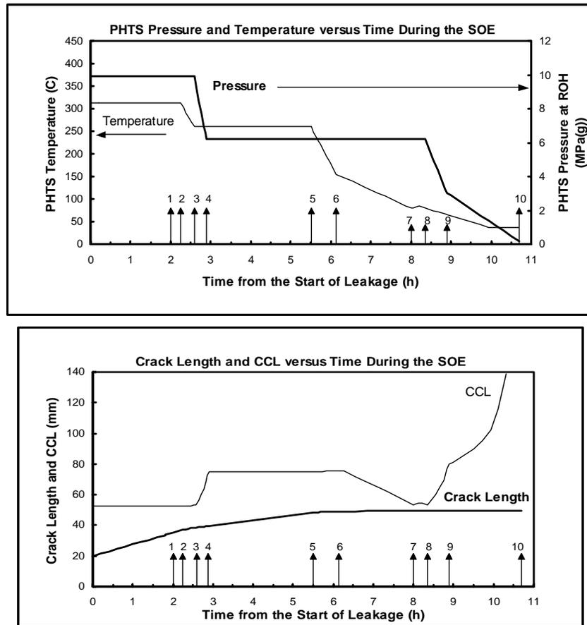
**Figure 12-8 Description of Events, Actions and Crack Length Development<sup>5</sup>**
