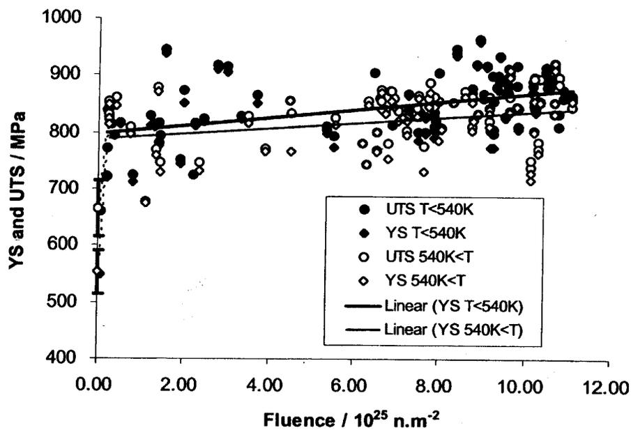
(Tested at 250°C at a strain rate of  $10^{-3}/s$ ).
