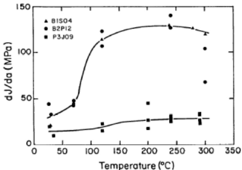
Figure 10-15 Effect of Test Temperature on the Crack Growth Toughness of Irradiated Zr-2.5Nb Pressure Tube Materials with High (P3J09) and Low (all others) Cl Concentrations [10.11]
