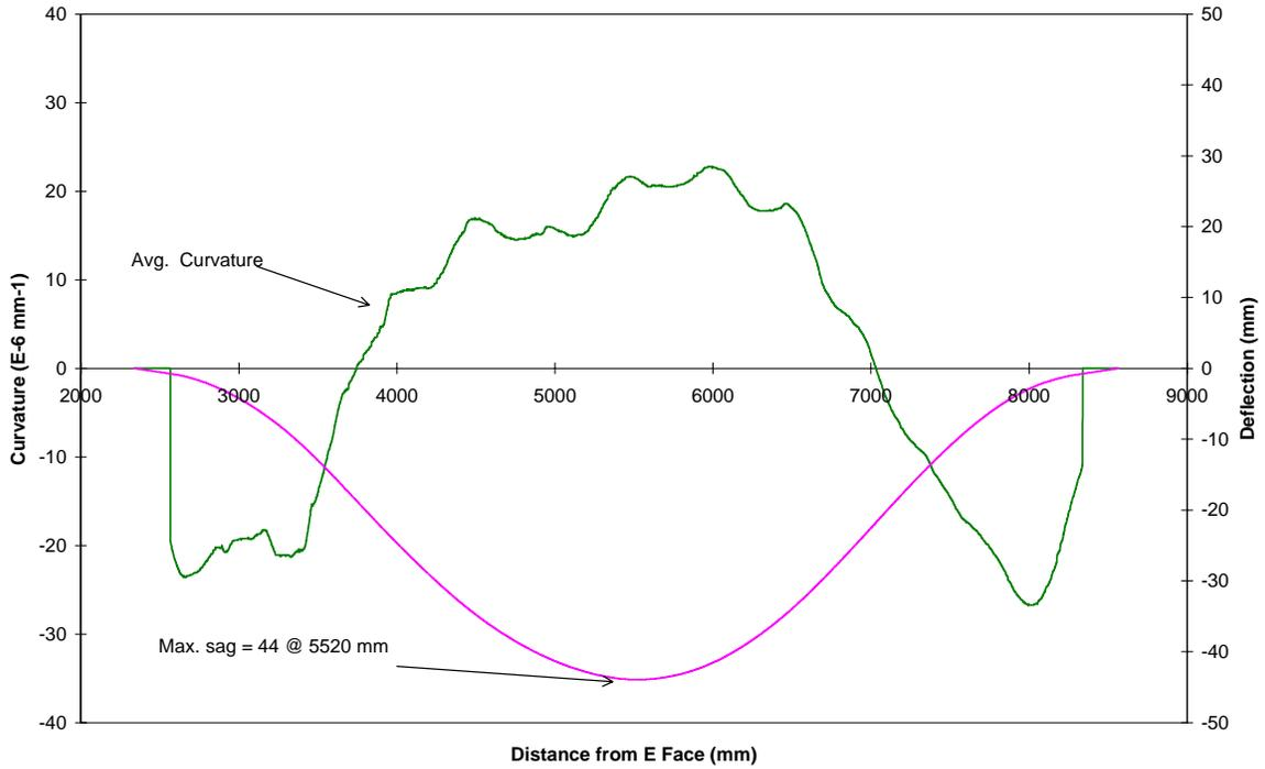
**Figure 11-10 Average Curvature and the Derived Sag Profile of a Fuel Channel after about 100,000 Hours of Reactor Operation**
