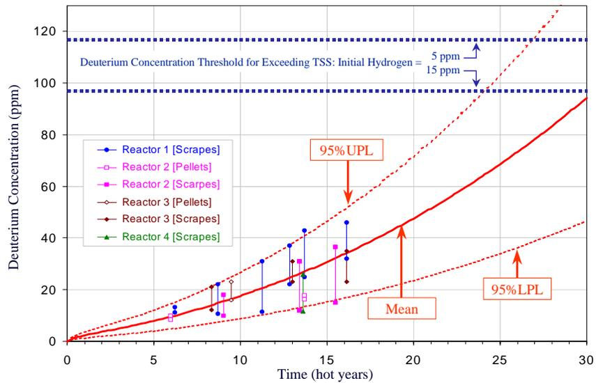
**Figure 9-8 Predicted and Measured Deuterium Uptake as a Function of Time at the Outlet End [T=307°C, Flux=2.0x10<sup>17</sup> n/m<sup>2</sup>.s]**
