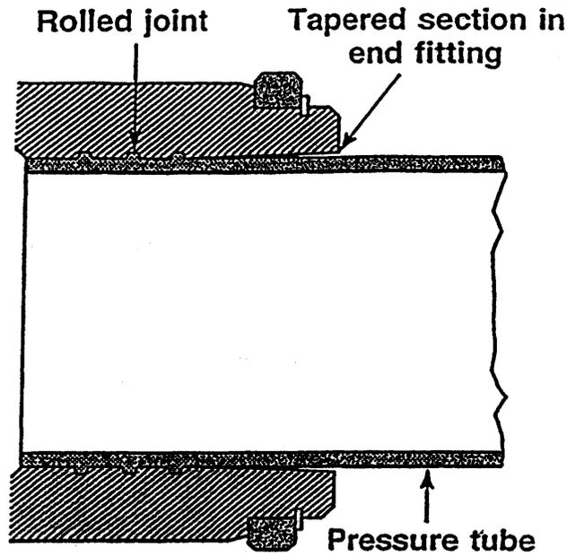
Figure 3-3 Typical Pressure Tube to End Fitting Rolled Joint
