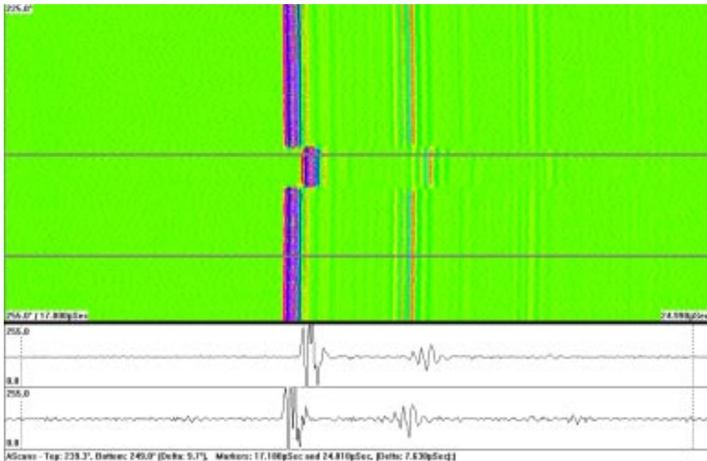
**Figure 11-2 Ultrasonic B-Scan (top) and the Corresponding A-Scans (Bottom) of a 0.15 mm Deep by 3 mm Wide Notch in a Pressure Tube**
