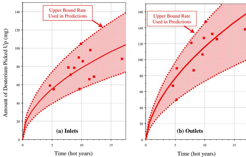
**Figure 9-13 Amount of Deuterium Picked Up at the Rolled as a Function of Time for Removed Pressure Tubes (Solid Squares). The solid curve is the best fit assuming a declining ingress rate and the dashed curves are the upper and lower bounds.**
