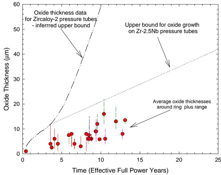
**Figure 9-4 The Measured Oxide Thickness on the Inside of Zr-2.5Nb Surveillance Pressure Tubes near the Outlet of the Fuel Channel as a Function of Time<sup>14</sup>**
