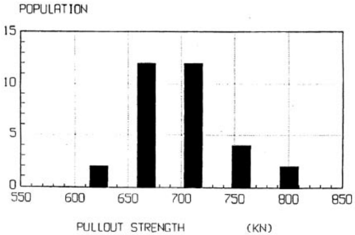
**Figure 7-6 A Histogram of Hot (300°C), Pressurized, Pull Out Test Results**
