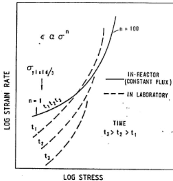
Figure 8-3 Stress Dependence of In-reactor Creep of Zirconium Alloys at ~ 300°C (Schematic)
