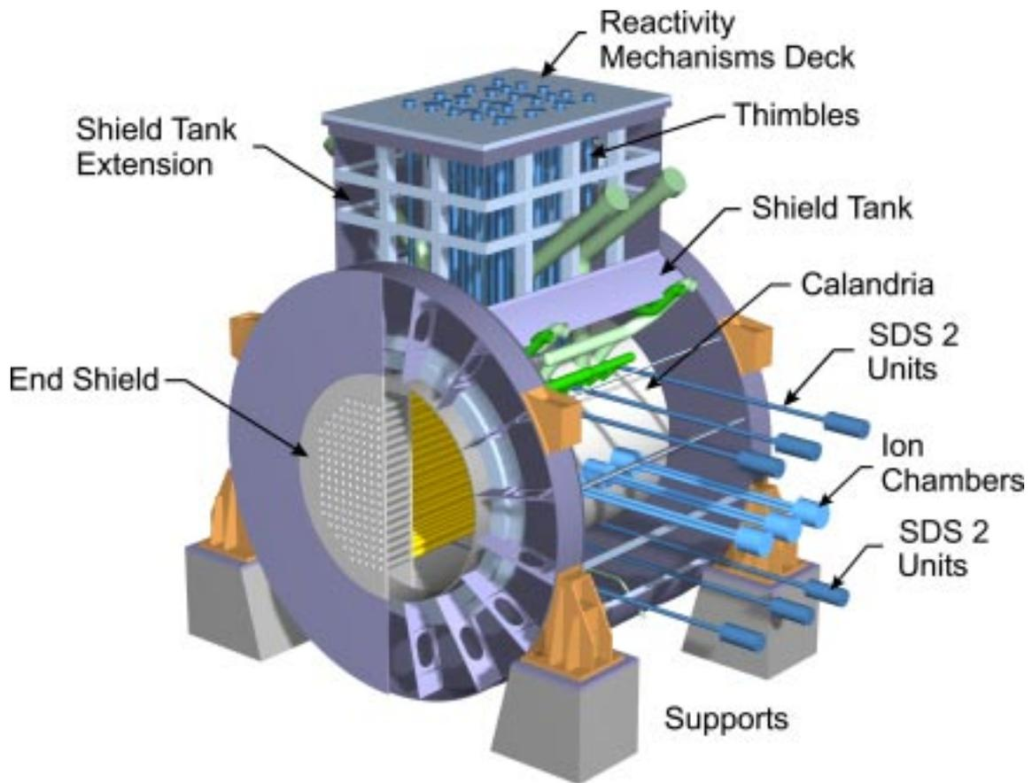
**Figure 1-2 The ACR Calandria and Shield Tank Assembly**
