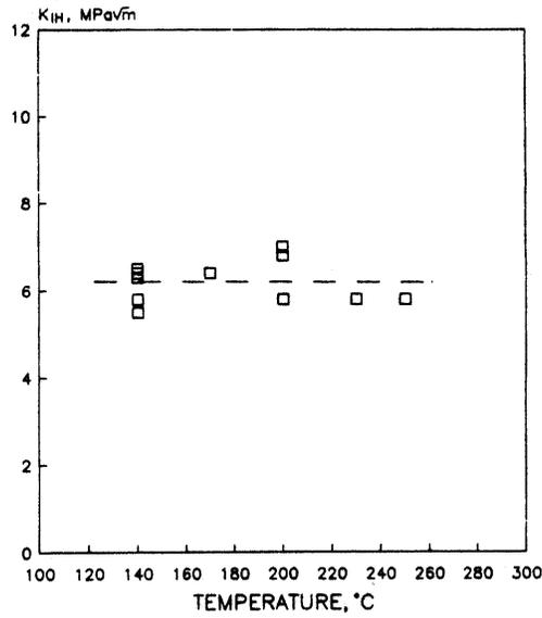
Figure 12-3 Effect of Test Temperature on  $K_{IH}$  [12.8]
