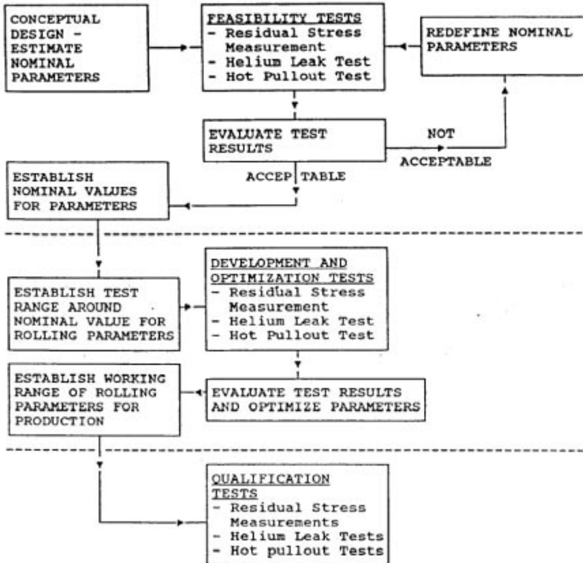
Figure 7-4 Three Stages of Rolled Joint Experimental Design
