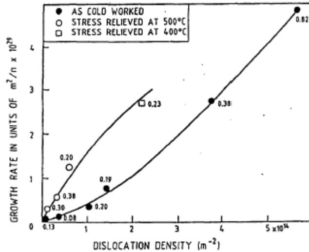
**Figure 8-15 Steady-state Irradiation of Zircaloy-2 at 60°C as a Function of Dislocation Density. The numbers beside each data point denote the ratio of  $\langle c \rangle$  to  $\langle a \rangle$  component dislocations.**
