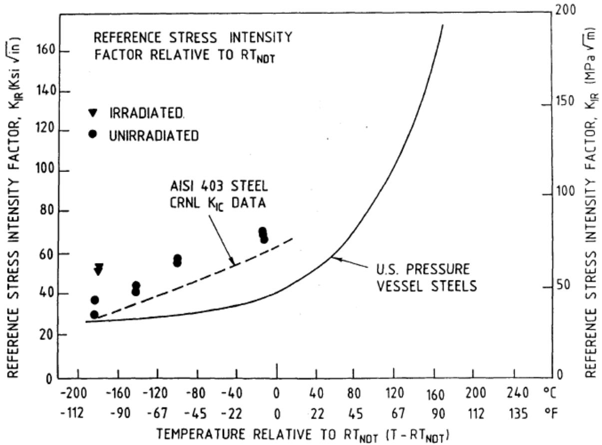
**Figure 15-1 Effect of Fast Neutron Irradiation of the V-notch Charpy Impact Properties of AISI 403 Heat A**
