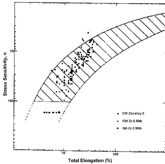
**Figure 8–19 A Plot of the Stress Exponent  $n$  against Total Elongation at Failure for Zirconium Alloys at 300 to 450°C. The hatched band is for the results from tensile tests on many other alloys (from [8.47]).**
