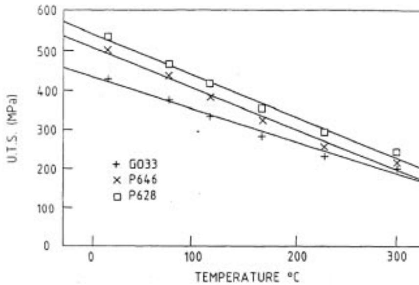
**Figure 16-2 The Ultimate Tensile Strength in the Longitudinal Direction as a Function of Temperature of Three Typical Calandria Tubes. The tests were done with a controlled strain rate of  $10^{-3}$ s $^{-1}$ .**
