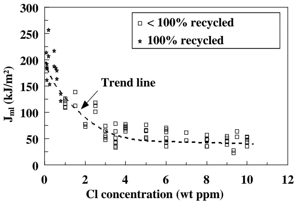
Figure 10-12 J at Maximum load, J<sub>m1</sub>, from Curved Compact Specimens of Irradiated Material Tested at 250°C Versus Cl Concentration [10.9]
