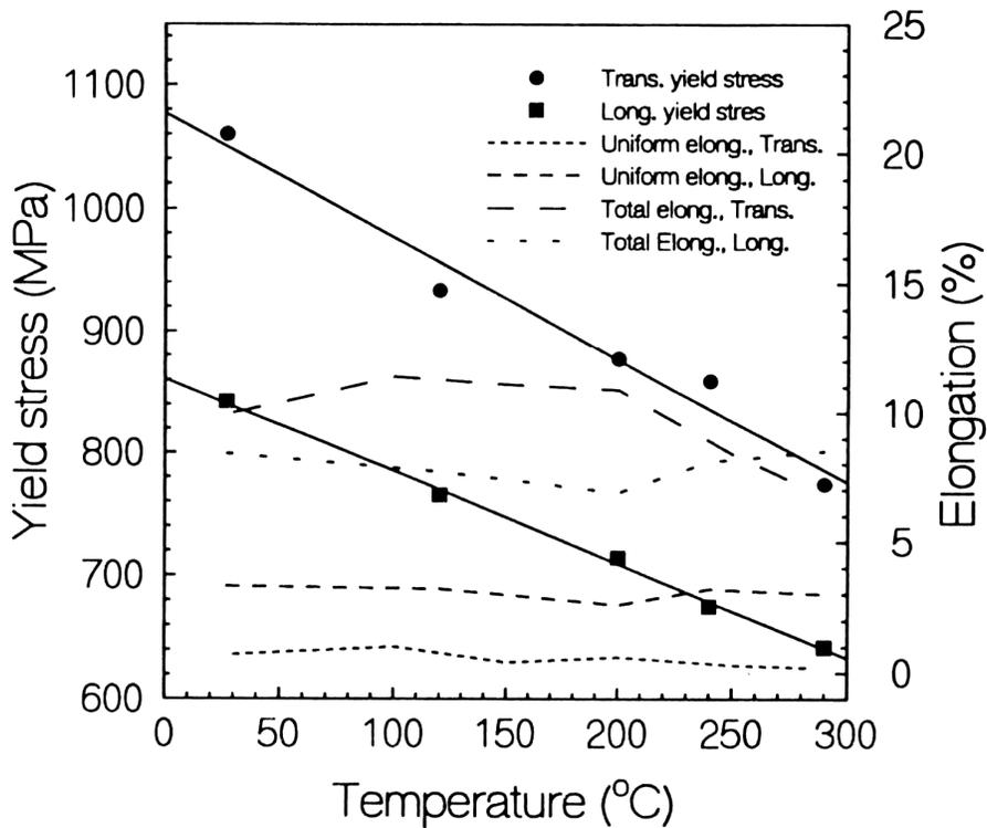
**Figure 10-10 Effect of Temperature on the Yield Stress and Uniform and Total Elongation for Transverse and Longitudinal Tensile Specimens (Tube 547) [10.8]**
