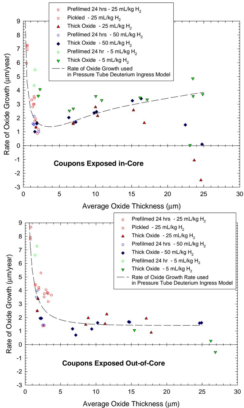
**Figure 9-6 The Rate of Oxide Growth on Zr-2.5Nb Coupons as a Function of Surface Oxide Thickness. Coupons exposed at ~300°C in light water U-2 Loop, NRU Reactor, at a pH ~10.2. The dissolved hydrogen concentration was either 5, 25 or 50 ml/kg. Oxide growth rates near or below zero are indicative of the spalling of the surface oxide from the coupon.**
