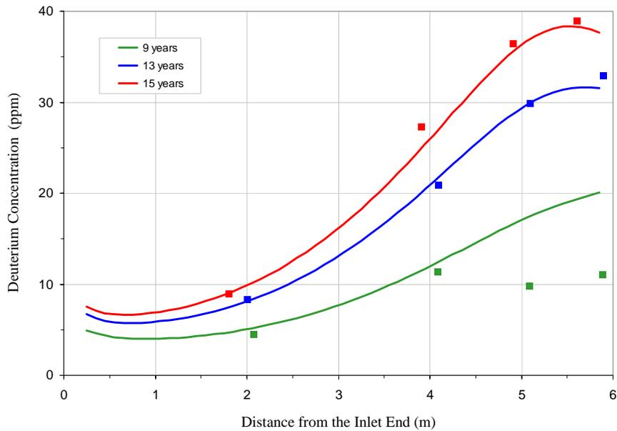
**Figure 9-7 Predicted and Measured Deuterium Concentration along a Pressure Tube as a Function of Time. Model predictions are normalized to the 13 Hot Year data (the 9 Hot Year data at > 5 m are considered erroneous).**
