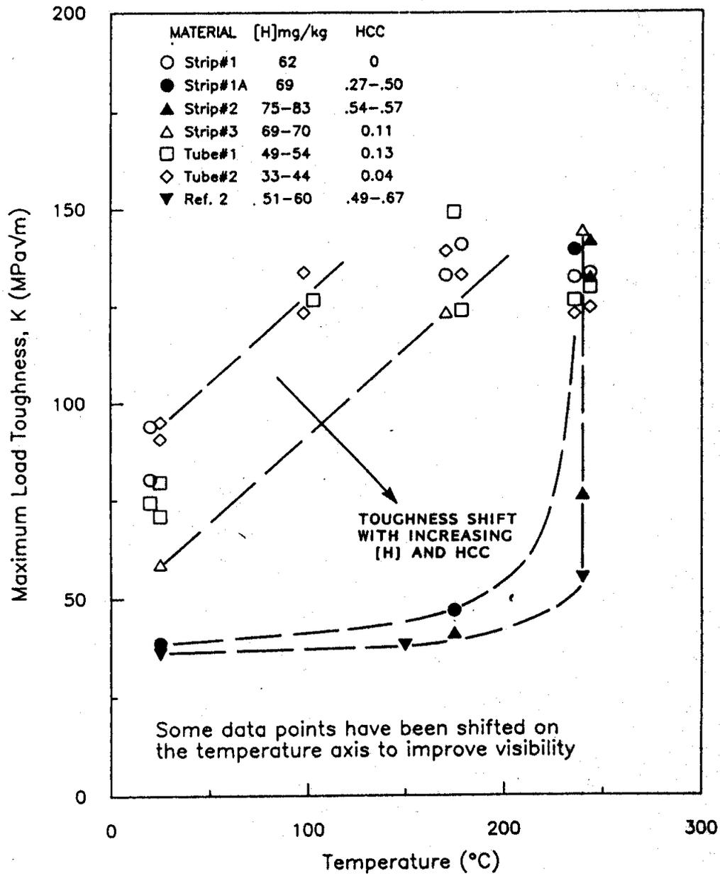
Figure 10-14 Fracture Toughness Versus Temperature for Unirradiated Zr-2.5Nb with Various Hydride Morphologies [10.19]
