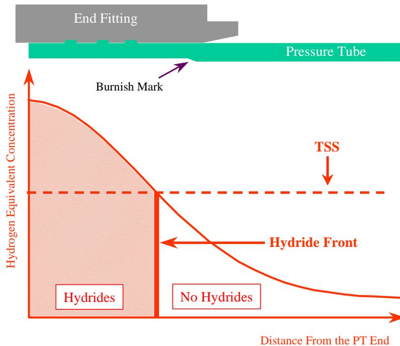
**Figure 9-14 Schematic of the Rolled Joint Showing the Hydrogen Equivalent Concentration along the Pressure Tube**
