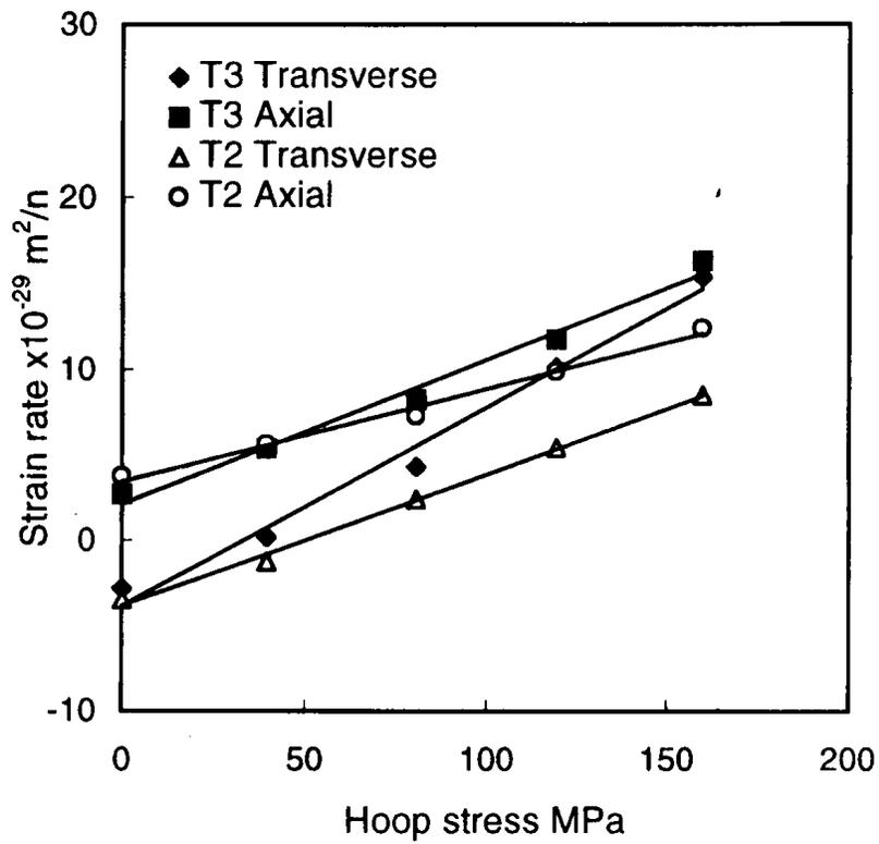
**Figure 8-4 Strain Rate as a Function of Hoop Stress for Internally Pressurized Capsules Irradiated in the Osiris Reactor (from [8.14])**
