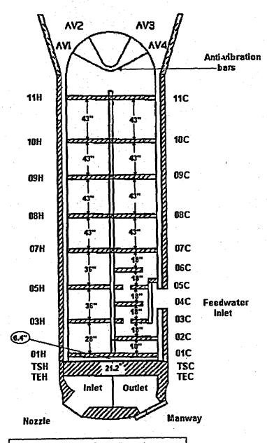
Note: Tube Support Plate dimensions are centerline to centerline.
