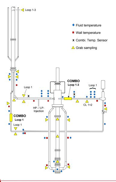
Continuous Measurement of Boron Concentration (COMBO)
