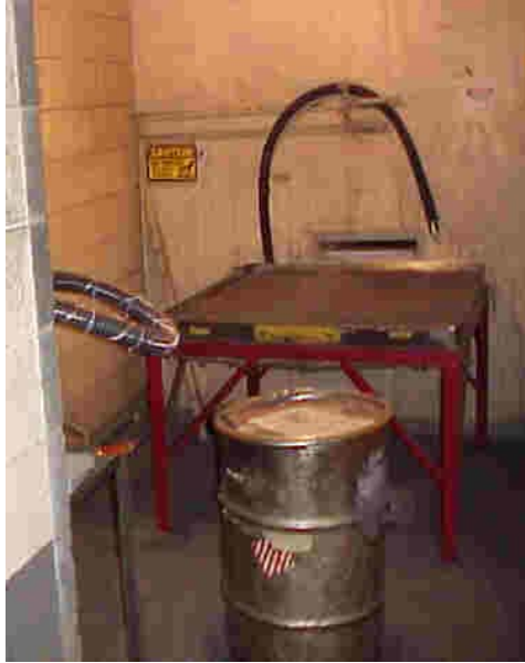
Figure 7. Slot hood, steam table and drum into which thorium-doped powder is collected.
