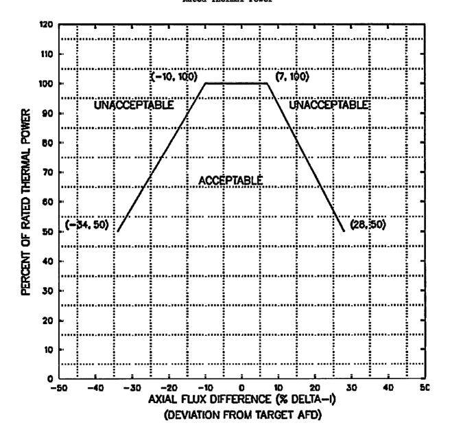
Note: At power levels less than HFP, the deviation is applied to the target AFD appropriate to that power level. The target AFD varies linearly between the HFP target and zero at zero power.
