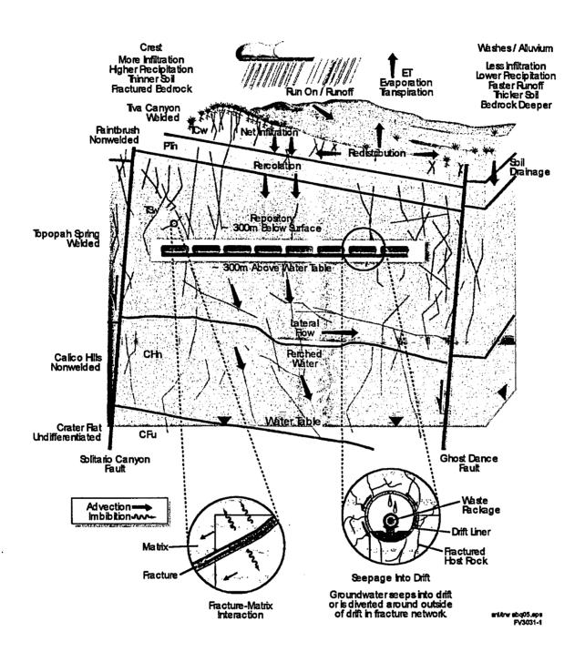
Figure 1. Schematic of a Repository in the Unsaturated Zone at Yucca Mountain
