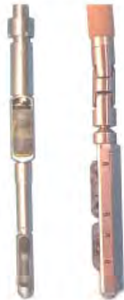
ET / UT probe for defect detection (left) UT pulse echo probe for socket weld inspection UT TOFD probe for defect sizing (right)
