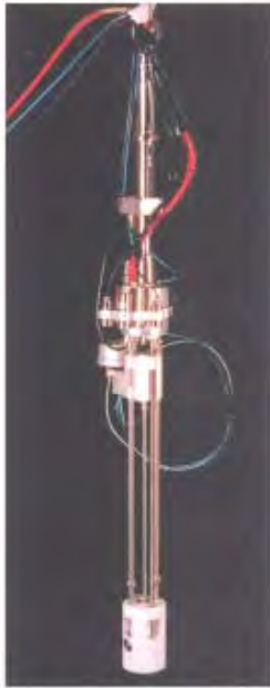
Bottom nozzle inspection manipulator
