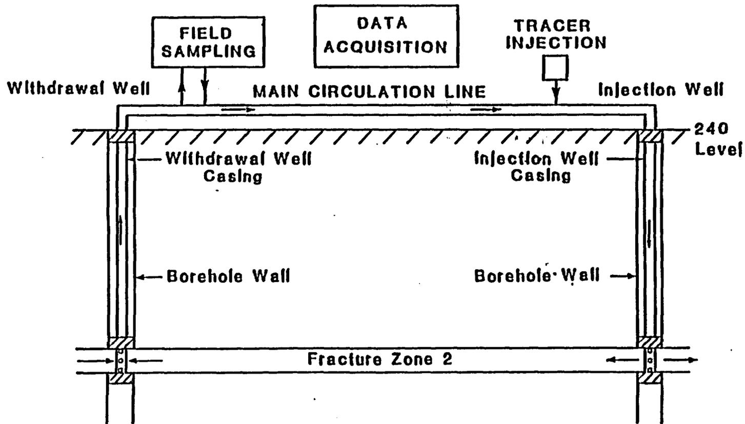
FIGURE 5: Schematic of Two-Well Recirculating Tracer Test
