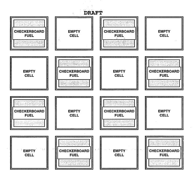
Checkerboard Fuel: Fuel which does <u>not</u> meet the minimum burnup requirements of Table 3.7.15-1. (Fuel which does meet the requirements of Table 3.7.15-1, or non-fuel components, or an empty location may be placed in checkerboard fuel locations as needed)
