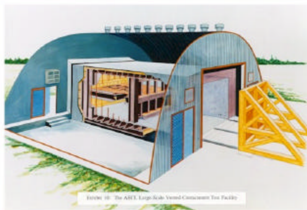
Figure 4. A Schematic of the Large-Scale Vented Combustion Test Facility
