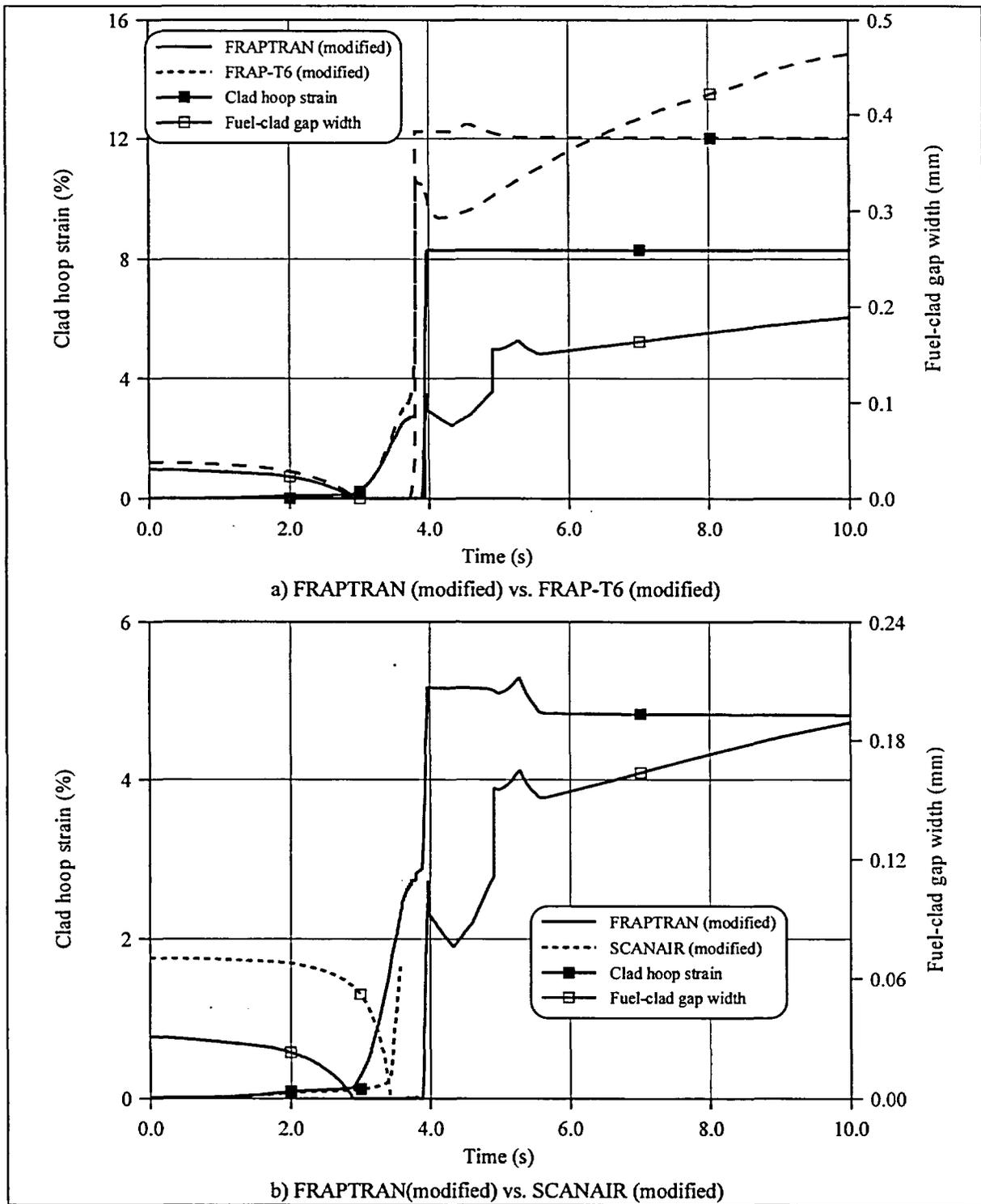
Fig. 17. Cladding hoop strains and gap widths vs. time calculated by modified FRAP-T6, SCANAIR and FRAPTRAN codes (H7T test case).
