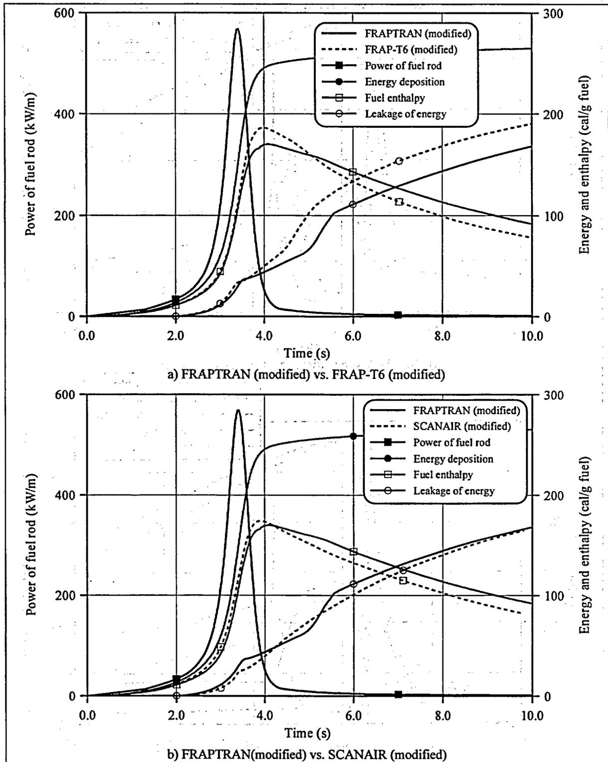
Fig. 14. Energy characteristics vs. time calculated by modified FRAP-T6, SCANAIR and FRAPTRAN codes (H7T test case).
