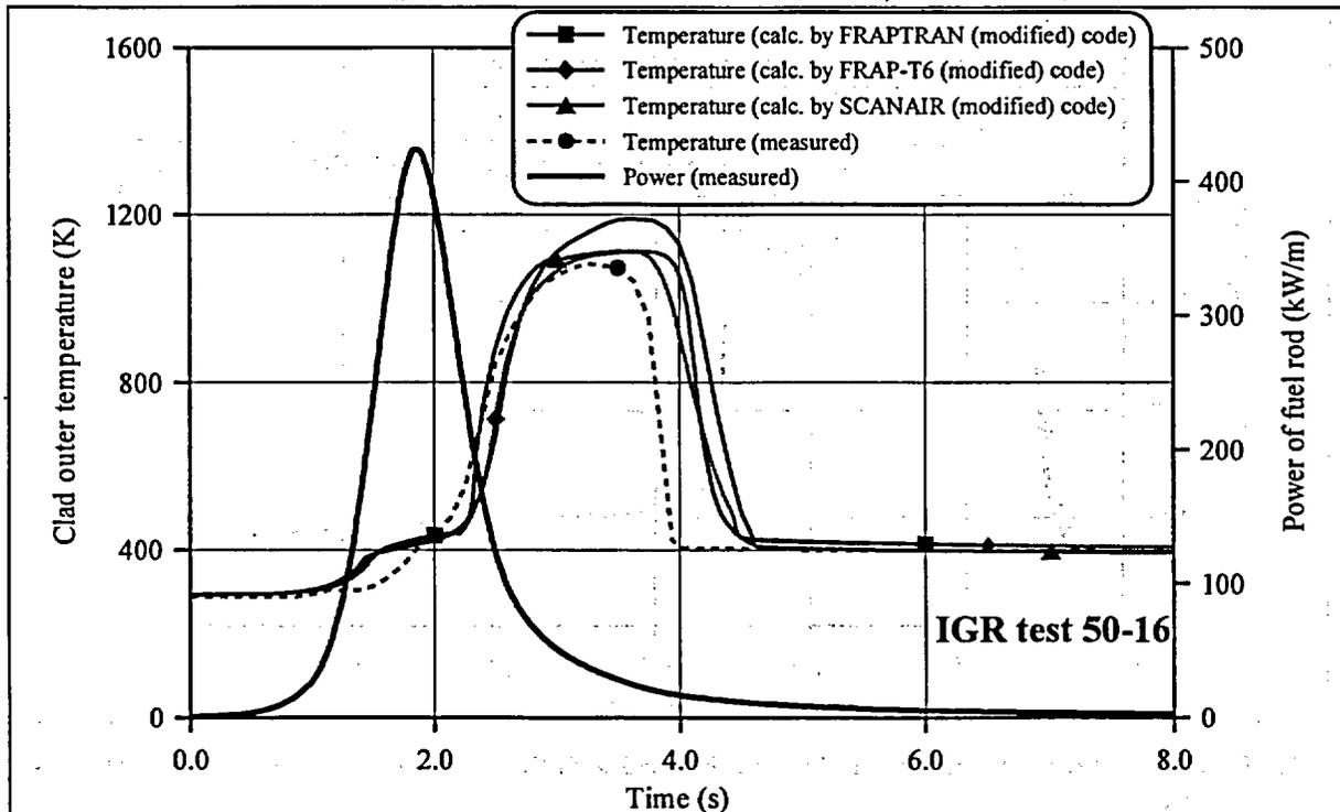
Fig. 6. Clad outer temperature in 50F-16 test: comparison between measured and calculated with FRAP-T6 (modified), SCANAIR (modified), and FRAPTRAN (modified) codes.
