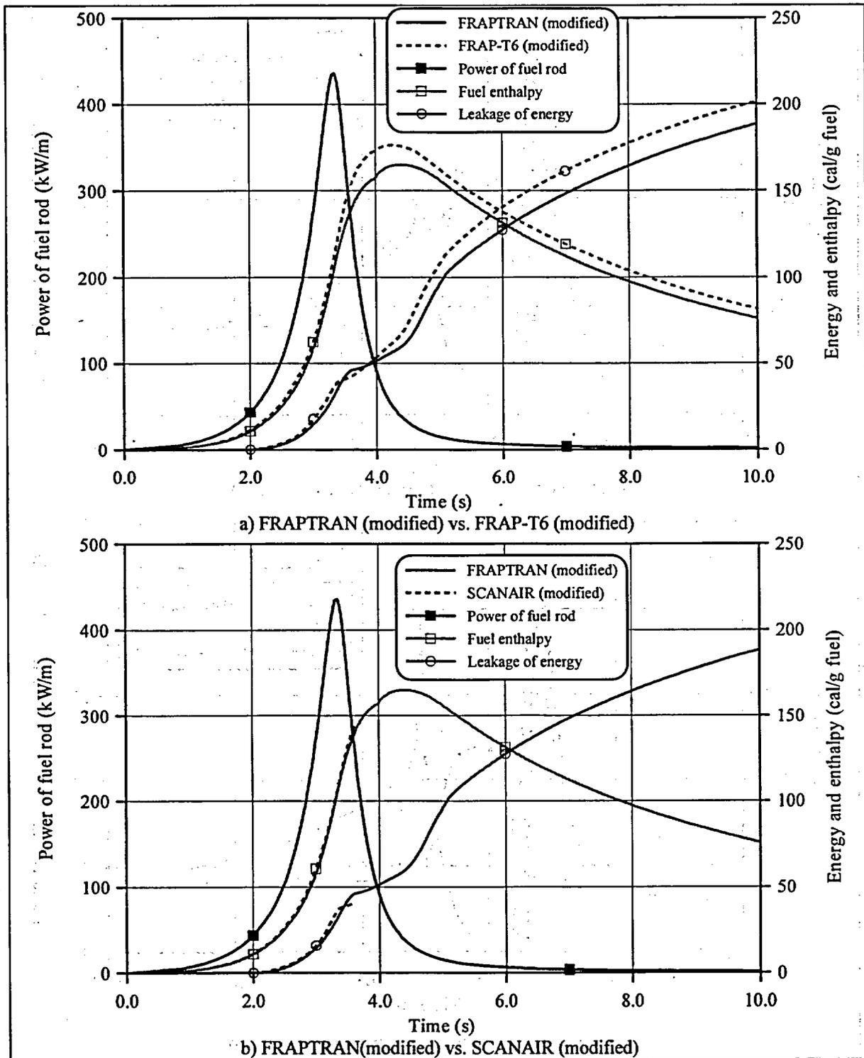
Fig. 10. Energy characteristics vs. time calculated by modified FRAP-T6, SCANAIR and FRAPTRAN codes (H5T test case).
