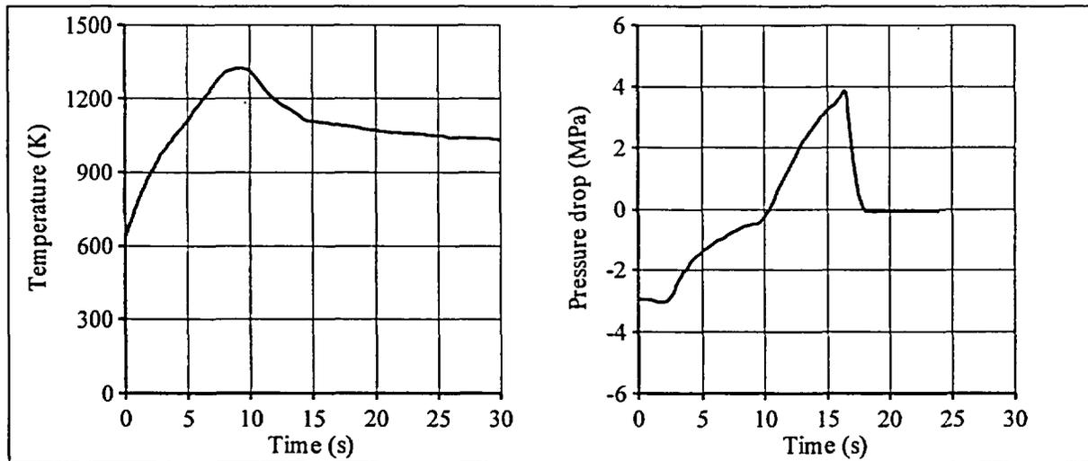
Fig. 26. Simulator cladding temperature and cladding pressure drop.
