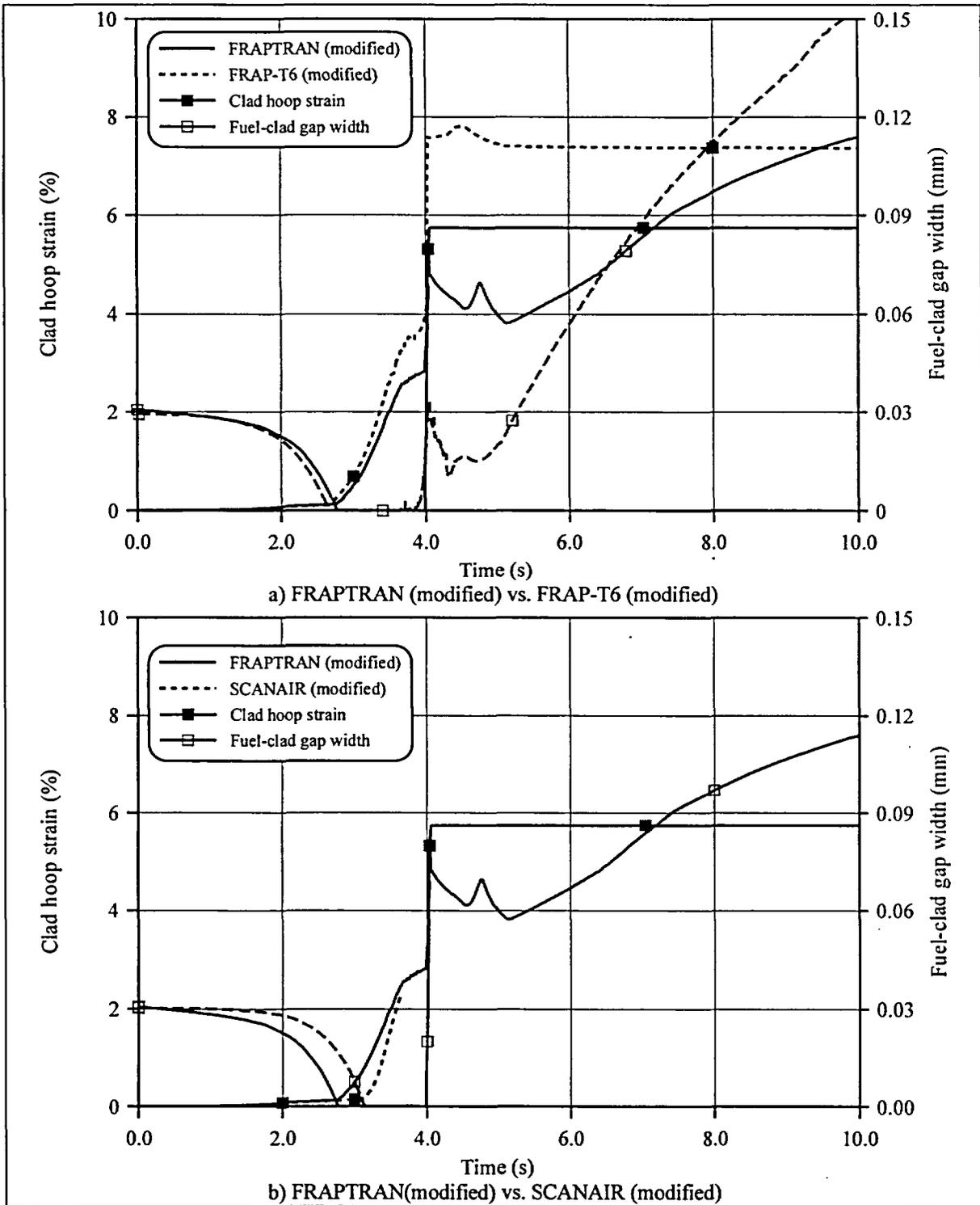
Fig. 13. Cladding hoop strains and gap widths vs. time calculated by modified FRAP-T6, SCANAIR and FRAPTRAN codes (HST test case).
