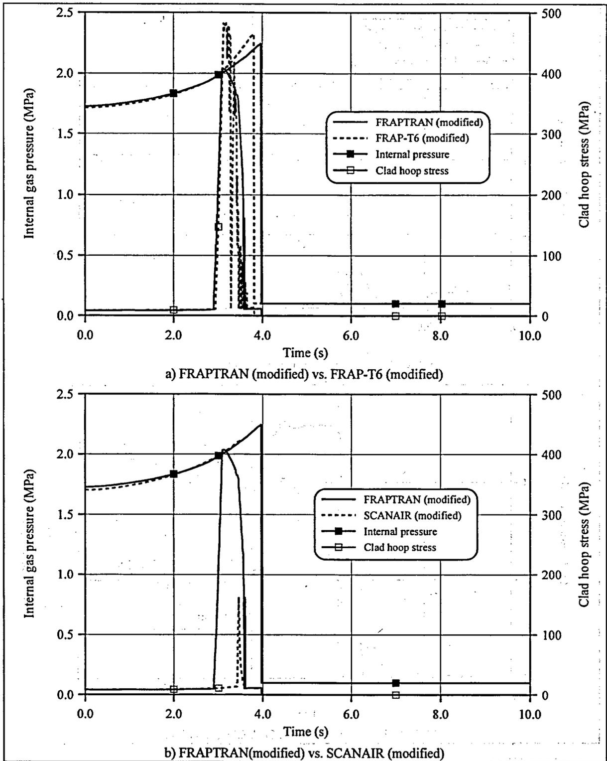
Fig. 16. Cladding hoop stresses and internal pressures vs. time calculated by modified FRAP-T6, SCANAIR and FRAPTRAN codes (H7T test case).
