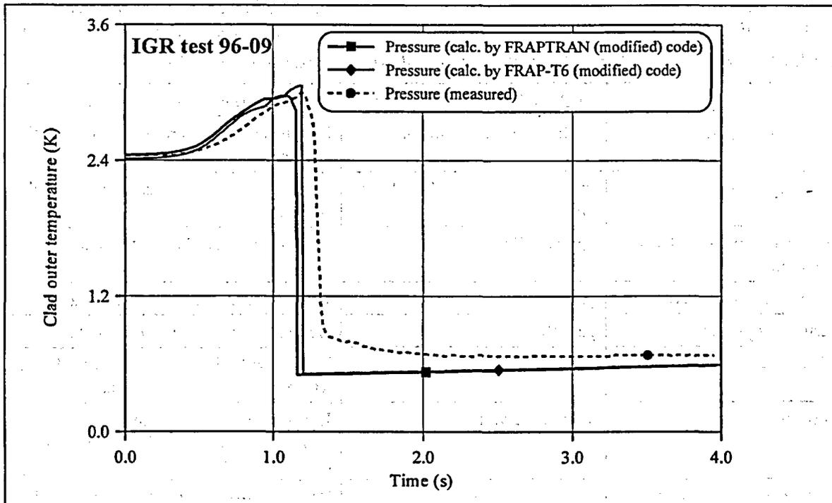
Fig. 9. Comparison of internal rod pressure in 96F-09 test, calculated with FRAP-T6 (modified) and FRAPTRAN (modified) codes.
