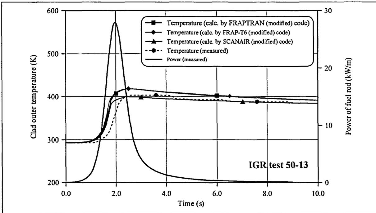
Fig. 4. Clad outer temperature in 50F-13 test: comparison between measured and calculated with FRAP-T6 (modified), SCANAIR (modified) and FRAPTRAN (modified) codes.
