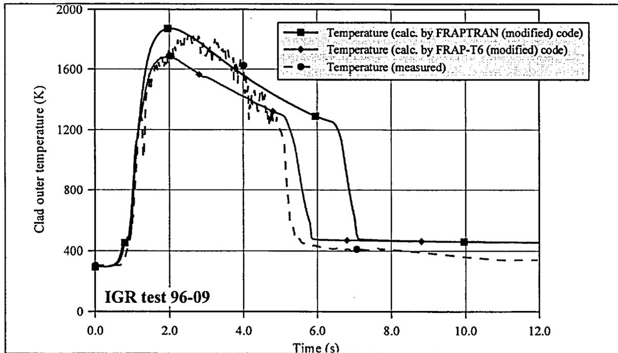
Fig. 8. Clad outer temperature in 96F-09 test calculated with Labuntzov post-CHF heat transfer.
