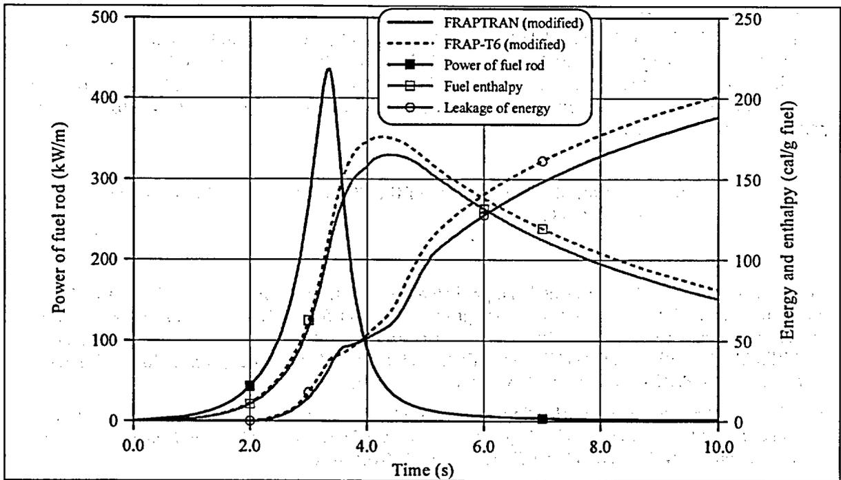
Fig. 23. Peak enthalpy calculated by FRAP-T6 (modified) and FRAPTRAN (modified).
