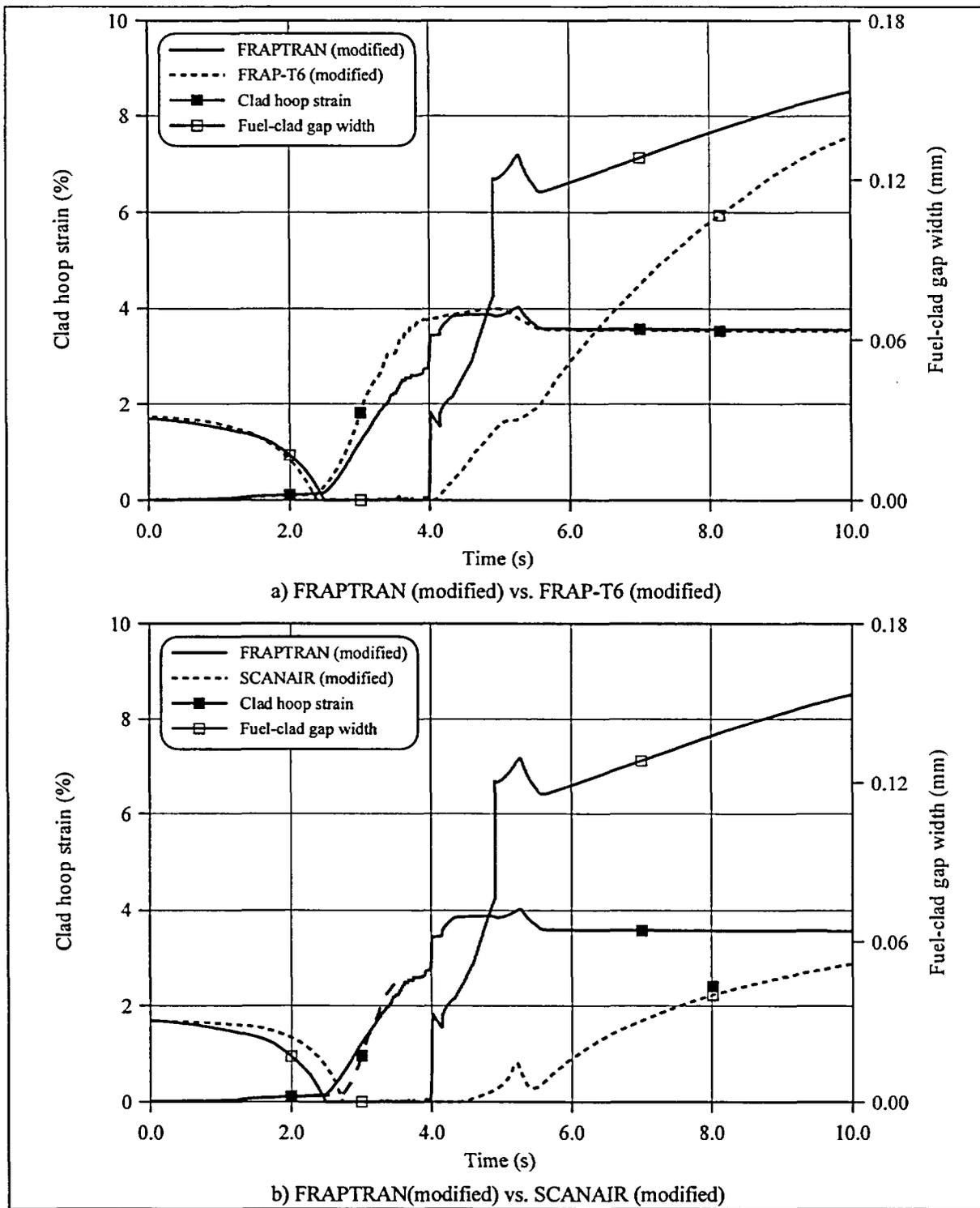
Fig. 21. Cladding hoop strains and gap widths vs. time calculated by modified FRAP-T6, SCANAIR and FRAPTRAN codes (H1T test case).
