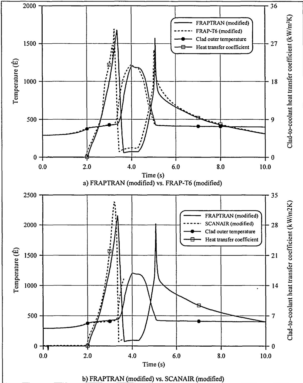
Fig. 11. Cladding temperatures and heat transfer coefficients vs. time calculated by modified FRAP-T6, SCANAIR and FRAPTRAN codes (H5T test case).
