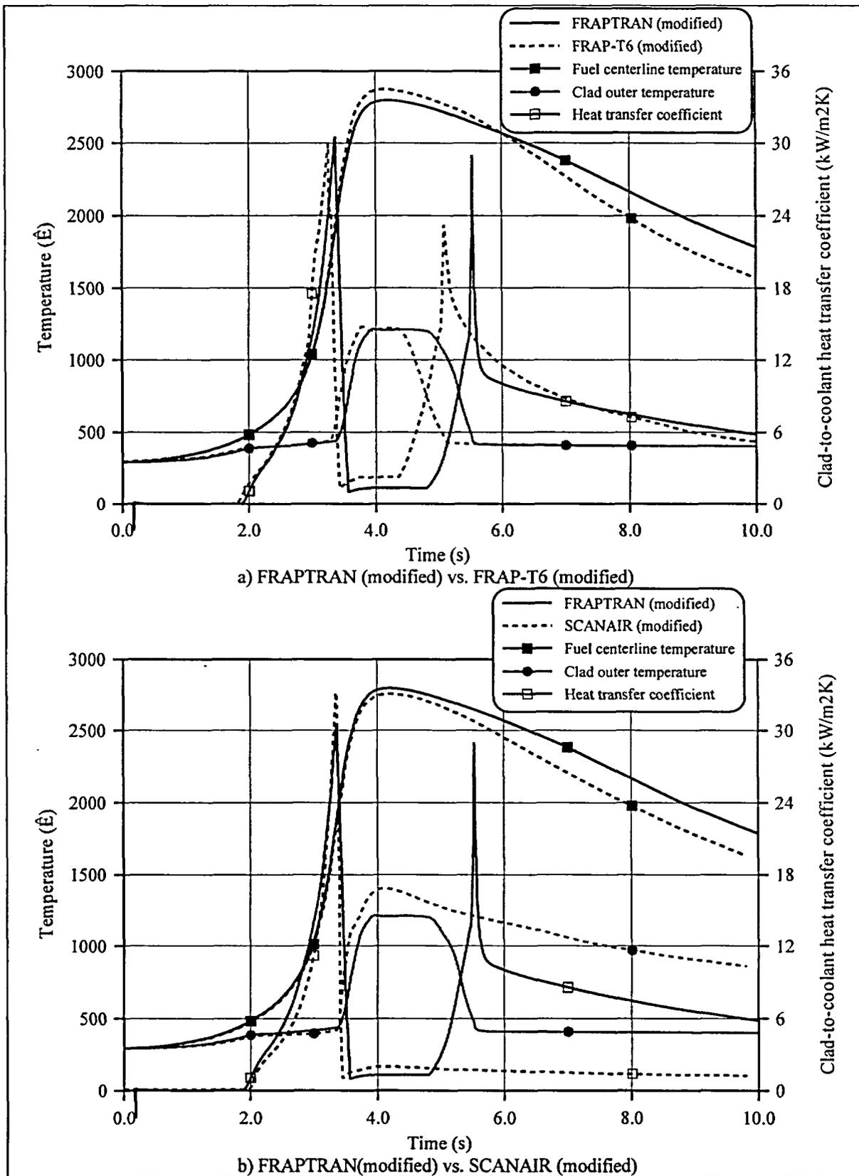
Fig. 15. Cladding temperatures and heat transfer coefficients vs. time calculated by modified FRAP-T6, SCANAIR and FRAPTRAN codes (H7T test case).
