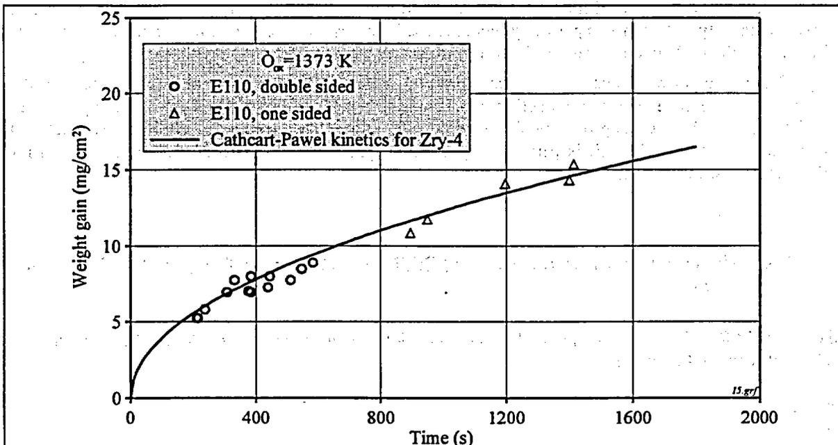
**Fig. 2. Comparison of test data on Zr-1%Nb steam oxidation with Cathcart-Pawel model predictions.**
