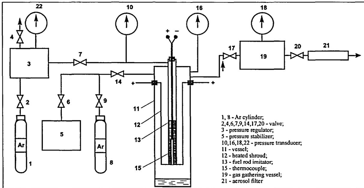
Fig. 25. Schematic diagram of electrically heated facility for studying the first stage of LOCA.
