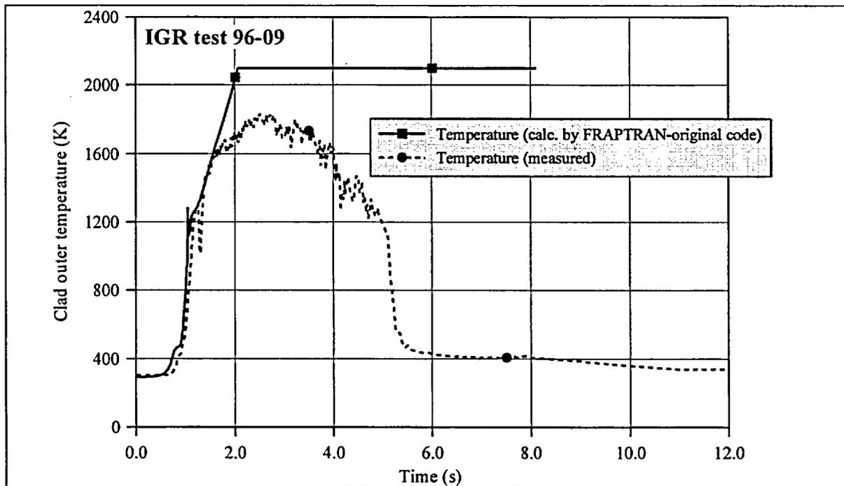
Fig. 7. Clad outer temperature in 96F-09 test calculated with Bromley-Pomerantz post-CHF heat transfer.
