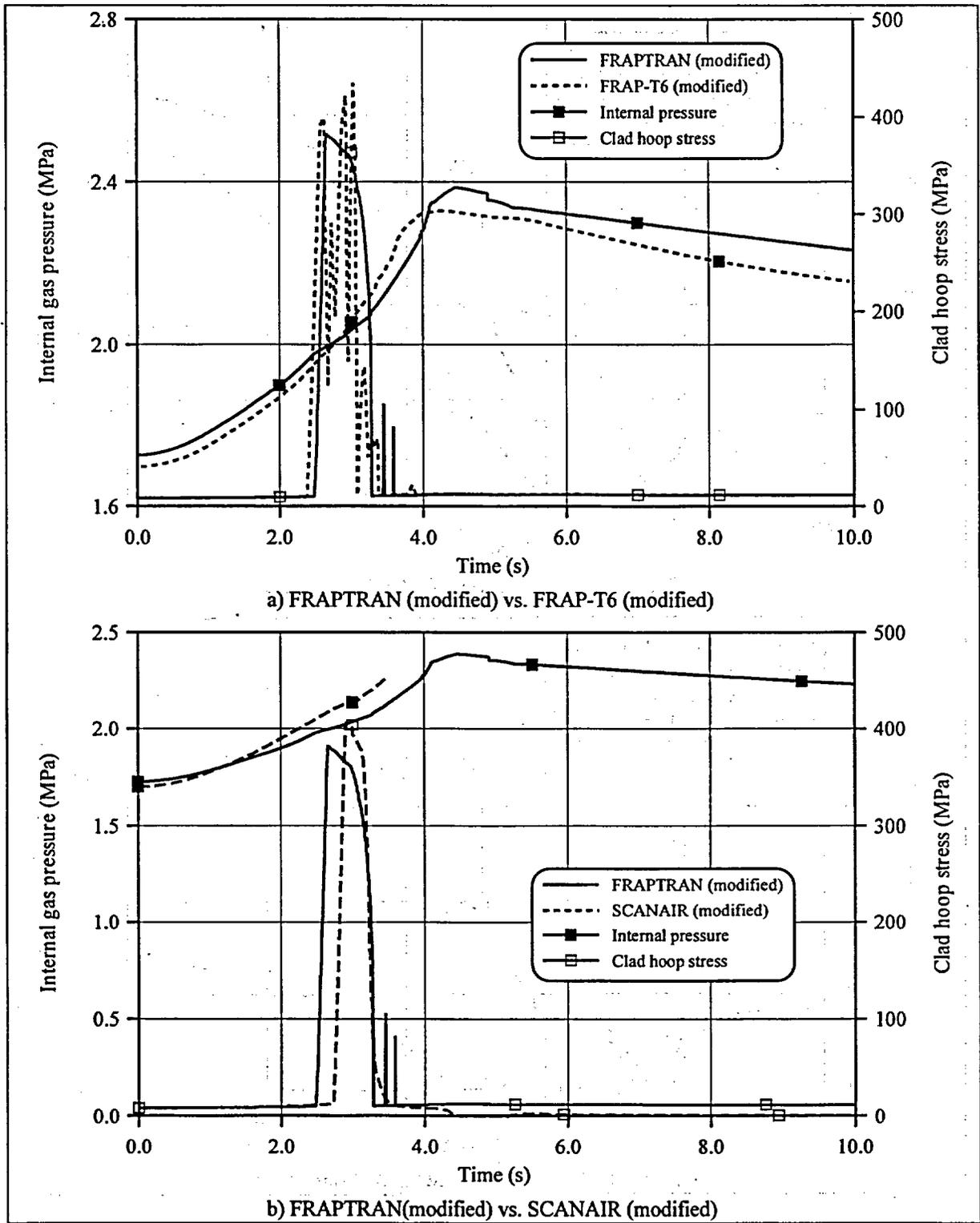
Fig. 20. Cladding hoop stresses and internal pressures vs. time calculated by modified FRAP-T6, SCANAIR and FRAPTRAN codes (HIT test case).
