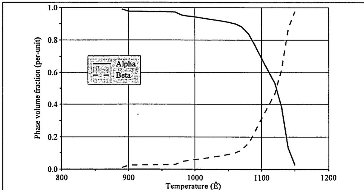
Fig. 1. Volumetric fractions of  $\alpha$  and  $\beta$ -phases depending on Zr-1%Nb alloy temperature [18].
