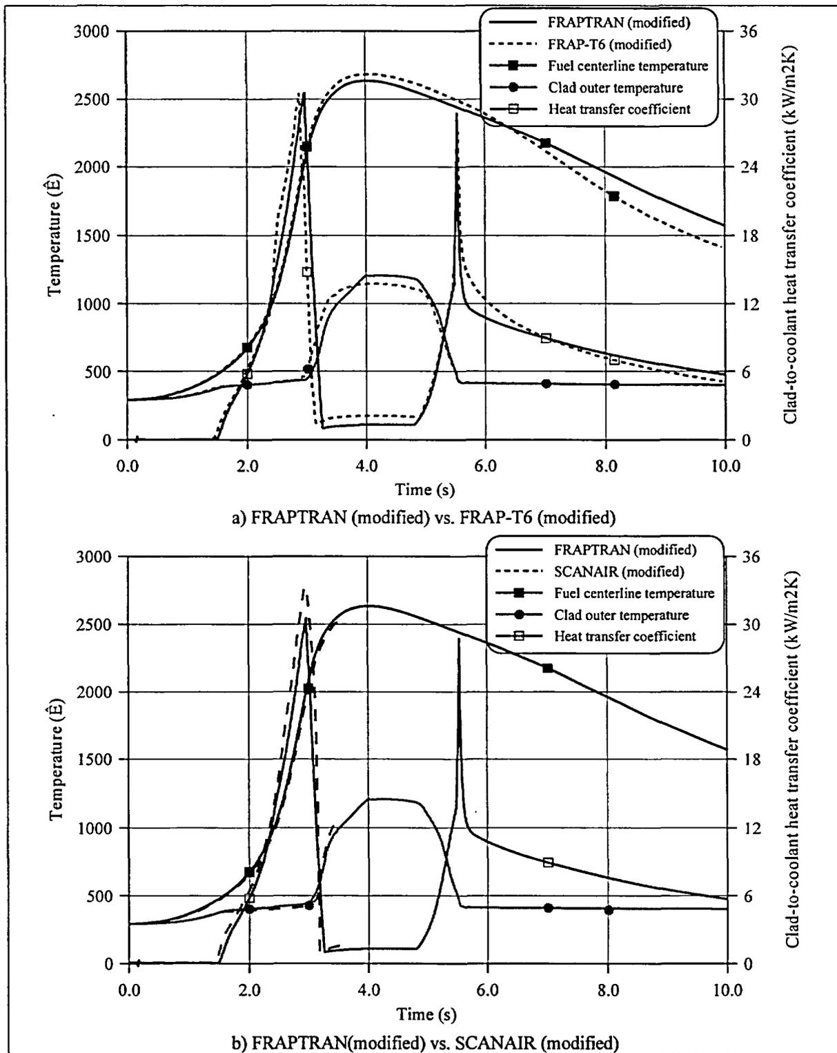
Fig. 19. Cladding temperatures and heat transfer coefficients vs. time calculated by modified FRAP-T6, SCANAIR and FRAPTRAN codes (HIT test case).
