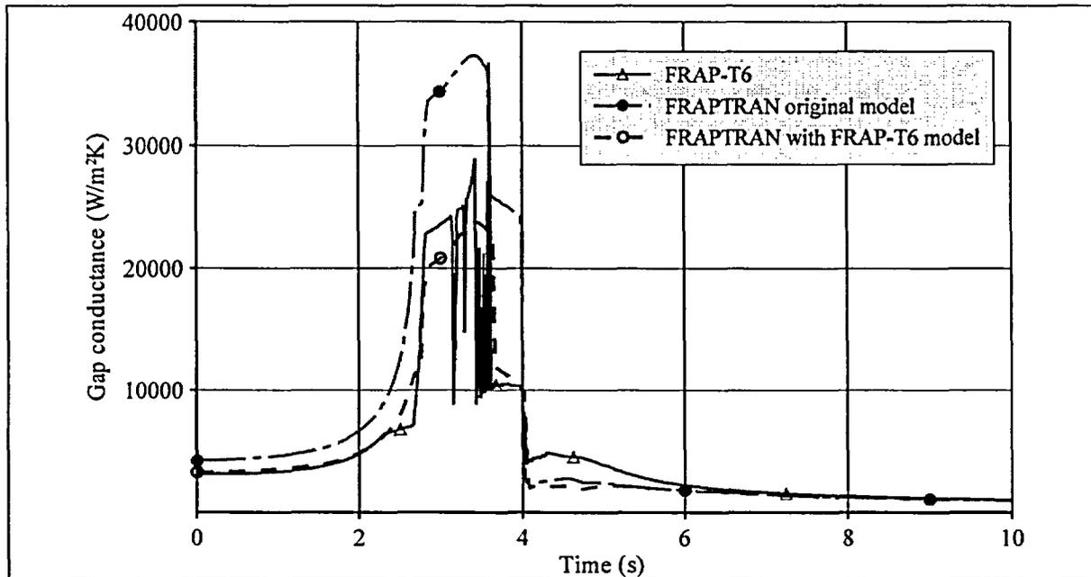
Fig. 22. Comparison of gap thermal conductivity models from FRAP-T6 (modified) and FRAPTRAN (modified) and FRAPTRAN (original).
