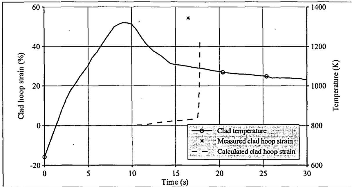
Fig. 29. Comparison of calculated and experimental values of cladding residual strain.
