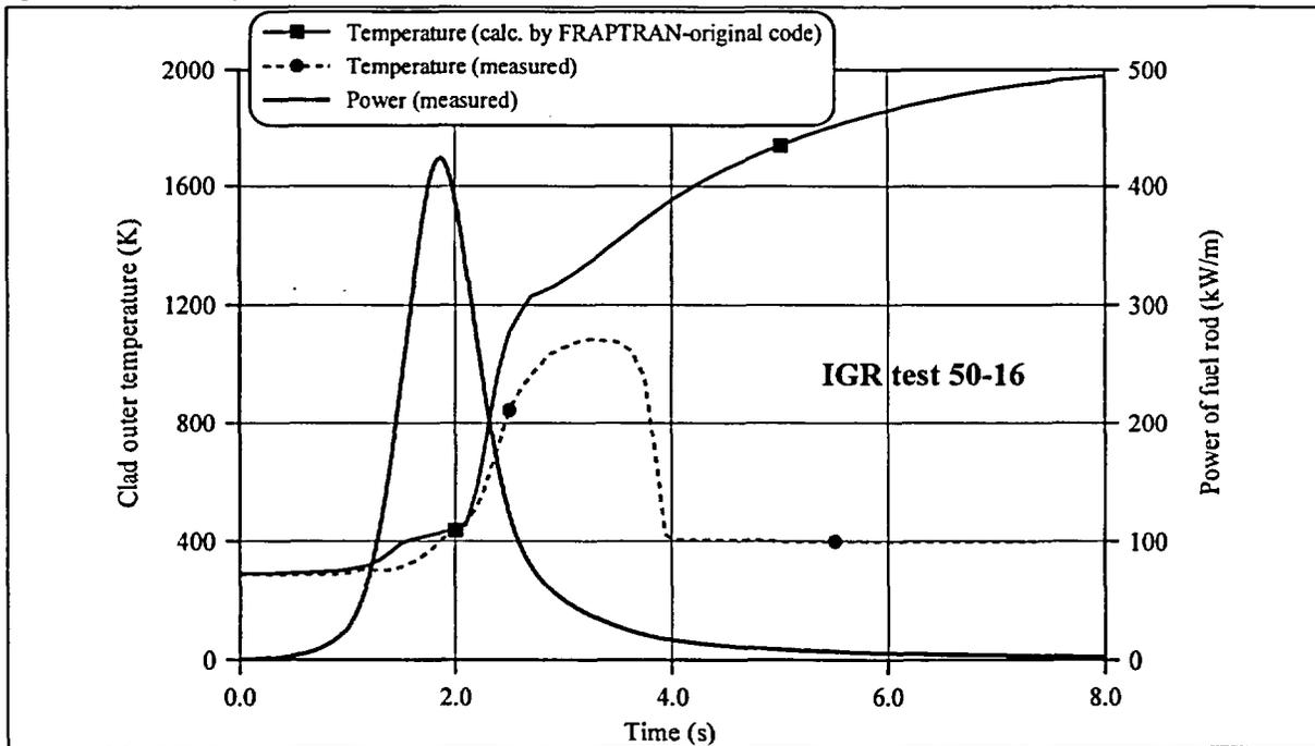
Fig. 5. Clad outer temperature in 50F-16 test: comparison between measured and calculated with original FRAPTRAN code.
