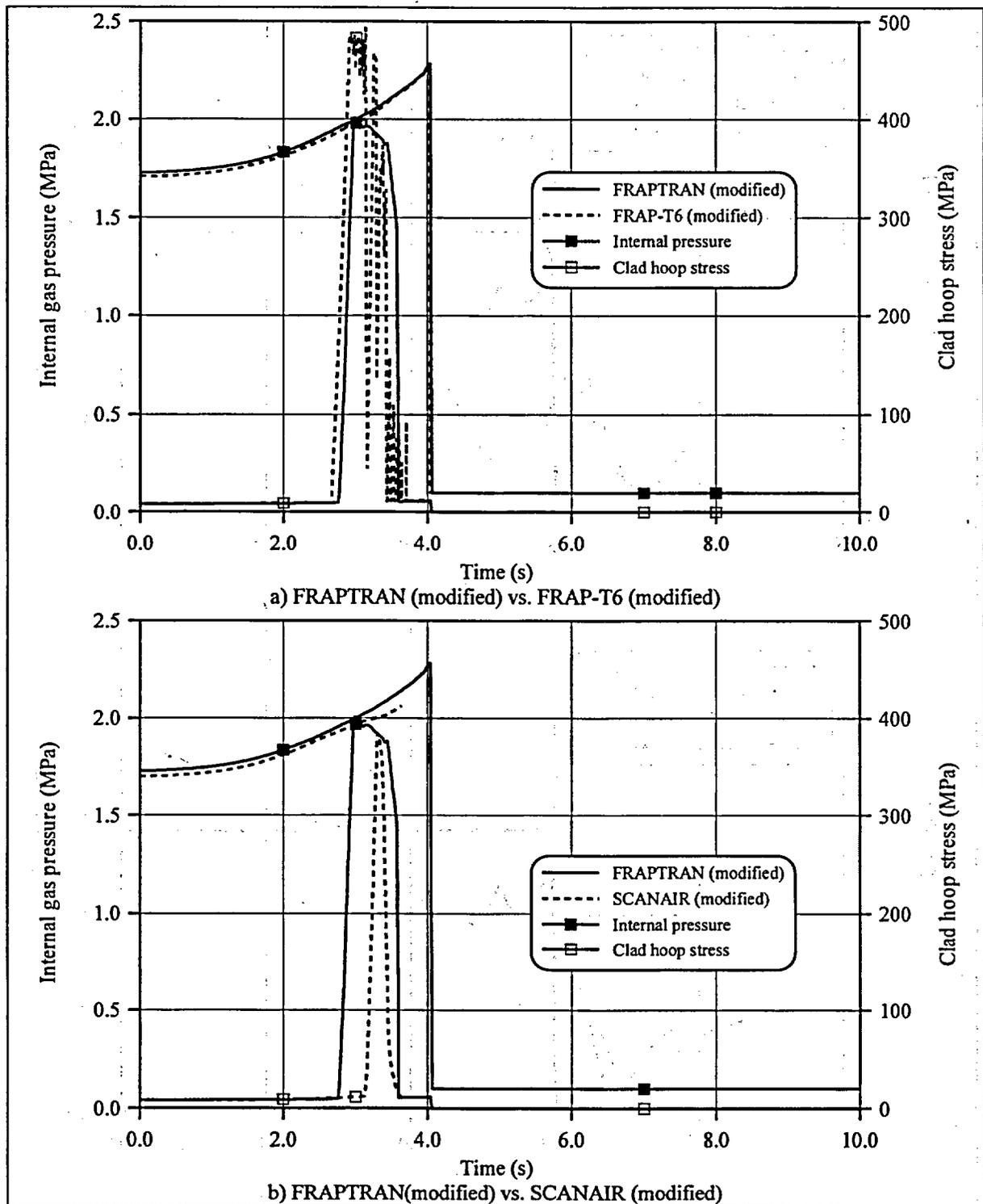
Fig. 12. Cladding hoop stresses and internal pressures vs. time calculated by modified FRAP-T6, SCANAIR and FRAPTRAN codes (H5T test case).
