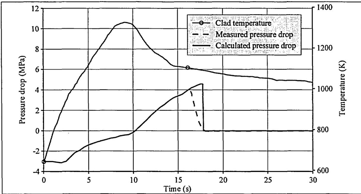
Fig. 28. Comparison of calculated and experimental values of failure pressure and temperature.
