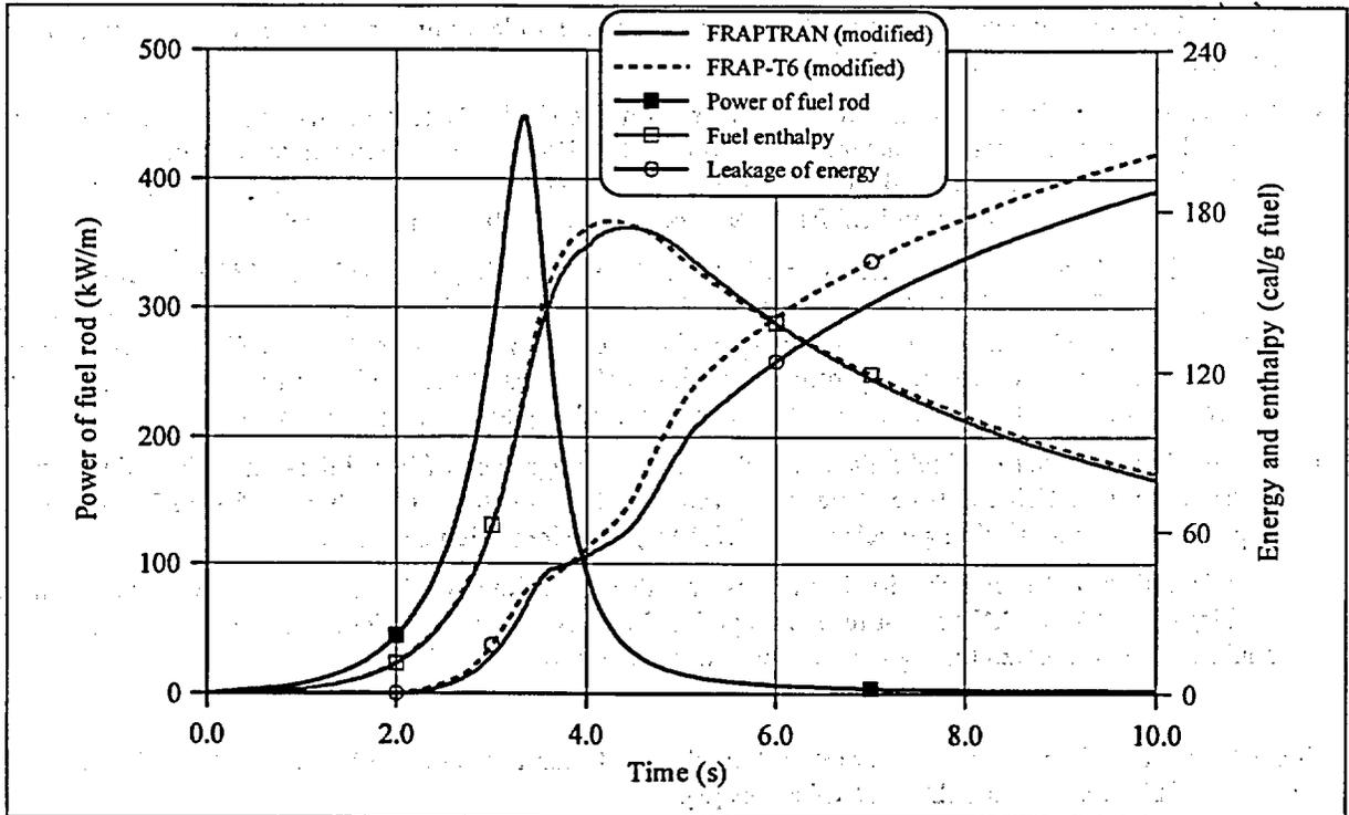
Fig. 24. Peak enthalpy calculated by FRAP-T6 (modified) and FRAPTRAN (modified) with gap thermal conductivity model from FRAP-T6 (modified).
