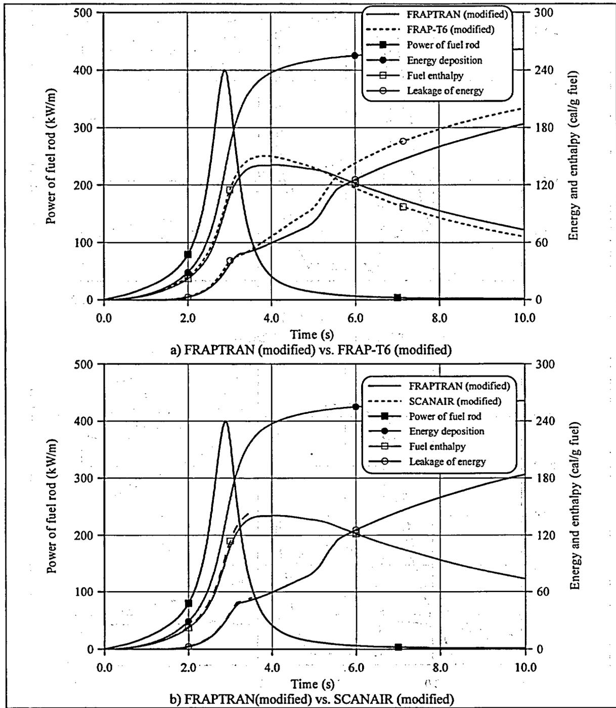
Fig. 18. Energy characteristics vs. time calculated by modified FRAP-T6, SCANAIR and FRAPTRAN codes (HIT test case).
