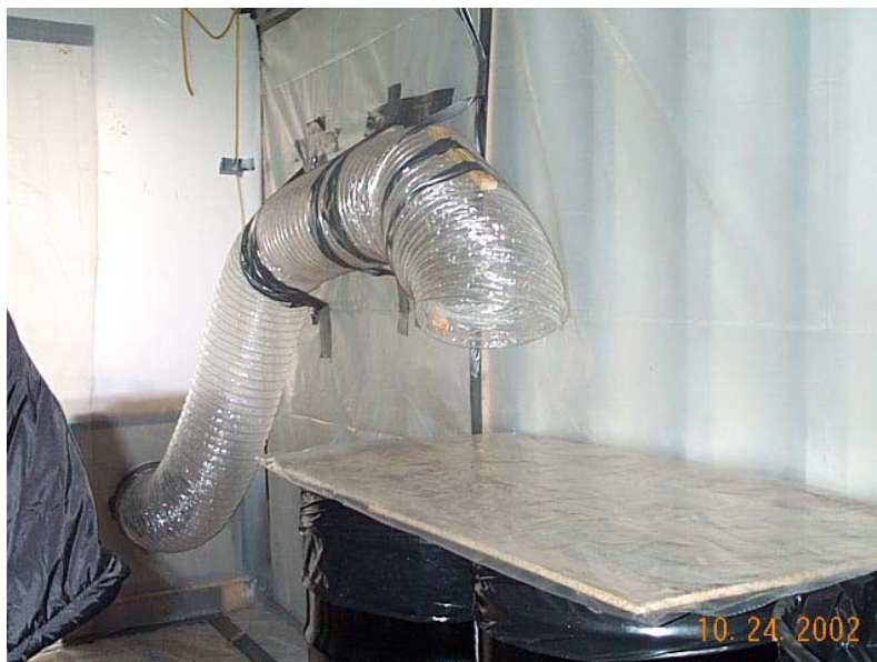
Figure 3-3: Sorting/segregation tent with exhaust system
