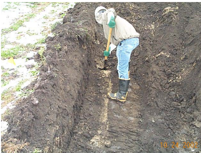
Figure 3-4: Photo showing backfill line in Pit 1. The soil to the right of the yellow line(clay) indicates the pit location.
