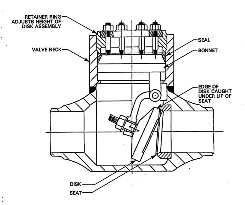
Figure 1. CHECK VALVE SHOWN WITH DISK JAMMED IN OPEN POSITION
