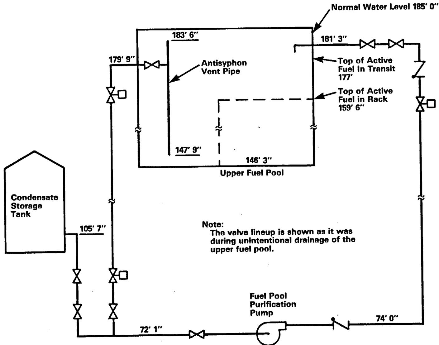
Figure 1. Simplified Flow Path Diagram of Upper Pool Purification System at River Bend.
