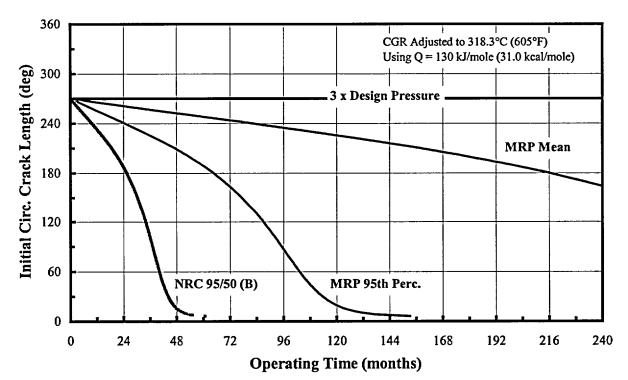
Calculated Remaining Operating Time for a Circumferential Crack to Grow to the 3× Limit Load Condition at the Maximum U.S. Head Temp of 605°F
