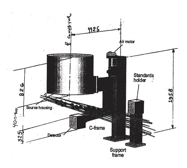
SCHEMATIC OF MODEL CM100 (The dimensions are in millimeters)
