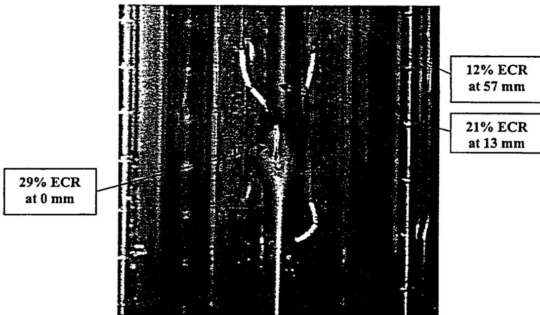
Fig. 8a. OCL#3 test specimen after 10 minutes in steam at 1204°C, 3°C/s cool-down to 800°C and water quench initiated at 800°C.
